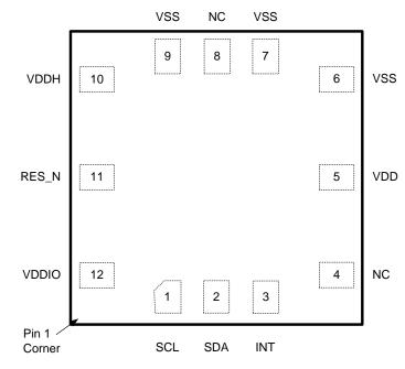
Figure 3. Pin Assignments – Top View
