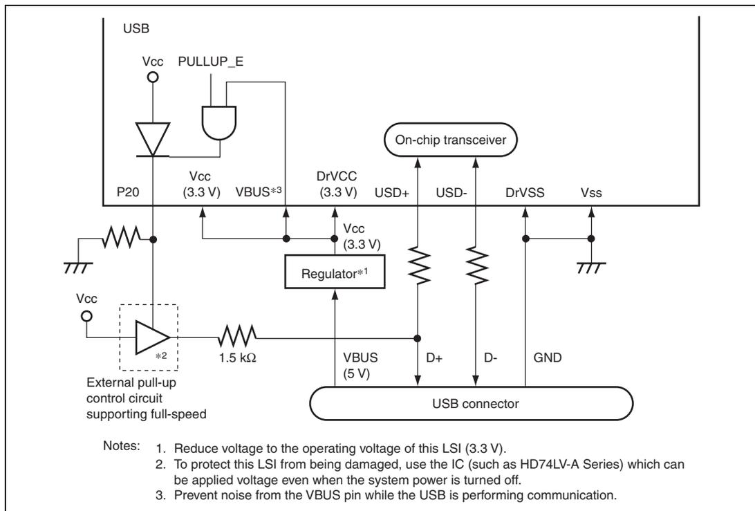
**Figure 16.23 Example of Circuitry in Bus Power Mode**
