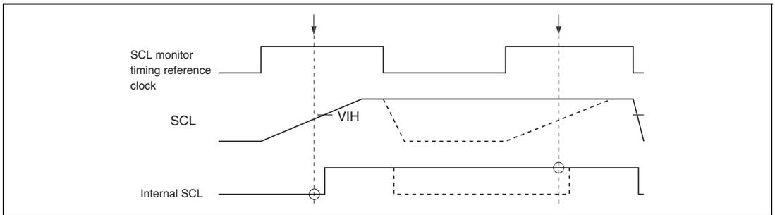
**Figure 17.18 Timing of the Bit Synchronous Circuit**
