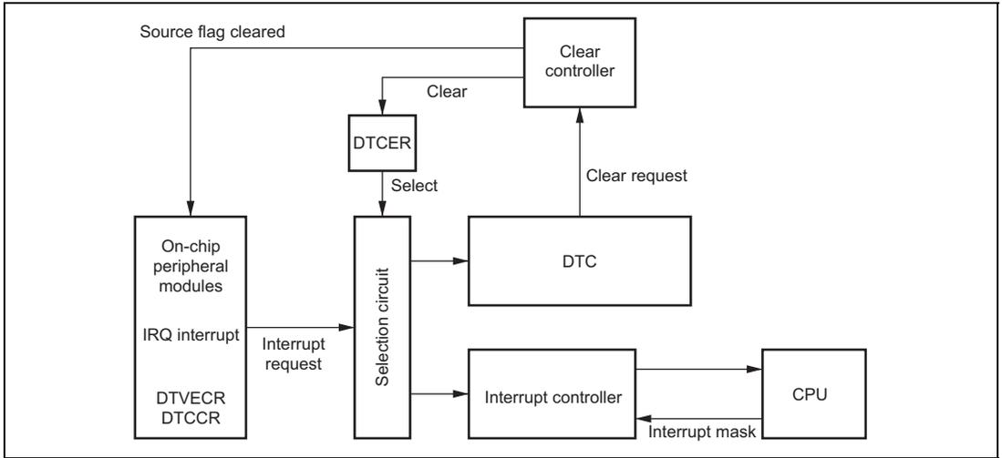
**Figure 9.2 Block Diagram of DTC Activation Source Control**
