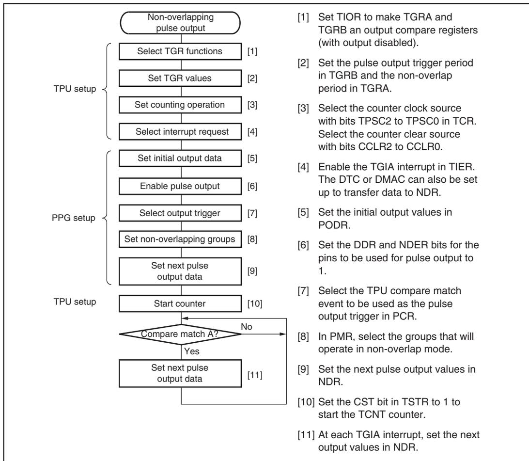
**Figure 12.8 Setup Procedure for Non-Overlapping Pulse Output (Example)**
