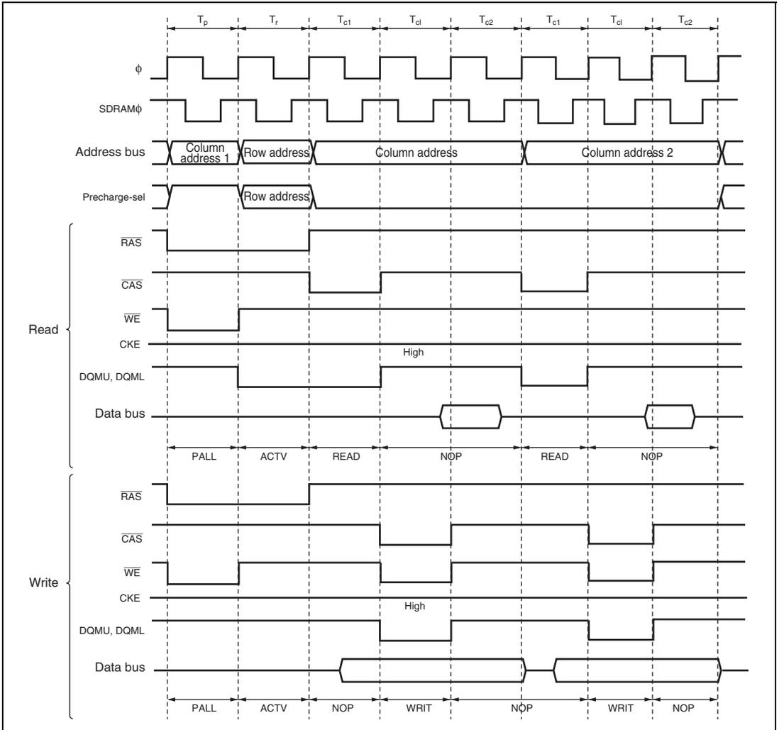
**Figure 6.64 Operation Timing of Burst Access**
