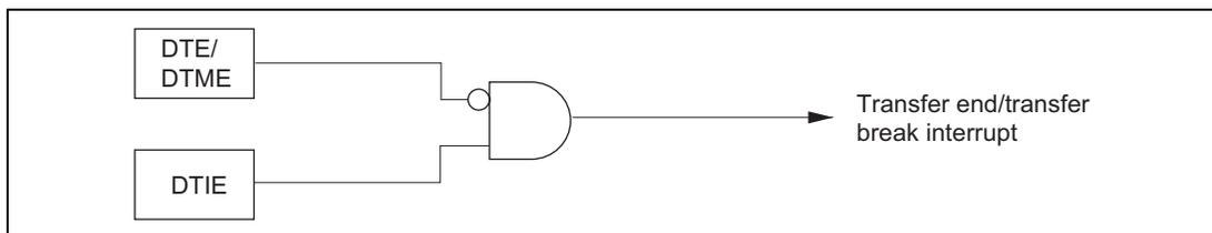
**Figure 7.38 Block Diagram of Transfer End/Transfer Break Interrupt**
