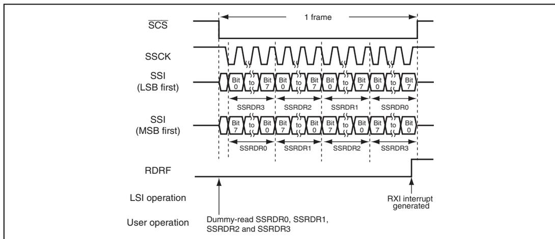
**Figure 20.7 Example of Reception Operation (SSU Mode)**
