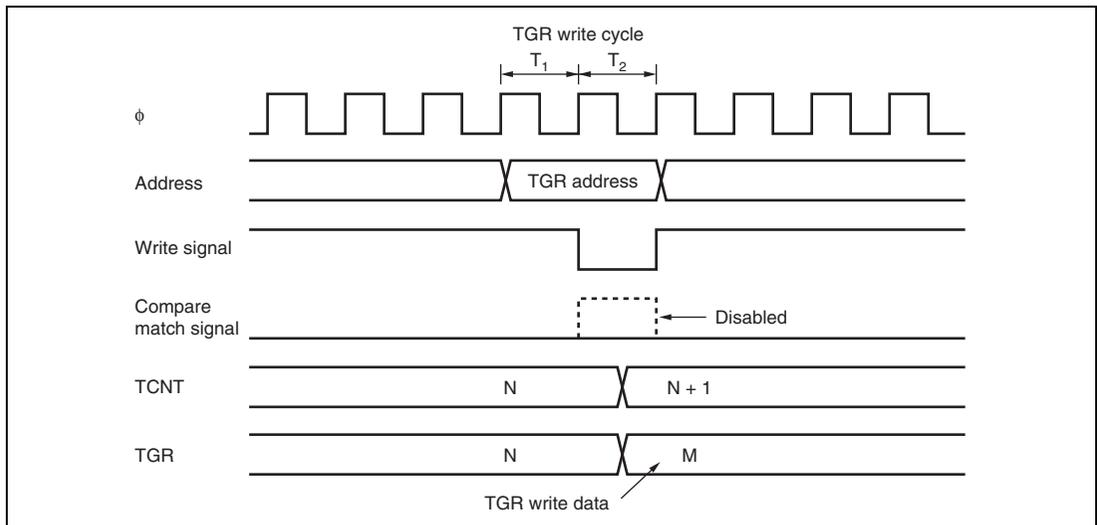
**Figure 11.48 Contention between TGR Write and Compare Match**
