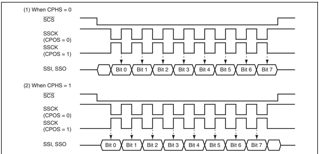
**Figure 20.2 Relationship of Clock Phase, Polarity, and Data**
