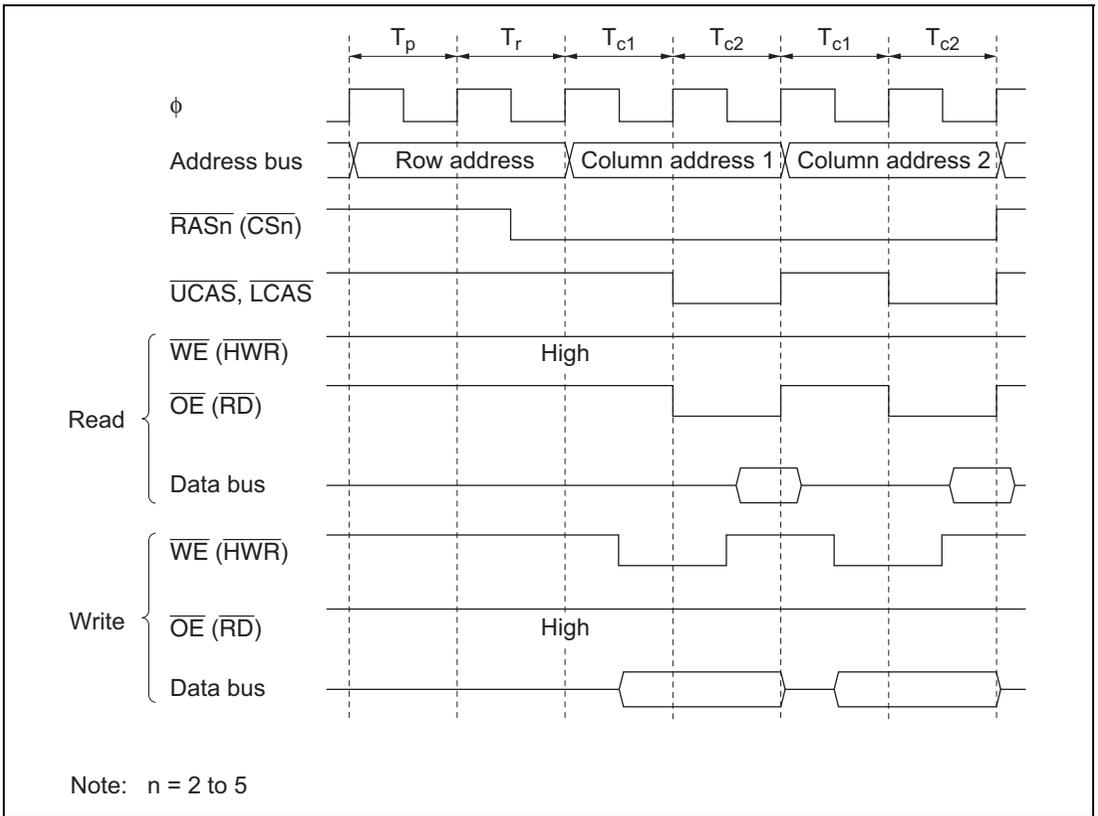
**Figure 6.42 Operation Timing in Fast Page Mode
