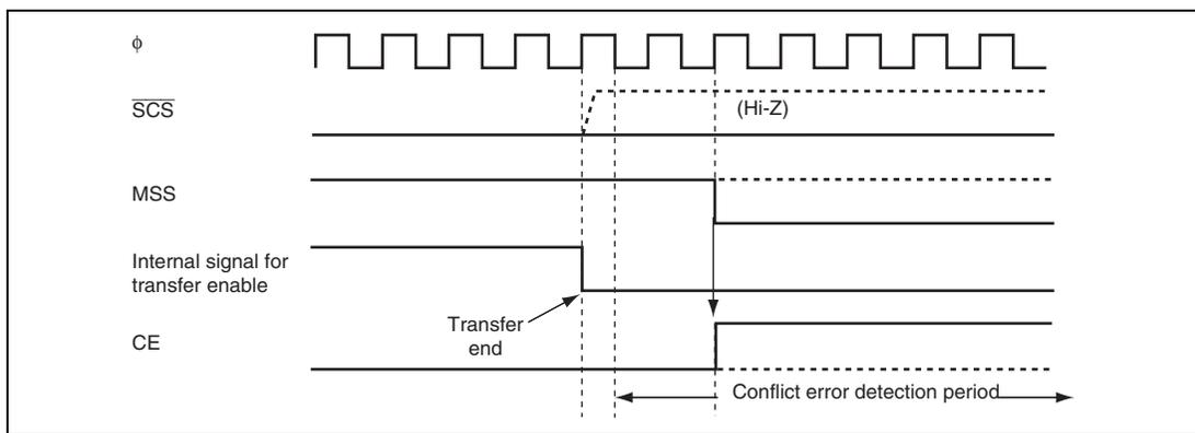
**Figure 20.11 Conflict Error Detection Timing (After Transfer End)**
