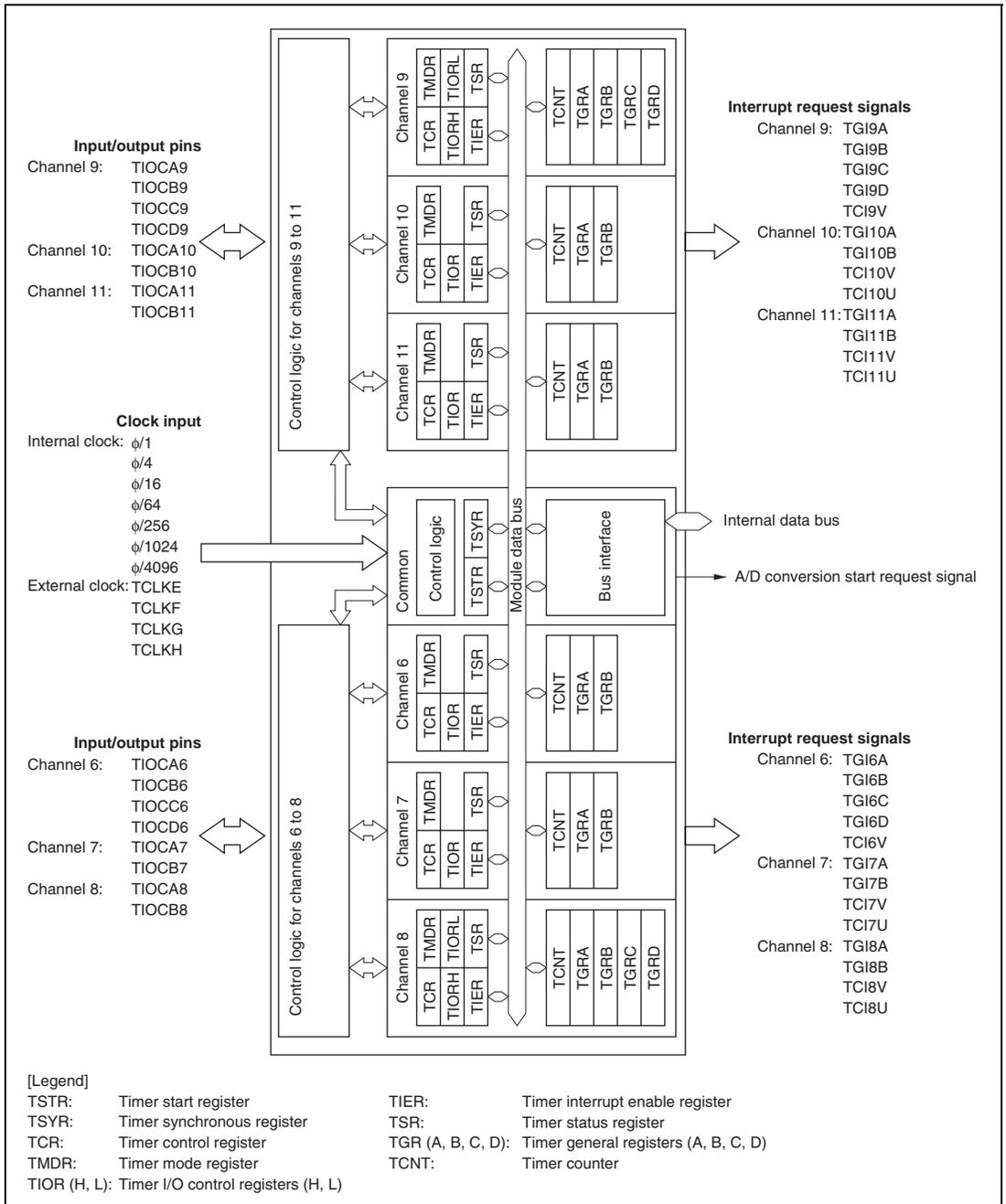
**Figure 11.2 Block Diagram of TPU (Unit 1)**
