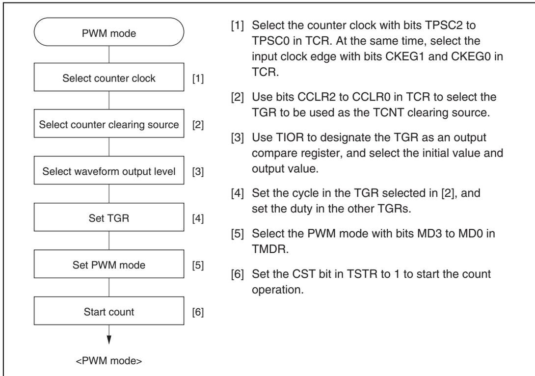
**Figure 11.21 Example of PWM Mode Setting Procedure**
