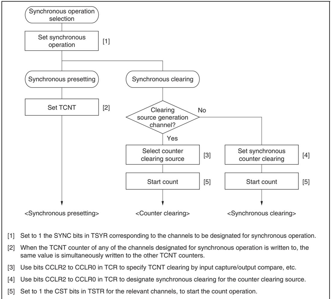
**Figure 11.11 Example of Synchronous Operation Setting Procedure**
