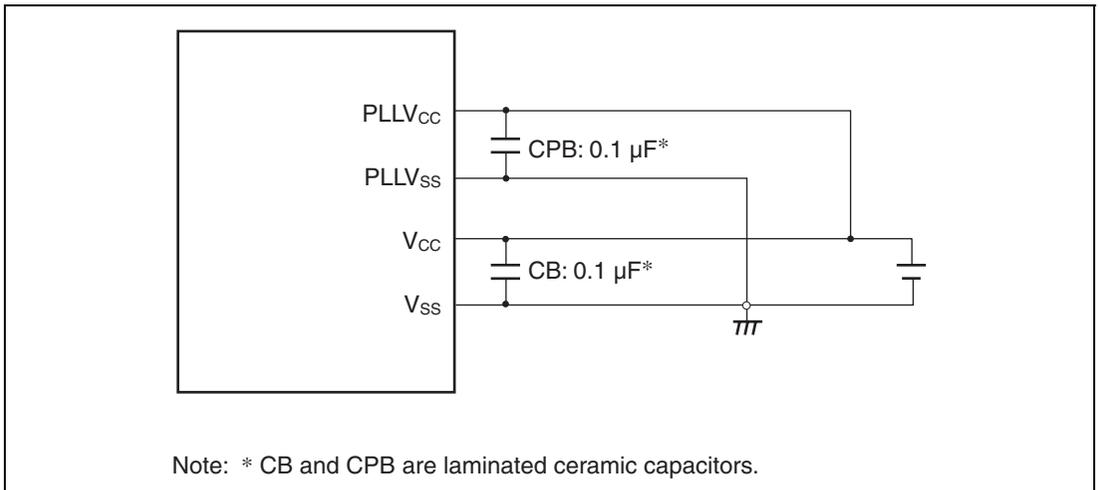
**Figure 23.7 Recommended External Circuitry for PLL Circuit**
