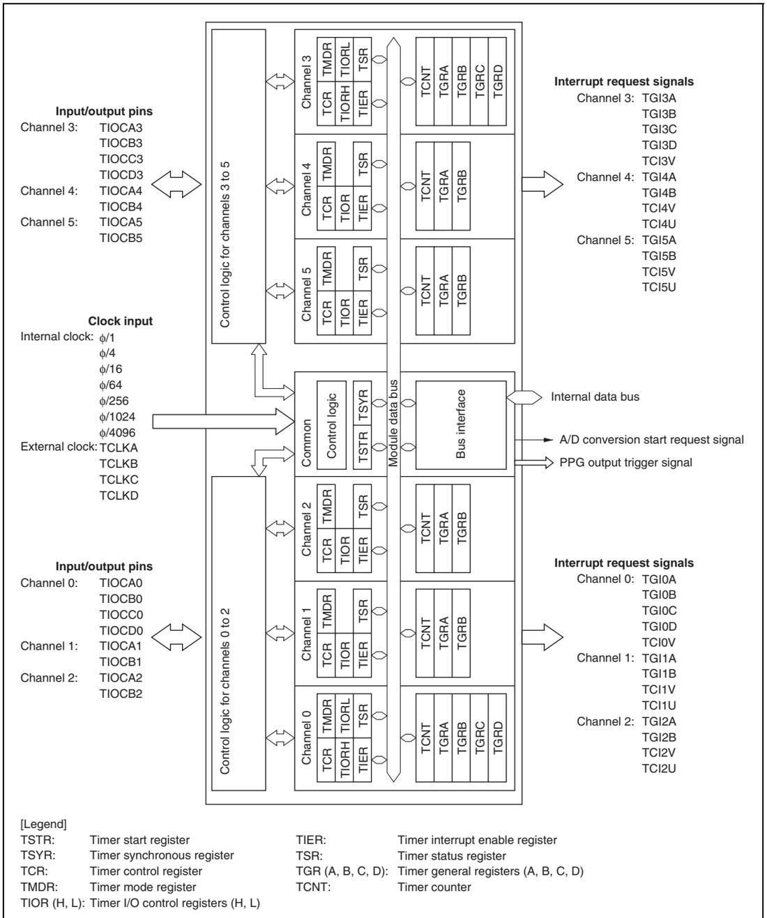
**Figure 11.1 Block Diagram of TPU (Unit 0)**
