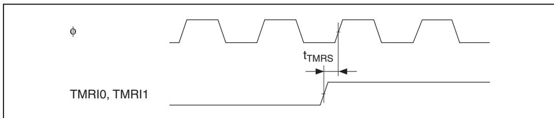
**Figure 26.45 8-Bit Timer Reset Input Timing**
