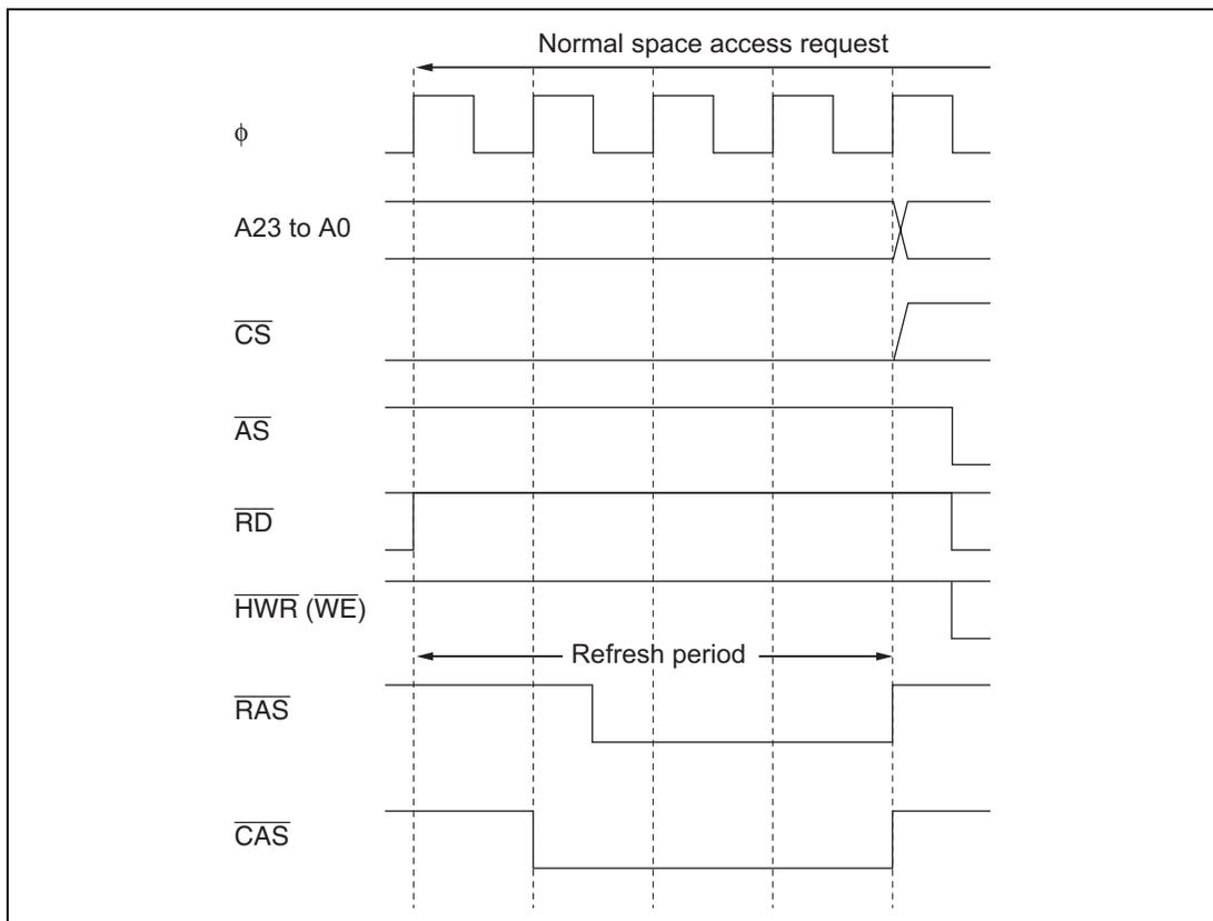
**Figure 6.50 Example of CBR Refresh Timing (CBRM = 1)**
