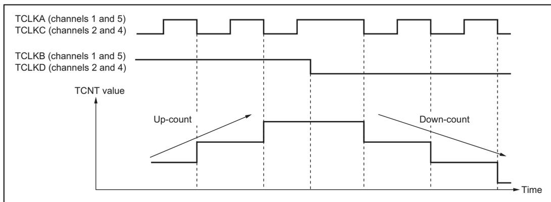
**Figure 11.27 Example of Phase Counting Mode 2 Operation**
