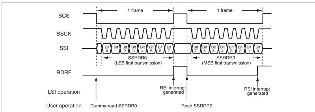
**Figure 20.7 (1) Example of Reception Operation (SSU Mode)**
