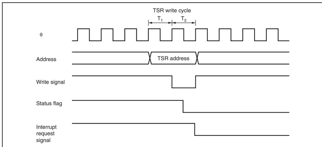
**Figure 11.43 Timing for Status Flag Clearing by CPU**
