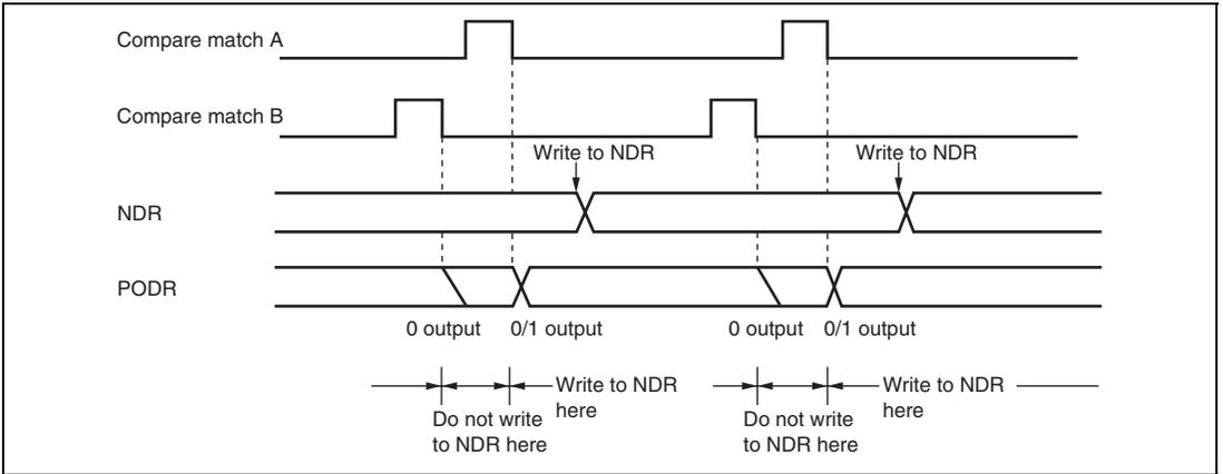
**Figure 12.7 Non-Overlapping Operation and NDR Write Timing**
