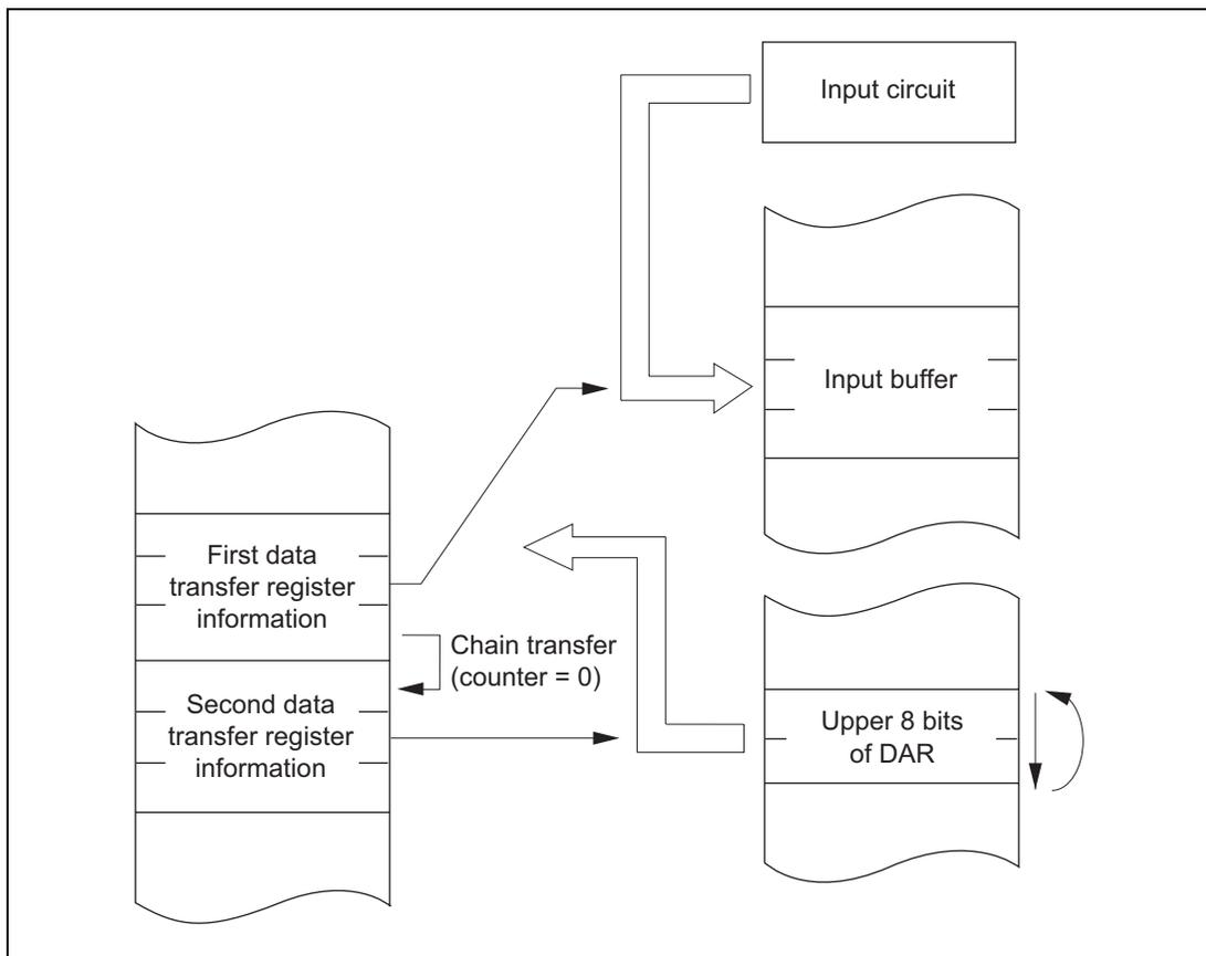
**Figure 9.13 Chain Transfer when Counter = 0**
