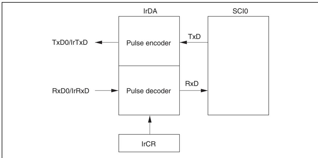
**Figure 15.33 Block Diagram of IrDA**
