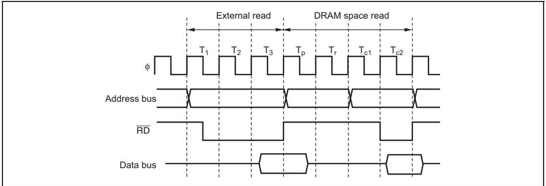
**Figure 6.81 Example of DRAM Full Access after External Read
