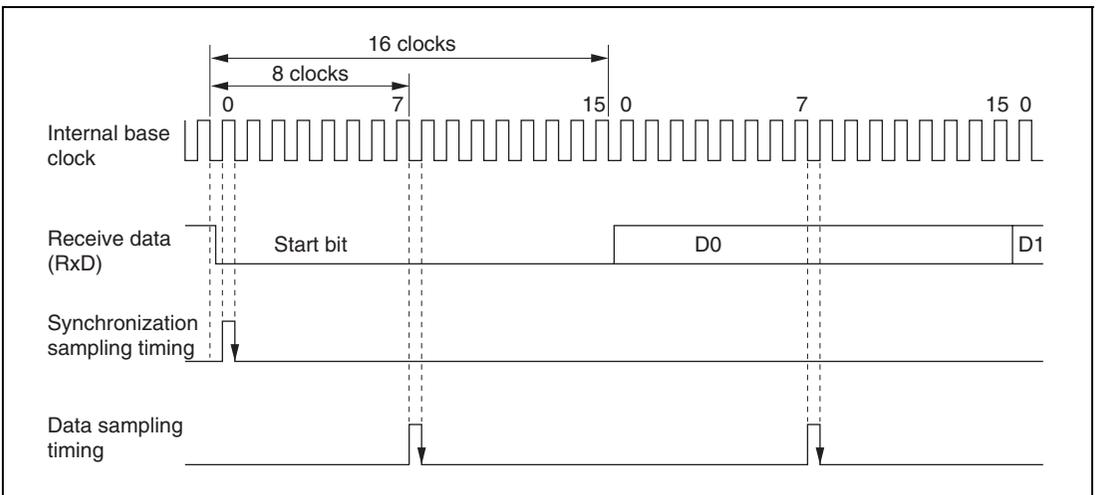
**Figure 15.3 Receive Data Sampling Timing in Asynchronous Mode**
