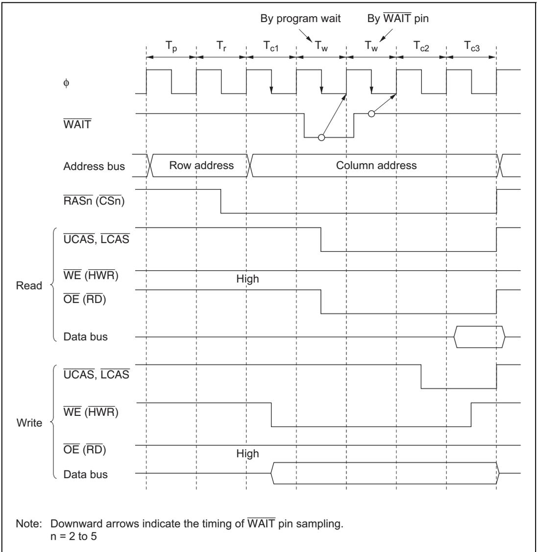
**Figure 6.39 Example of Wait State Insertion Timing
