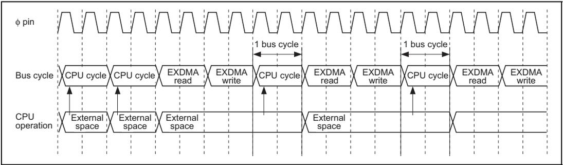
**Figure 8.32 Auto Request/Burst Mode/Normal Transfer Mode
