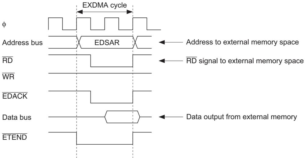
Transfer from external device with DACK to external memory
