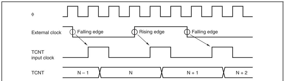
**Figure 11.32 Count Timing in External Clock Operation**
