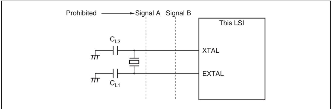
**Figure 23.6 Note on Board Design for Oscillation Circuit**
