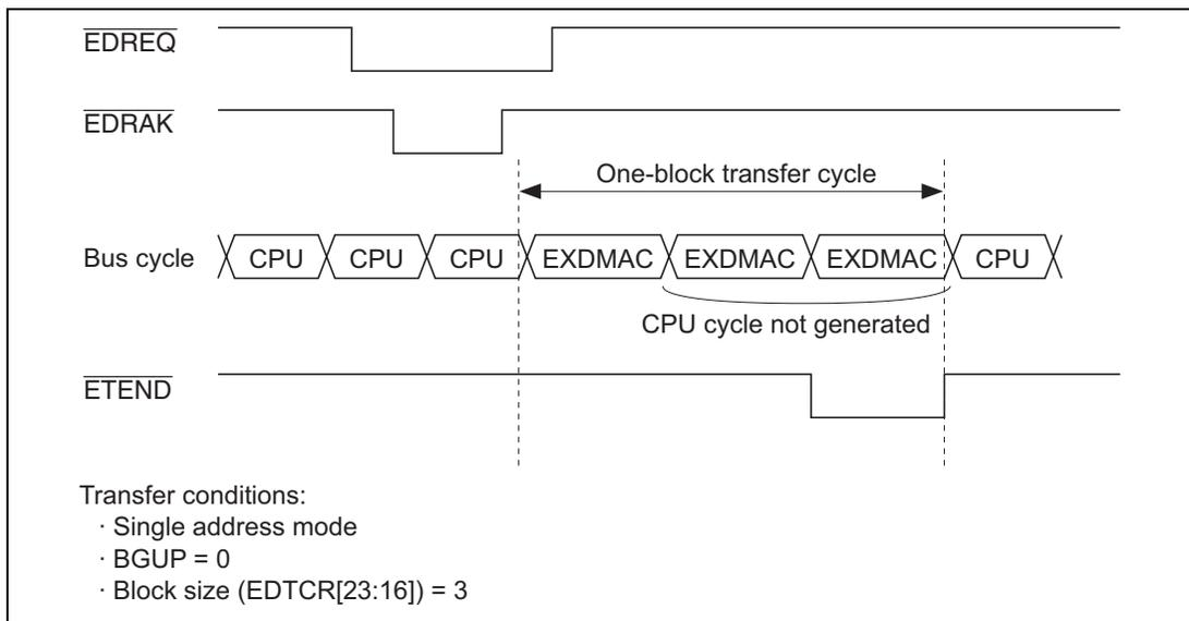
**Figure 8.8 Example of Timing in Block Transfer Mode**
