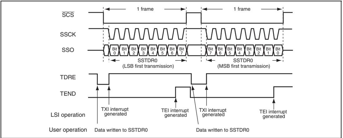
**Figure 20.5 (1) Example of Transmission Operation (SSU Mode)**
