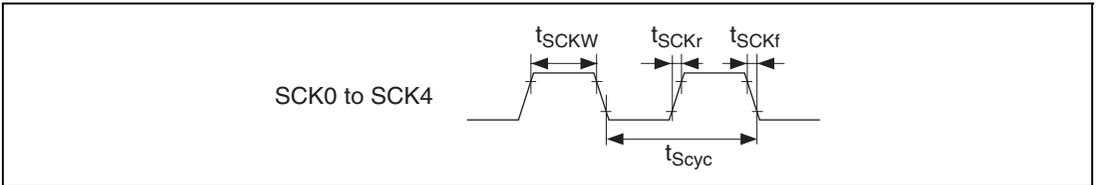
**Figure 26.47 SCK Clock Input Timing**
