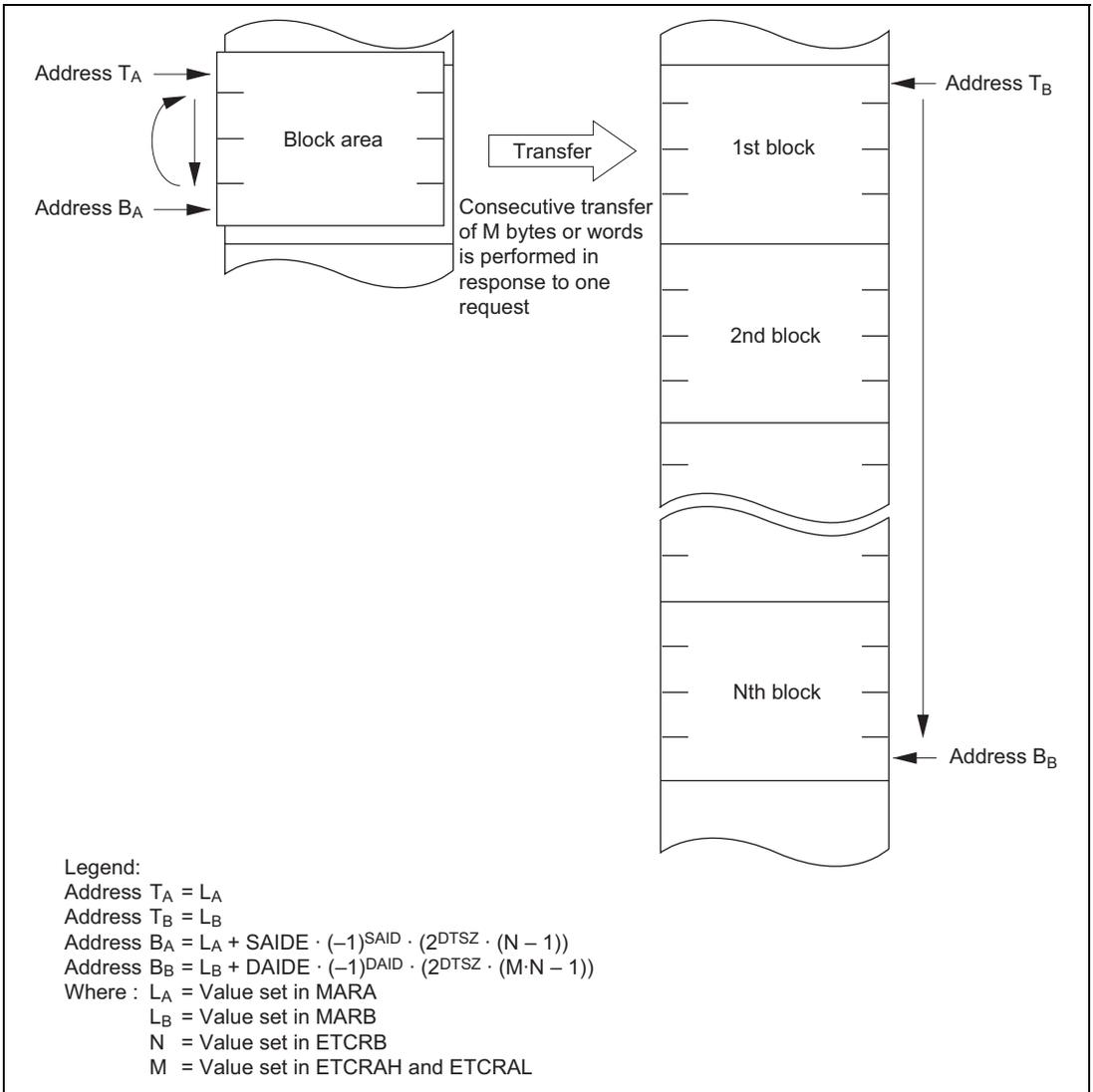
**Figure 7.14 Operation in Block Transfer Mode (BLKDIR = 1)**
