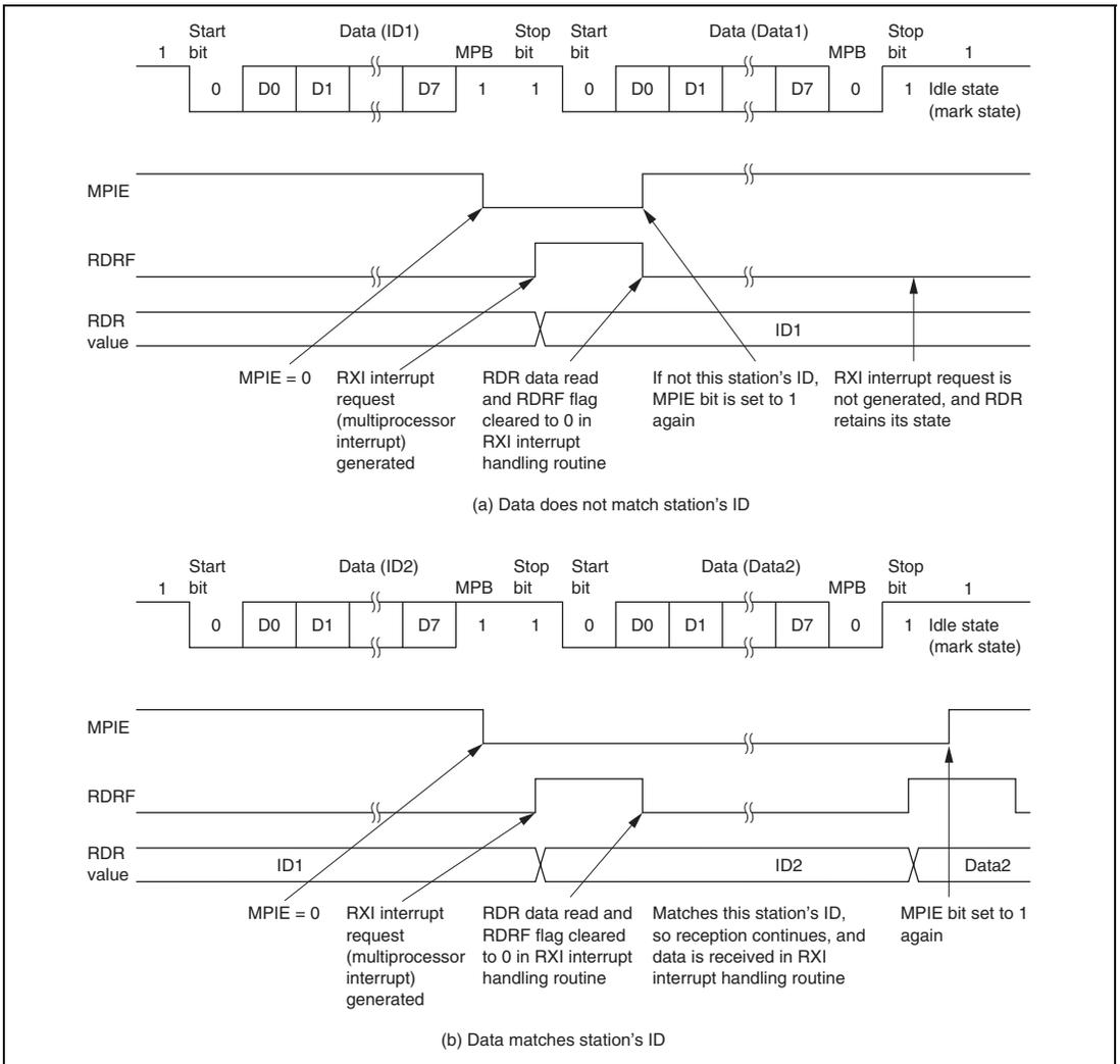
**Figure 15.12 Example of SCI Operation in Reception
