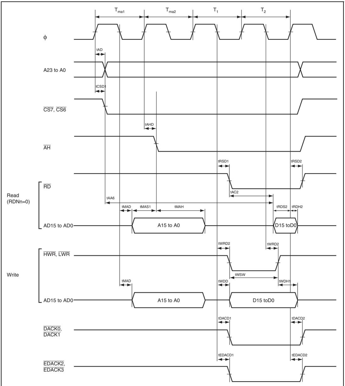
Figure 26.29 Multiplexed Bus Timing: Data Two-State Access
