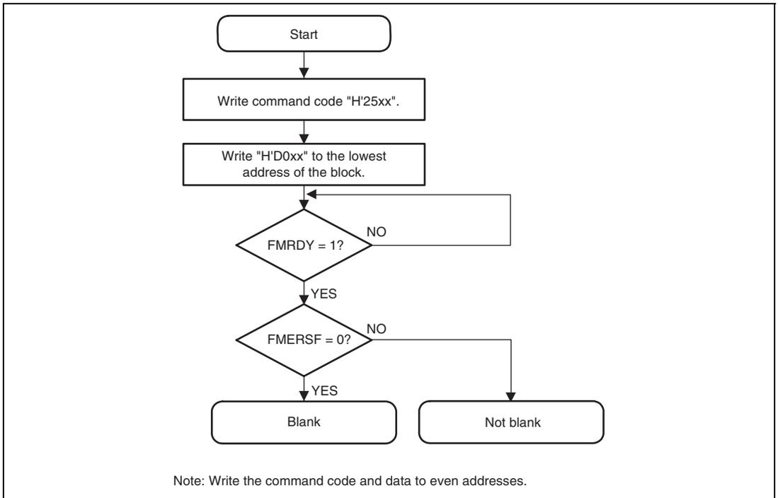
**Figure 22.5 Flowchart of Block Blank Check Command Processing**
