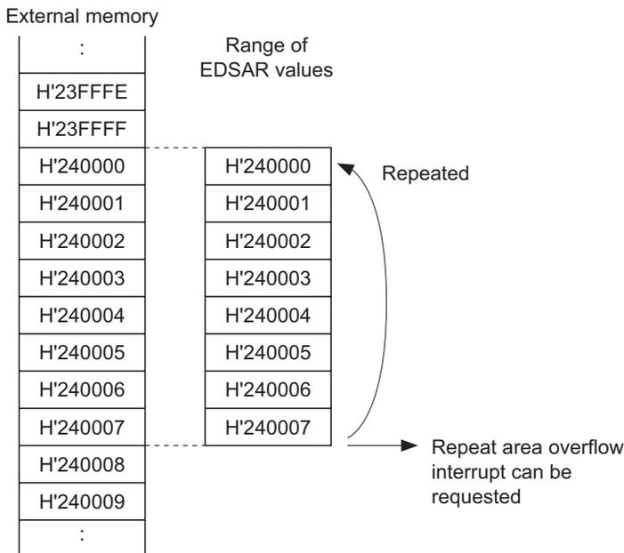
**Figure 8.9 Example of Repeat Area Function Operation**
