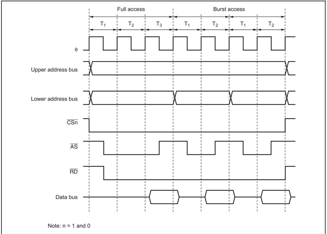
**Figure 6.75 Example of Burst ROM Access Timing
