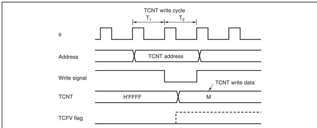
**Figure 11.54 Contention between TCNT Write and Overflow**
