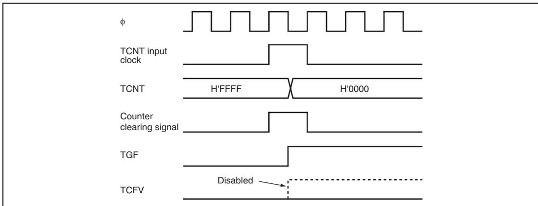
**Figure 11.53 Contention between Overflow and Counter Clearing**
