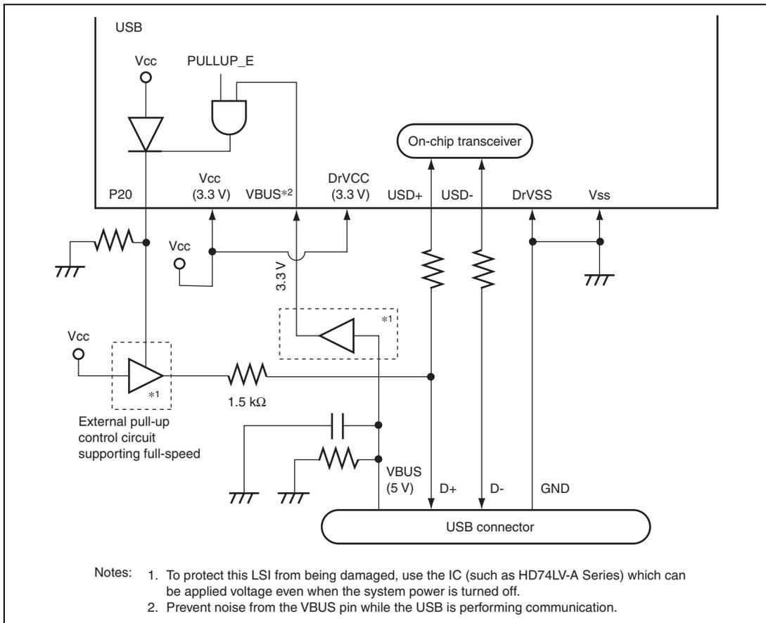
**Figure 16.24 Example of Circuitry in Self Power Mode**
