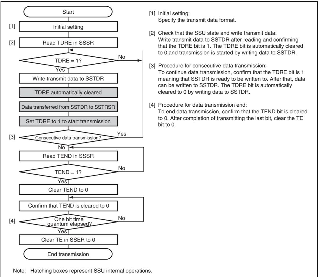
**Figure 20.6 Flowchart Example of Data Transmission (SSU Mode)**
