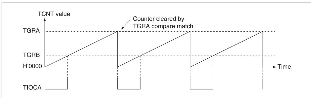
**Figure 11.22 Example of PWM Mode Operation (1)**
