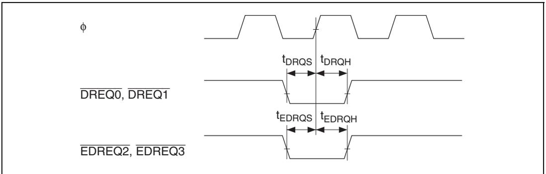
**Figure 26.34 DMAC and EXDMAC,  $\overline{DREQ}/\overline{EDREQ}$  Input Timing**
