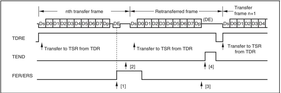
**Figure 15.26 Retransfer Operation in SCI Transmit Mode**
