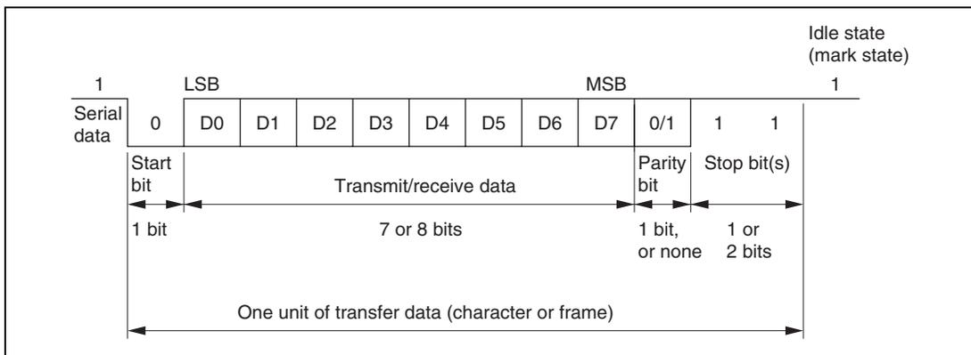
**Figure 15.2 Data Format in Asynchronous Communication
