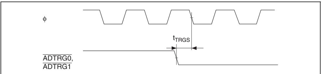
**Figure 26.49 A/D Converter External Trigger Input Timing**
