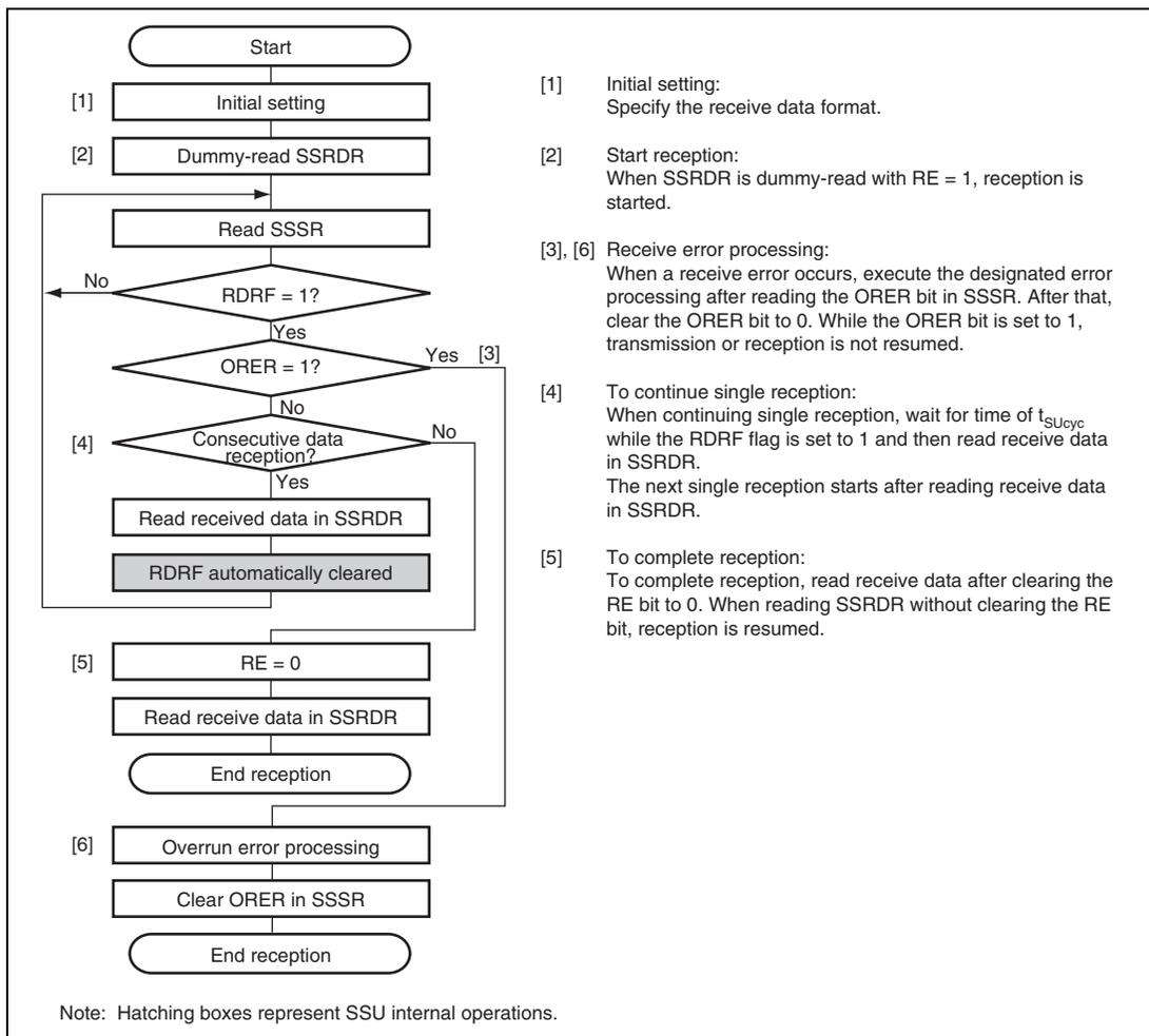
**Figure 20.8 Flowchart Example of Data Reception (SSU Mode)**
