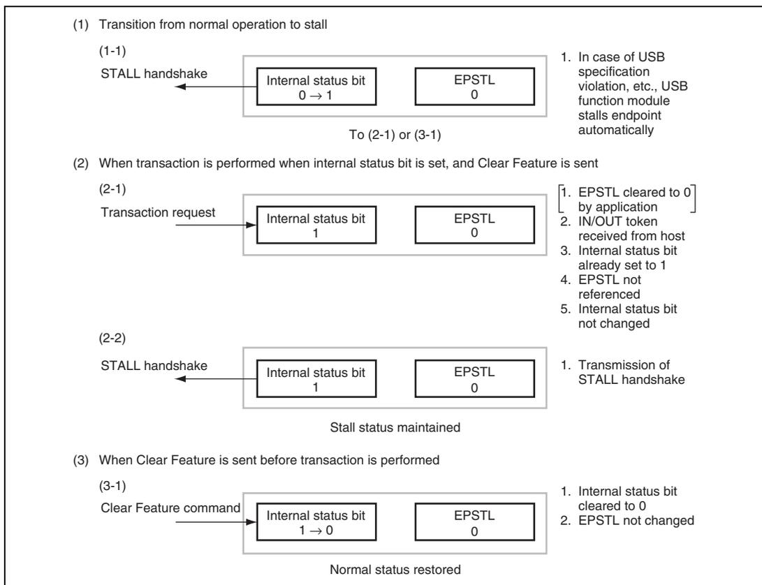
**Figure 16.20 Automatic Stall by USB Function Module**
