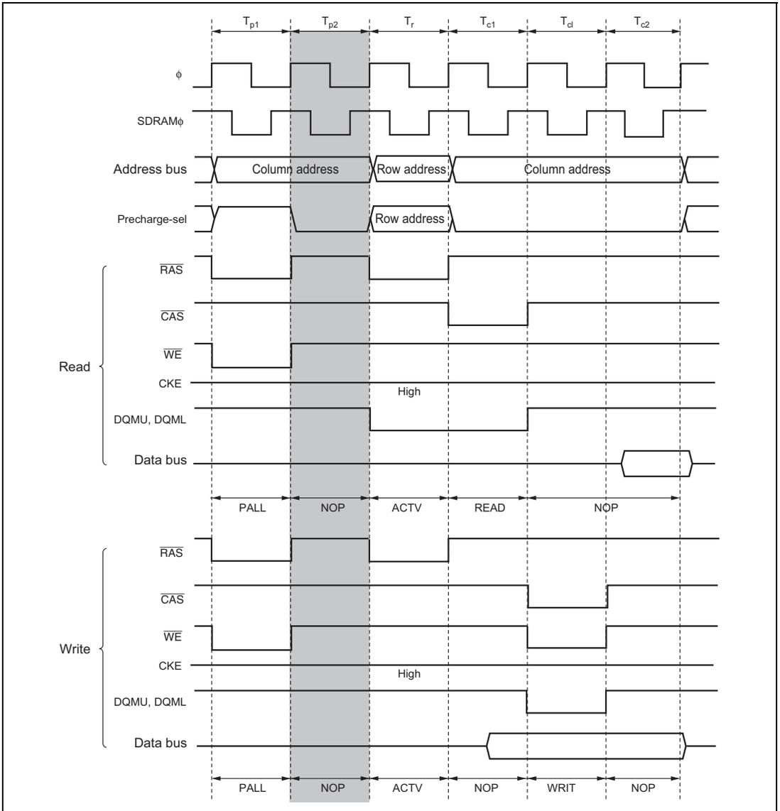
**Figure 6.59 Example of Timing with Two-State Precharge Cycle
