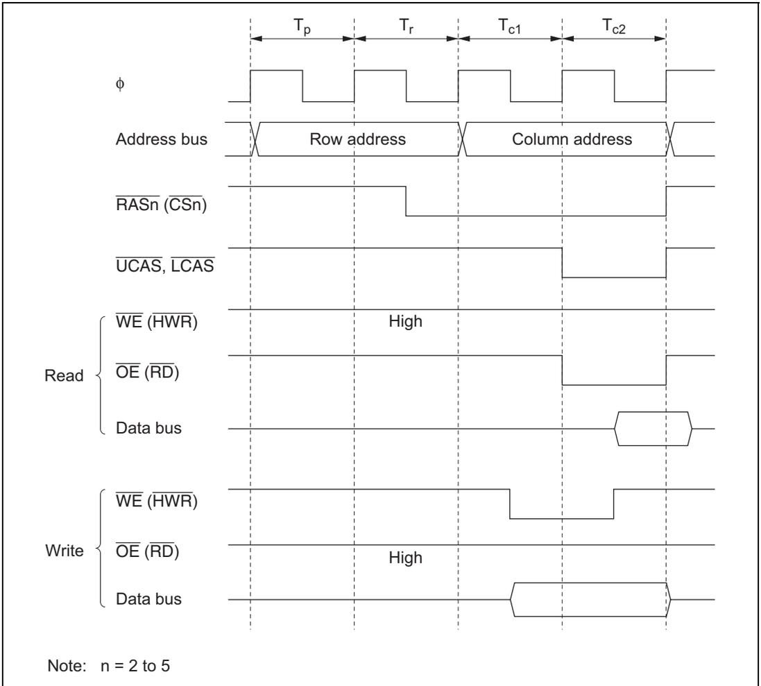
**Figure 6.33 DRAM Basic Access Timing (RAST = 0, CAST = 0)**
