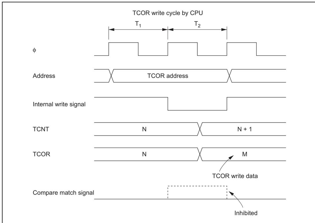
**Figure 13.13 Contention between TCOR Write and Compare Match**
