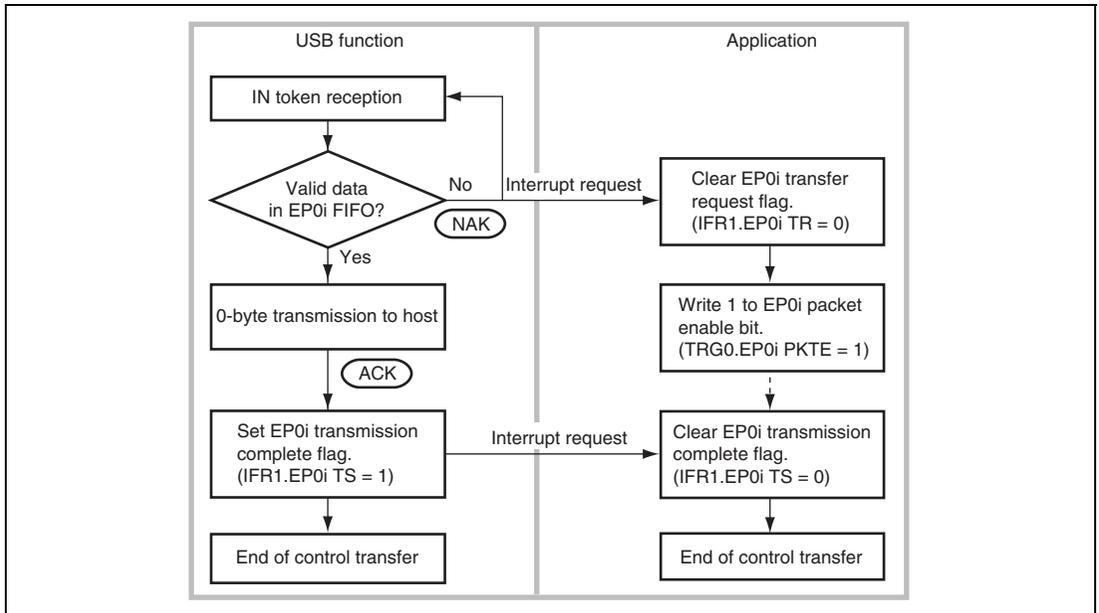
**Figure 16.15 Status Stage (Control-Out) Operation**
