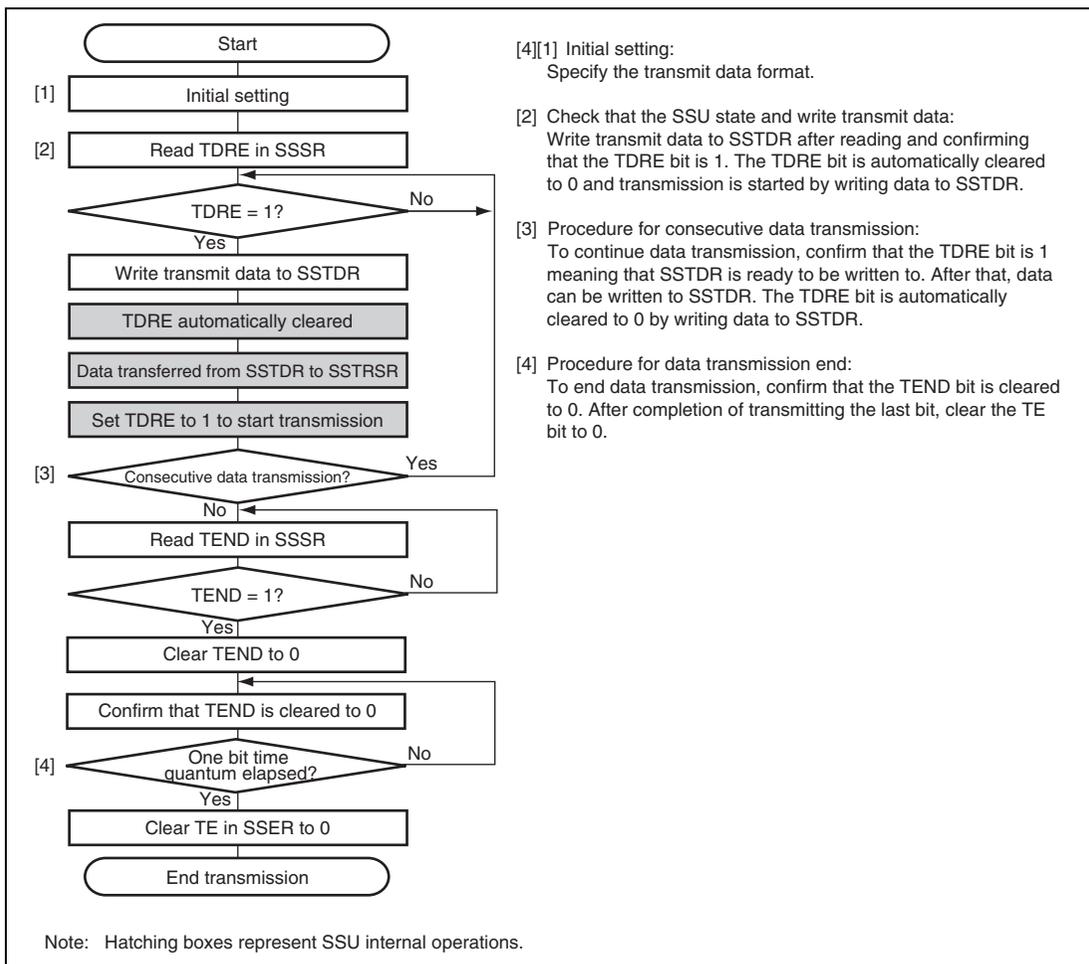
**Figure 20.14 Flowchart Example of Transmission Operation
