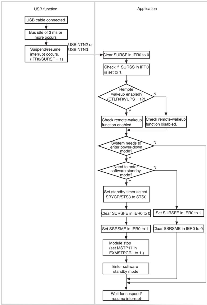
Figure 16.5 Suspend Operation
