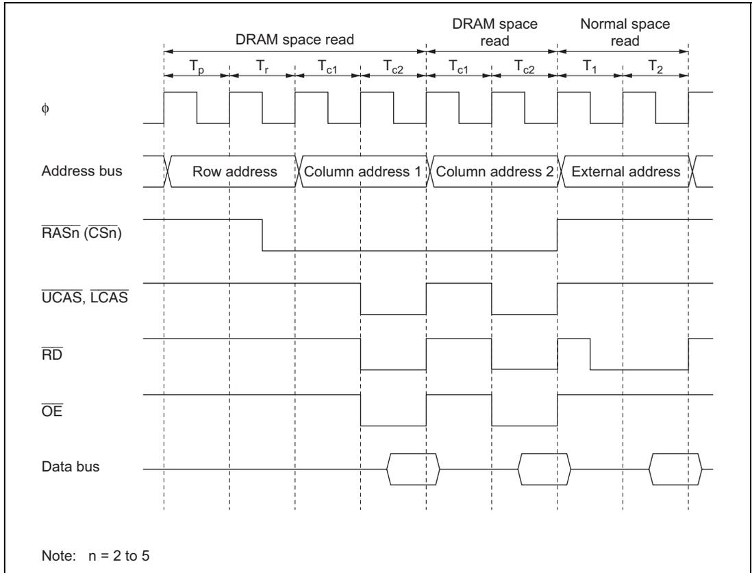
**Figure 6.45 Example of Operation Timing in RAS Up Mode
