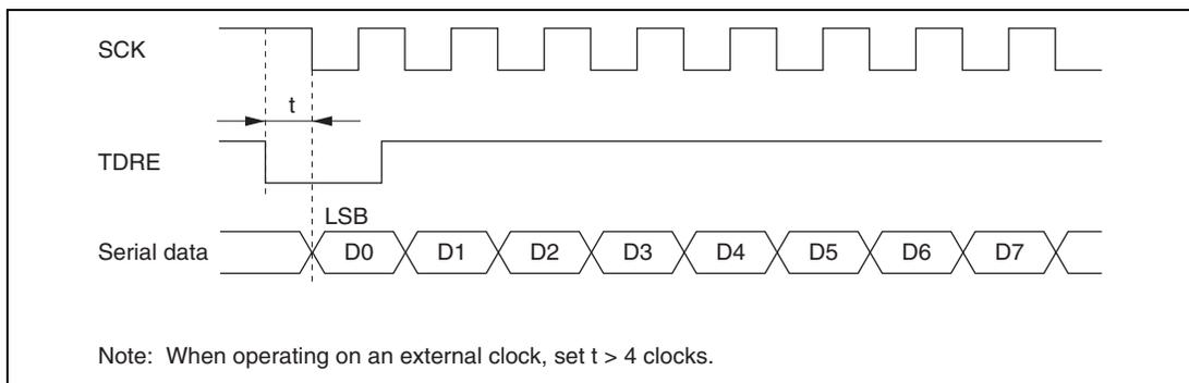
**Figure 15.35 Example of Synchronous Transmission Using DTC**
