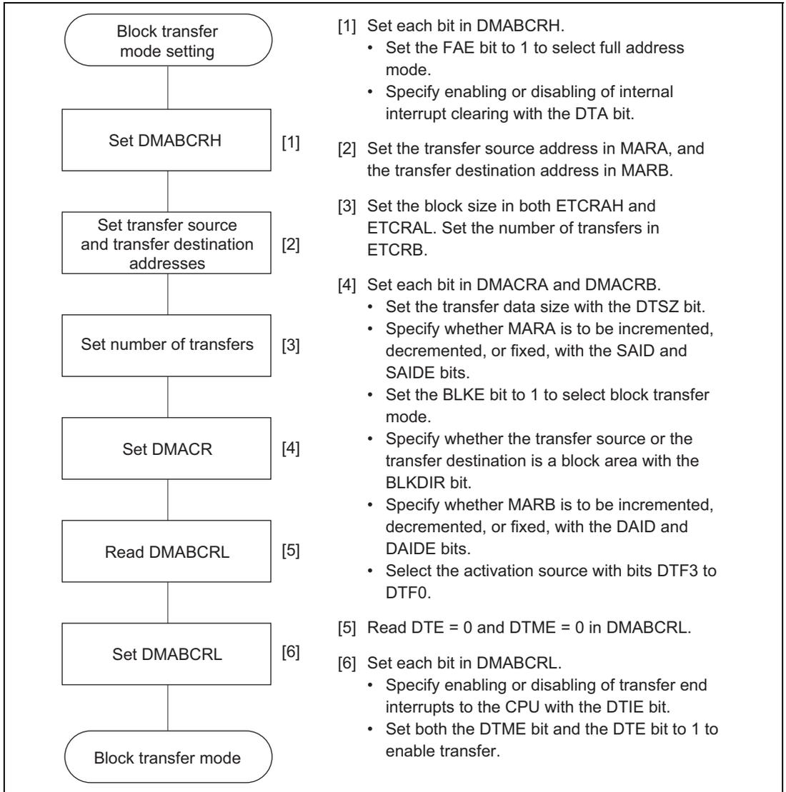
**Figure 7.16 Example of Block Transfer Mode Setting Procedure**
