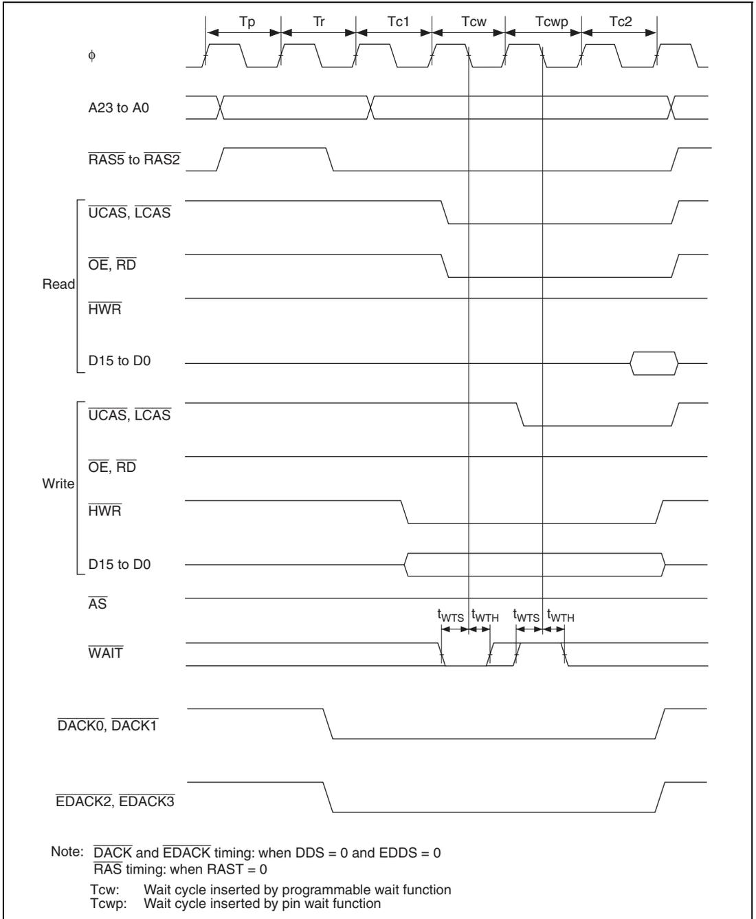
Figure 26.16 DRAM Access Timing: Two-State Access, One Wait
