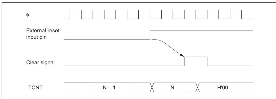
**Figure 13.9** Timing of Clearance by External Reset
