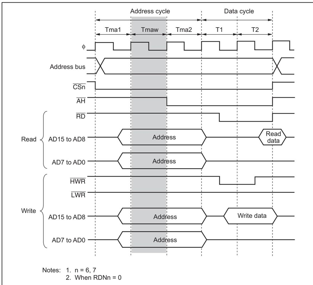
**Figure 6.29 Example of Access Timing with Address Wait**
