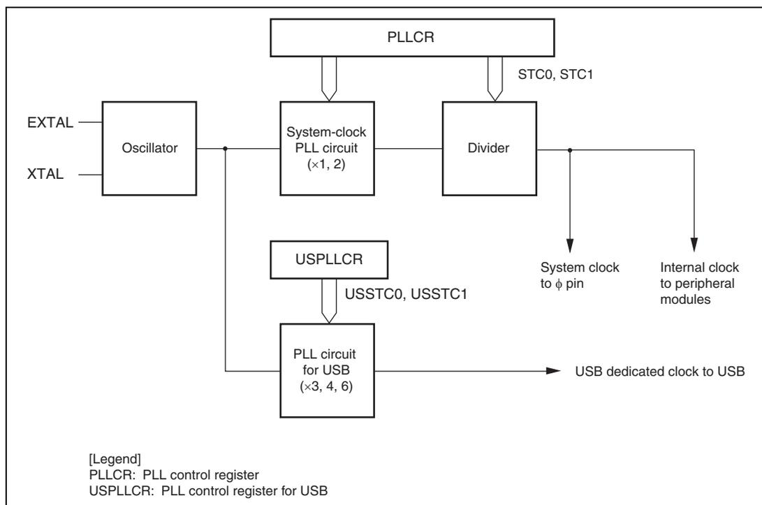
**Figure 23.1 Block Diagram of Clock Pulse Generator**
