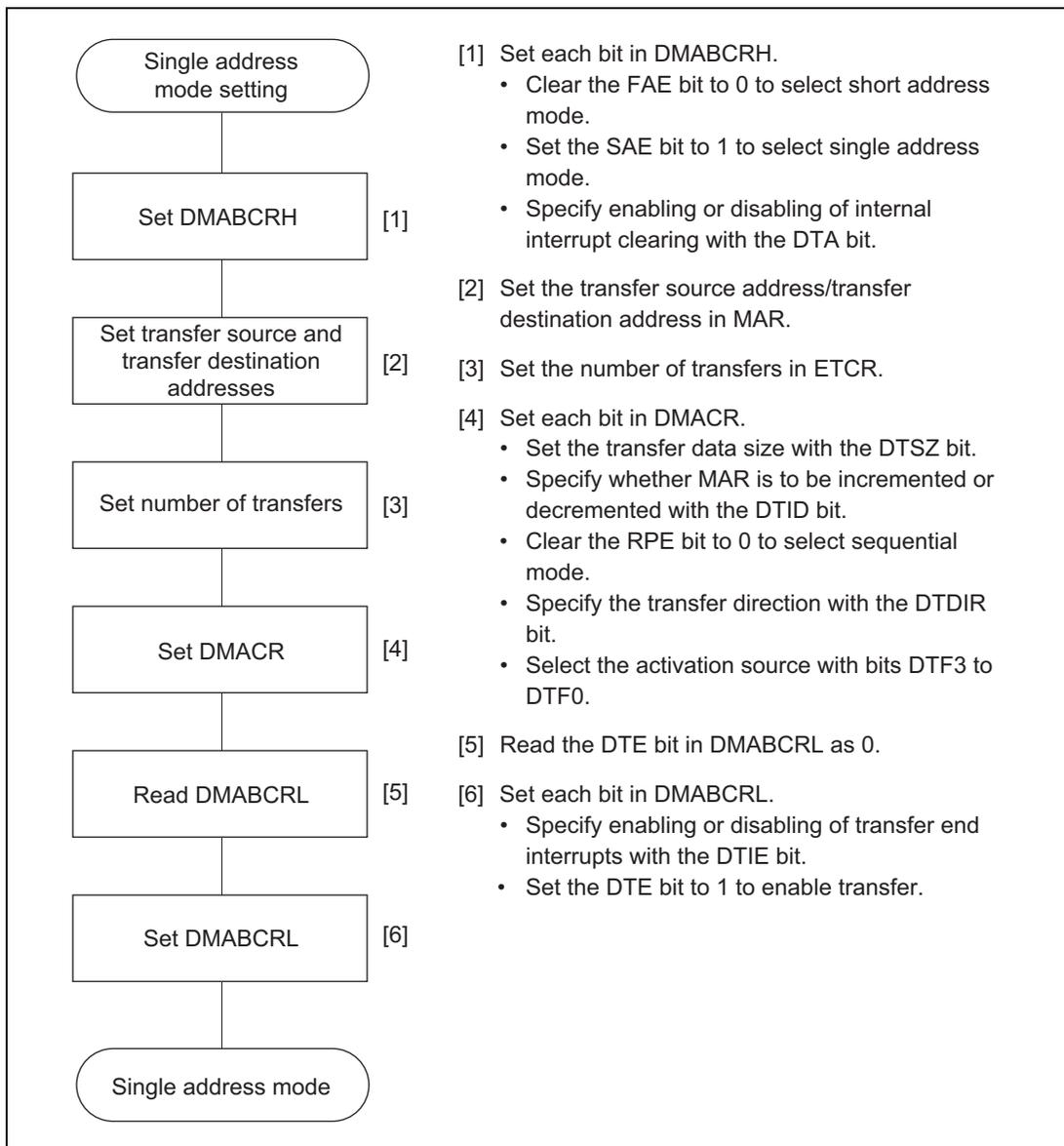
**Figure 7.10 Example of Single Address Mode Setting Procedure
