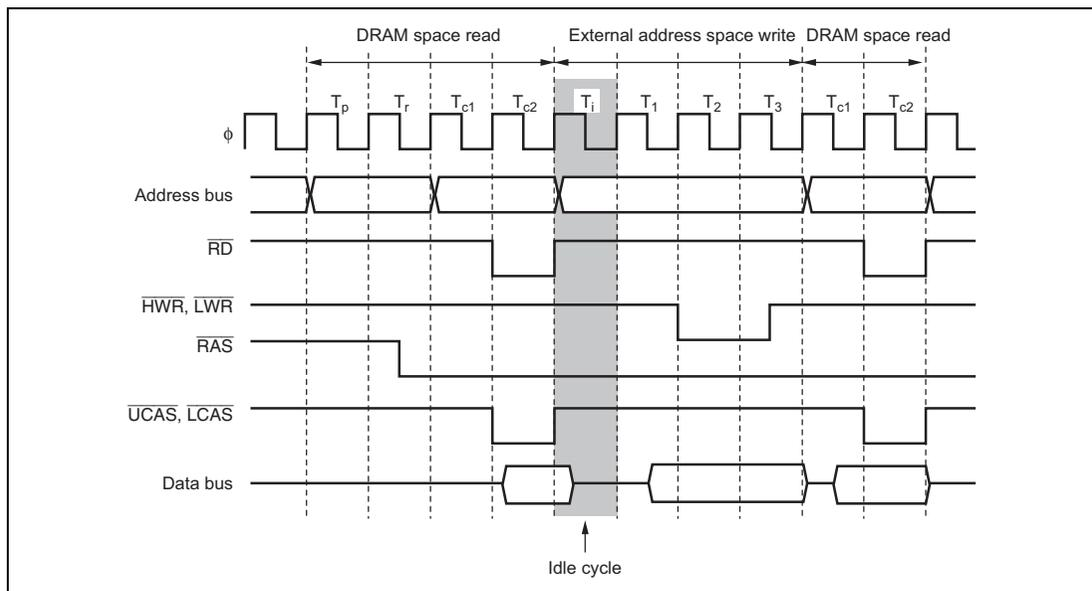
**Figure 6.89 Example of Idle Cycle Operation after DRAM Access
