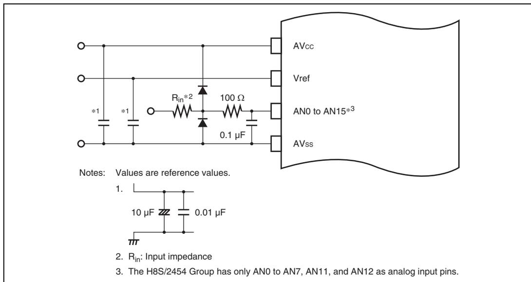
**Figure 18.12 Example of Analog Input Protection Circuit**
