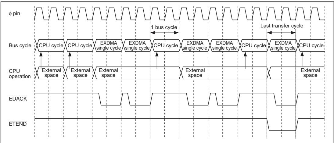
**Figure 8.33 Auto Request/Burst Mode/Normal Transfer Mode
