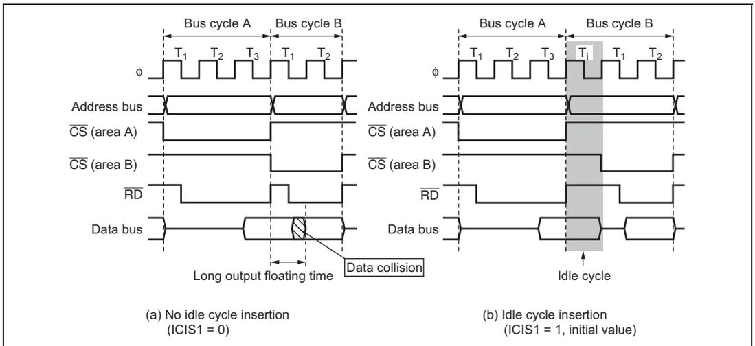
**Figure 6.77 Example of Idle Cycle Operation
