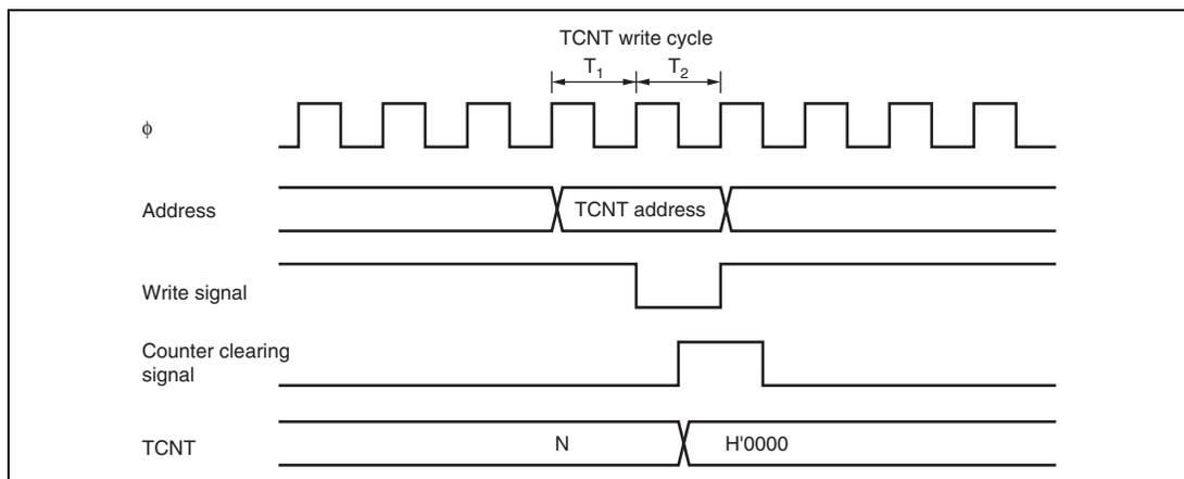
**Figure 11.46 Contention between TCNT Write and Clear Operations**
