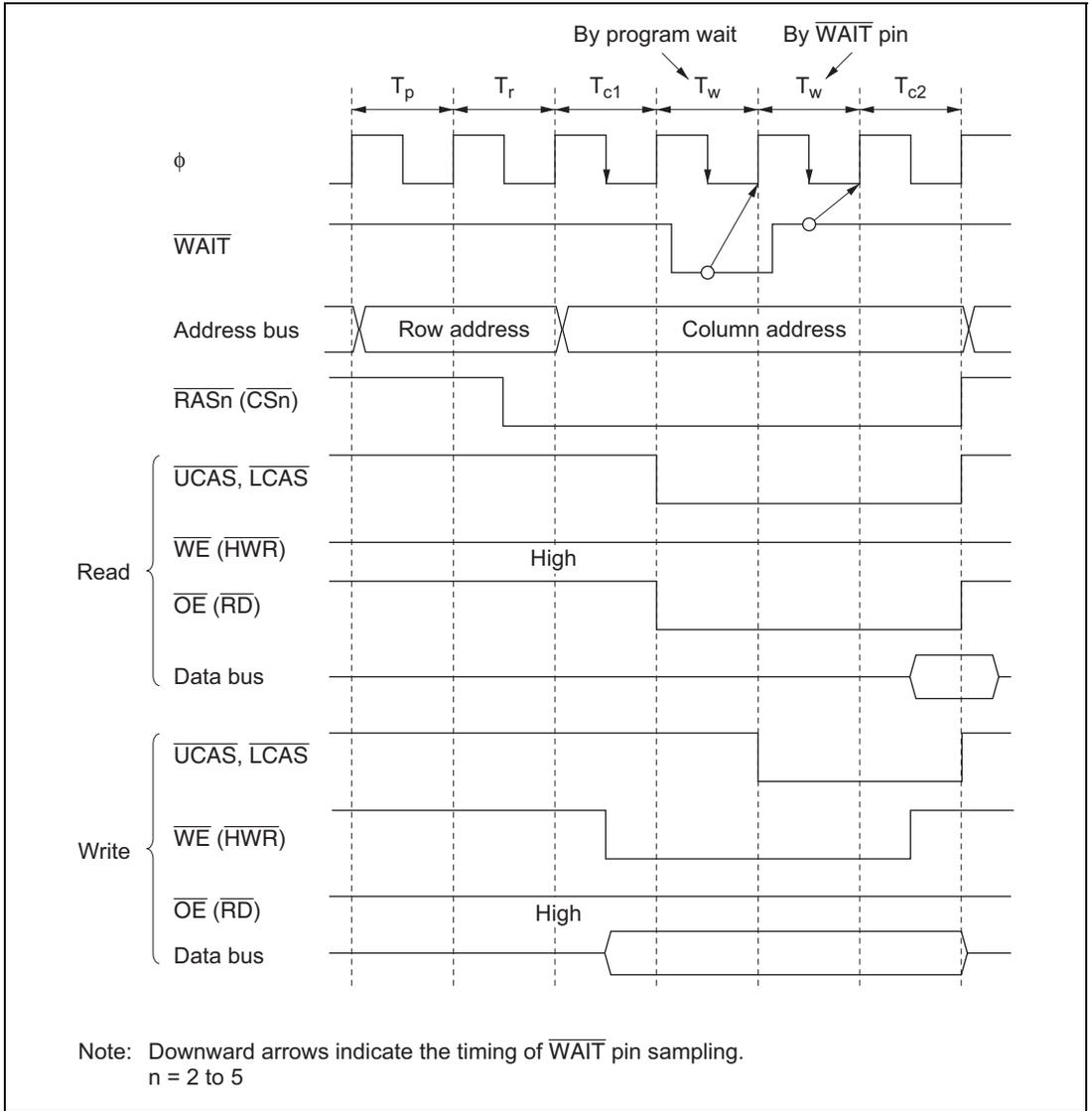
**Figure 6.38 Example of Wait State Insertion Timing
