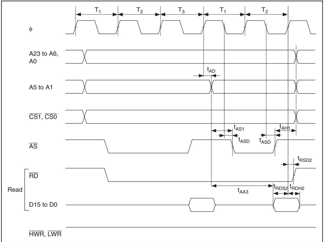
**Figure 26.14 Burst ROM Access Timing: Two-State Burst Access**
