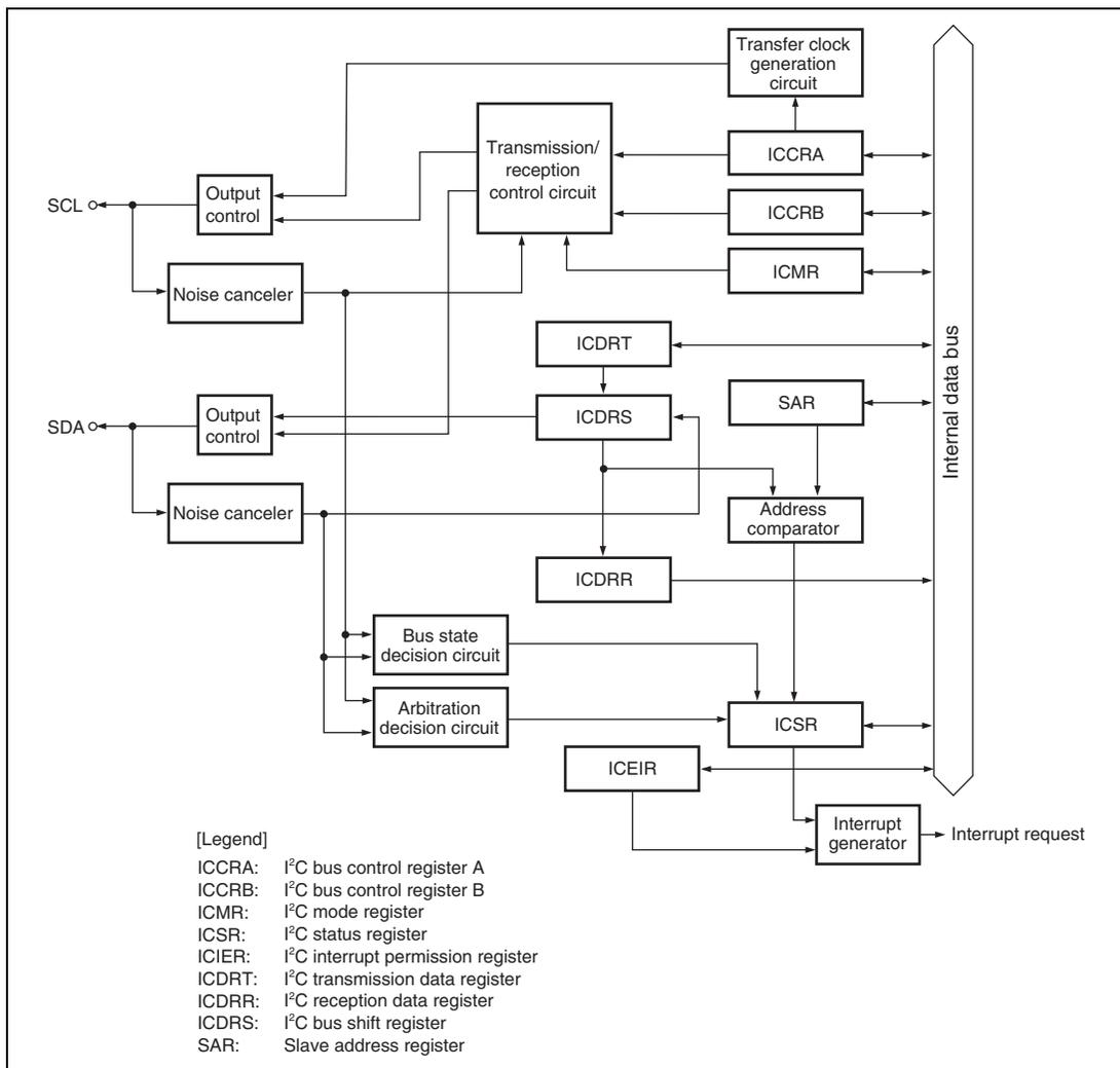
**Figure 17.1 Block Diagram of I<sup>2</sup>C Bus Interface 2**
