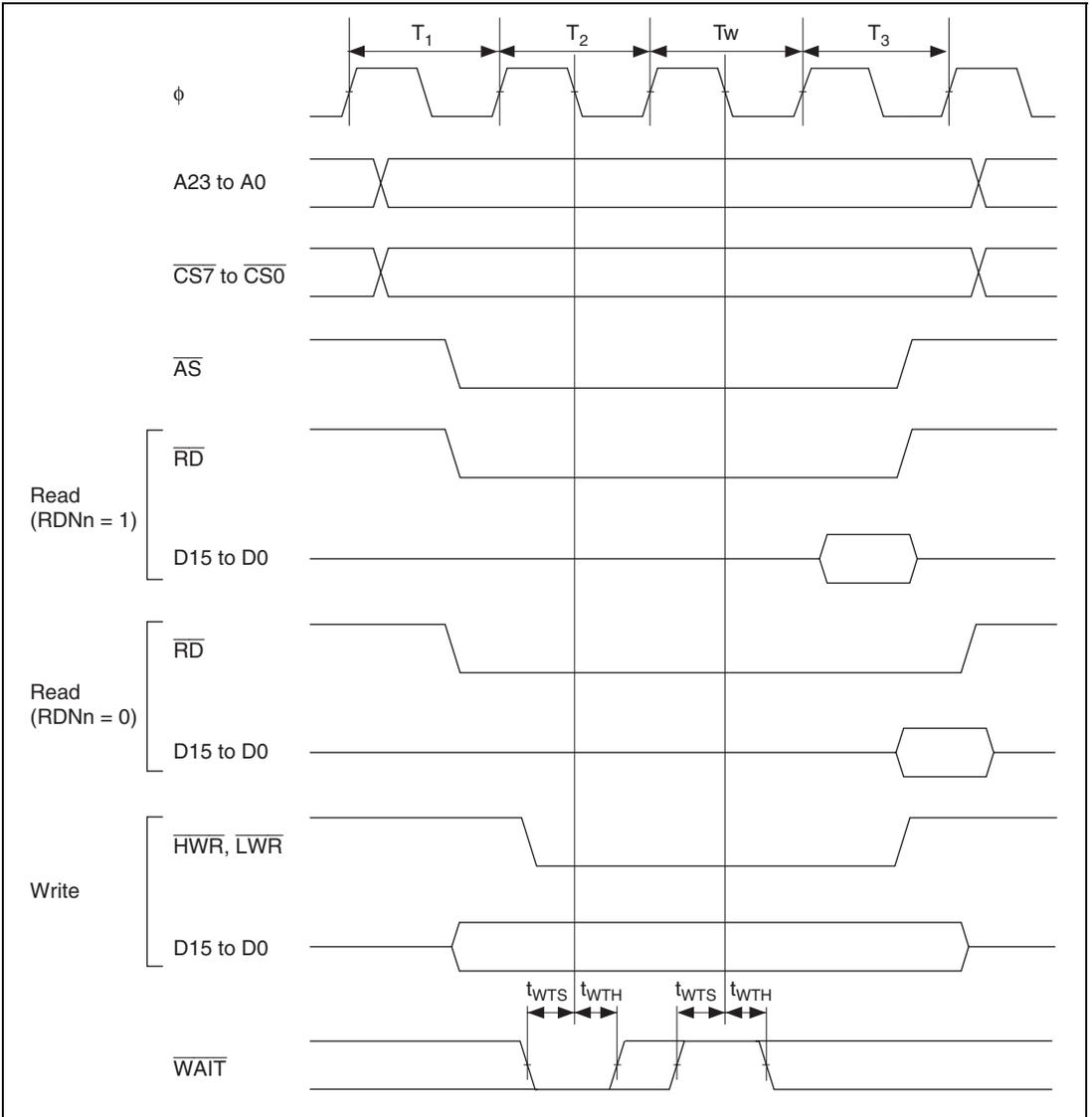
**Figure 26.10 Basic Bus Timing: Three-State Access, One Wait**
