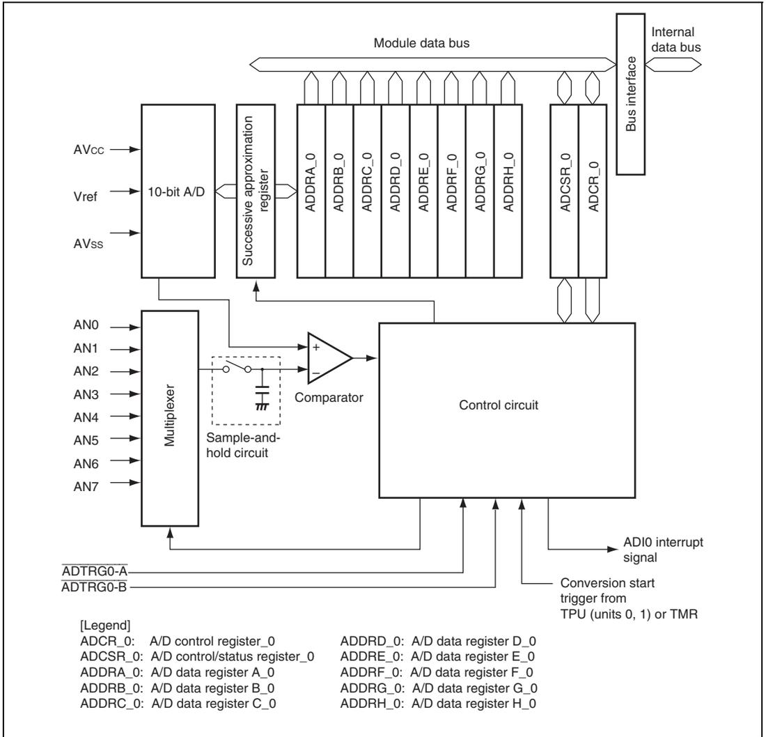
**Figure 18.1 Block Diagram of A/D Converter Unit 0 (AD\_0)**
