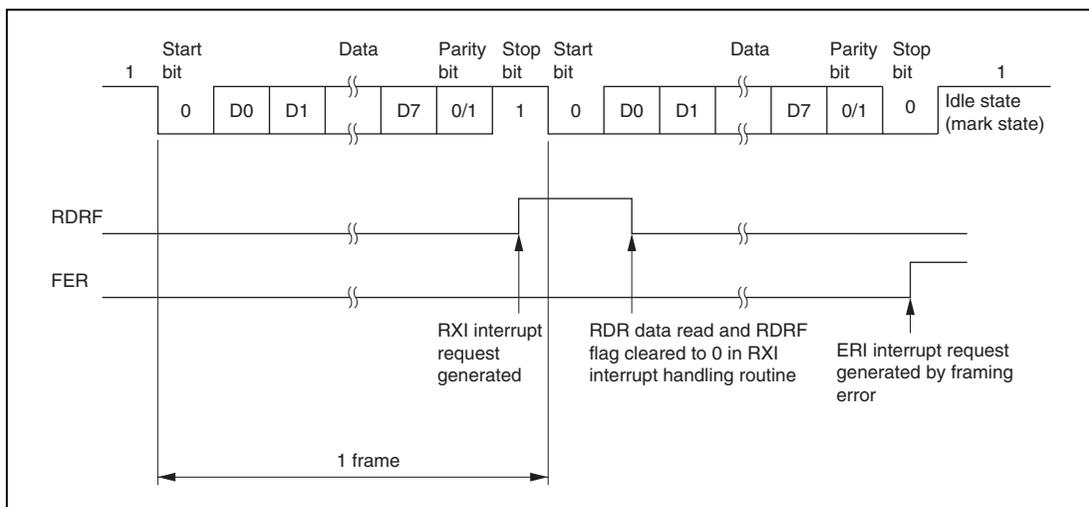
**Figure 15.8 Example of SCI Operation in Reception
