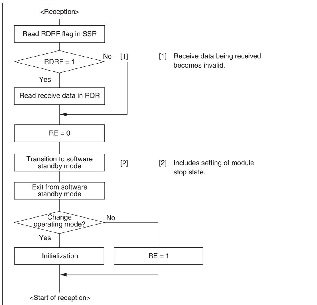
**Figure 15.39 Sample Flowchart for Mode Transition during Reception**
