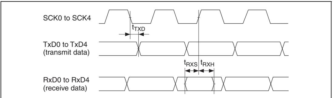
**Figure 26.48 SCI Input/Output Timing: Synchronous Mode**
