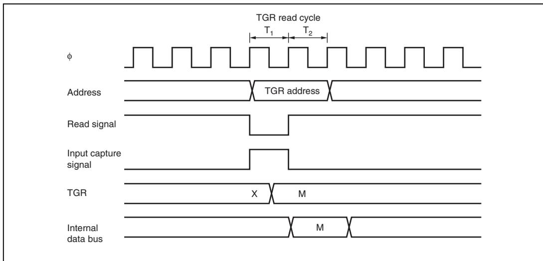
**Figure 11.50 Contention between TGR Read and Input Capture**
