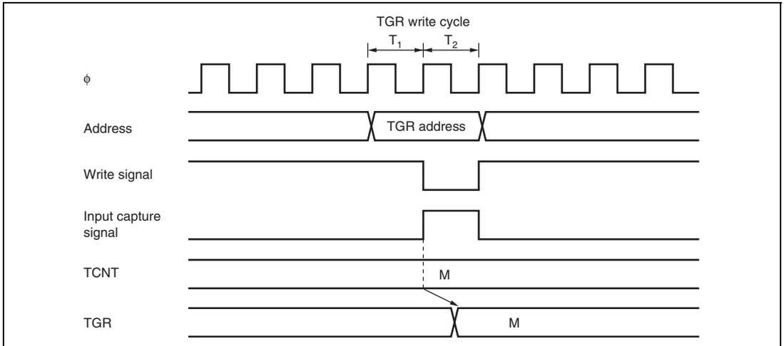
**Figure 11.51 Contention between TGR Write and Input Capture**
