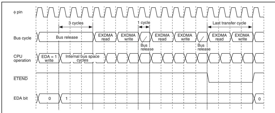
**Figure 8.28 Auto Request/Cycle Steal Mode/Normal Transfer Mode
