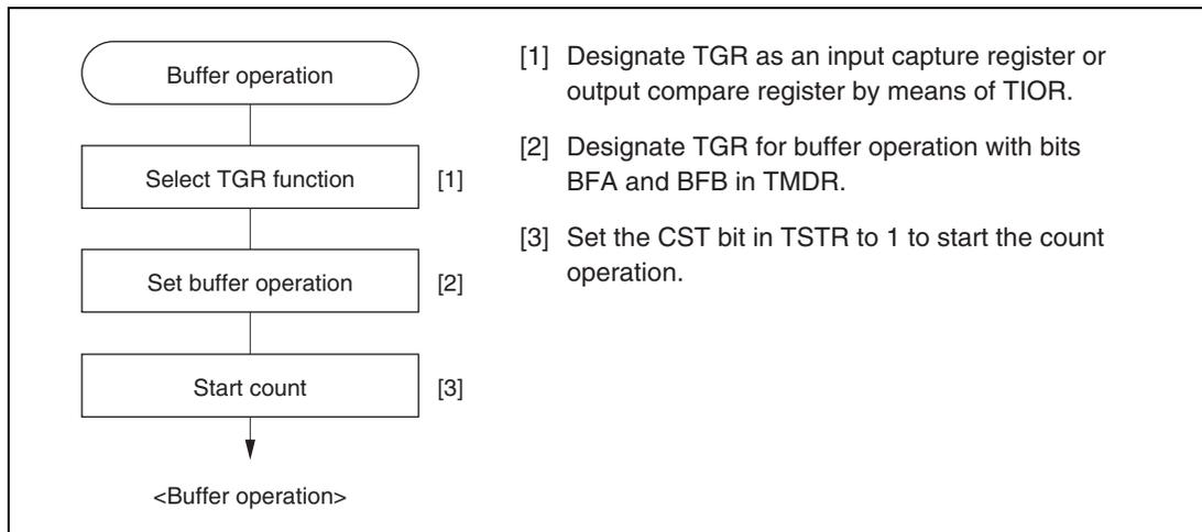
**Figure 11.15 Example of Buffer Operation Setting Procedure**
