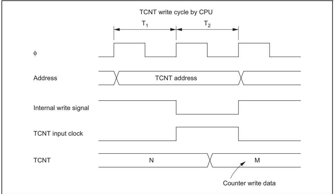
**Figure 13.12 Contention between TCNT Write and Increment**
