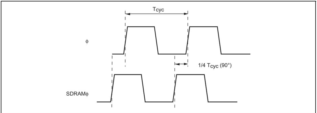
**Figure 6.55 Relationship between  $\phi$  and SDRAM $\phi$**
