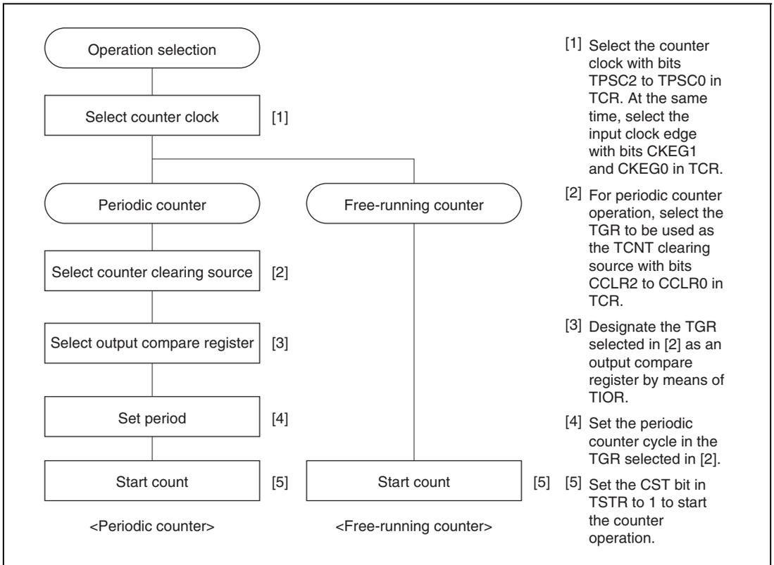
**Figure 11.3 Example of Counter Operation Setting Procedure**
