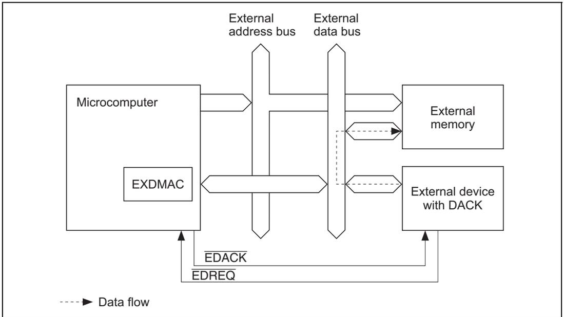
**Figure 8.3 Data Flow in Single Address Mode**
