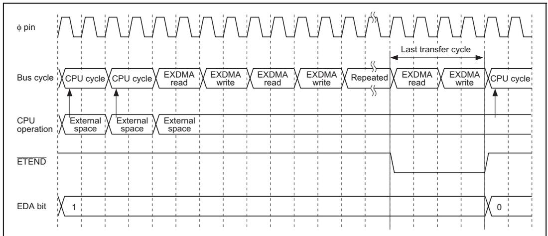
**Figure 8.31 Auto Request/Burst Mode/Normal Transfer Mode
