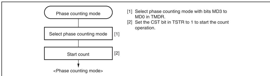
**Figure 11.25 Example of Phase Counting Mode Setting Procedure**
