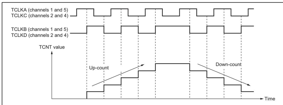
**Figure 11.29 Example of Phase Counting Mode 4 Operation**
