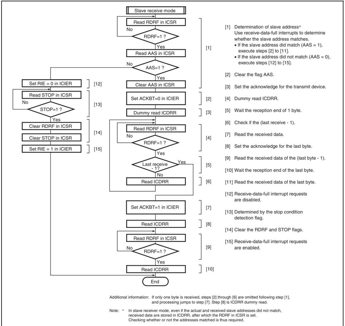
**Figure 17.17 Sample Flowchart for Slave Receive Mode**
