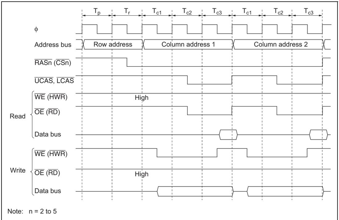
**Figure 6.43 Operation Timing in Fast Page Mode
