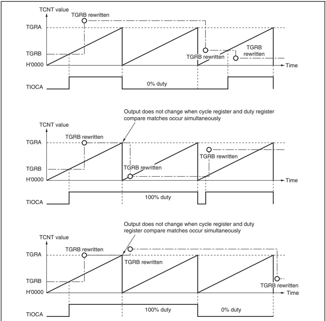
**Figure 11.24 Example of PWM Mode Operation (3)**
