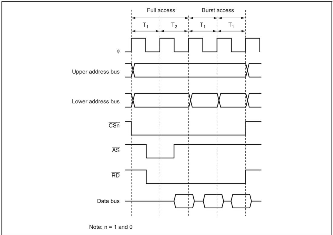
**Figure 6.76 Example of Burst ROM Access Timing
