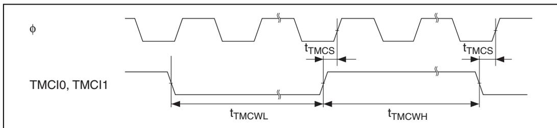
**Figure 26.44 8-Bit Timer Clock Input Timing**
