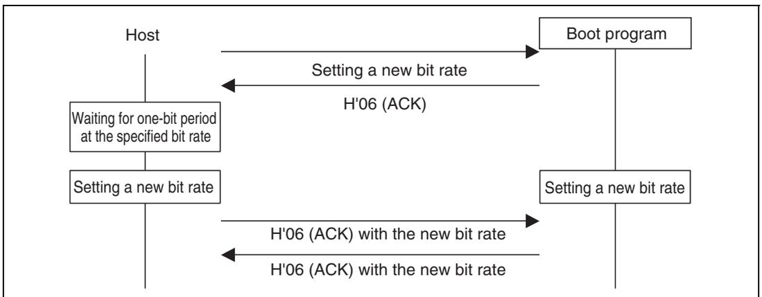
**Figure 22.13 New Bit-Rate Selection Sequence**
