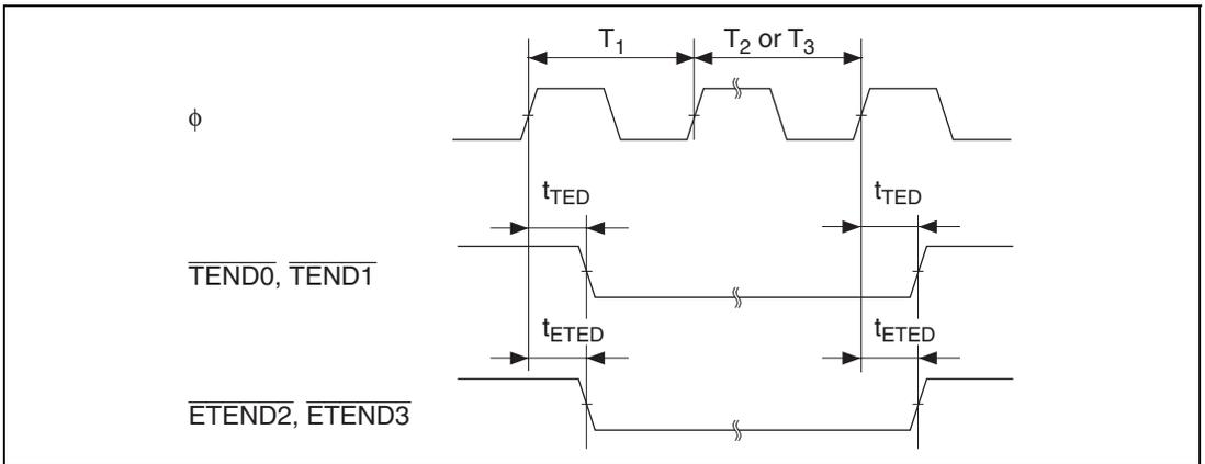
**Figure 26.33 DMAC and EXDMAC,  $\overline{TEND}/\overline{ETEND}$  Output Timing**
