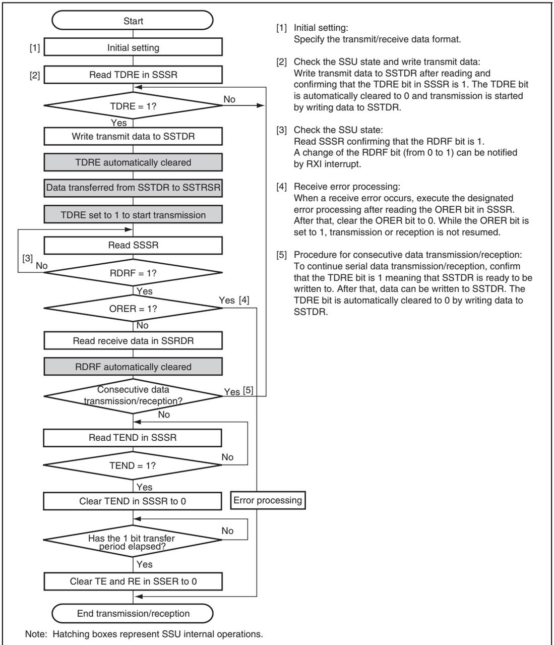
**Figure 20.17 Flowchart Example of Simultaneous Transmission/Reception
