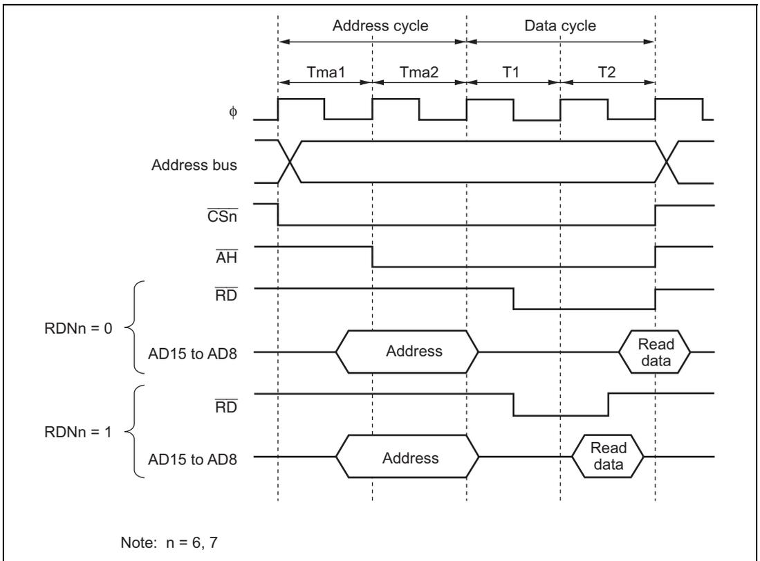
**Figure 6.30 Example of Read Strobe Timing**
