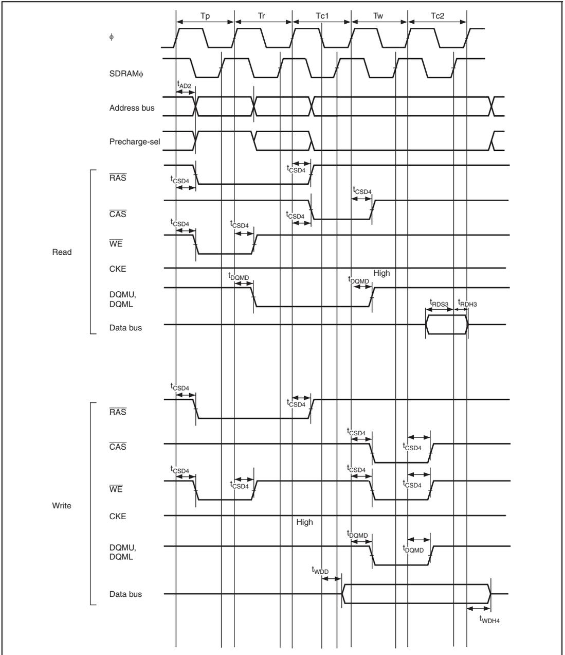
Figure 26.26 Synchronous DRAM Basic Access Timing (CAS Latency 2)
