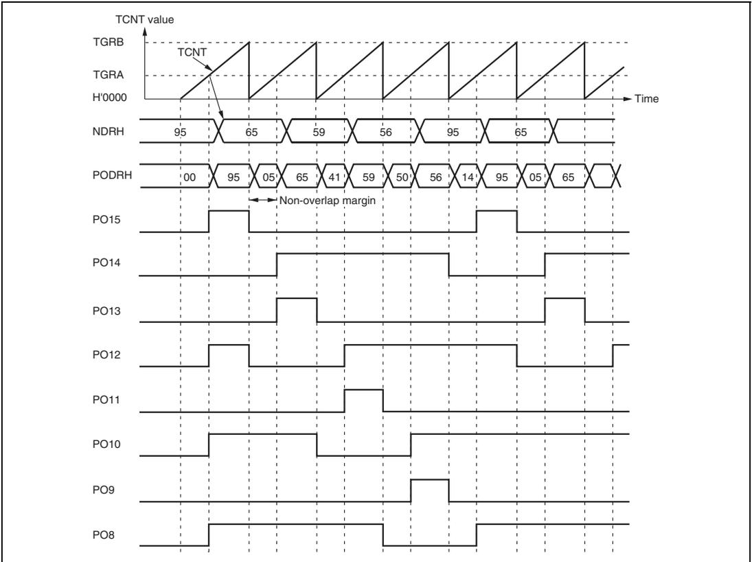
**Figure 12.9 Non-Overlapping Pulse Output Example (Four-Phase Complementary)**
