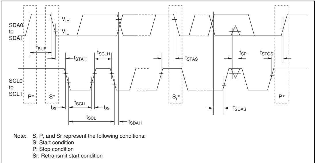
**Figure 26.50 I<sup>2</sup>C Bus Interface 2 Input/Output Timing**
