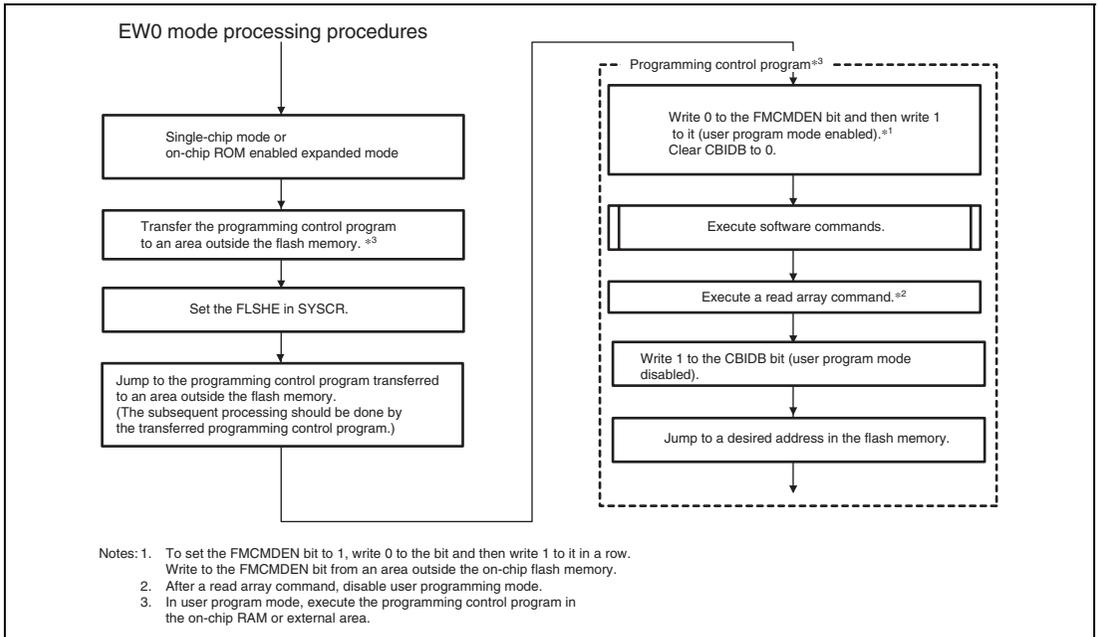
**Figure 22.2 Setting and Clearing EW0 Mode**
