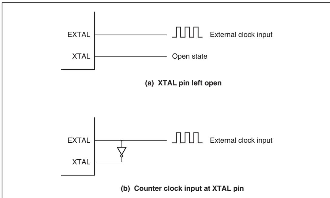
**Figure 23.4 Connection of External Clock Input (Examples)**
