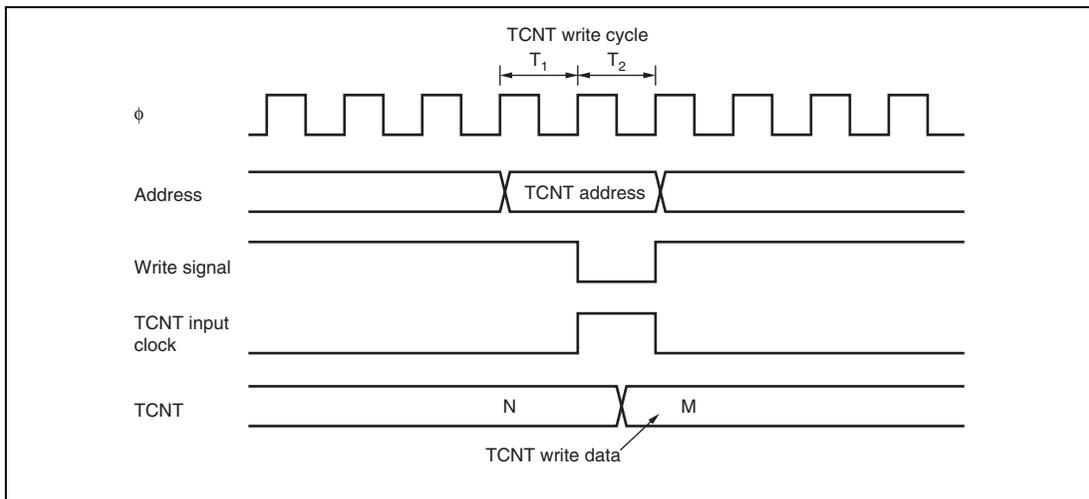
**Figure 11.47 Contention between TCNT Write and Increment Operations**
