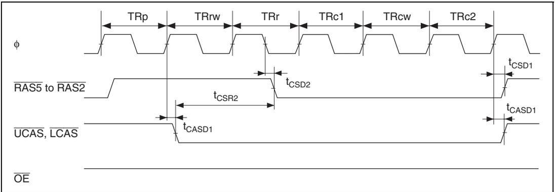
**Figure 26.21 CAS-Before-RAS Refresh Timing (with Wait Cycle Insertion)**
