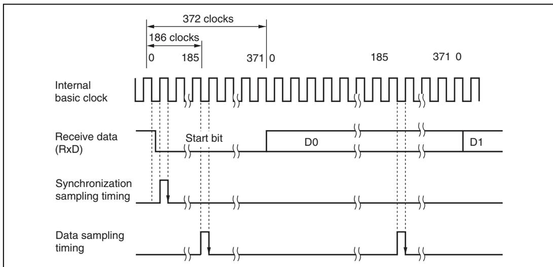
**Figure 15.25 Receive Data Sampling Timing in Smart Card Mode
