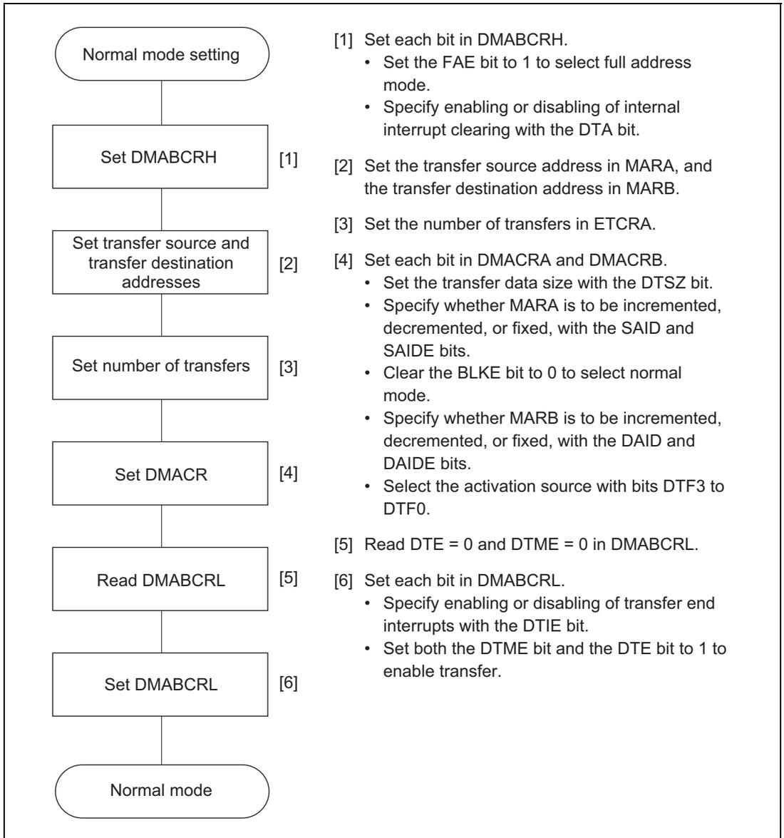
**Figure 7.12 Example of Normal Mode Setting Procedure**
