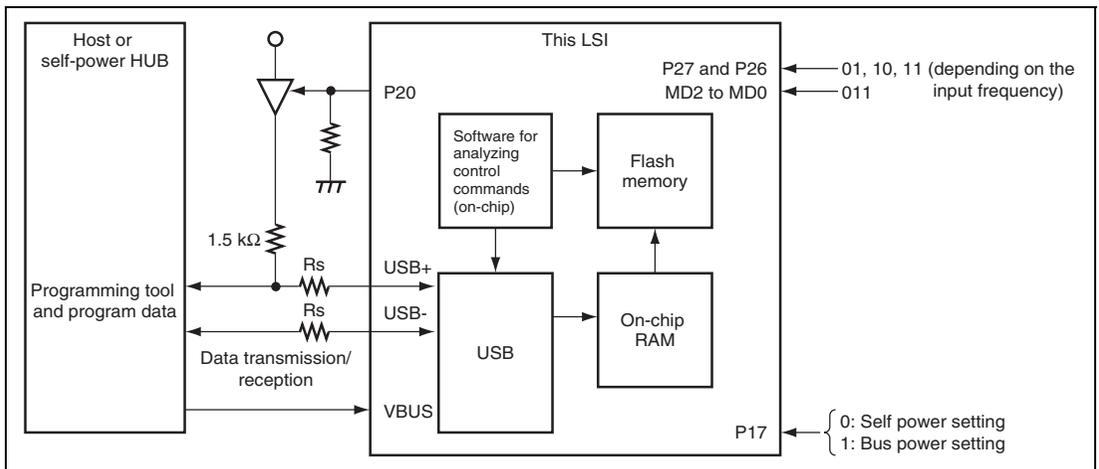
**Figure 22.8 System Configuration in USB Boot Mode**
