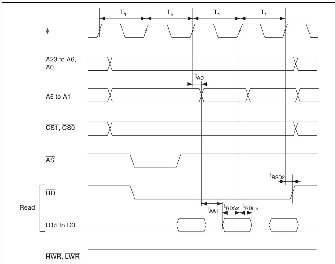
**Figure 26.13 Burst ROM Access Timing: One-State Burst Access**
