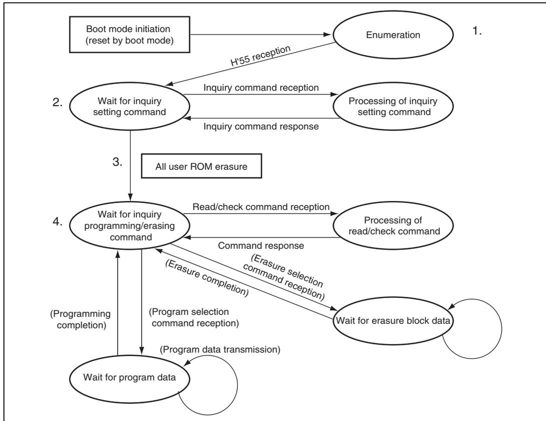
**Figure 22.9 USB Boot Mode State Transition Diagram**
