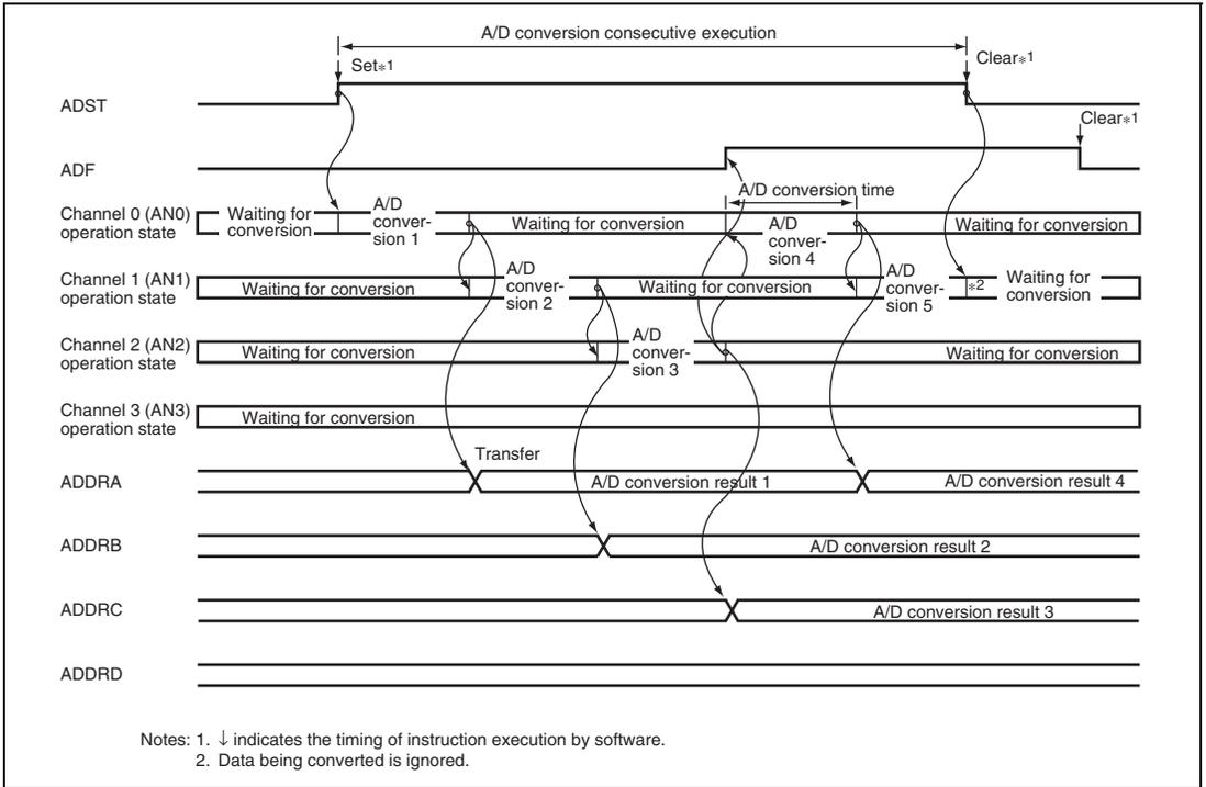
**Figure 18.4 Example of A/D Conversion
