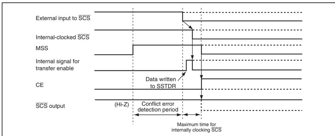
**Figure 20.10 Conflict Error Detection Timing (Before Transfer)**
