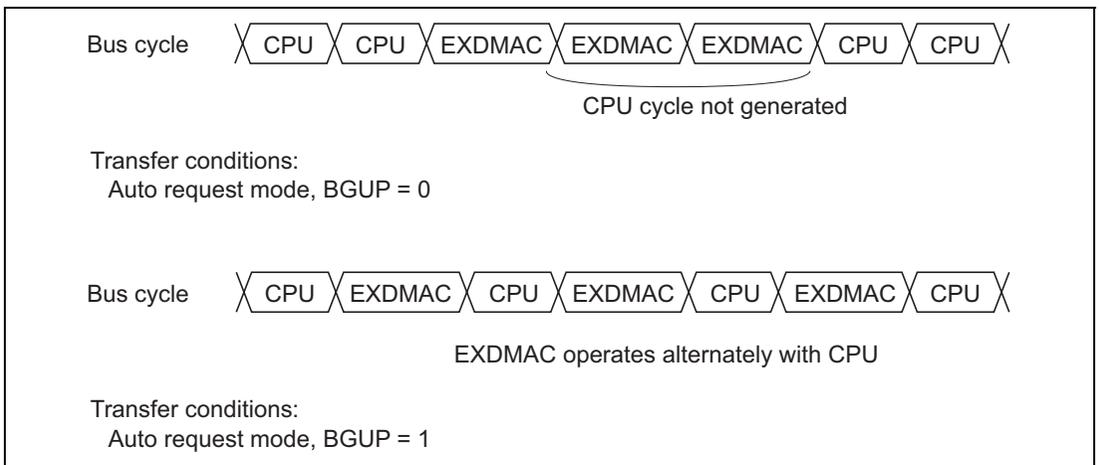
**Figure 8.6 Examples of Timing in Burst Mode**
