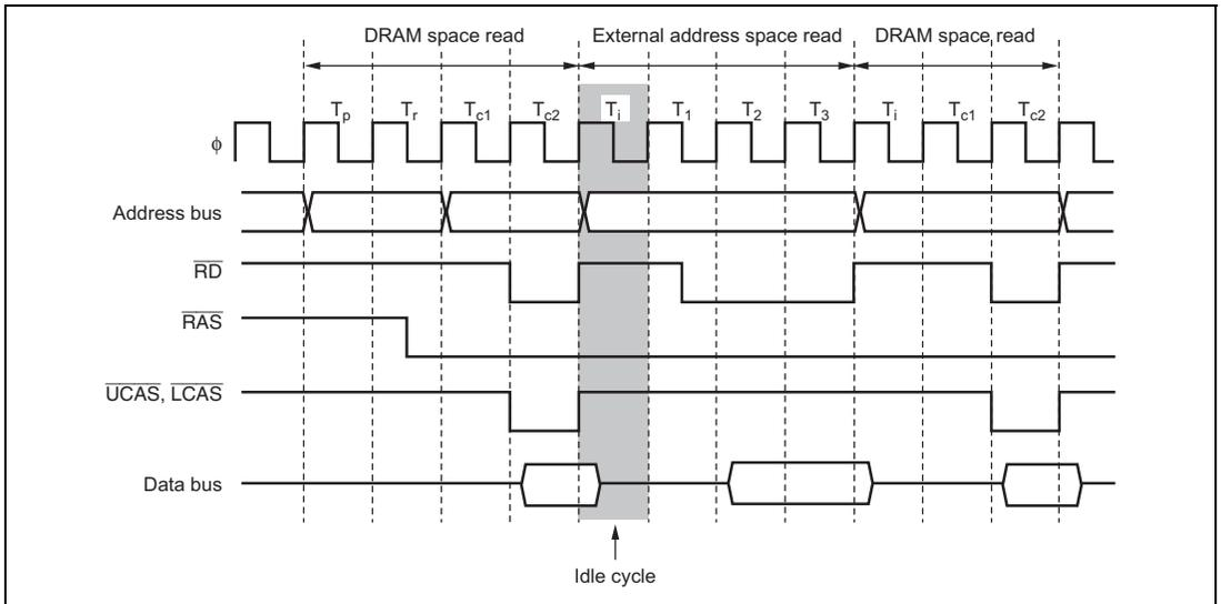
**Figure 6.88 Example of Idle Cycle Operation after DRAM Access
