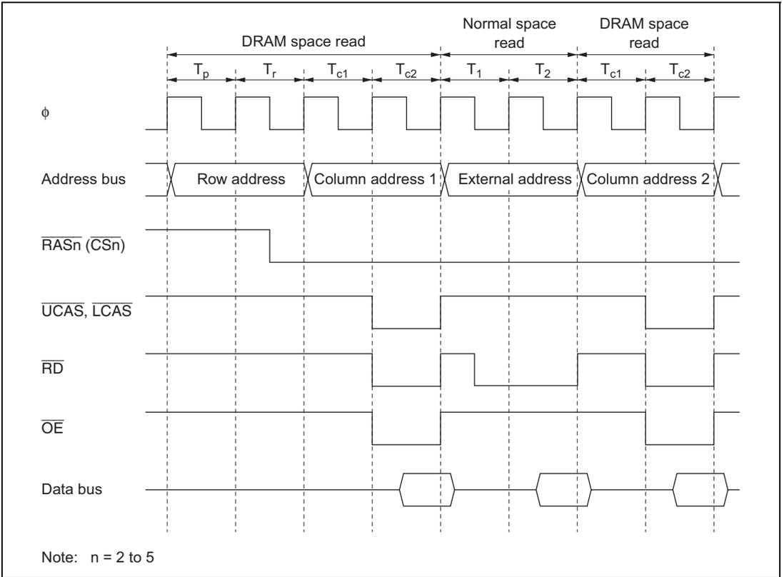
**Figure 6.44 Example of Operation Timing in RAS Down Mode
