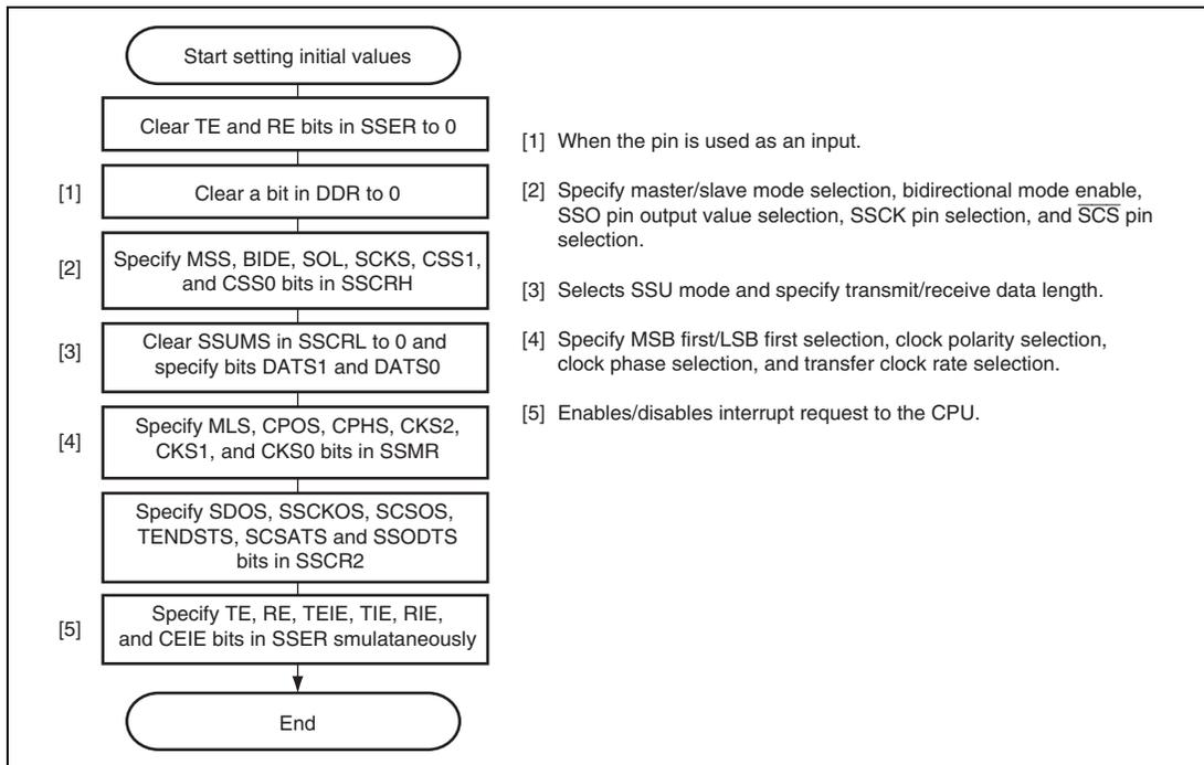
**Figure 20.4 Example of Initial Settings in SSU Mode**
