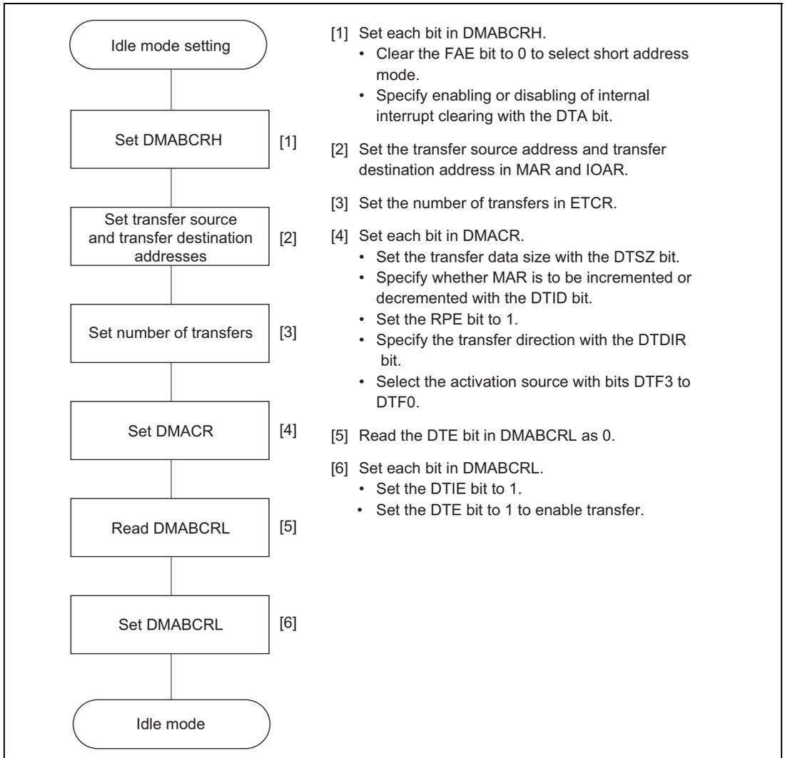
**Figure 7.6 Example of Idle Mode Setting Procedure**
