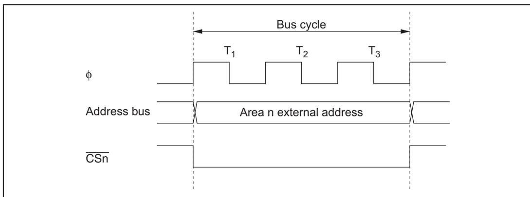
Figure 6.7  $\overline{CSn}$  Signal Output Timing (n = 0 to 7)
