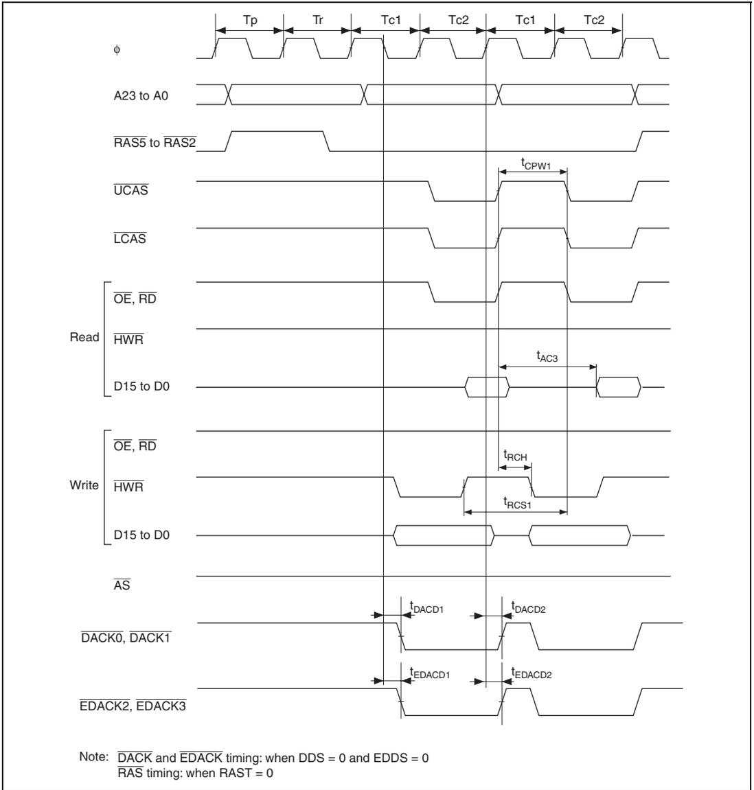
**Figure 26.17 DRAM Access Timing: Two-State Burst Access**
