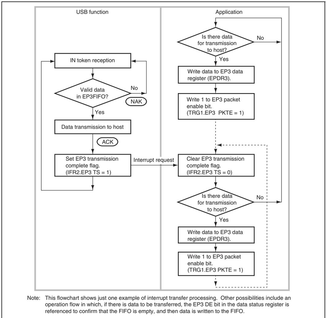
**Figure 16.18 Operation of EP3 Interrupt-In Transfer**
