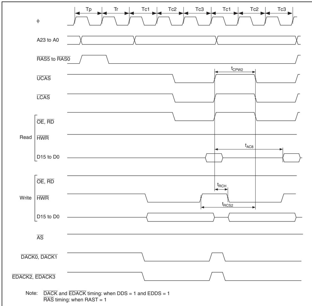
**Figure 26.19 DRAM Access Timing: Three-State Burst Access**
