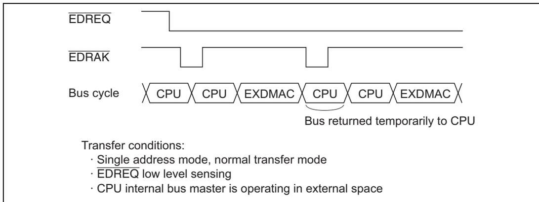
**Figure 8.5 Example of Timing in Cycle Steal Mode**
