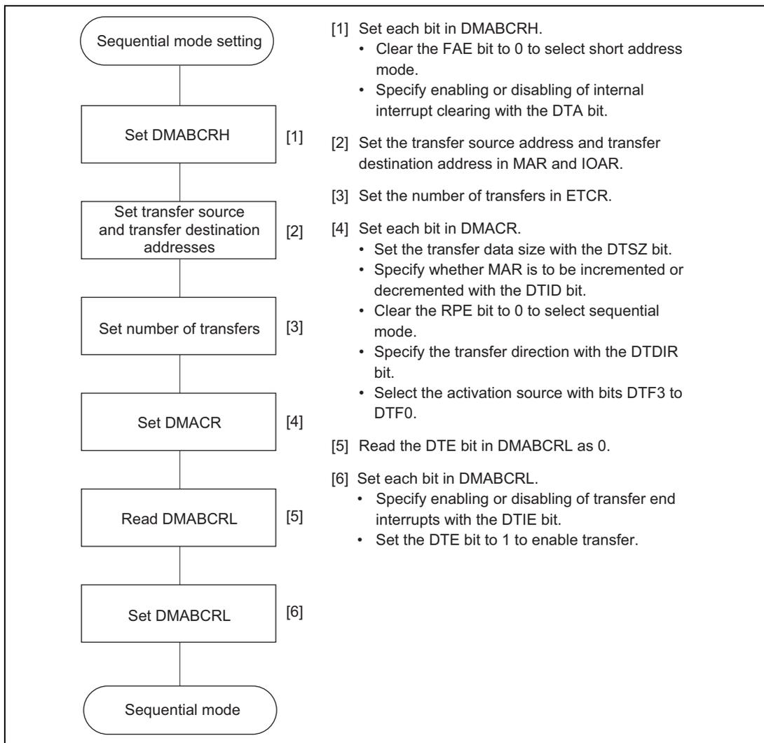
**Figure 7.4 Example of Sequential Mode Setting Procedure**
