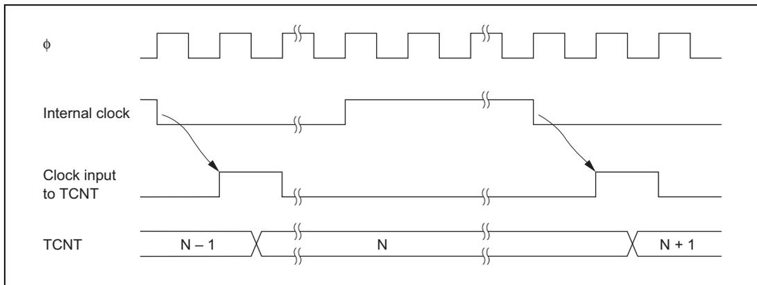
**Figure 13.4 Count Timing for Internal Clock Input**
