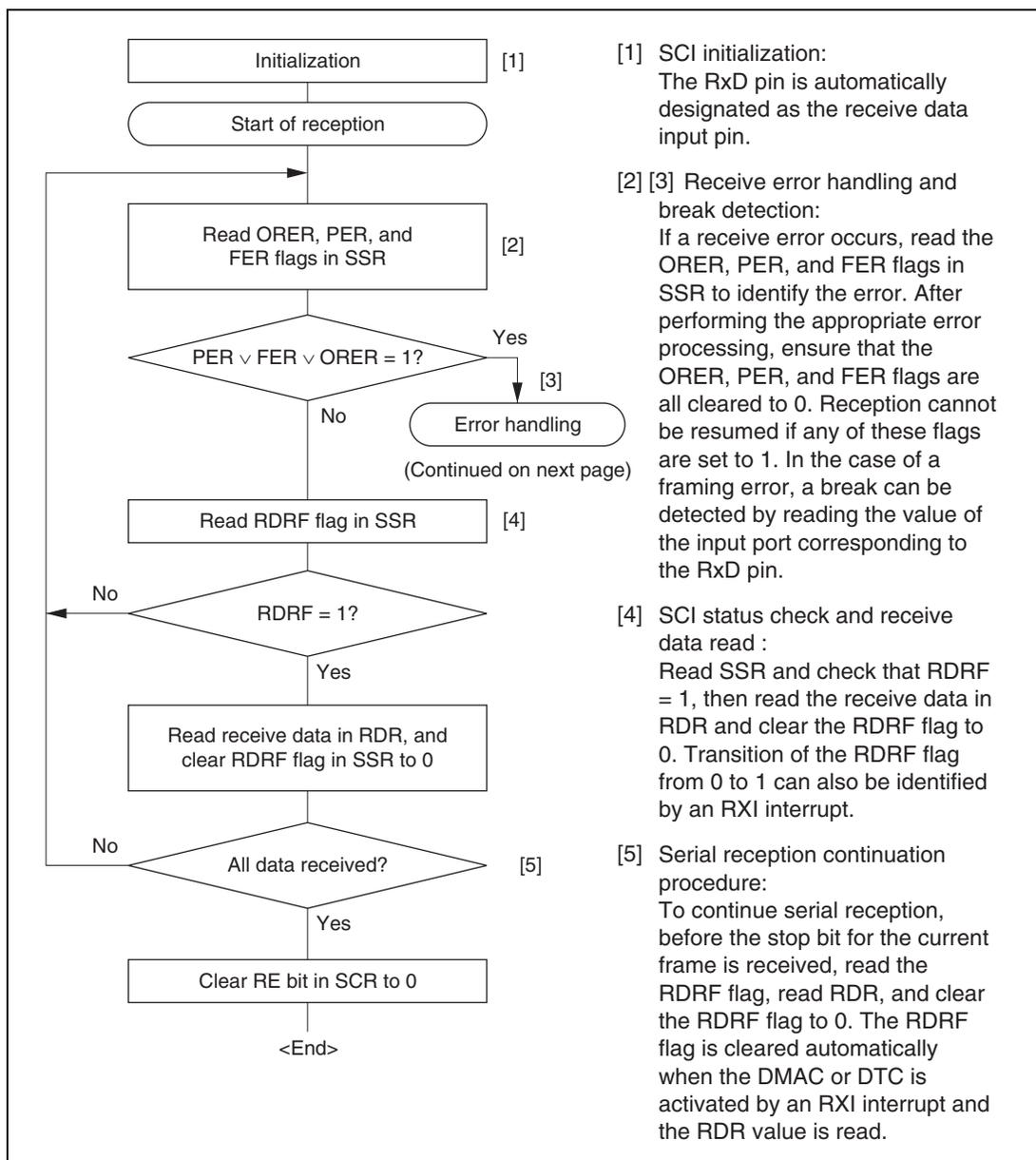
**Figure 15.9 Sample Serial Reception Data Flowchart (1)**
