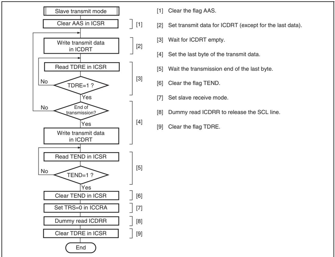
**Figure 17.16 Sample Flowchart for Slave Transmit Mode**
