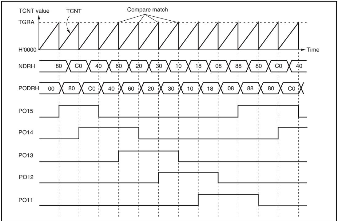
**Figure 12.5 Normal Pulse Output Example (Five-Phase Pulse Output)**
