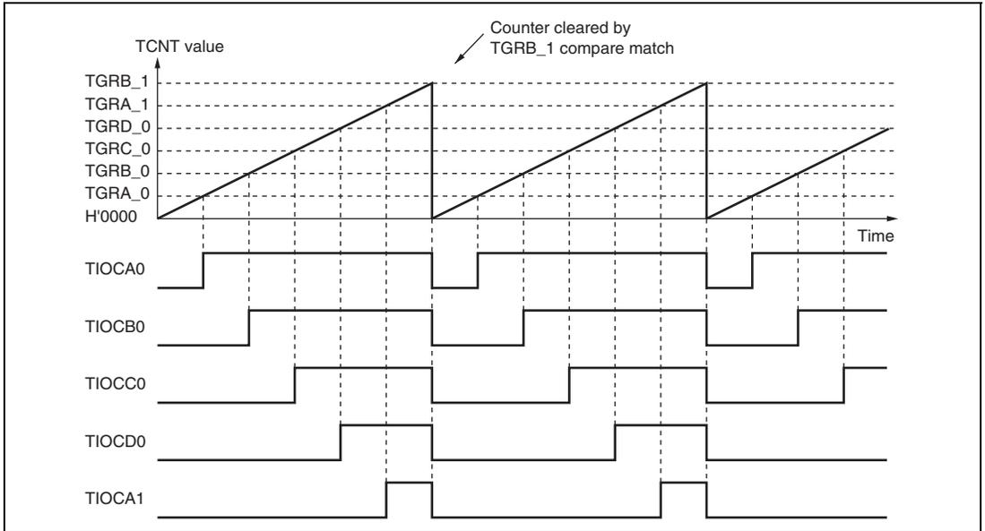
**Figure 11.23 Example of PWM Mode Operation (2)**
