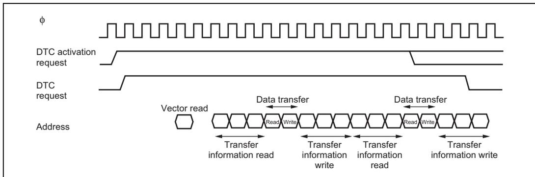
**Figure 9.12 DTC Operation Timing (Example of Chain Transfer)**
