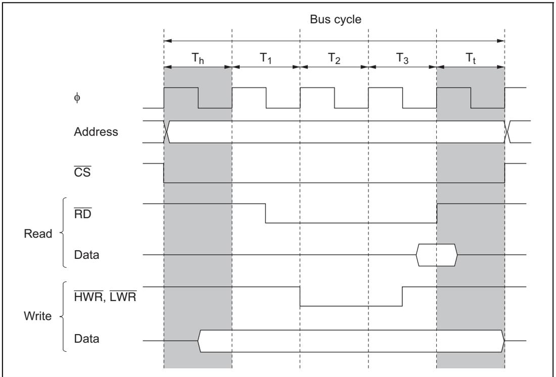
**Figure 6.3  $\overline{CS}$  and Address Assertion Period Extension**
