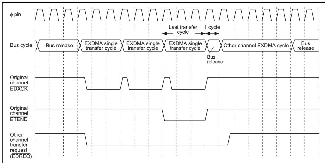
**Figure 8.34 Auto Request/Burst Mode/Normal Transfer Mode
