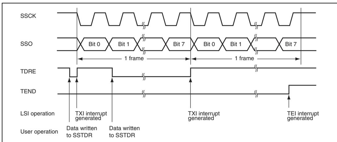
**Figure 20.13 Example of Transmission Operation
