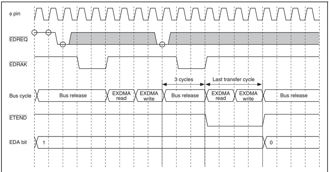
**Figure 8.35 External Request/Cycle Steal Mode/Normal Transfer Mode
