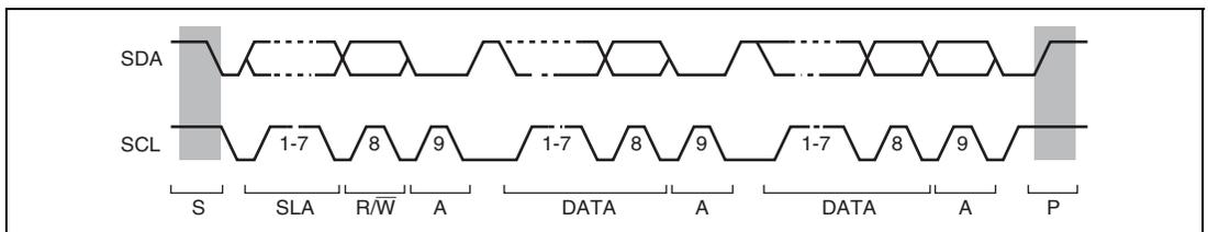
**Figure 17.4 I<sup>2</sup>C Bus Timing**
