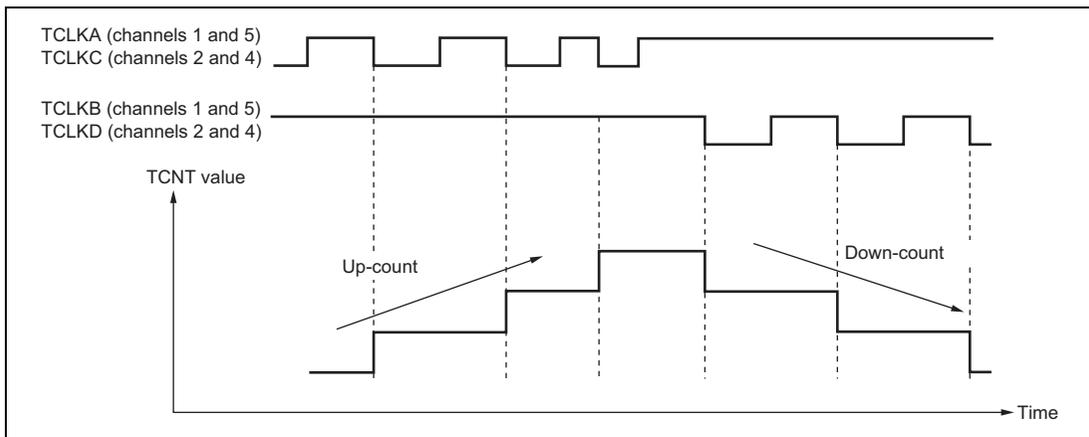
**Figure 11.28 Example of Phase Counting Mode 3 Operation**
