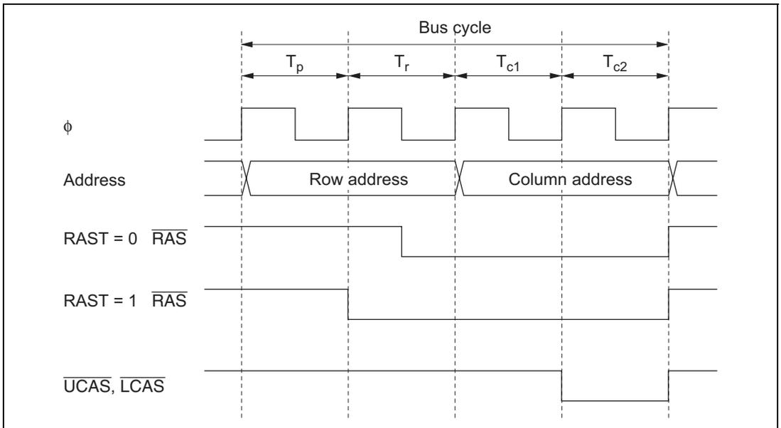
**Figure 6.4  $\overline{\text{RAS}}$  Signal Assertion Timing
