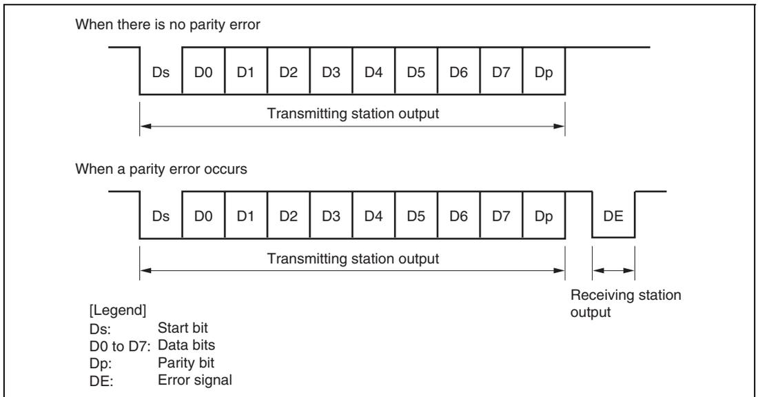
**Figure 15.22 Normal Smart Card Interface Data Format**
