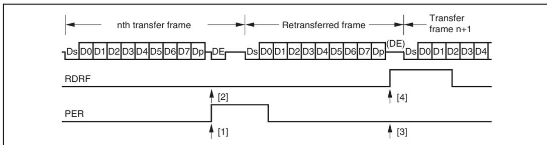
**Figure 15.29 Retransfer Operation in SCI Receive Mode**
