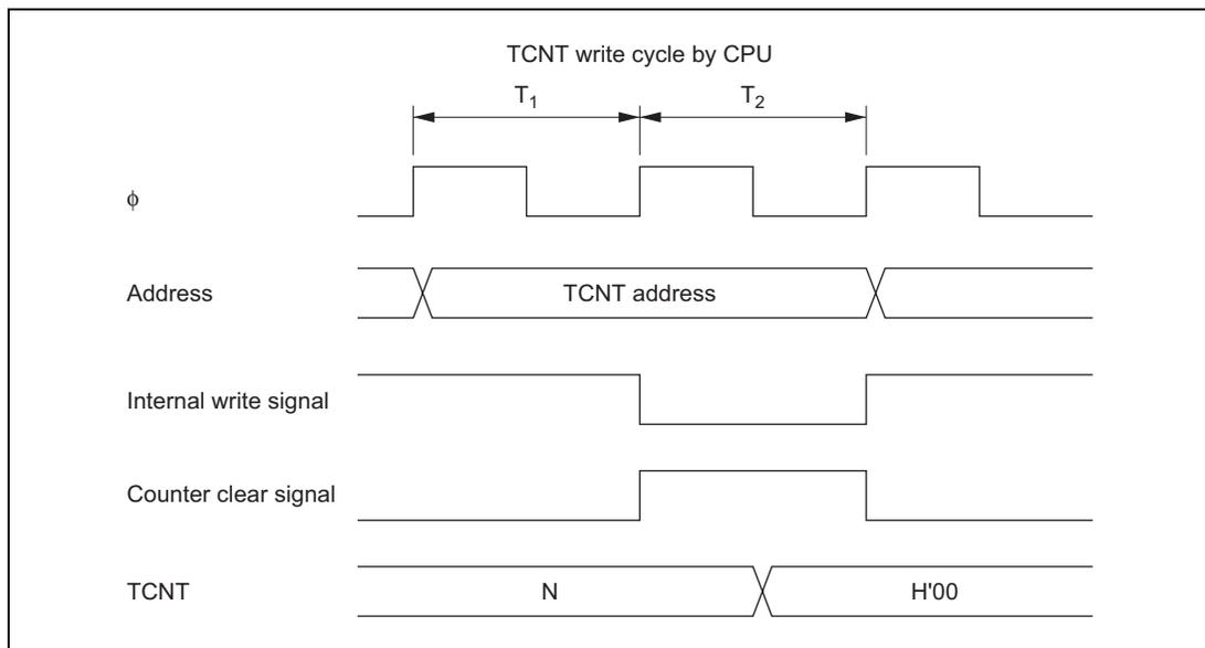
**Figure 13.11 Contention between TCNT Write and Clear**
