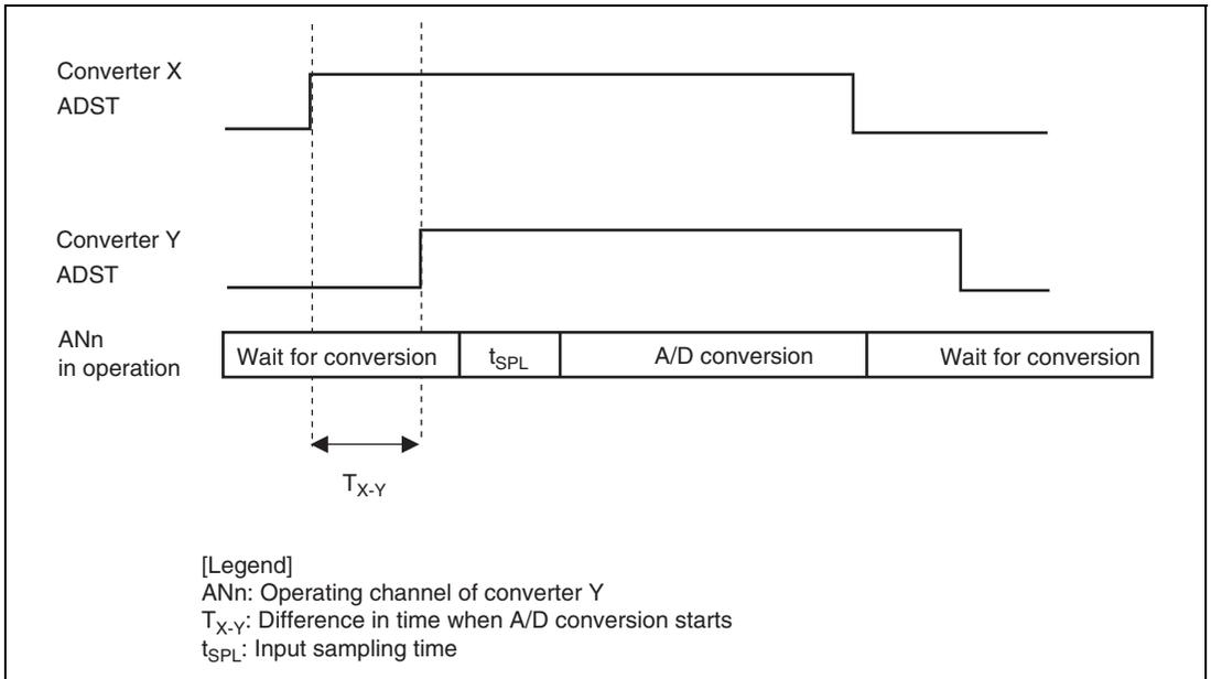
**Figure 18.13 An Example of Timing Where Accuracy of A/D Conversion is not Guaranteed**
