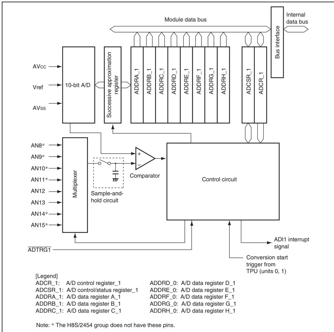
**Figure 18.2 Block Diagram of A/D Converter Unit 1 (AD\_1)**
