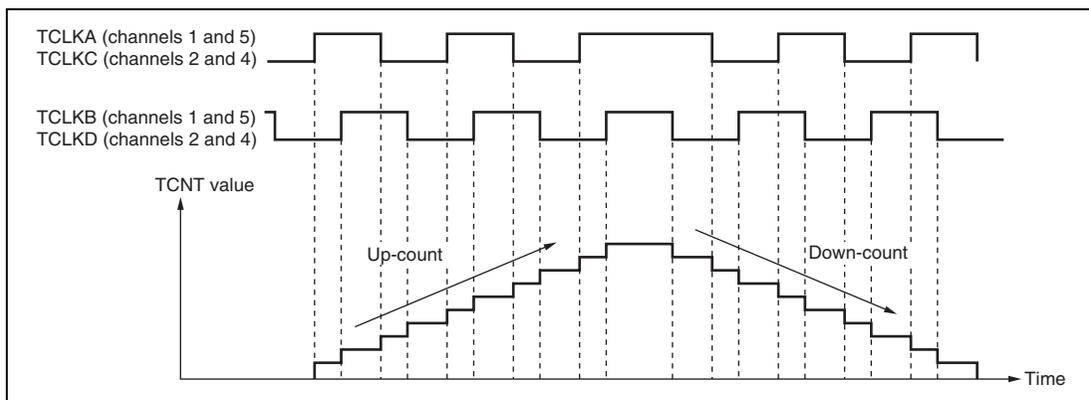
**Figure 11.26 Example of Phase Counting Mode 1 Operation**
