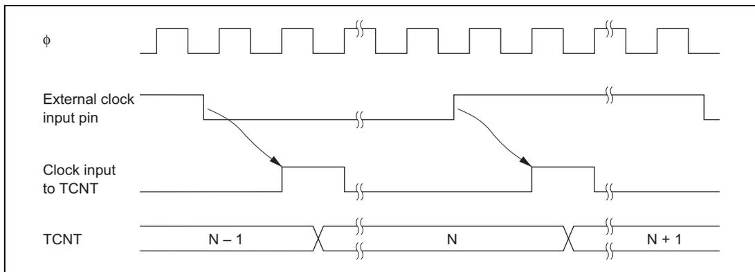
**Figure 13.5 Count Timing for External Clock Input**
