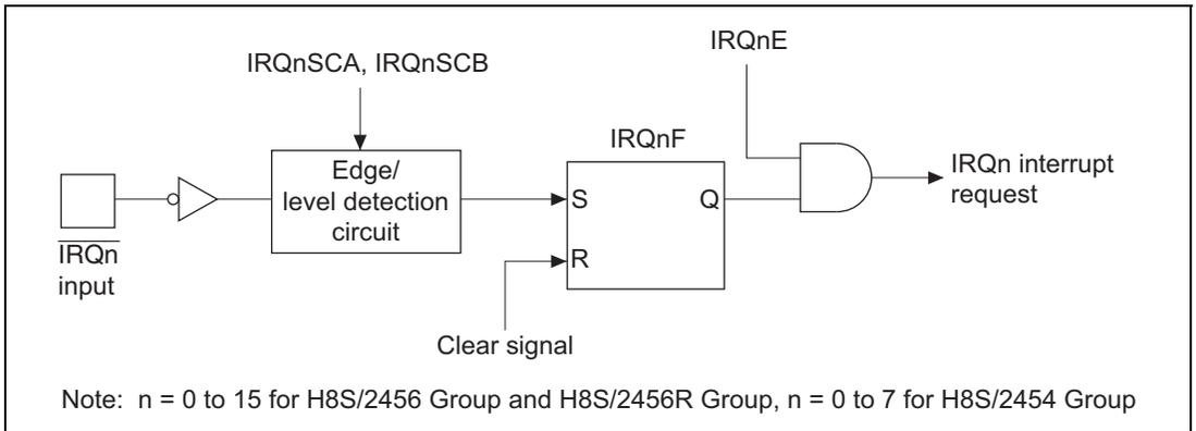
**Figure 5.2 Block Diagram of IRQ Interrupts**
