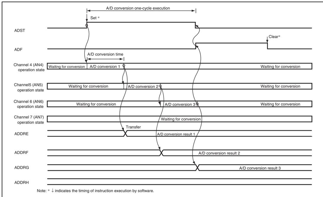
**Figure 18.5 Example of A/D Conversion
