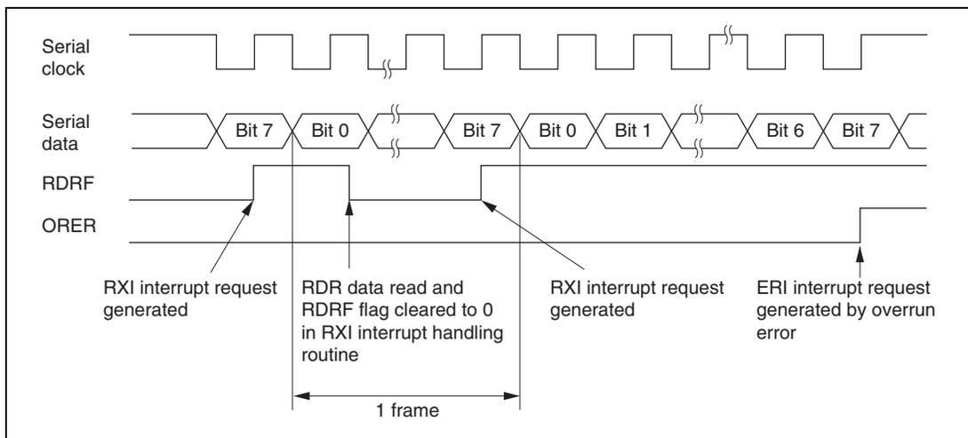
**Figure 15.18 Example of SCI Operation in Reception**
