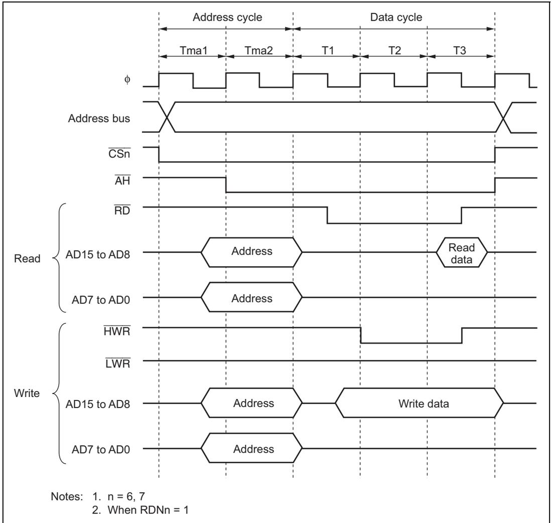
**Figure 6.26 Bus Timing for 16-Bit, 3-State Data Access Space
