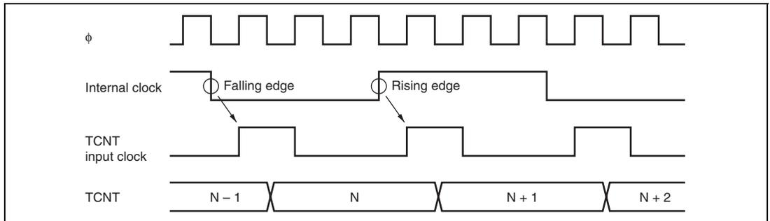
**Figure 11.31 Count Timing in Internal Clock Operation**
