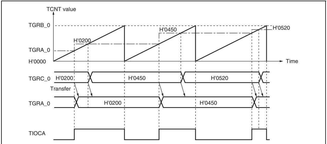
**Figure 11.16 Example of Buffer Operation (1)**
