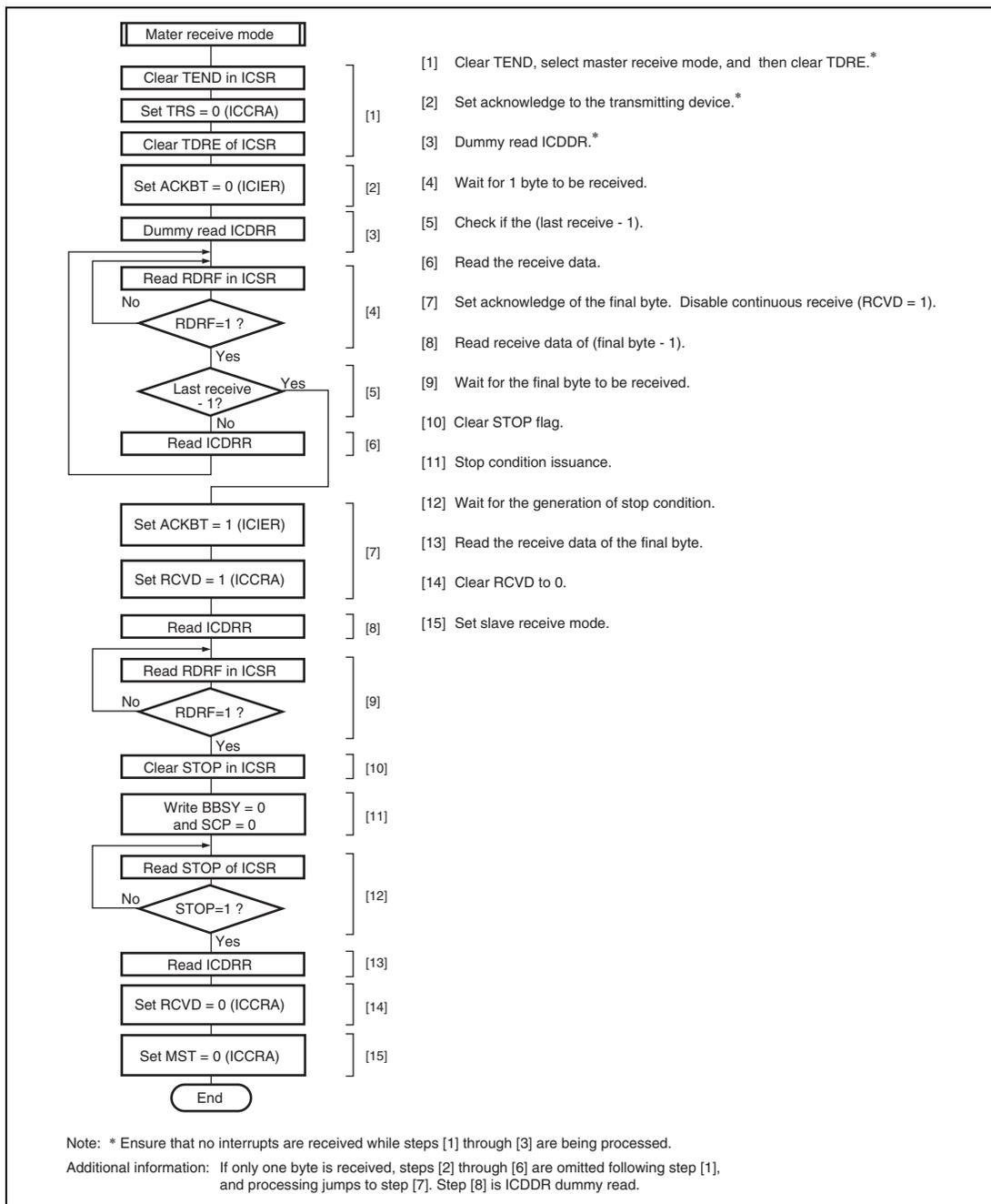
**Figure 17.15 Sample Flowchart for Master Receive Mode**
