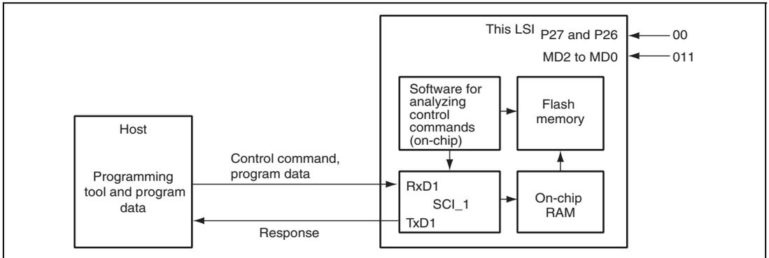
**Figure 22.7 System Configuration in SCI Boot Mode**
