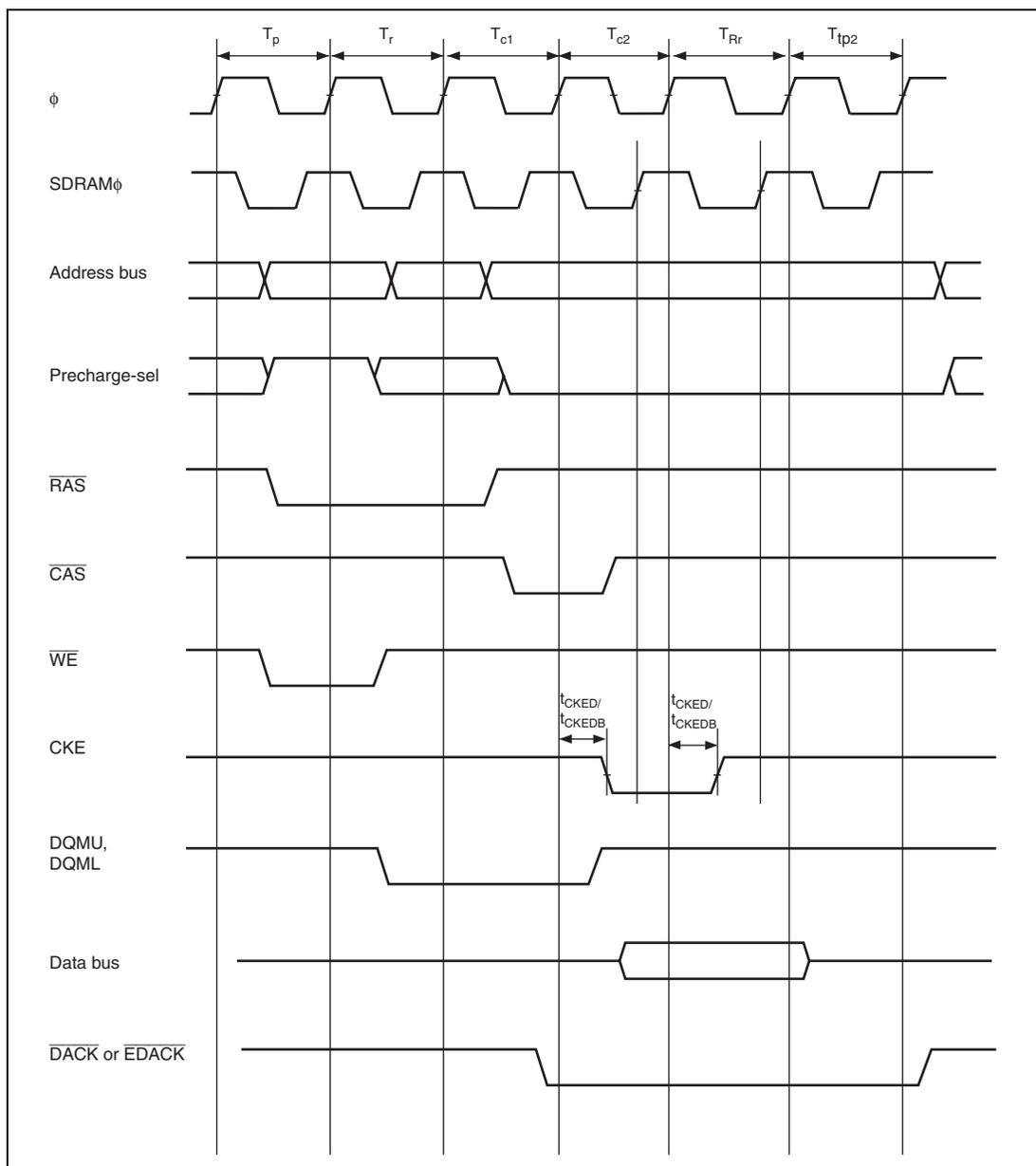
**Figure 26.28 Read Data: Two-State Expansion (CAS Latency 2)**
