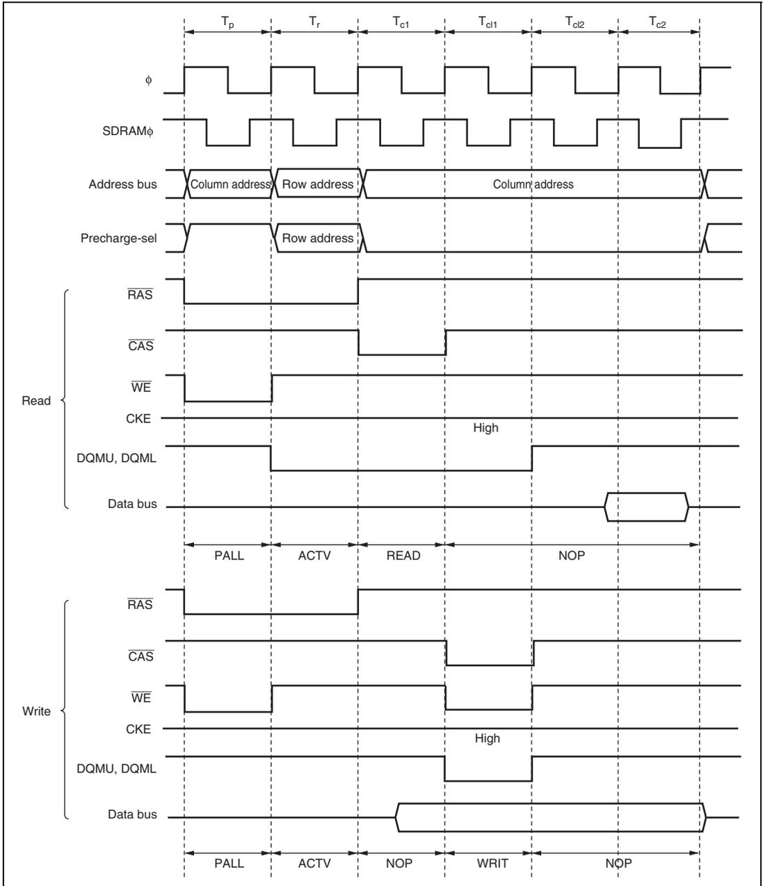
**Figure 6.57 CAS Latency Control Timing (SDWCD = 0, CAS Latency 3)**
