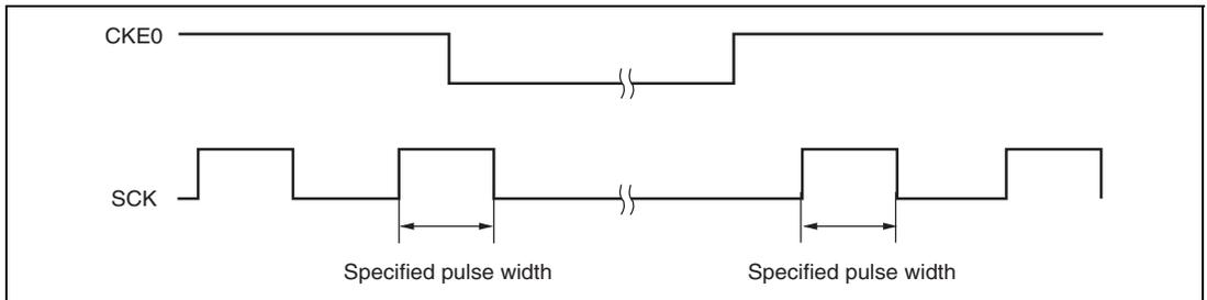
**Figure 15.31 Timing for Fixing Clock Output Level**
