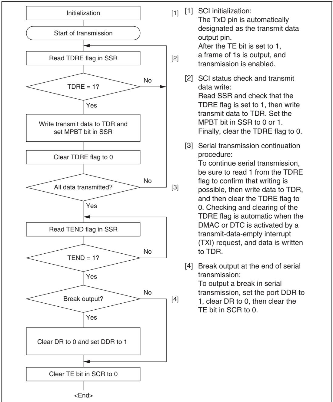
**Figure 15.11 Sample Multiprocessor Serial Transmission Flowchart**
