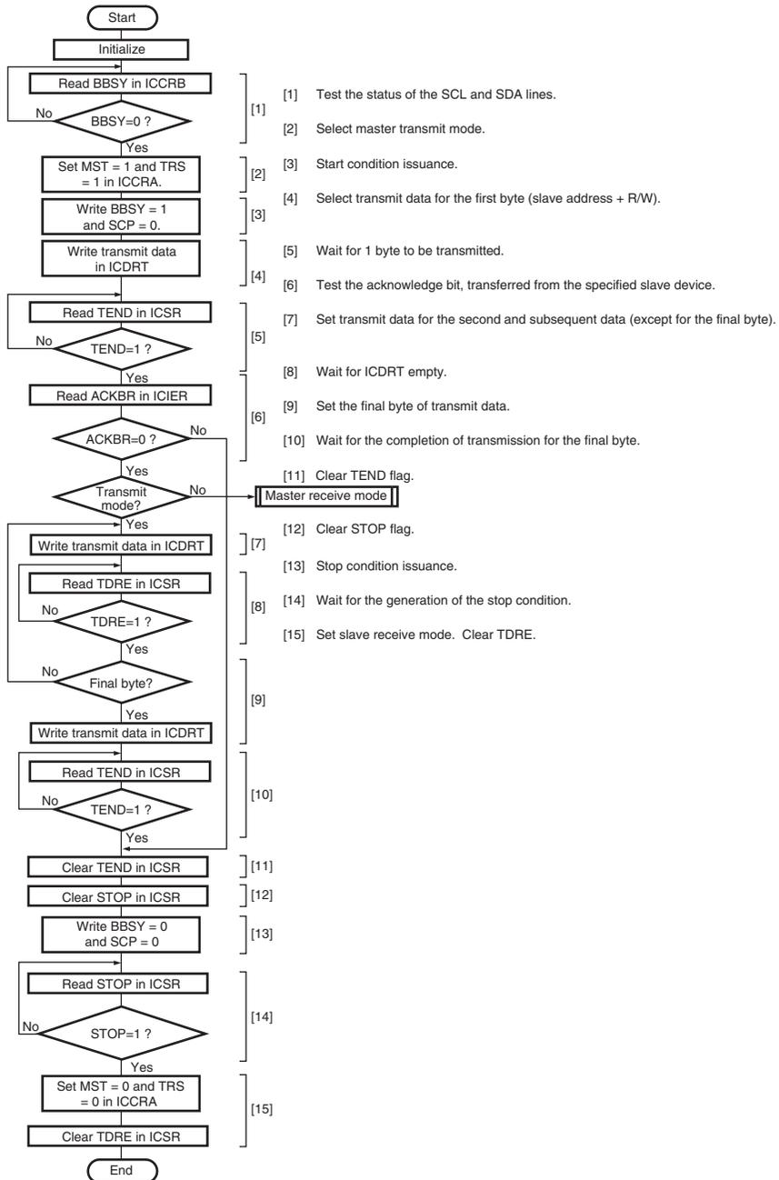
**Figure 17.14 Sample Flowchart for Master Transmit Mode**
