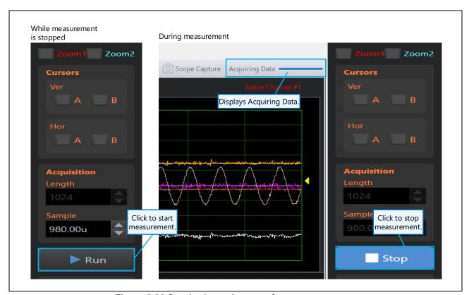
Figure 5-23 Starting/stopping waveform measurement
