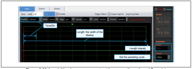
Figure 5-22 Acquisition in measurement settings area (Length and Sample)
