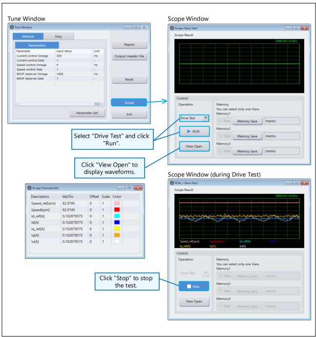
Figure 14-8 Drive Test view
