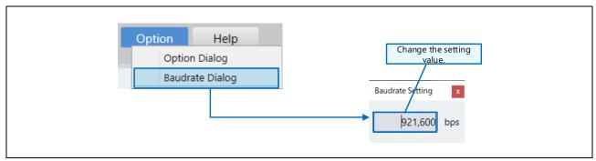
Figure 2-23 Baud rate setting
