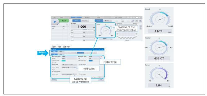
Figure 12-19 Example of setting meter
