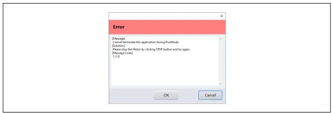
Figure 2-25 Error message for switching tools during processing.
