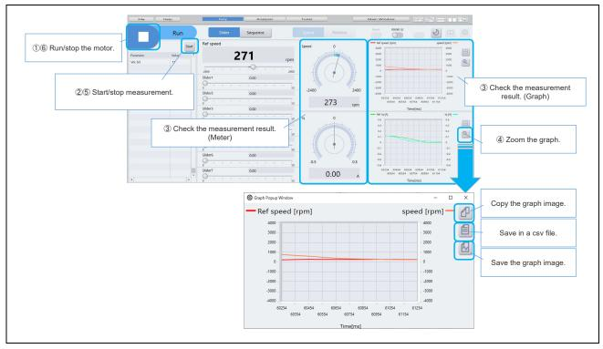
**Figure 12-9 Measurement function**
