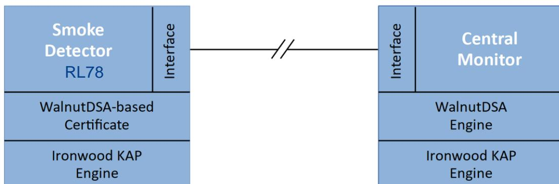
Wireless smoke, gas, and motion detectors are at risk for cyber attacks. Implementing security within the detectors enables the central monitoring station to authenticate them before acting on their messages, and to ensure that the messages they send have not been altered.
