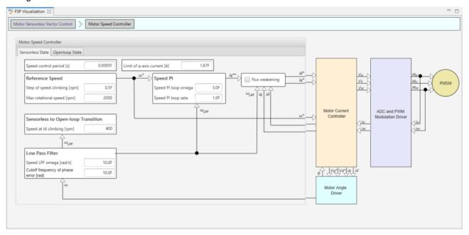
The configuration GUI is displayed on [FSP Visualization] view in e2 studio. [FSP Visualization] view is opened in [FSP Configuration] perspective. Also, [FSP Visualization] view can be opened from main menu of e2 studio, [Renesas Views]->[C/C++]->[FSP Visualization].
