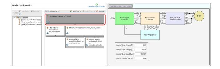
QE automatically sets the necessary settings for Renesas Motor Workbench, so you can tune and analyze the motor by clicking on the button.
