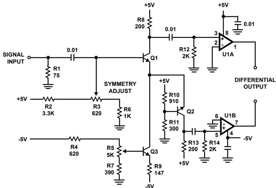
FIGURE 1. SINGLE ENDED TO DIFFERENTIAL TWISTED PAIR DRIVER
