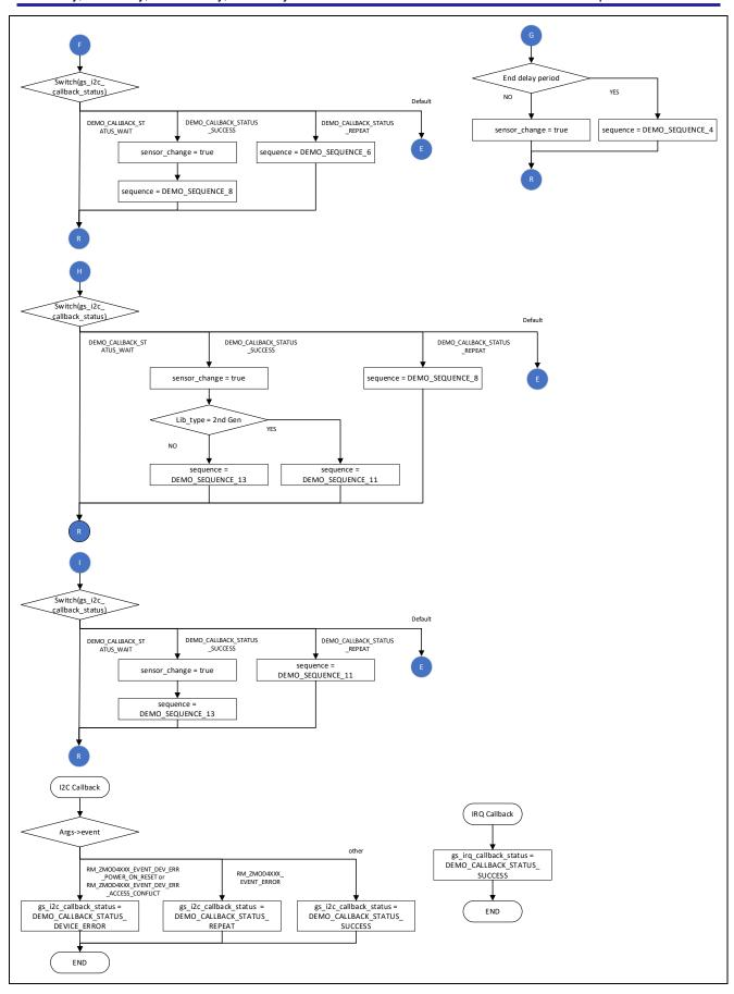
Figure 6-8 Flow 3 of ZMOD4510 Sample Software Main Processing
