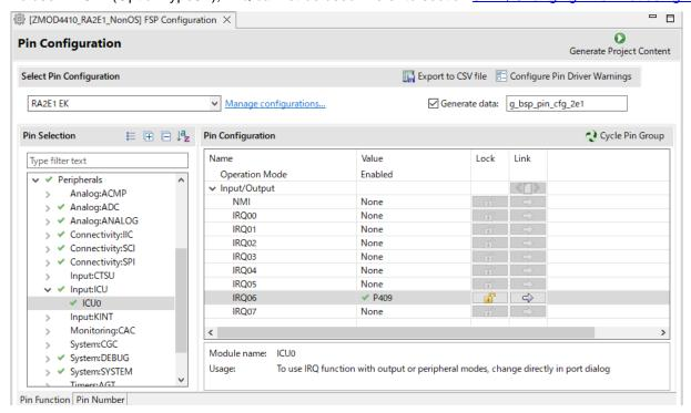
In "Select Pin Configuration", it is automatically assigned as Type 2A.
