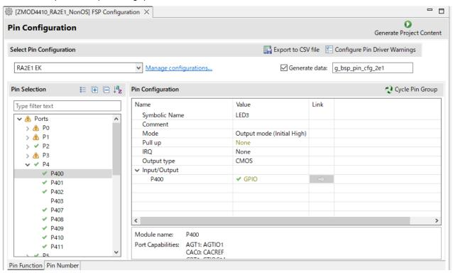
To enable generation of pin settings, check [Generate data] check-box and enter a desired name in the text field.
