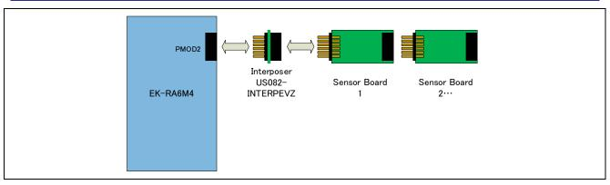
Figure 2-1 Hardware Connections for RA6M4 Family
