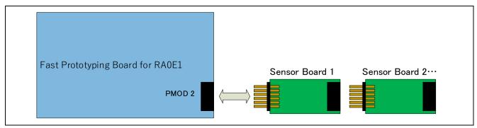
Figure 2-2 Hardware Connections for the RA0E1 Family
