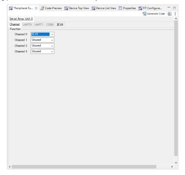
In the tabbed page for IICxx enabled in the serial array unit, set "Transfer rate" to 400000 or 100000, set "Transfer end interrupt priority" to a desired value, and enable all functions under "Callback function setting". Note: When using a serial array unit, the Nch open drain of the pin to be used is set automatically. If an error icon on the port was displayed, open the Ports tab and check the port settings.
