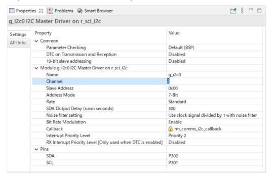
(b) When using the different I2C driver as the original sample project
