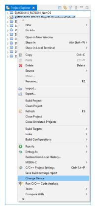
Select a desired board or device in the "Change Device" window and press the [Next] button.
