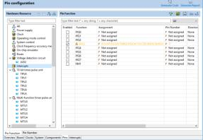
As the use of PMOD Type 2A (extended SPI) is specified in the RSK RX231 board information, a warning message will appear when I2C is used, but this does not produce any problems.
