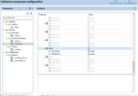
And IRQ3 is assigned to PMOD on the RSK RX231 board, check the settings of "IRQ3 Pin" for "Interrupts" under "Resources" in  $r_{irq_rx}$  and change the settings of "IRQ number for ZMOD4XXX sensor device0" to "IRQ3" in  $r_{zmod4xxx_rx}$ .
