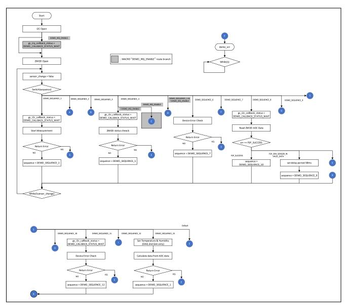
Figure 6-6 Flow 1 of ZMOD4510 Sample Software Main Processing
