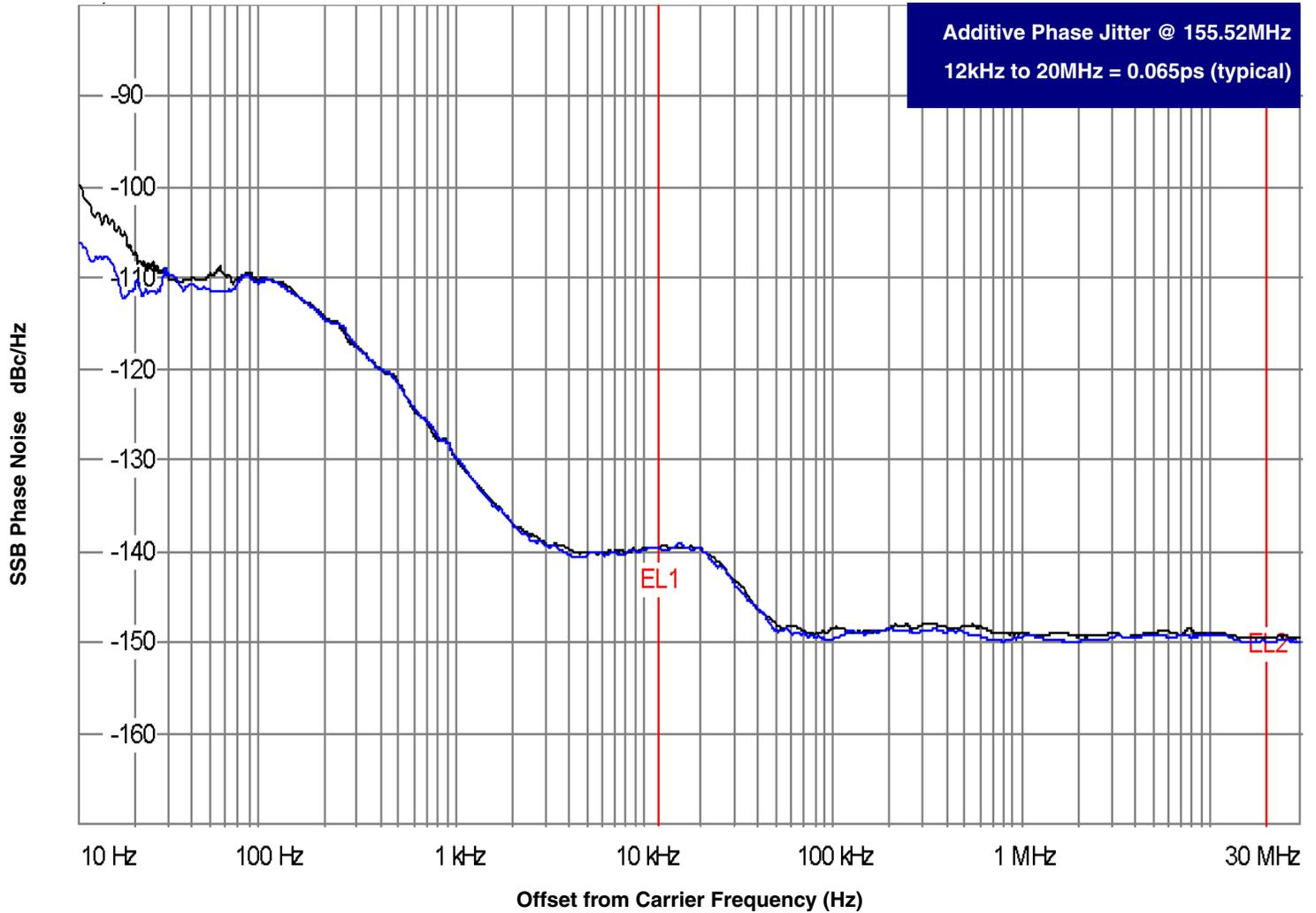
As with most timing specifications, phase noise measurements has issues relating to the limitations of the equipment. Often the noise floor of the equipment is higher than the noise floor of the device. This is illustrated above. The device meets the noise floor of what is shown, but can actually be lower. The phase noise is dependent on the input source and measurement equipment.
