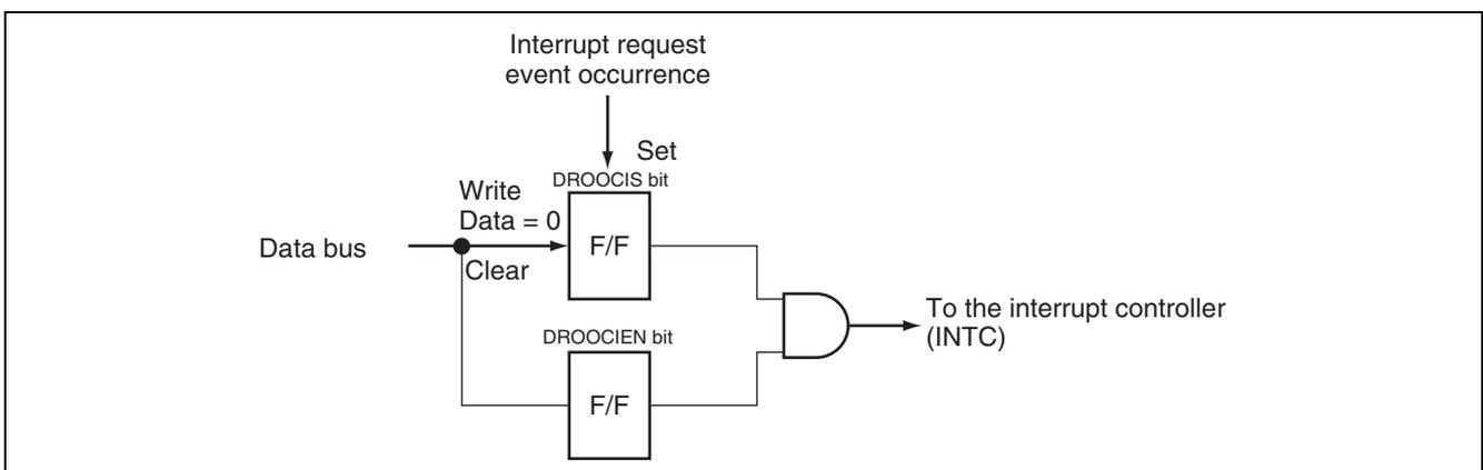
**Figure 29.2 Relationship Between DROIST and DROIEN Registers**
