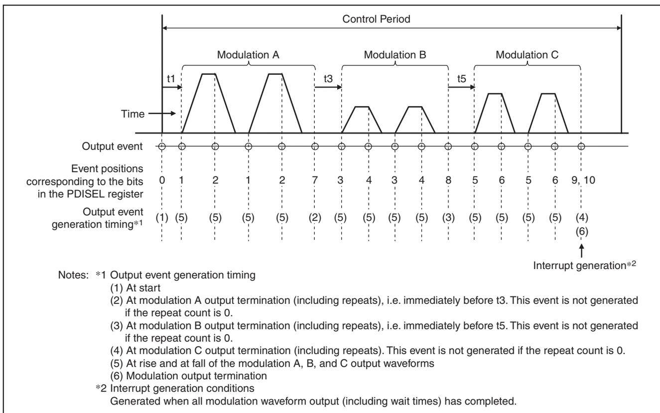
Figure 30.12 Output Event and Interrupt Generation Timing
