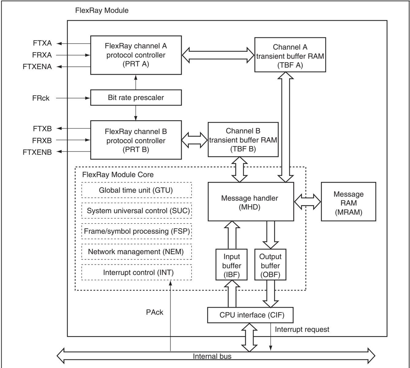
Figure 32.1 Block Diagram of FlexRay Module
