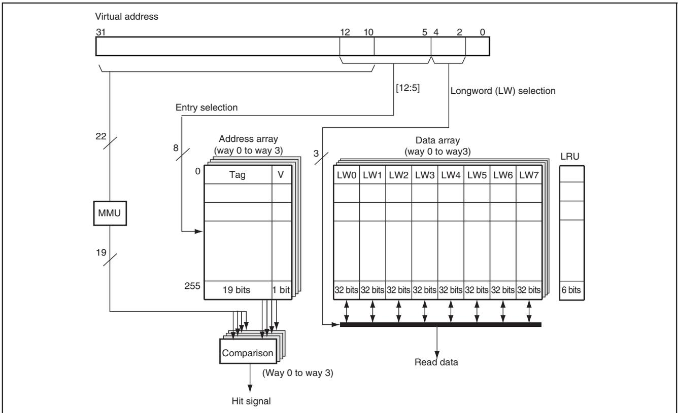
Figure 8.2 Configuration of Instruction Cache (Cache size = 32 Kbytes)
