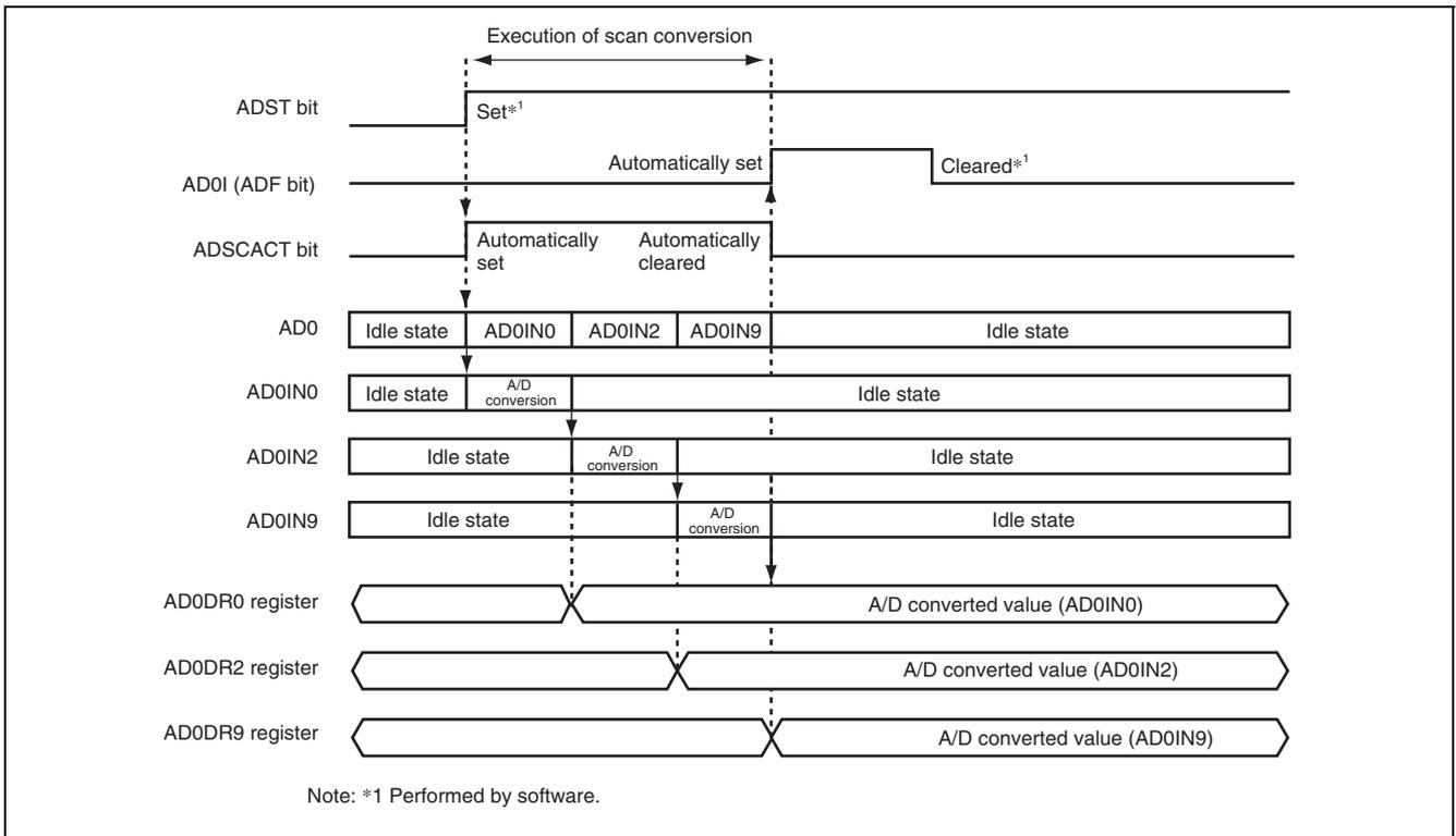
**Figure 27.4 Example Operation in Single-Cycle Scan Mode**
