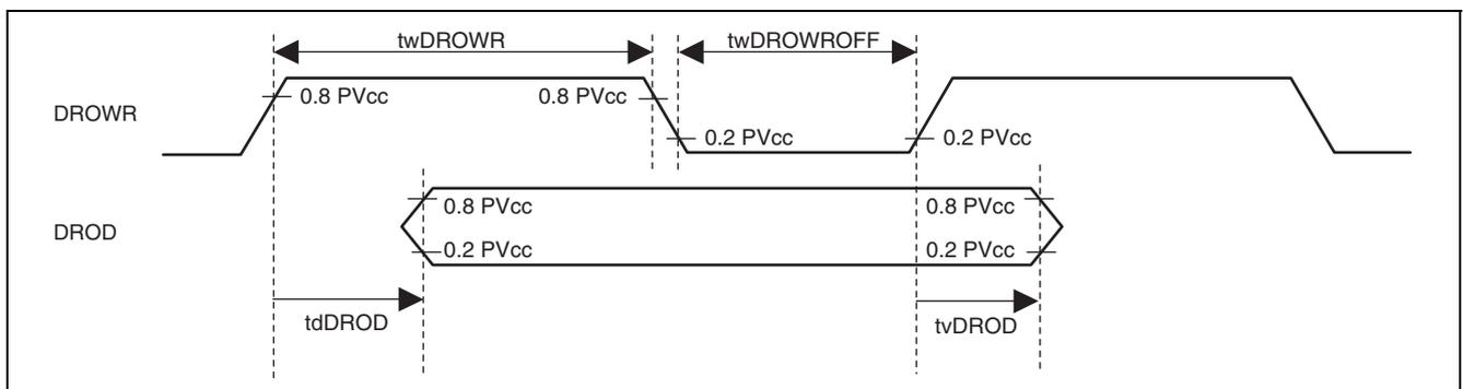
**Figure 38.38 Strobe Polarity with "H" Active Selected**
