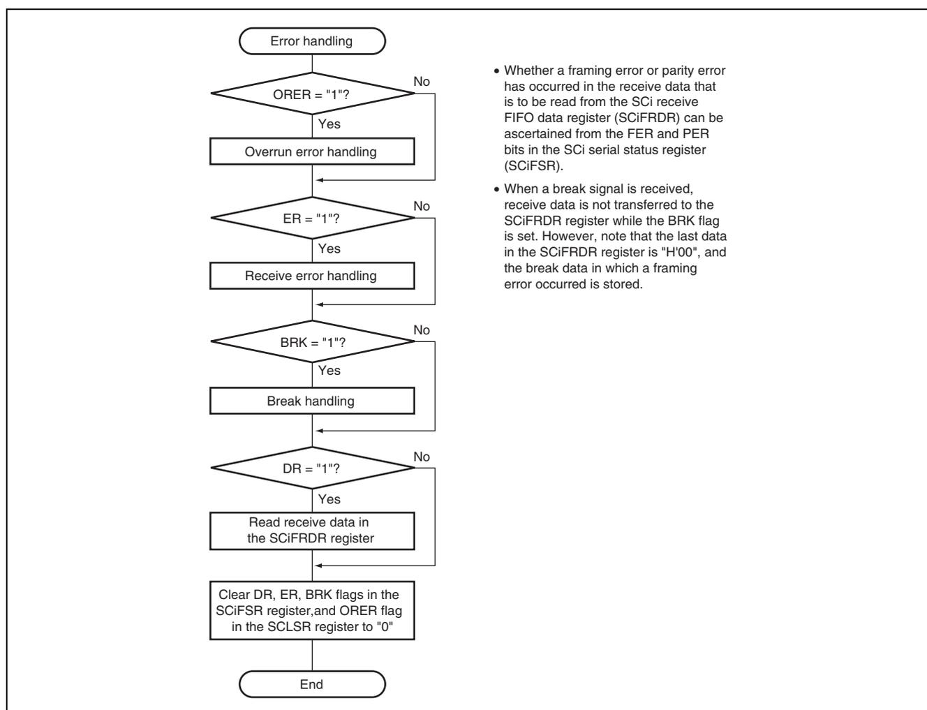
**Figure 23.8 Sample Flowchart for Receiving Serial Data (2)**
