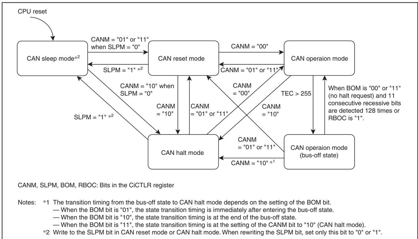
Figure 26.9 Transition between CAN Operating Modes (i = 0 to 4)
