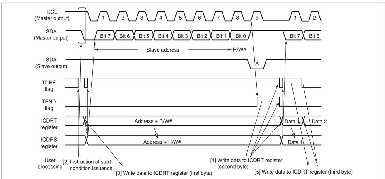
Figure 25.5 Master Transmit Mode Operation Timing (1)
