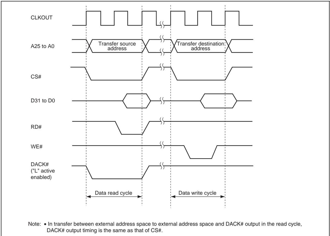
**Figure 20.16 Example of DACK# Signal Output Timing**
