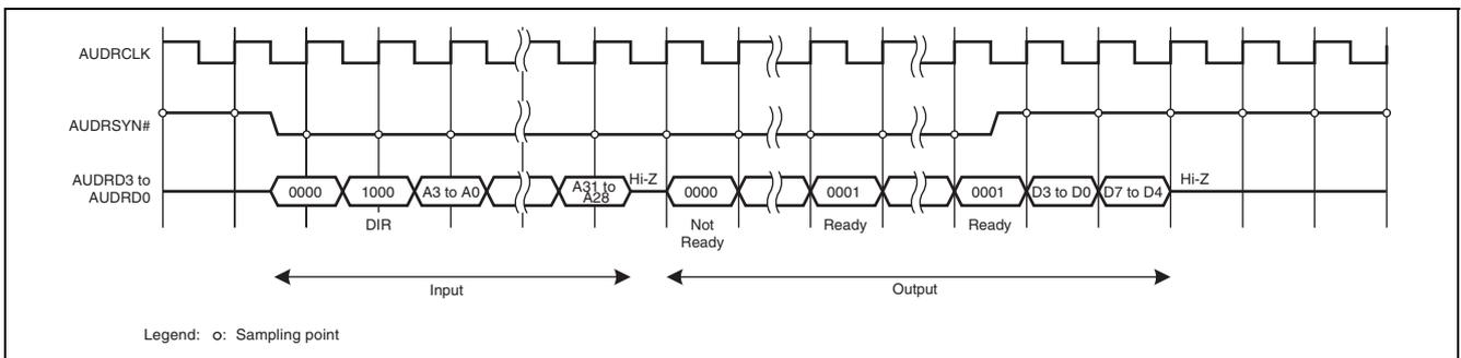
**Figure 36.5 Read Operation Example (byte read)**
