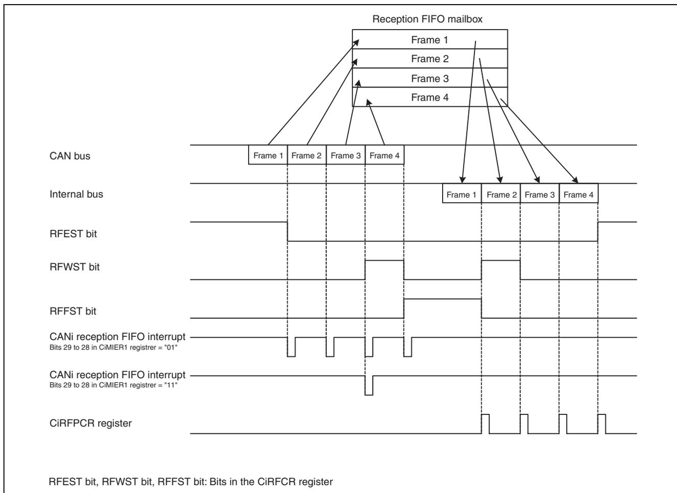
**Figure 26.2 Receive FIFO Mailbox Operation (Bits 29 and 28 in CiMIER1 Register = "01" and "11")
