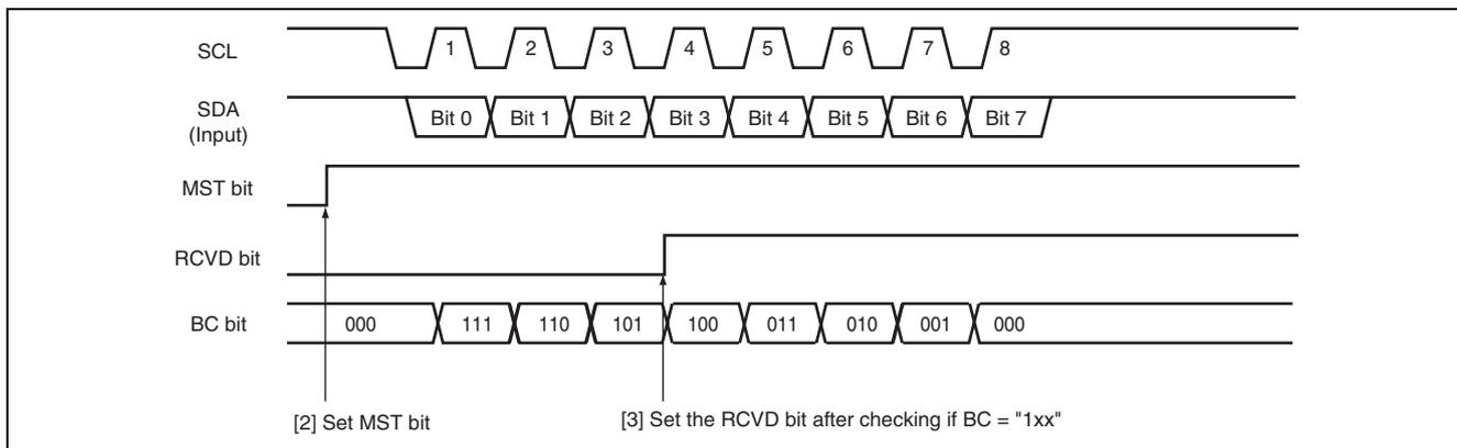
**Figure 25.16 Operation Timing For Receiving One Byte (MST = "1")**
