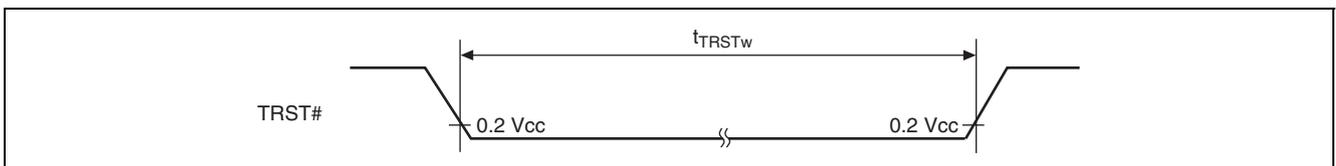
**Figure 38.44 TRST# Input Timing**
