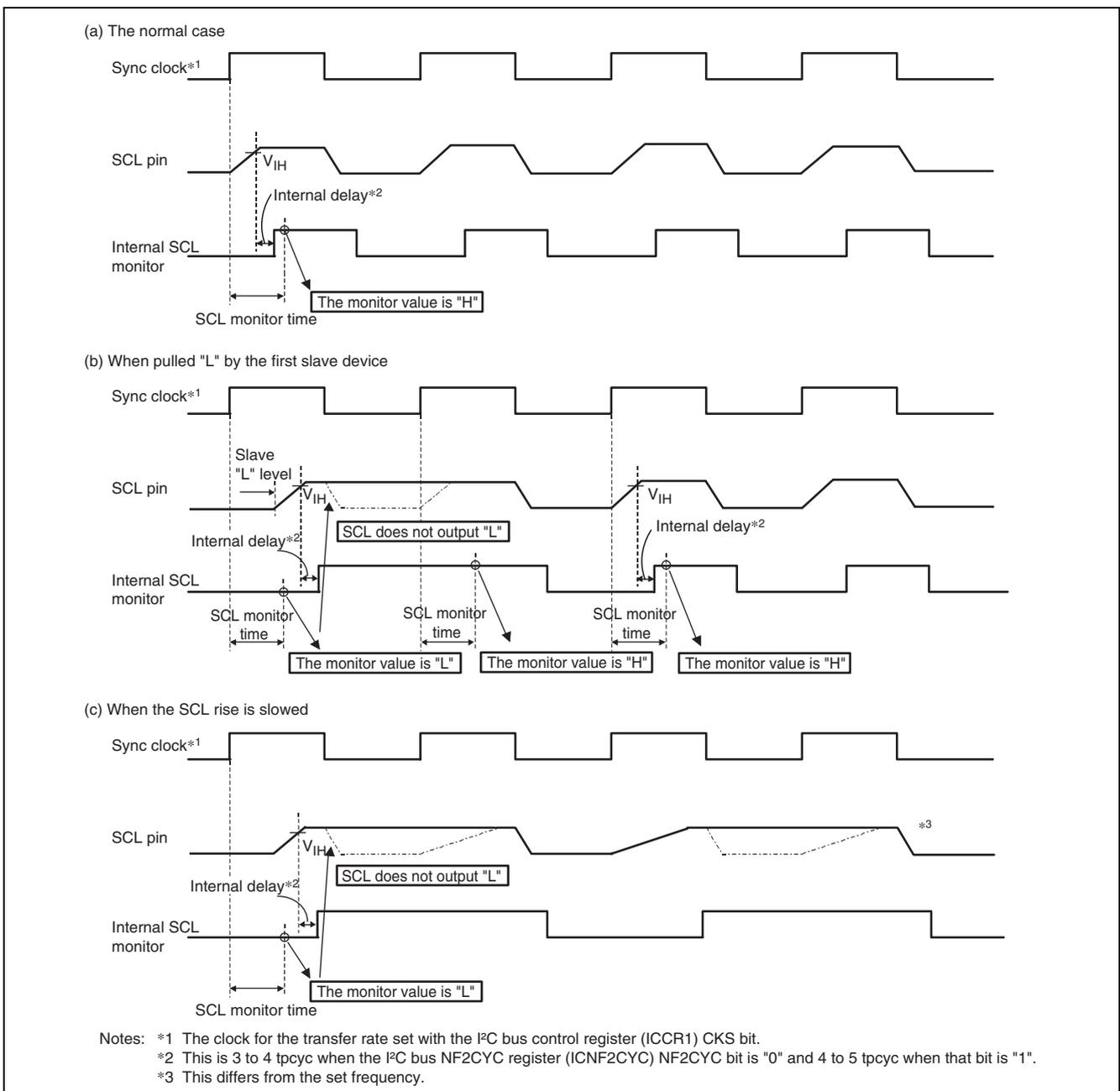
**Figure 25.23 Bit Synchronous Circuit Timing**
