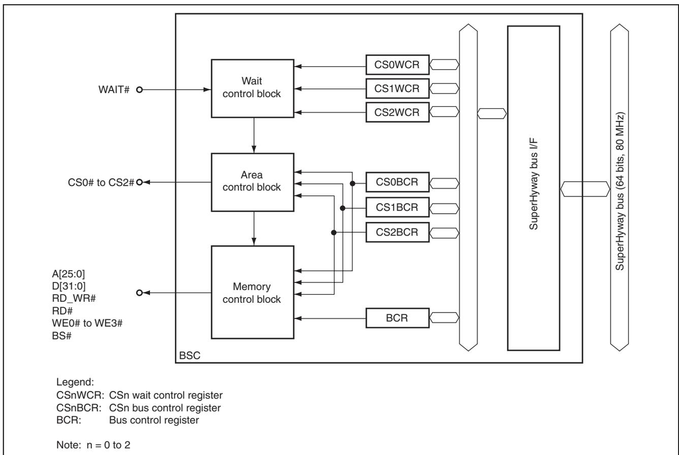
Figure 19.1 Block Diagram of BSC
