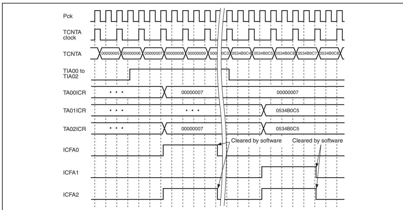
Figure 21.12 Example of Input Capture of Timer A
