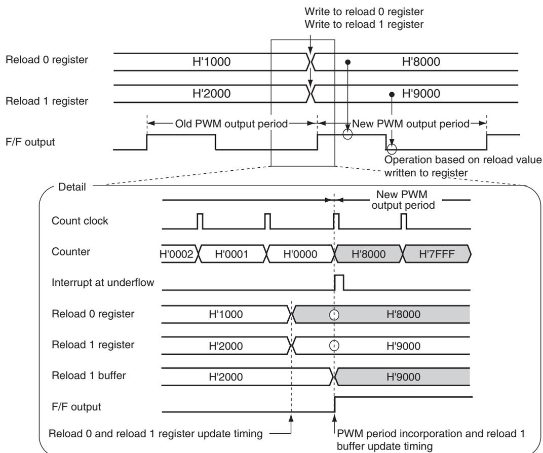
**Figure 21.30 Reload 0 and Reload 1 Register Updating in PWM Output Mode**
