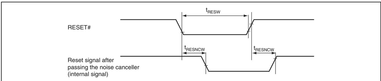
**Figure 38.9 Reset Input Timing**
