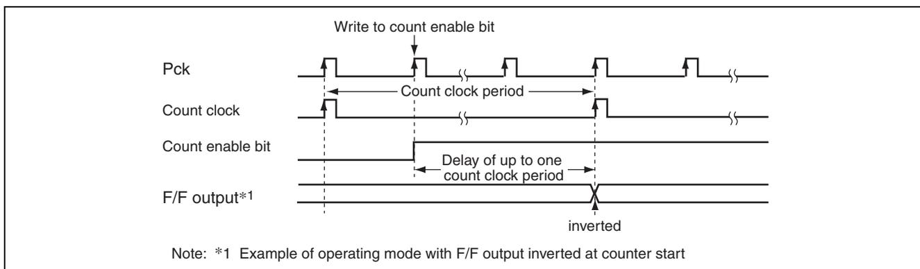
Figure 21.26 Count Clock Delay
