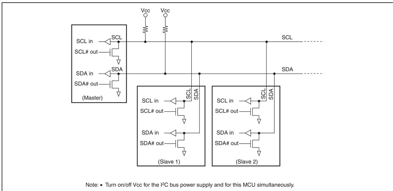
**Figure 25.2 External Circuit Connections of I/O Pins**
