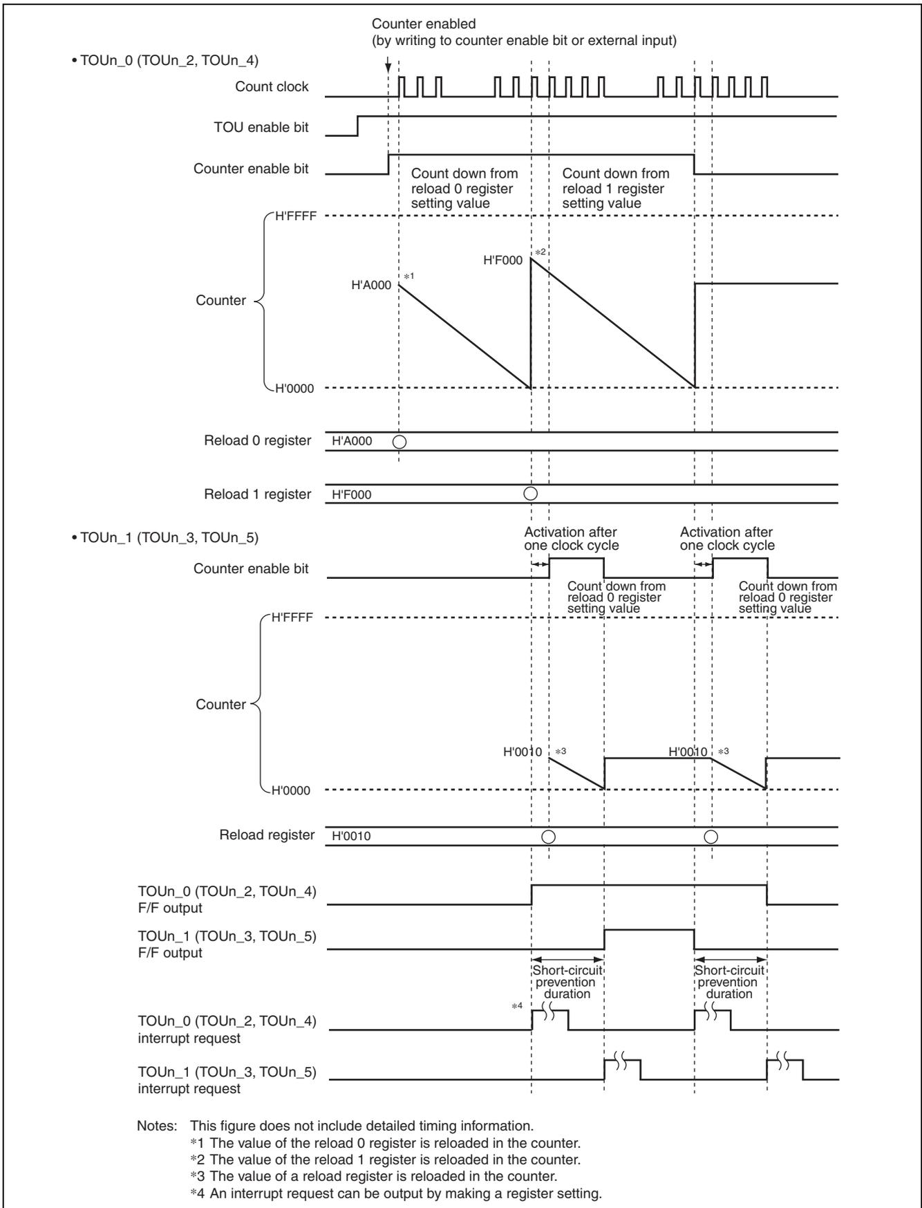
Figure 21.44 Overview of Short-Circuit Prevention Function Operation
