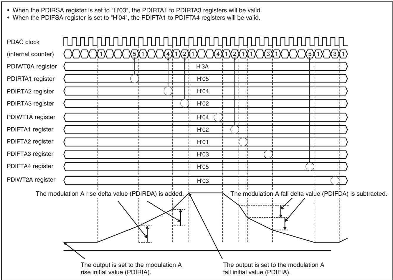
**Figure 30.16 Modulation Waveform Output Timing (Example: Modulation A)**
