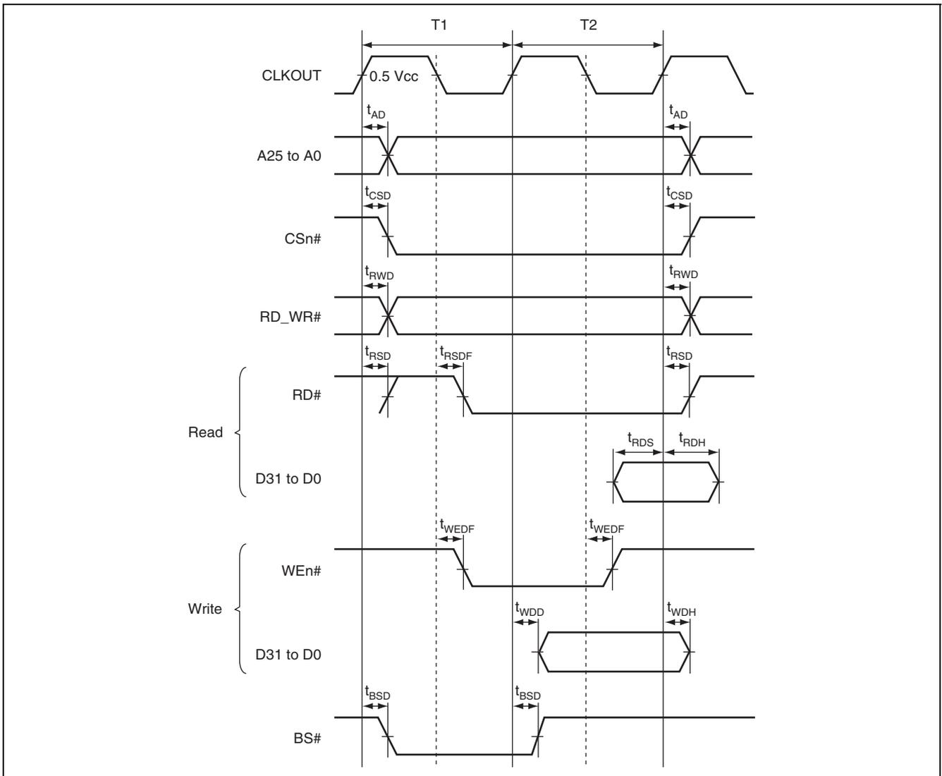
Figure 38.12 SRAM Bus Cycle (No Waits)
