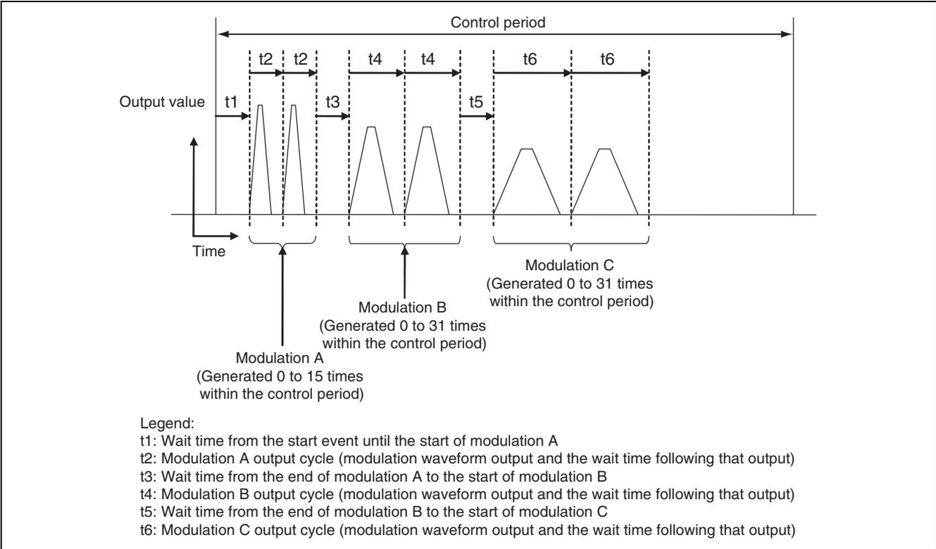
Figure 30.4 PDAC Module Control Period Operation Overview
