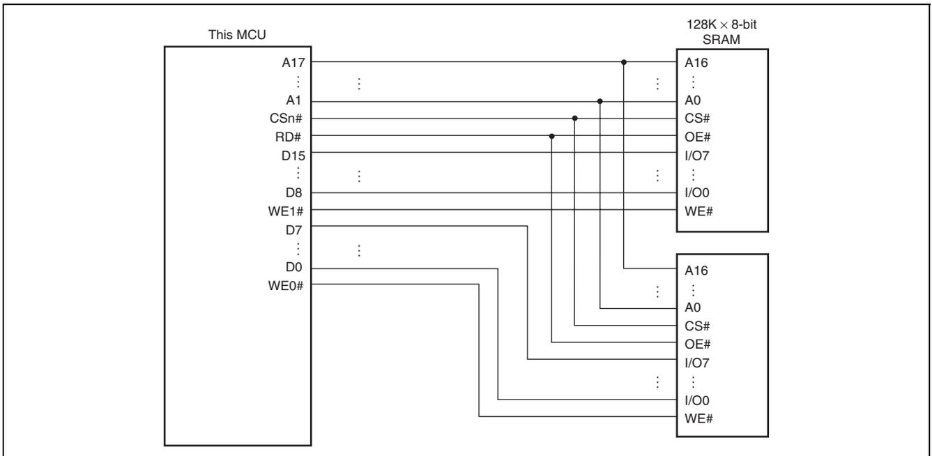
**Figure 19.5 Example of 16-Bit Data-Width SRAM Connection**
