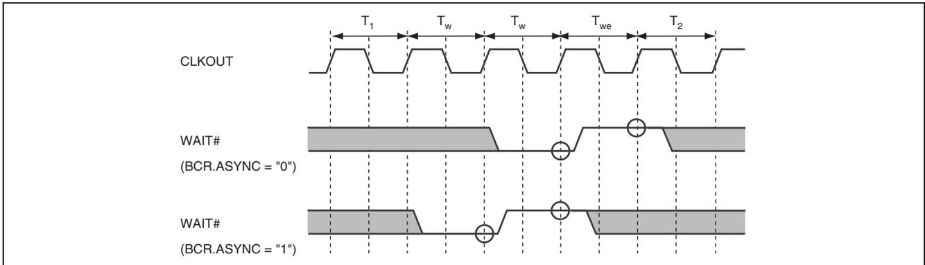
**Figure 19.2 BCR.ASYNC Setting WAIT# Sampling Timing Example**
