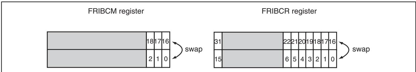
**Figure 32.13 Swapping of Bits in Registers FRIBCM and FRIBCR**
