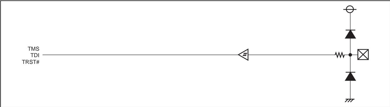
Figure 18.9 Port Peripheral Circuit Diagram (Input Port 5)
