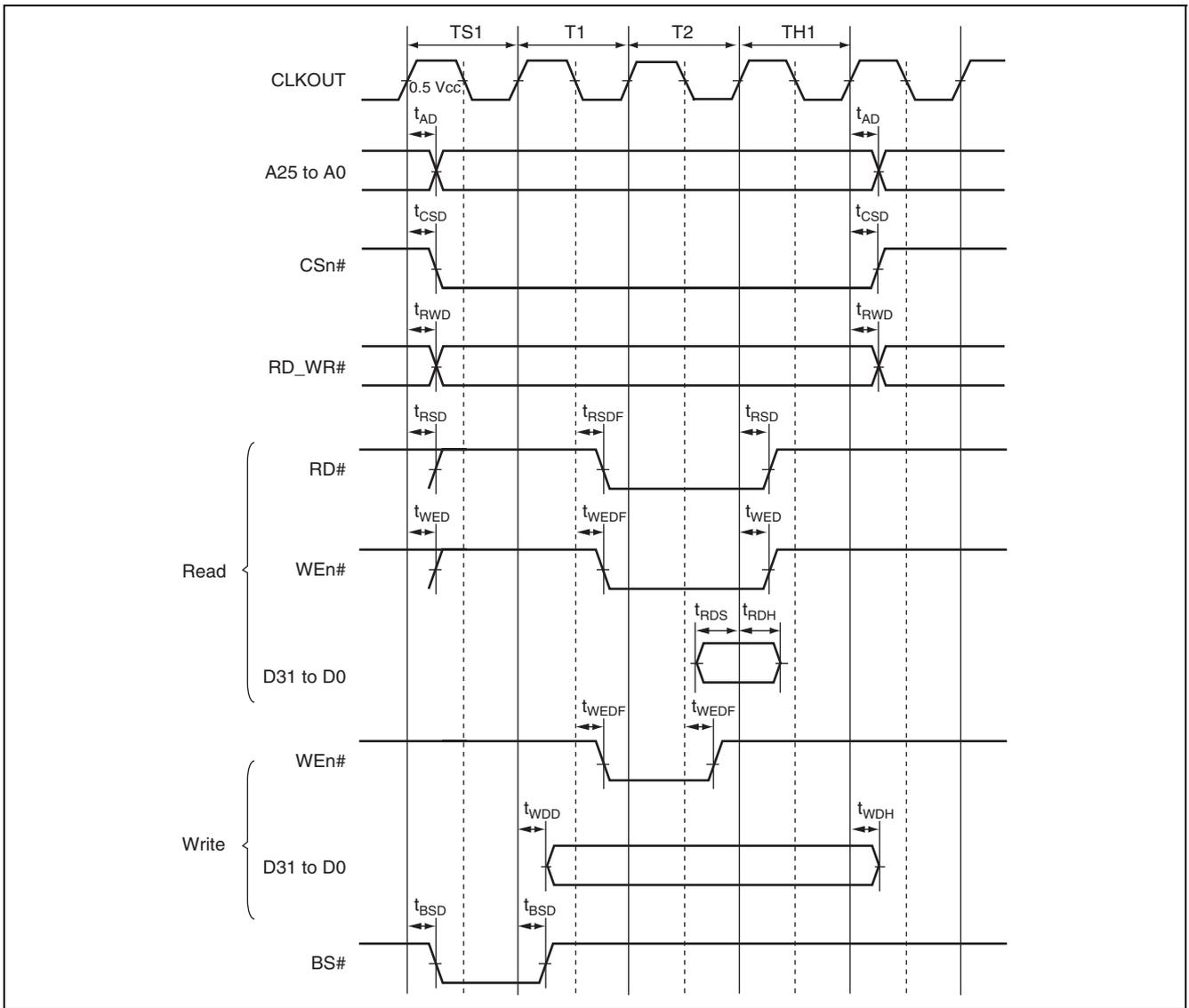
**Figure 38.19 SRAM Bus Cycle with Byte Control**
