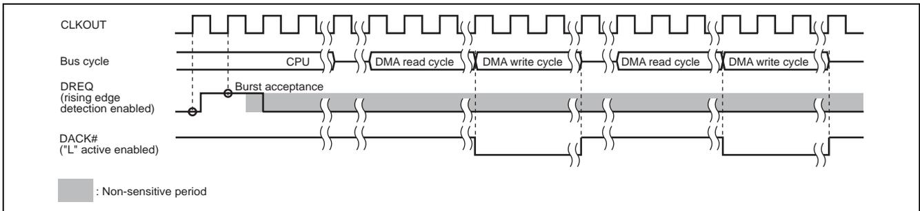
**Figure 20.15 Example of DREQ Input Detection (Burst mode, DACK Write Cycle Output)**
