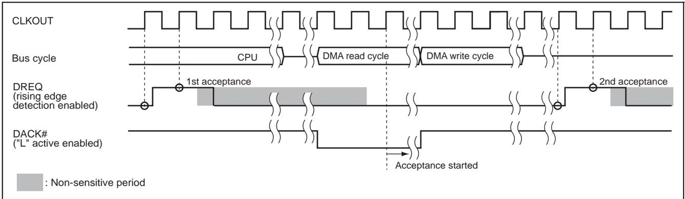
**Figure 20.10 Example of DREQ Input Detection (Cycle Steal Mode 1, DACK Read Cycle Output)**
