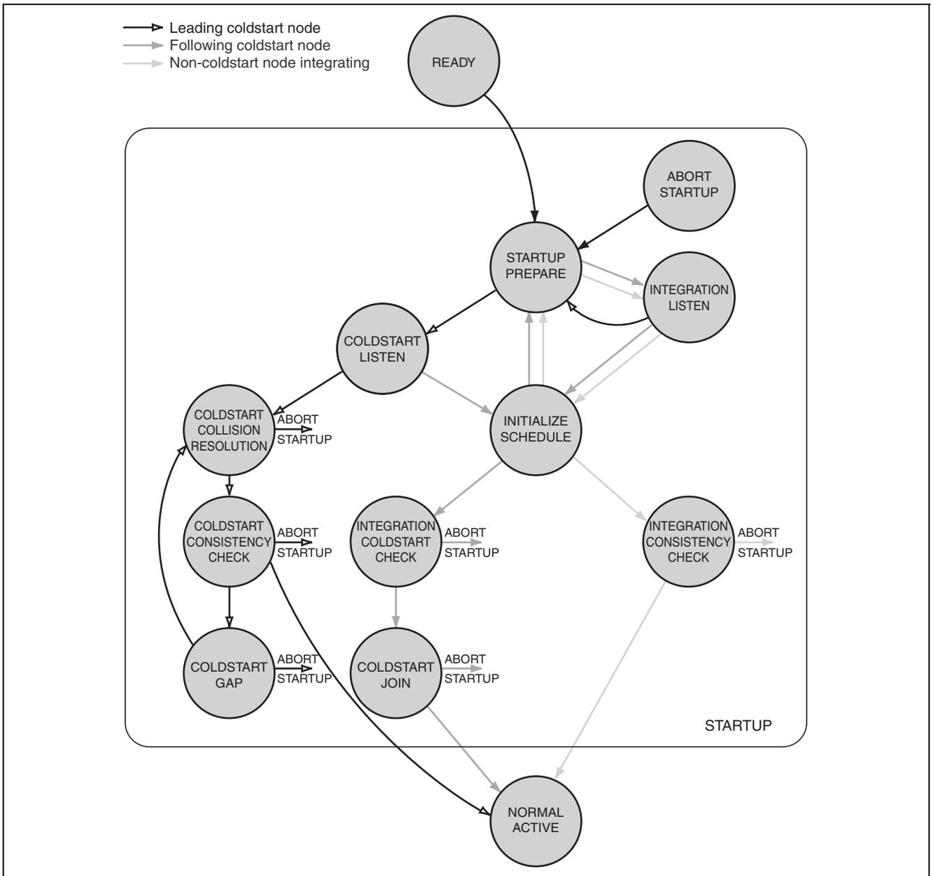
Figure 32.9 State Diagram Time-Triggered Startup
