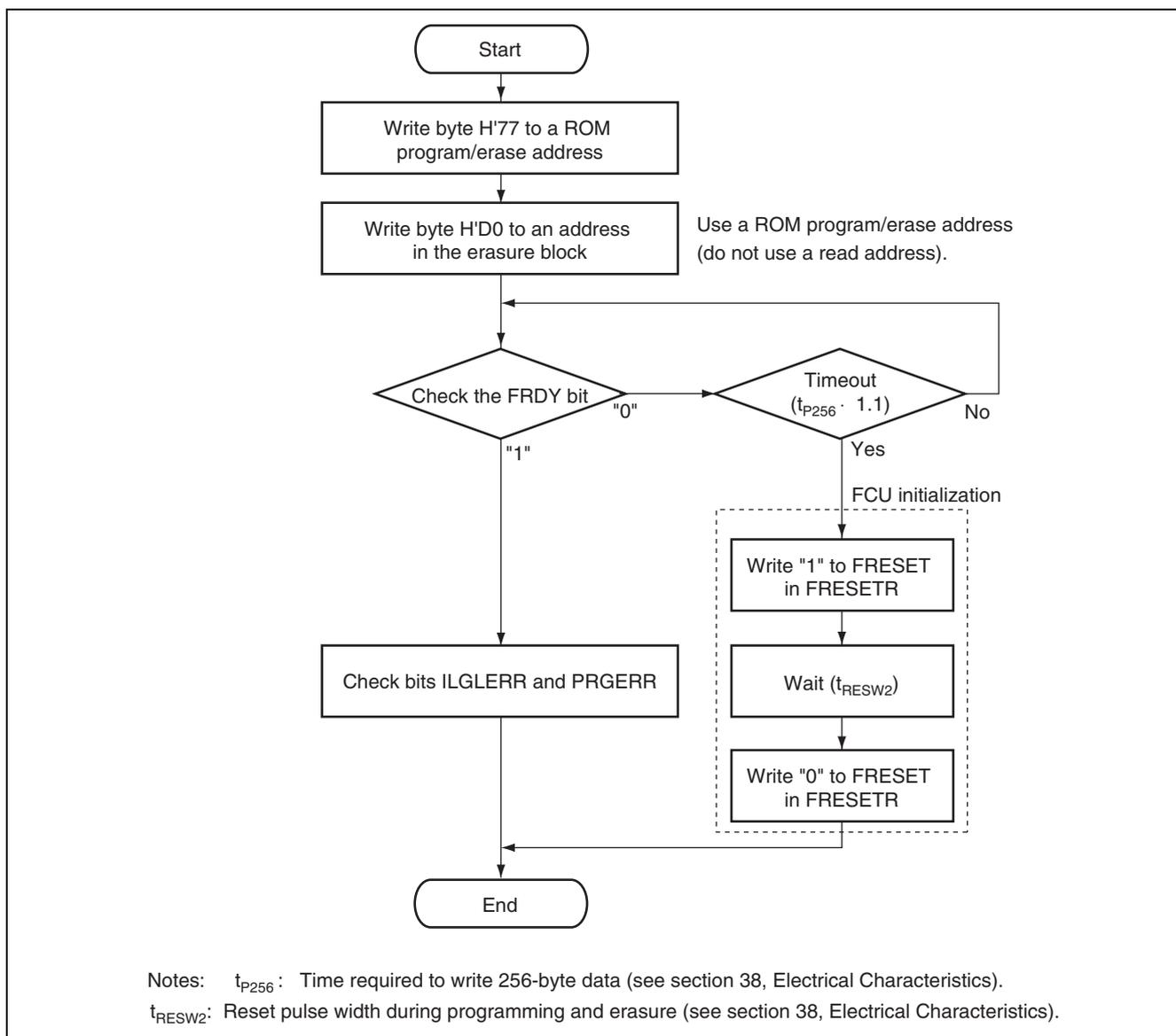
**Figure 12.15 Procedure for Writing to the Lock Bit**
