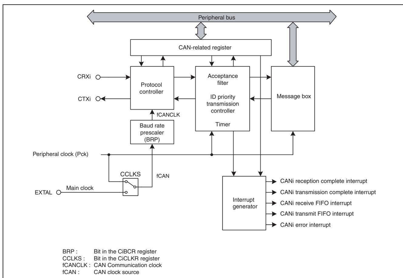
**Figure 26.1 Block Diagram of CAN Module (i = 0 to 4)**
