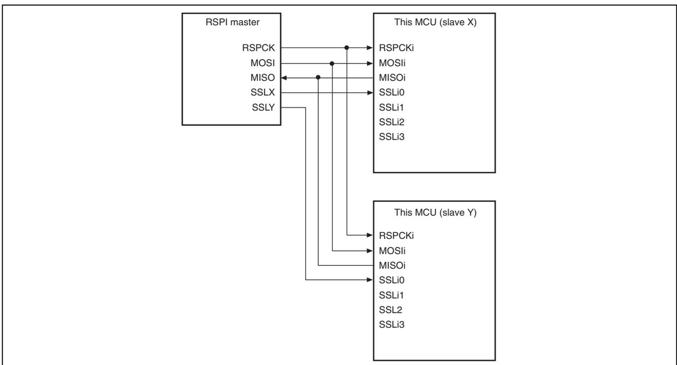
**Figure 24.7 Single-Master/Multi-Slave Configuration Example (This MCU = Slave)**
