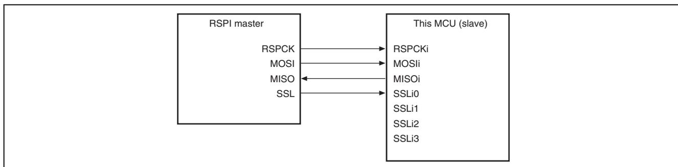
**Figure 24.4 Single-Master/Single-Slave Configuration Example (This MCU = Slave)**
