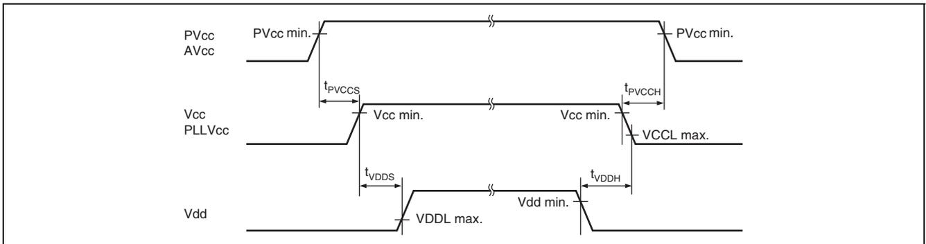
**Figure 38.4 Power-On/Off Timing**
