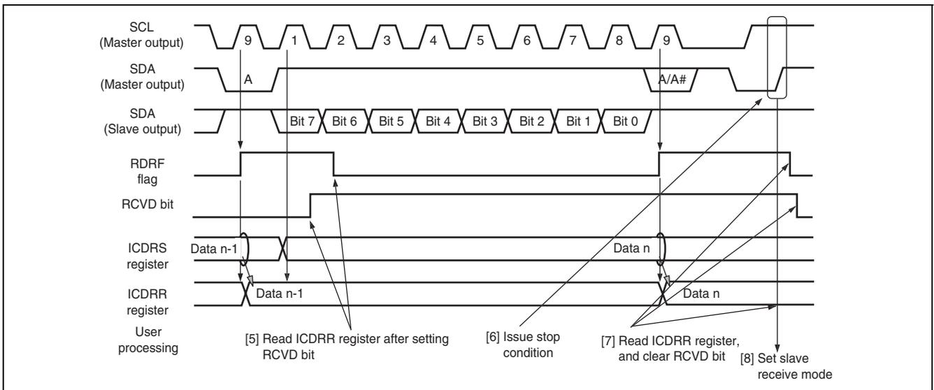
**Figure 25.8 Master Receive Mode Operation Timing (2)**
