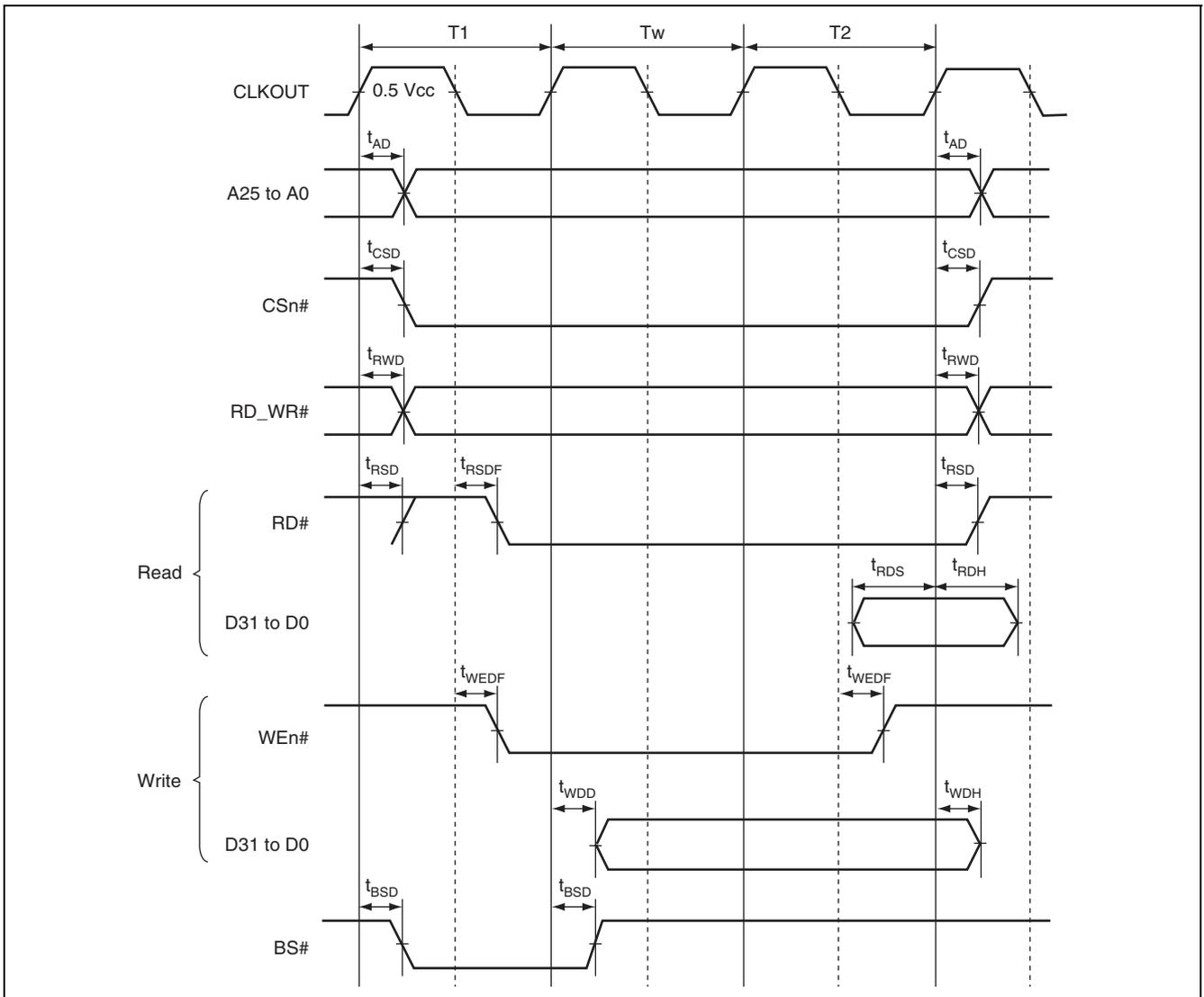
Figure 38.13 SRAM Bus Cycle (One Software Wait Cycle)
