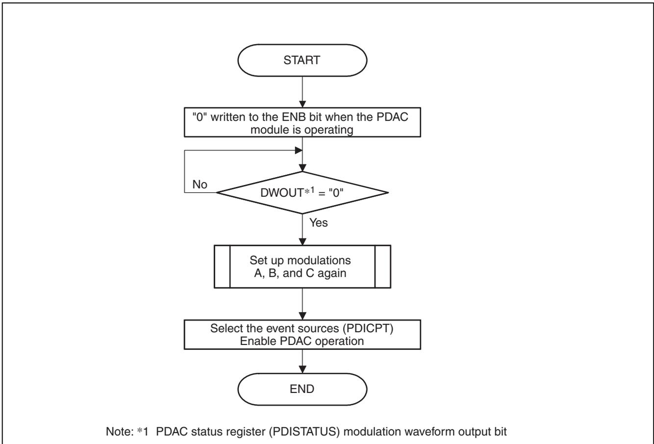
**Figure 30.14 Example Procedure for Register Modification During PDAC Operation**
