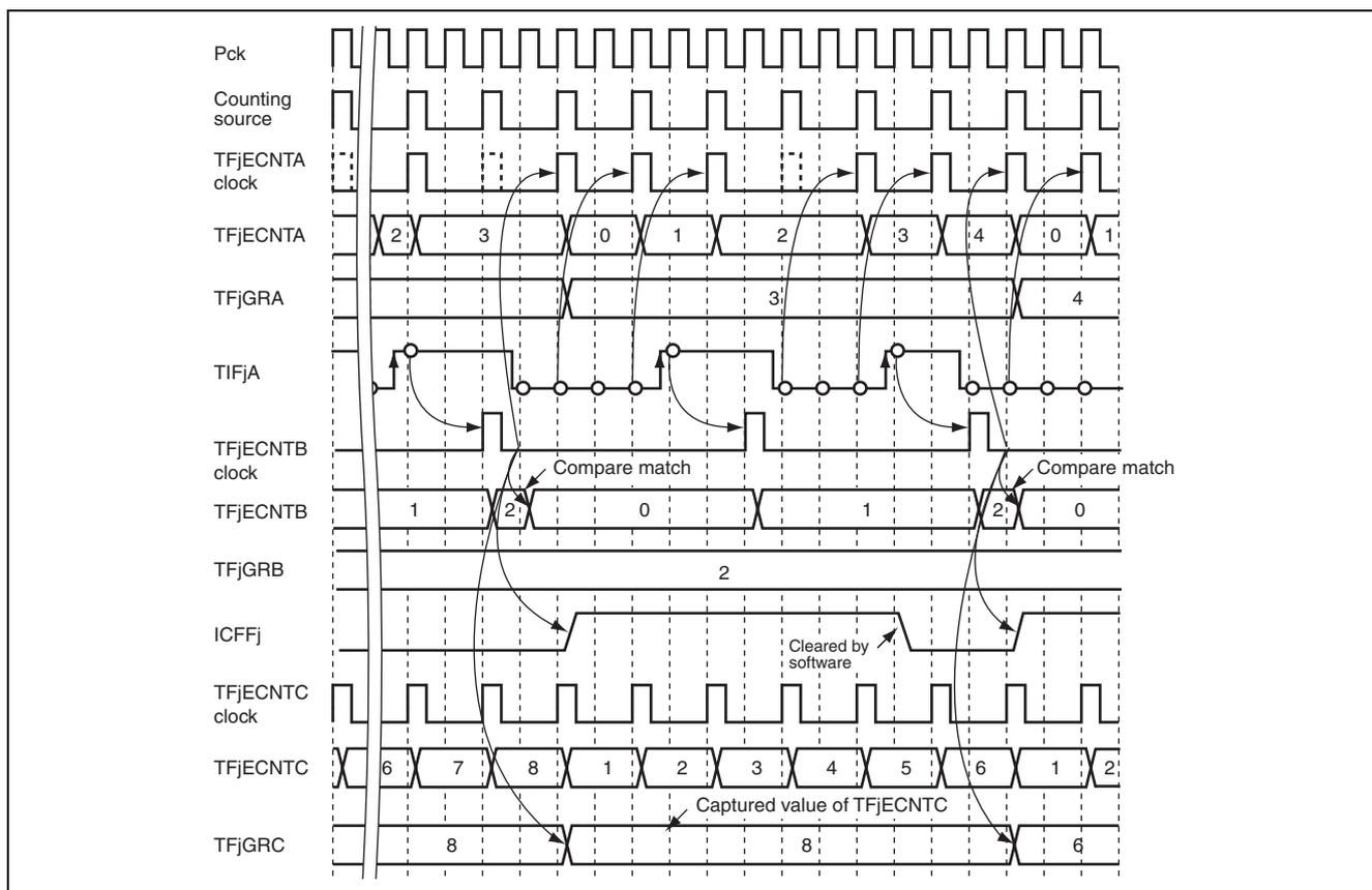
**Figure 21.19 Operation Example of Measurement of PWM Input Waveform Timing**
