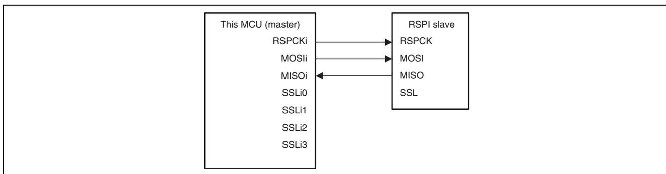
**Figure 24.9 Master (Clock-Synchronous Operation)/Slave (Clock-Synchronous Operation) Configuration Example (This MCU = Master)**
