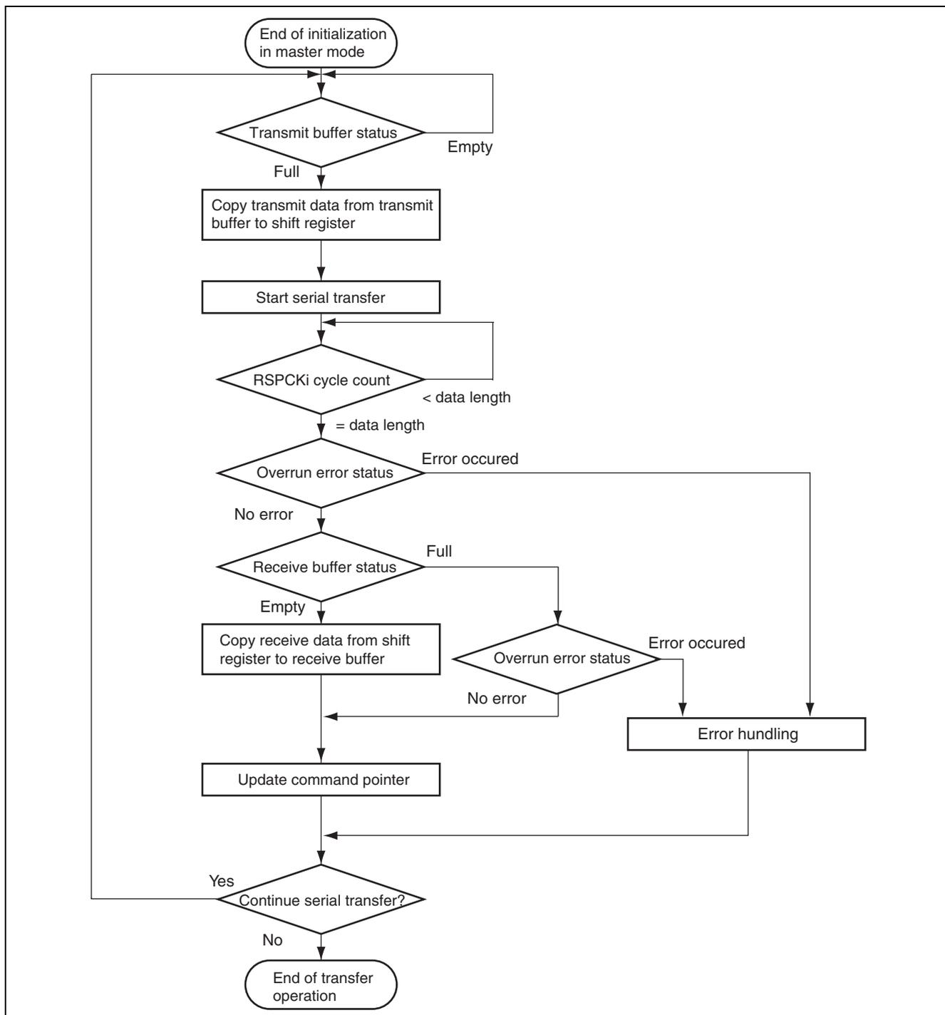
**Figure 24.28** Flowchart of Transfer Operation in Master Mode
