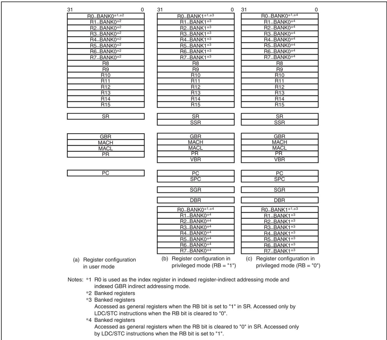
**Figure 2.2 CPU Register Configuration in Each Processing Mode**
