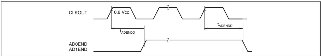
**Figure 38.42 Analog Conversion Timing**
