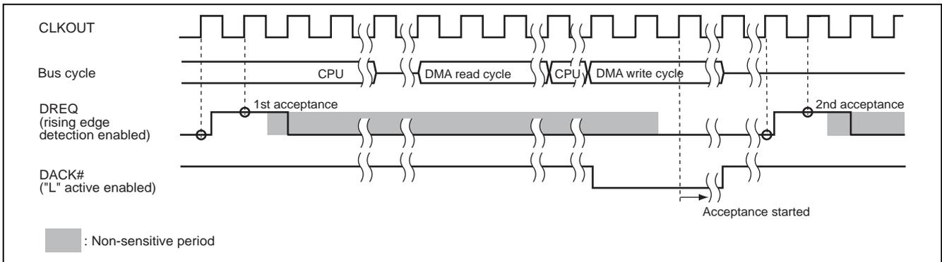
**Figure 20.13 Example of DREQ Input Detection (Cycle Steal Mode 2, DACK Write Cycle Output)**
