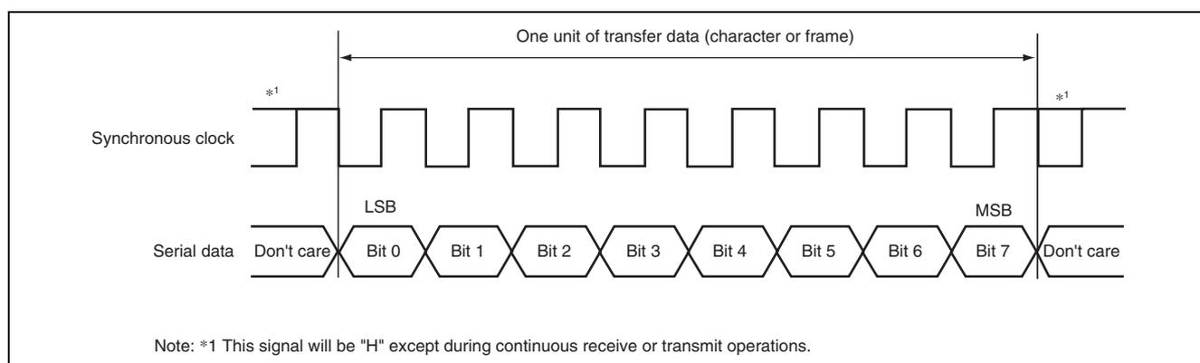
**Figure 23.11 Data Format in Clock Synchronous Communication**
