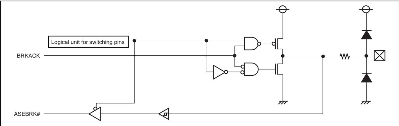
Figure 18.4 Port Peripheral Circuit Diagram (Input/Output Ports 4)
