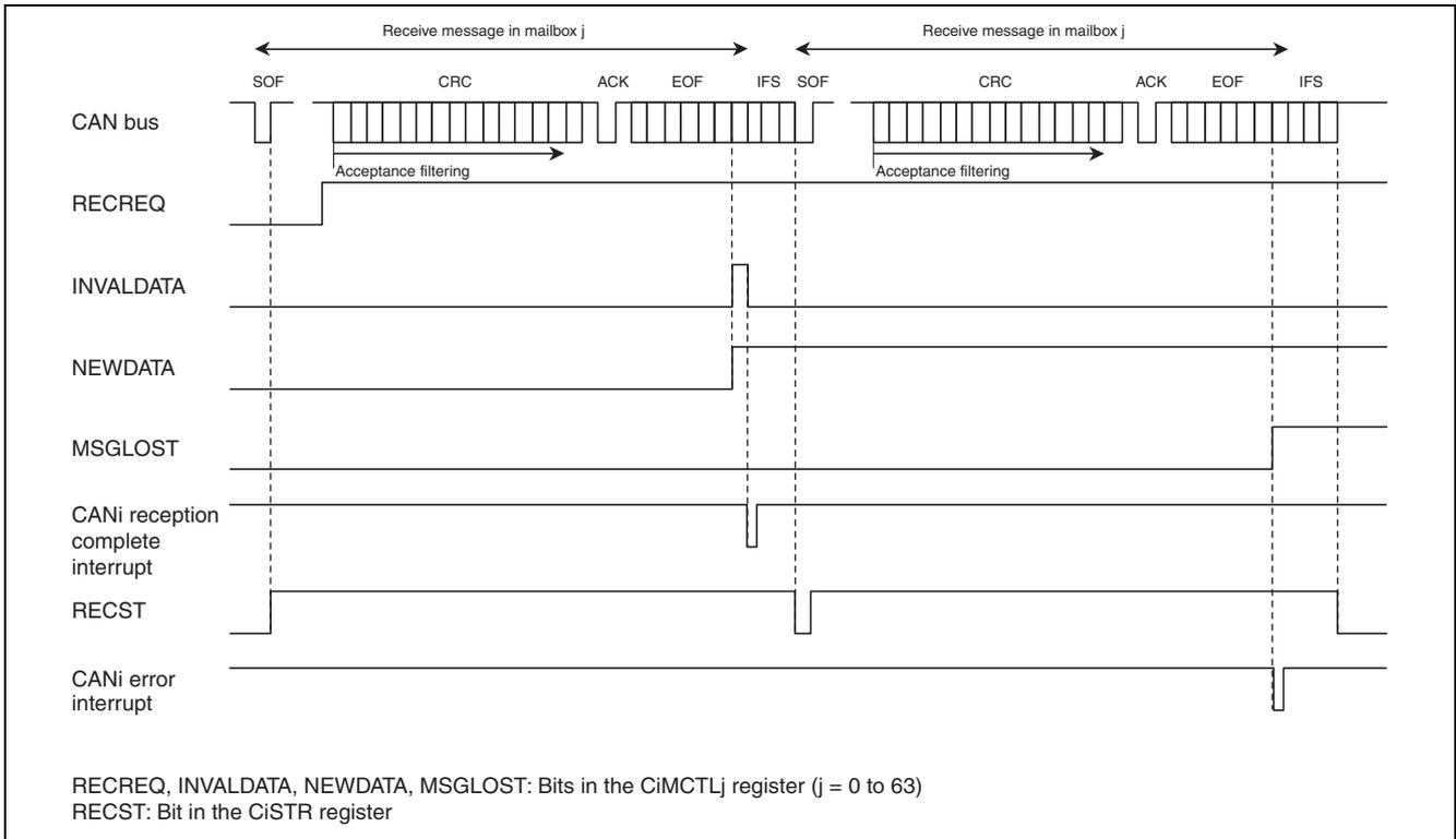
**Figure 26.19 Operation Example of Data Frame Reception in Overrun Mode (i = 0 to 4)**
