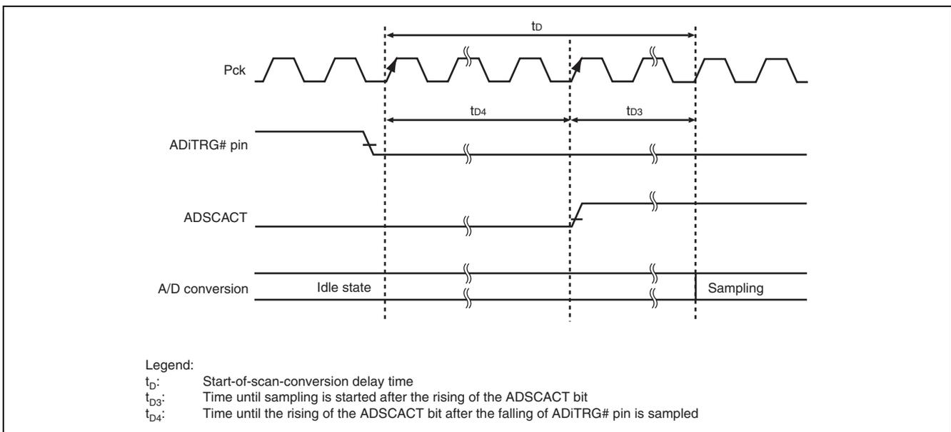
**Figure 27.9 External Trigger Input Timing****27.5.9 Starting Scan Conversion with ATU-IIIS Timer Trigger**
