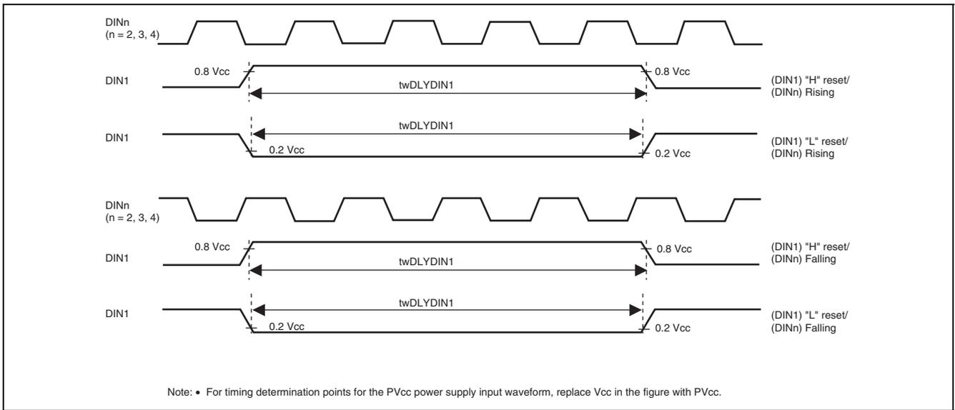
**Figure 38.36 Minimum Edge Count at DIN1 Initialization Level in Delayed Reset Mode (Minimum Width at Initialization Level)**
