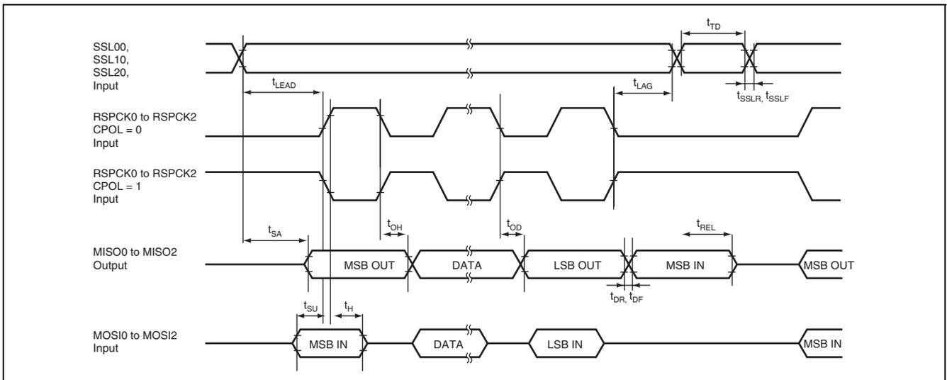
Figure 38.30 RSPI Timing (Slave, CPHA = "0")
