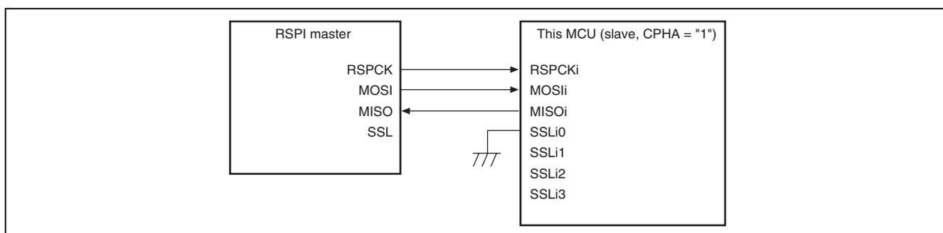
**Figure 24.5 Single-Master/Single-Slave Configuration Example (This MCU = Slave, CPHA = "1")**
