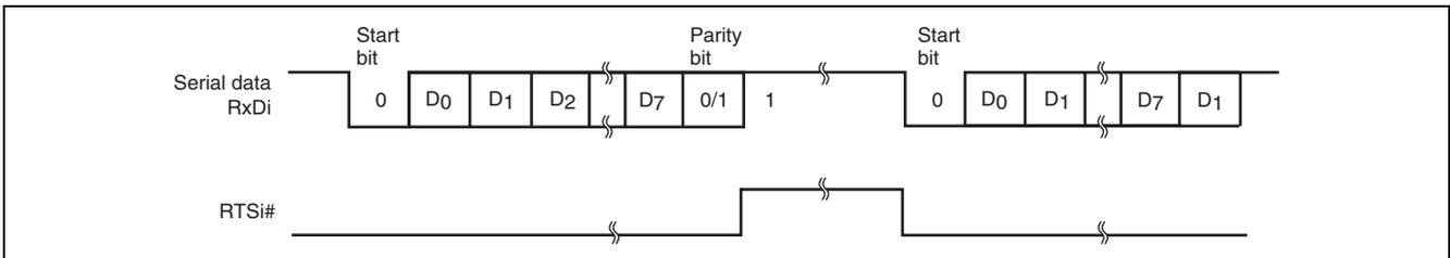
**Figure 23.10 Example of Operation Using Modem Control (RTSi#)**
