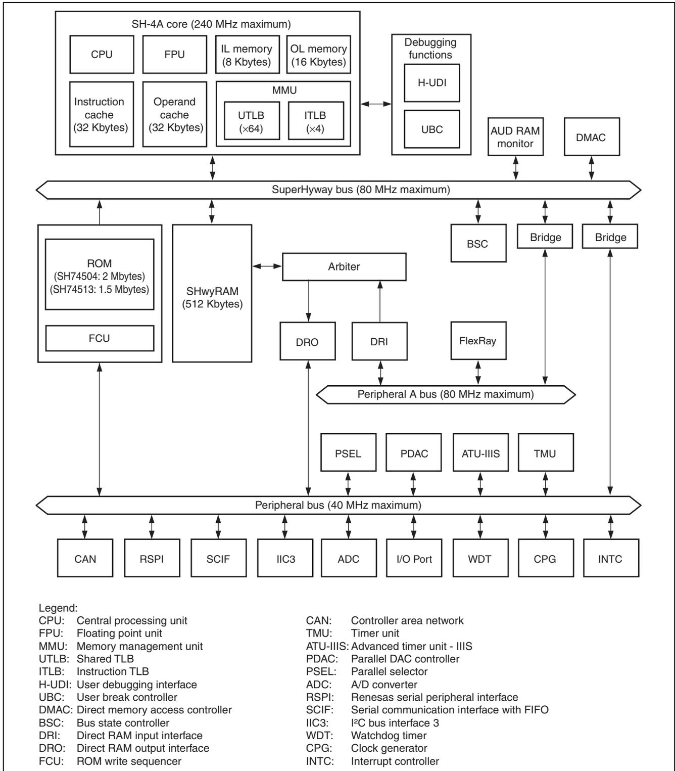
Figure 1.1 Block Diagram
