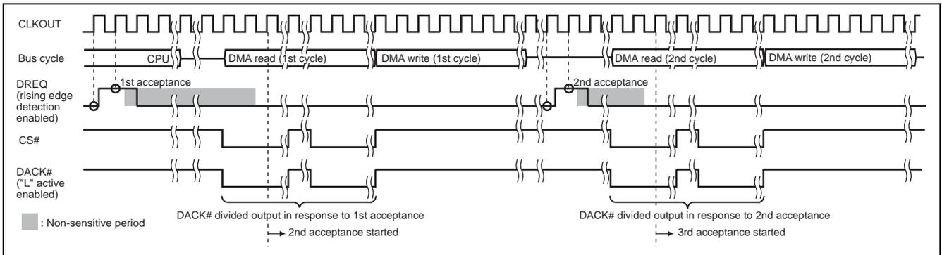
**Figure 20.17 Timing Example during DACK# Signal Output Division
