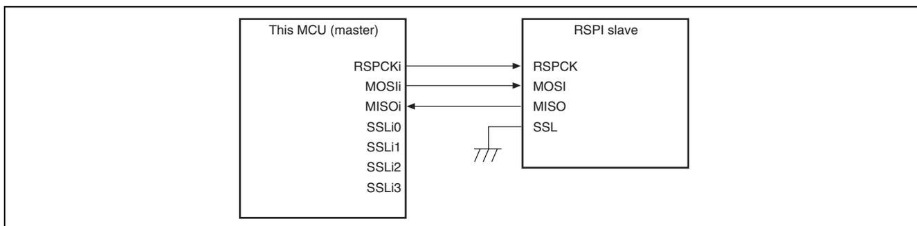
**Figure 24.3 Single-Master/Single-Slave Configuration Example (This MCU = Master)**
