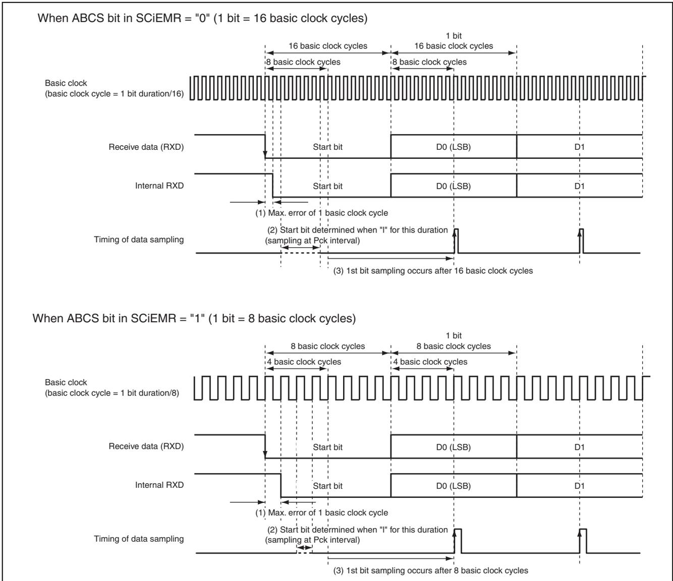
**Figure 23.19 Receive Data Sampling Timing in Asynchronous Mode**
