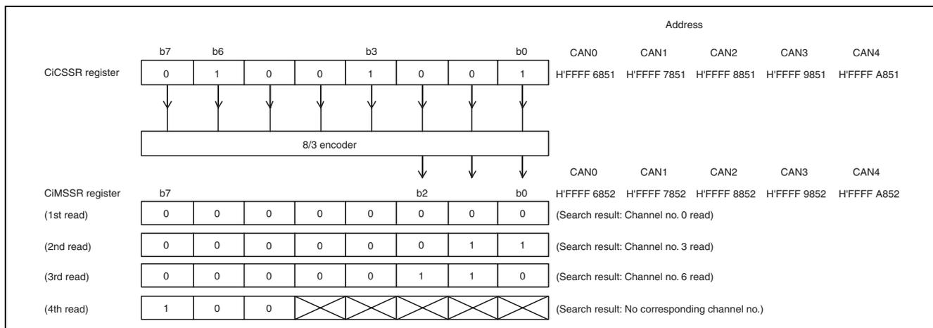
**Figure 26.4 Write and Read of Registers CiCSSR and CiMSSR (i = 0 to 4)**
