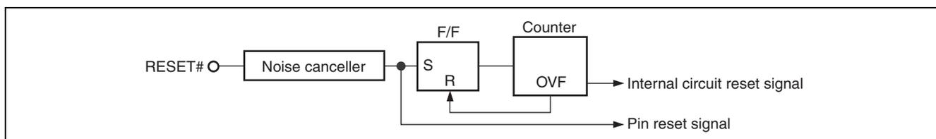
Figure 16.1 Reset Circuit
