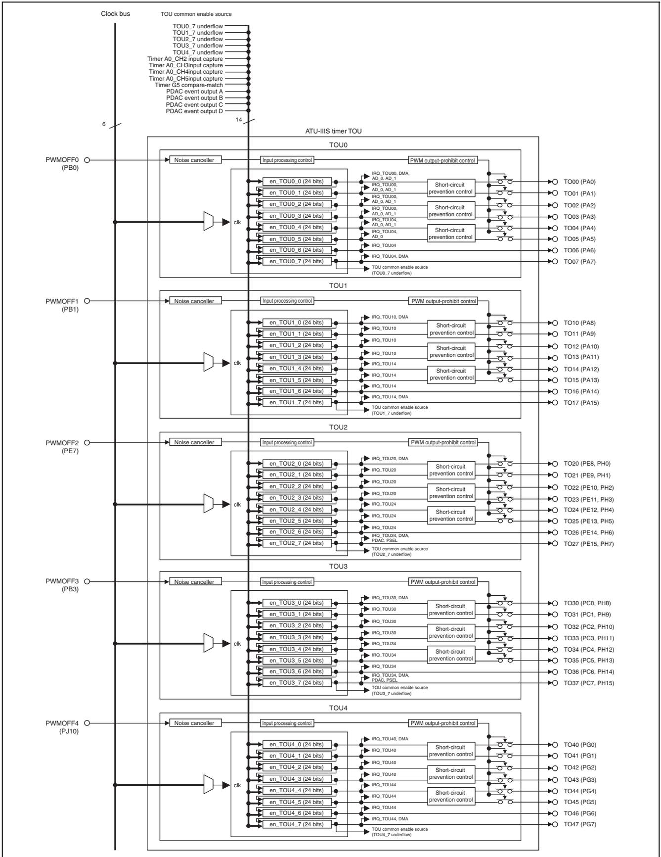
Figure 21.1 Block Diagram of ATU-IIIS (2)
