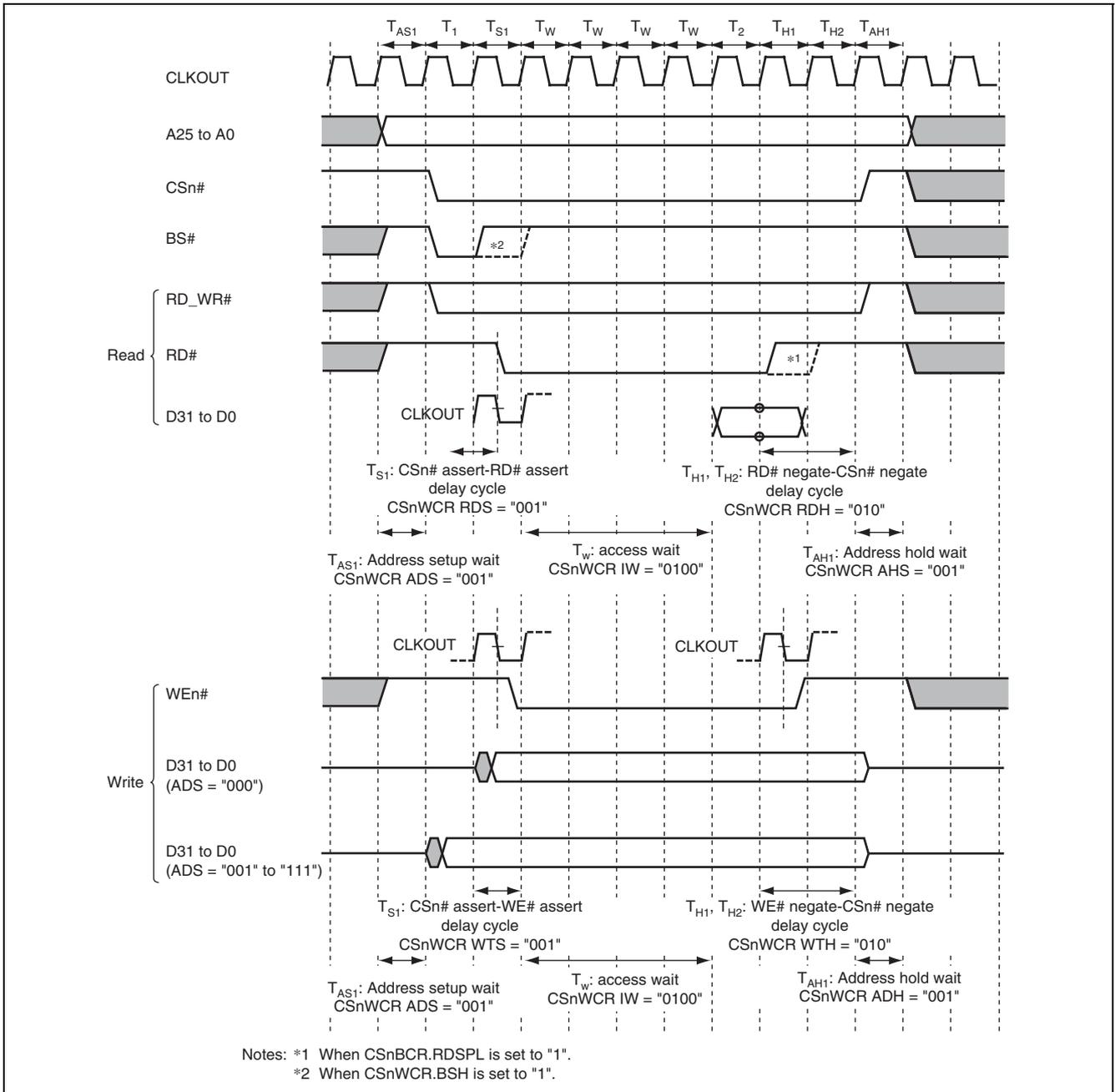
Figure 19.9 SRAM Interface Wait State Timing (Read-Strobe Negate Timing Setting)
