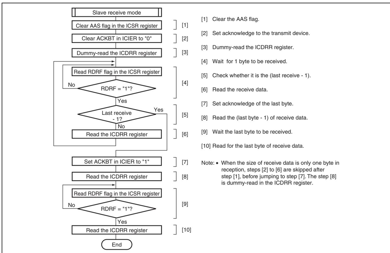
Figure 25.22 Sample Flowchart for Slave Receive Mode
