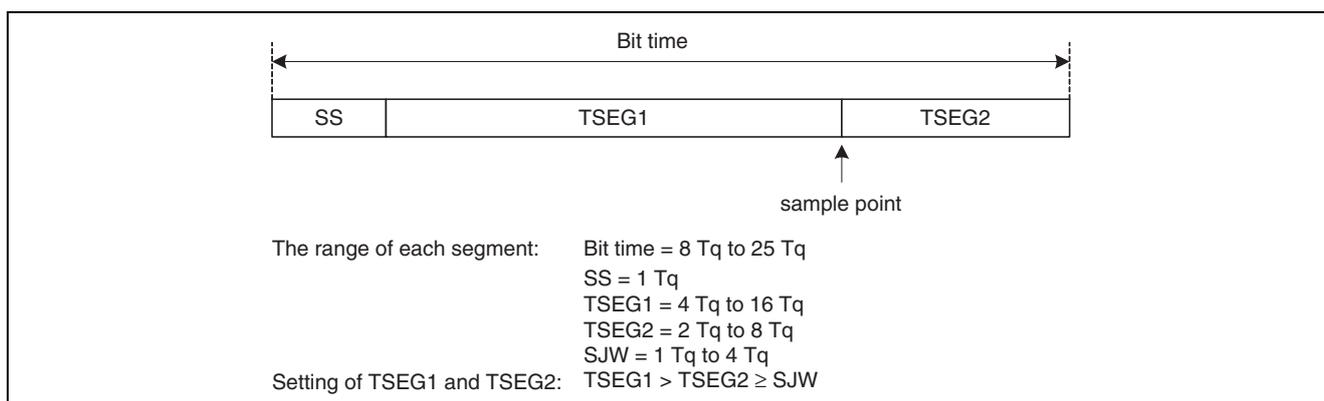
**Figure 26.12** Bit Timing
