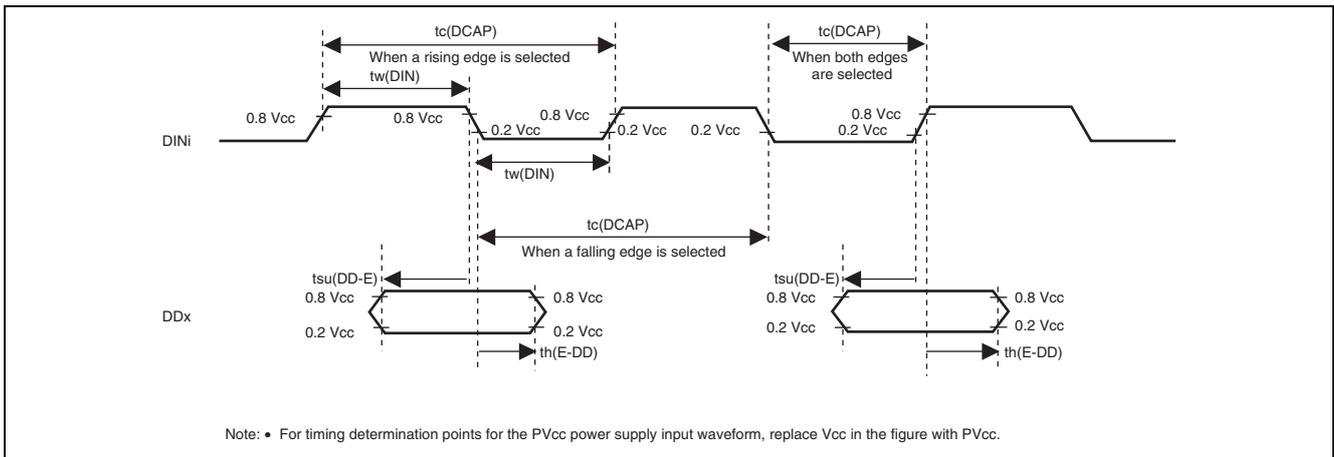
**Figure 38.33 Data Acquisition Related Timing**
