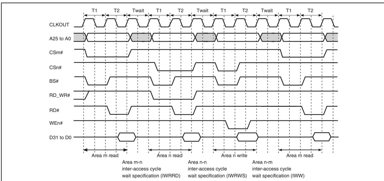
Figure 19.15 Inter-Access Cycle Wait Insertion
