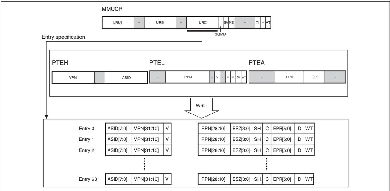
Figure 7.17 Operation of LDTLB Instruction (TLB Extended Mode)
