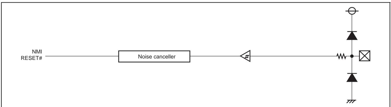
**Figure 18.6 Port Peripheral Circuit Diagram (Input Port 2)**
