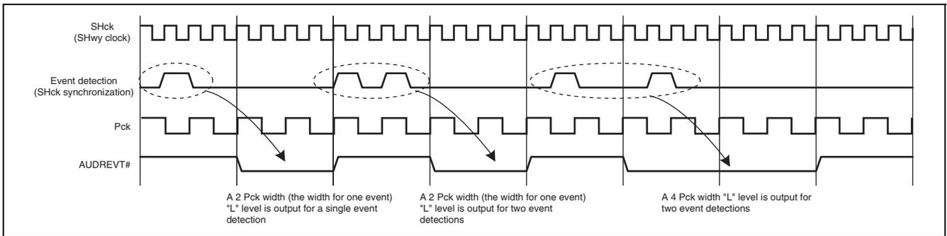
Figure 36.8 AUDR Event Detection and AUDREVT# Pin Operation
