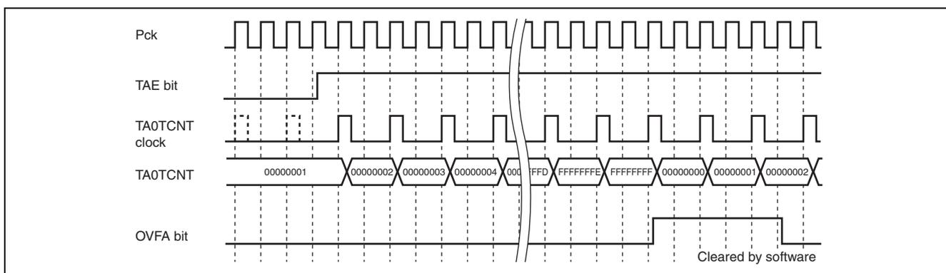
**Figure 21.11 Timer A Free-Running Operation: Overflow Timing**
