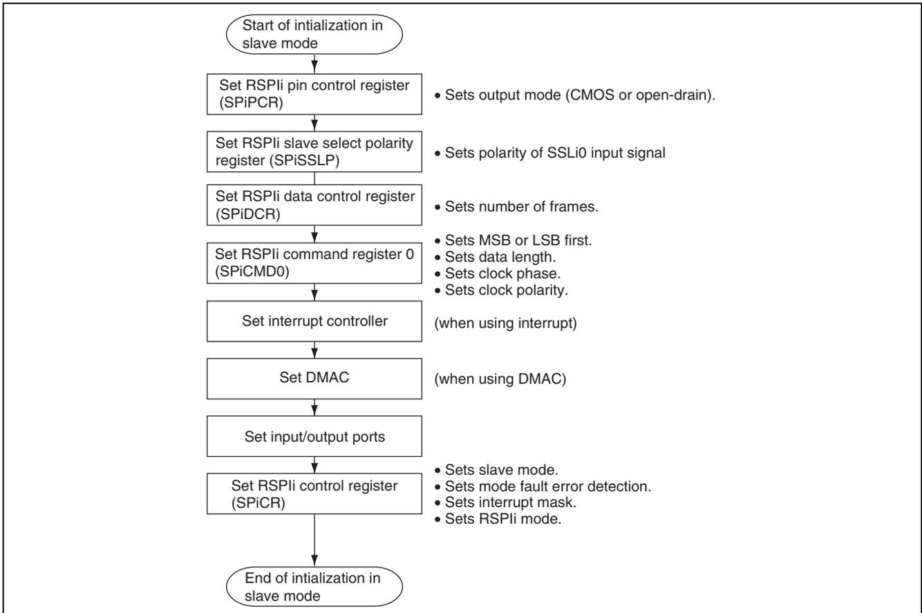
**Figure 24.23 Example of Initialization Flowchart in Slave Mode**
