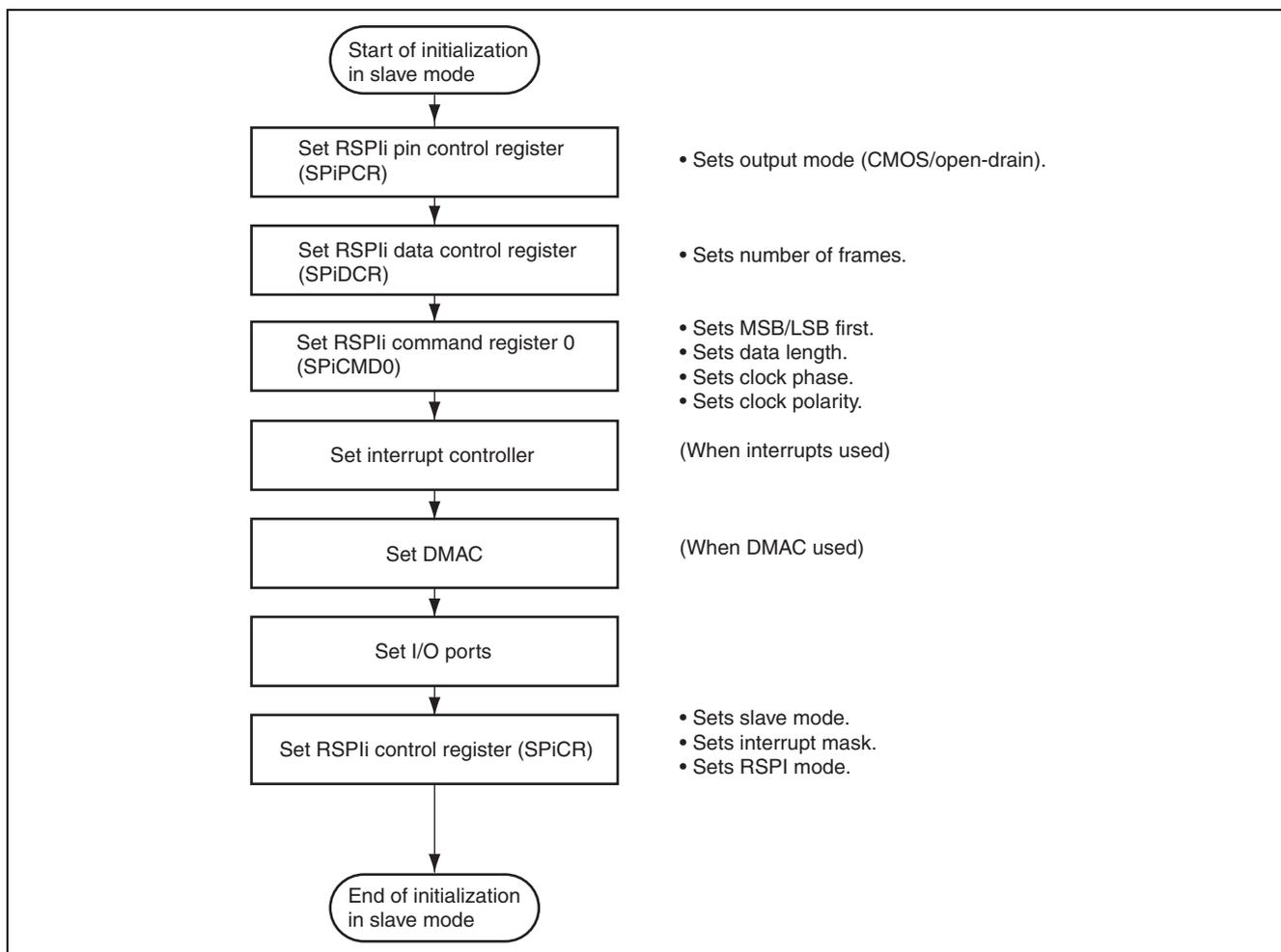
**Figure 24.29 Flowchart of Initialization in Slave Mode**
