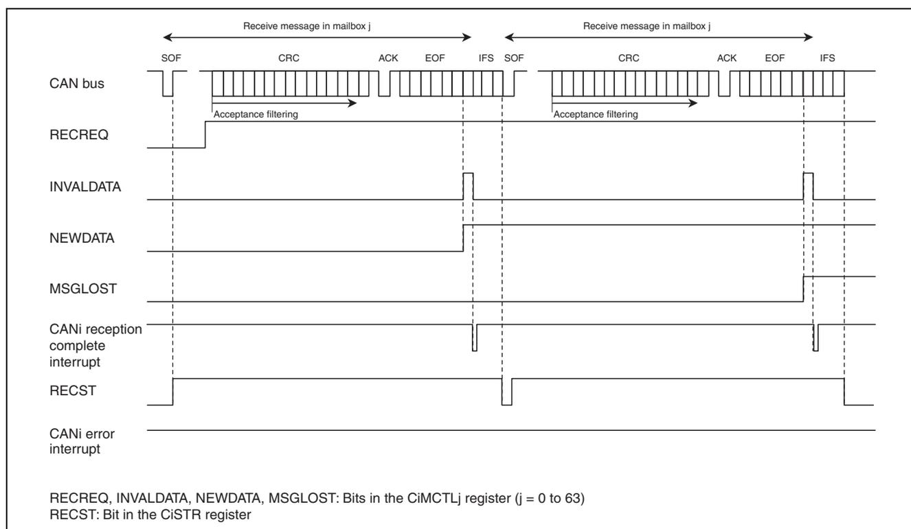
**Figure 26.18 Operation Example of Data Frame Reception in Overwrite Mode (i = 0 to 4)**
