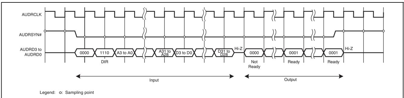
**Figure 36.6 Write Operation Example (long word write)**
