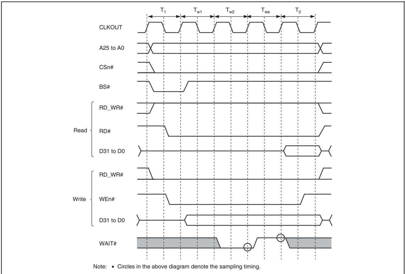
Figure 19.8 External Space Access Wait Timing (WAIT# Signal Wait Insertion)
