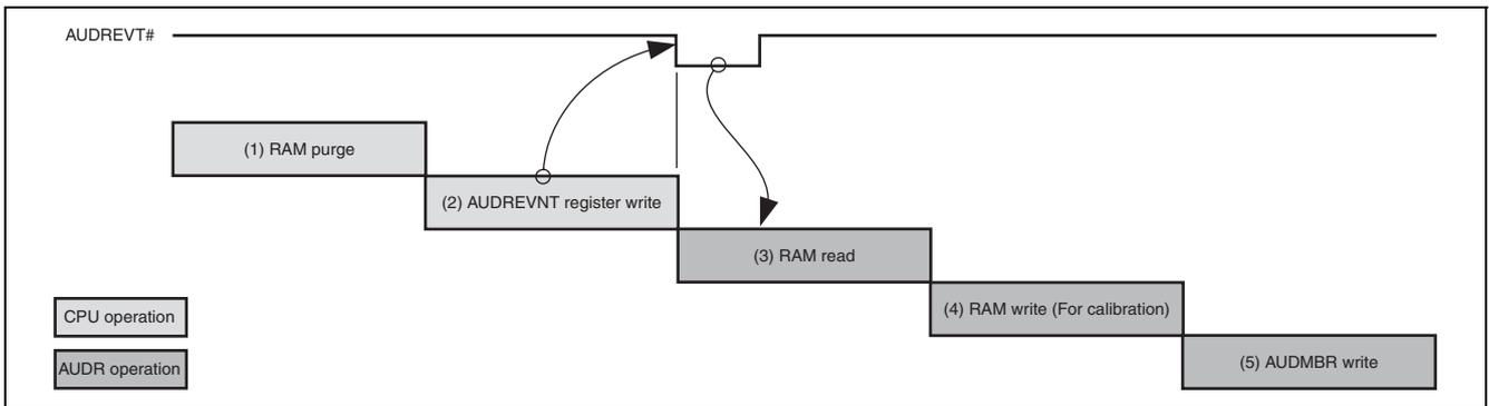
Figure 36.2 AUDR Module Usage Example (RAM monitor/calibration procedure)
