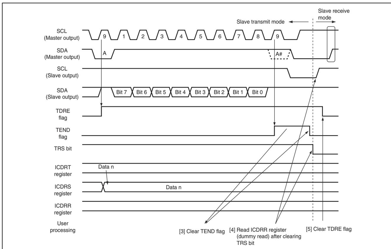
**Figure 25.10 Slave Transmit Mode Operation Timing (2)**
