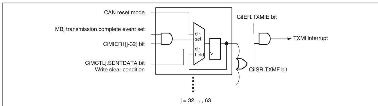
**Figure 26.23 Block Diagram of CAN<sub>i</sub> Transmission Complete Interrupt (Mailbox 32 to 63) [TXMi]**
