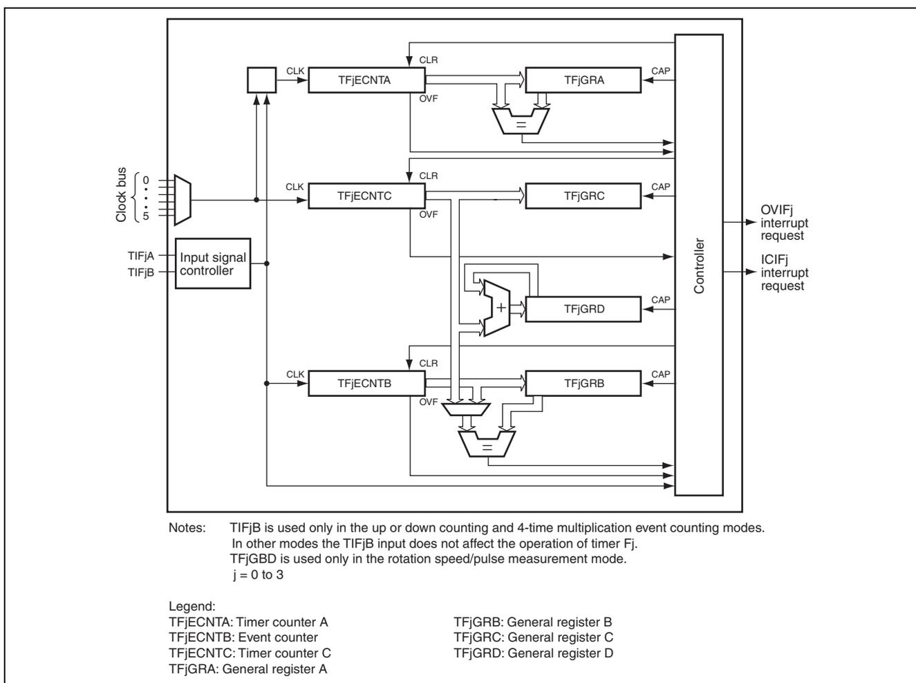
**Figure 21.13 Block Diagram of Subblocks of Timer F**
