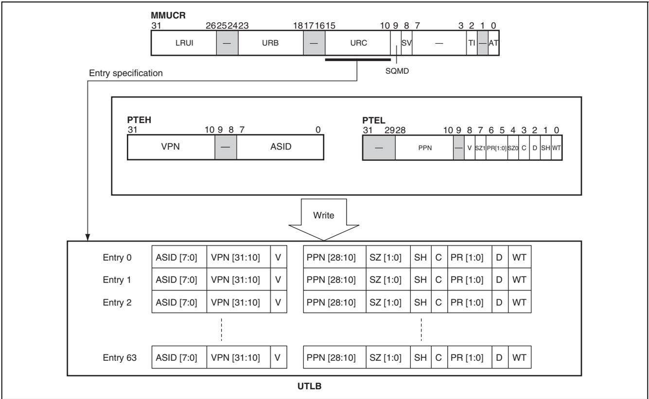
Figure 7.16 Operation of LDTLB Instruction (TLB Compatible Mode)
