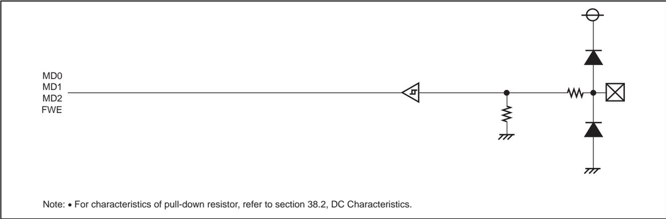
Figure 18.8 Port Peripheral Circuit Diagram (Input Port 4)
