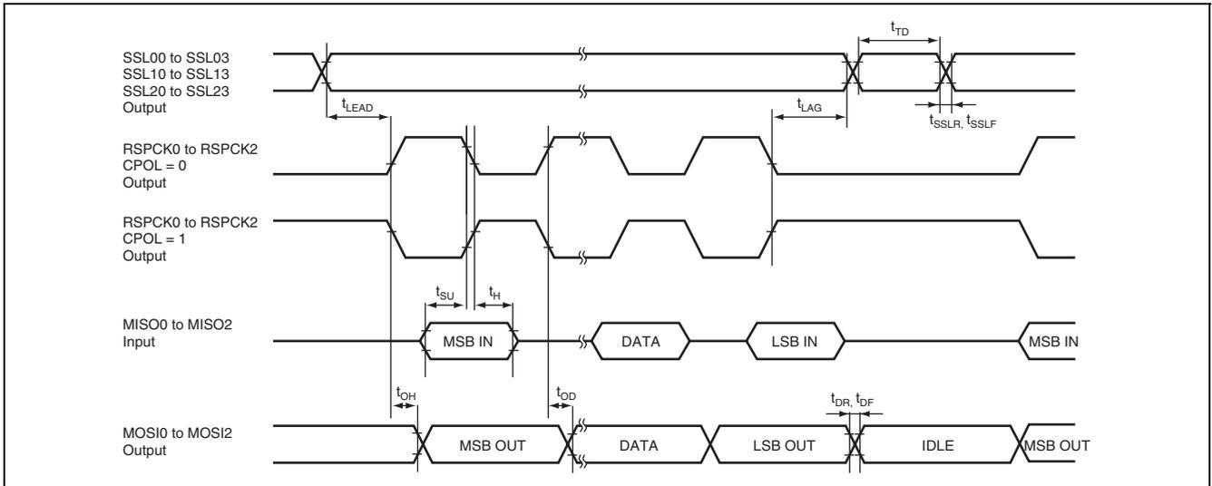
Figure 38.29 RSPI Timing (Master, CPHA = "1")
