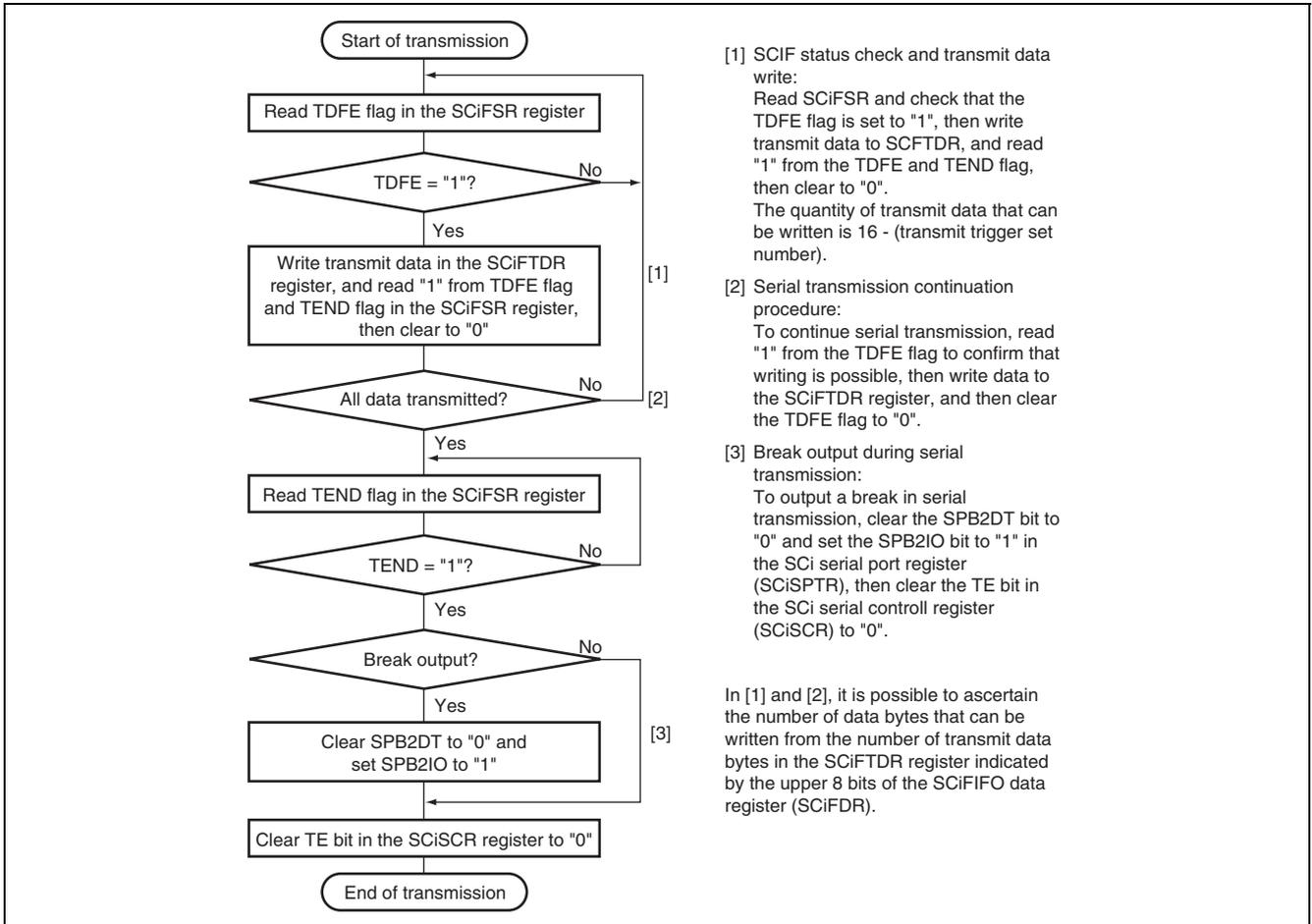
Figure 23.4 Sample Flowchart for Transmitting Serial Data
