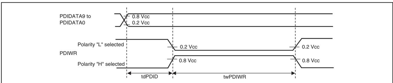
**Figure 38.39 PDAC Output Timing**
