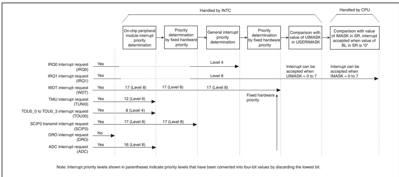
**Figure 15.2 Priority Determination at Interrupt Request Acceptance**
