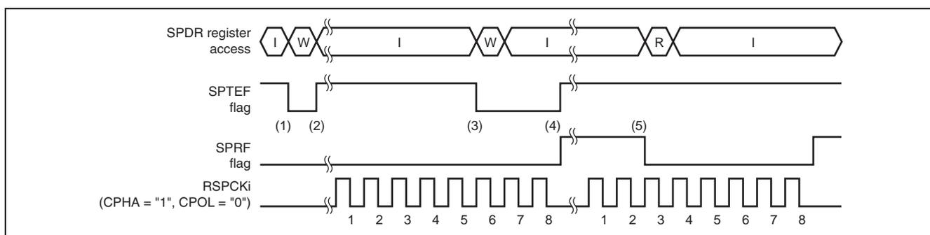
**Figure 24.17 SPTEF and SPRF Bit Operation Example**
