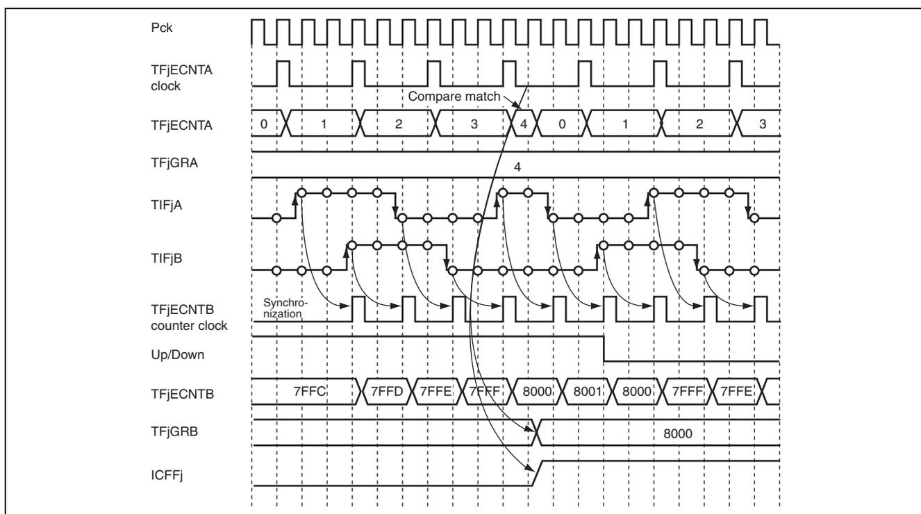
**Figure 21.22 Operation Example of Four-time Multiplication Event Count**
