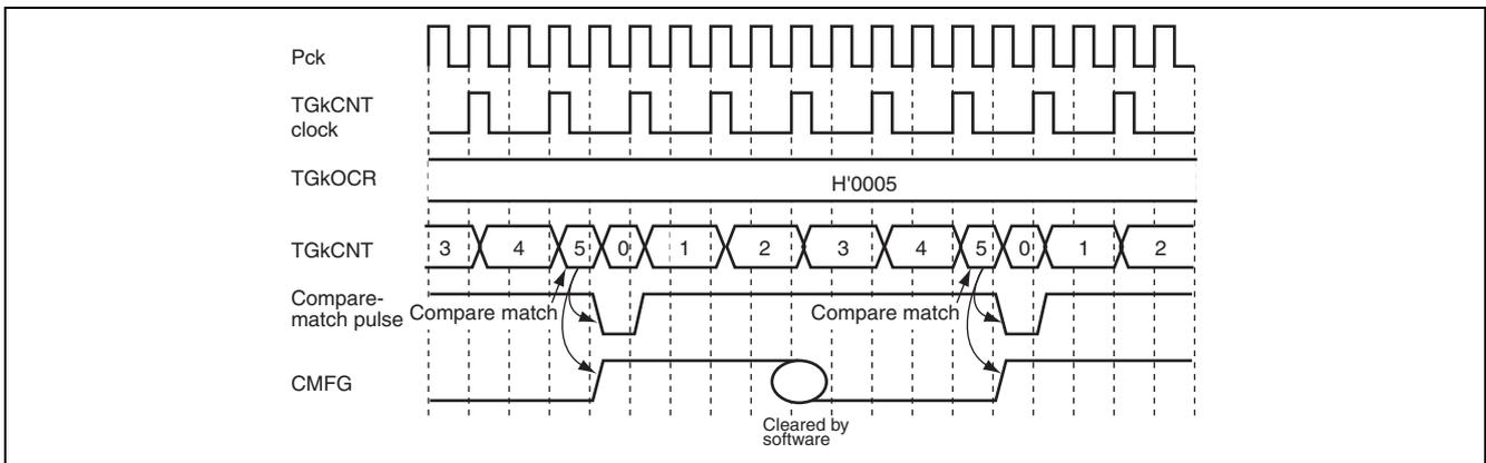
**Figure 21.24 Operation Example of Counter and Compare Match**
