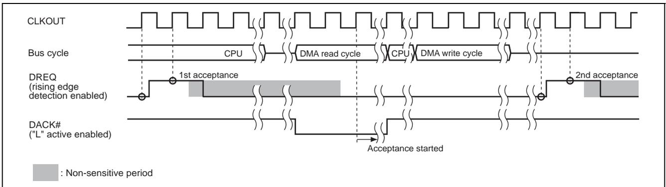
**Figure 20.12 Example of DREQ Input Detection (Cycle Steal Mode 2, DACK Read Cycle Output)**
