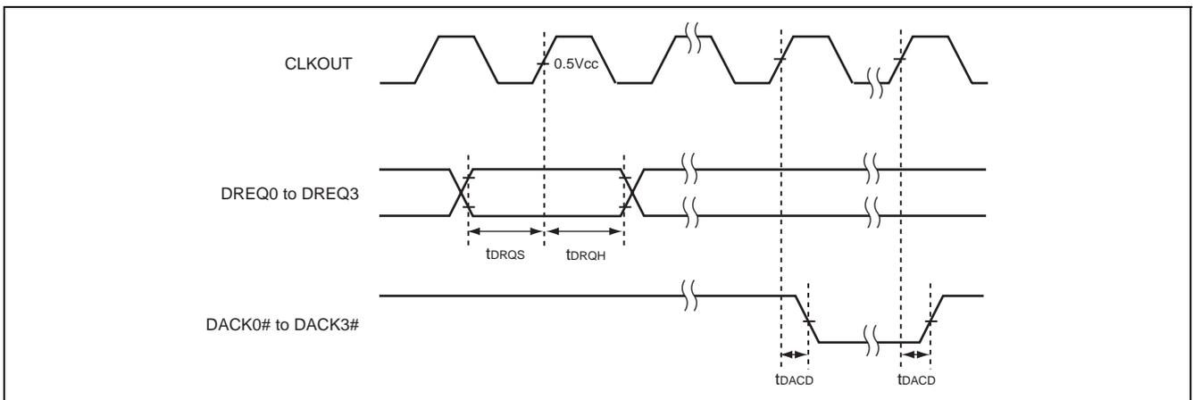
**Figure 38.20 DMAC Timing**
