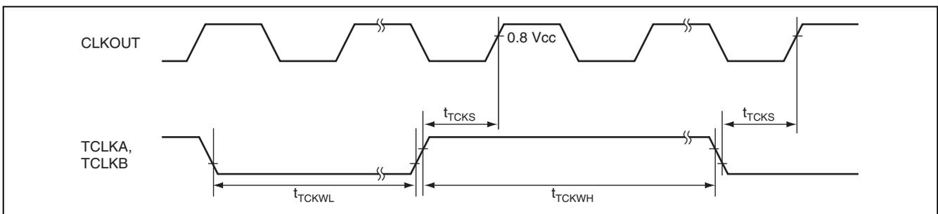
**Figure 38.22 ATU-IIIS Clock Input Timing**
