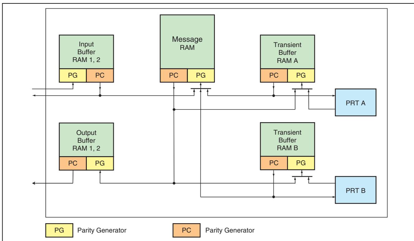
**Figure 32.20 Parity Generation and Check**
