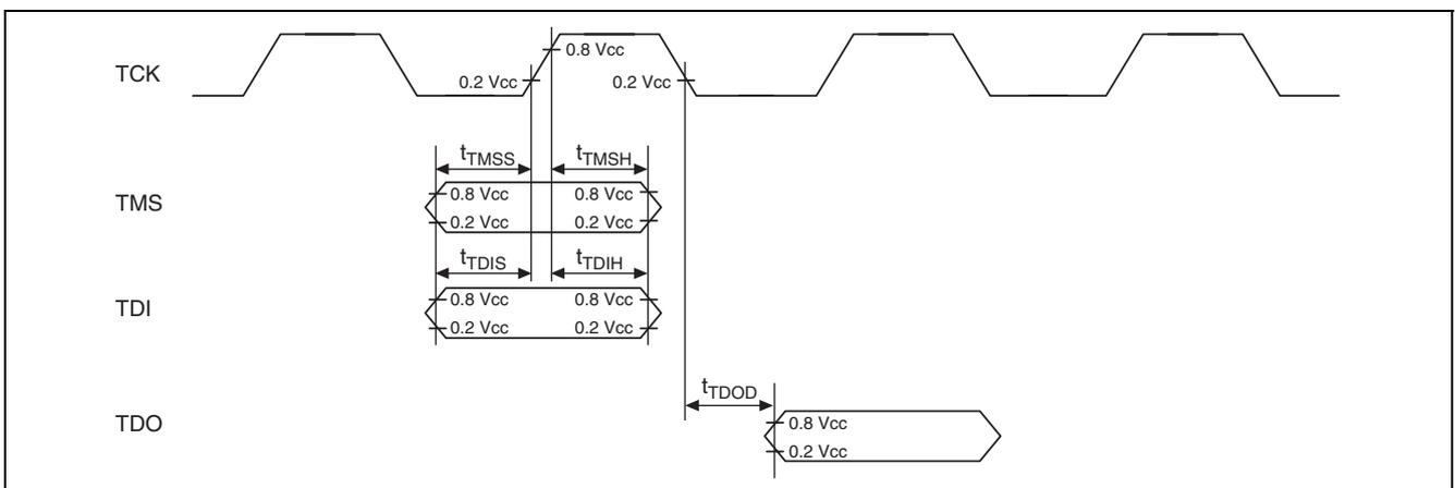
**Figure 38.45 H-UDI Data Transfer Timing**
