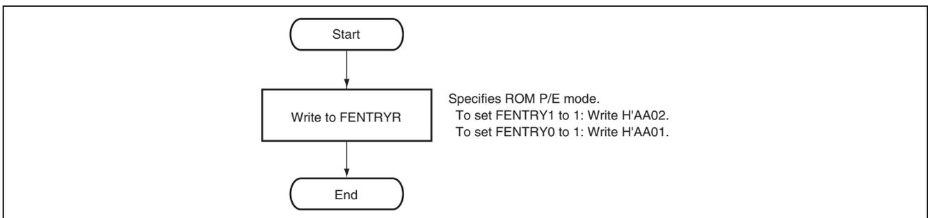
**Figure 12.9 Procedure for Transition to ROM P/E Mode**
