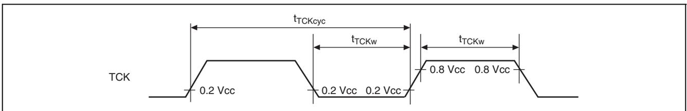
**Figure 38.43 TCK Input Timing**
