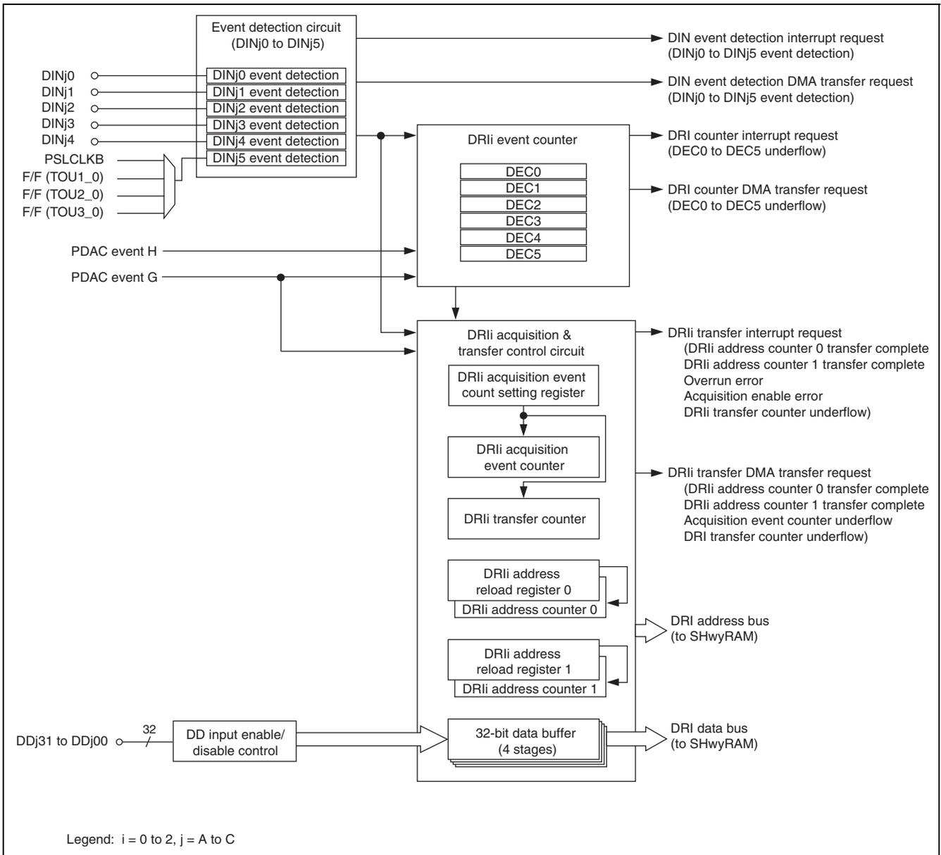
Figure 28.1 Block Diagram of DRli
