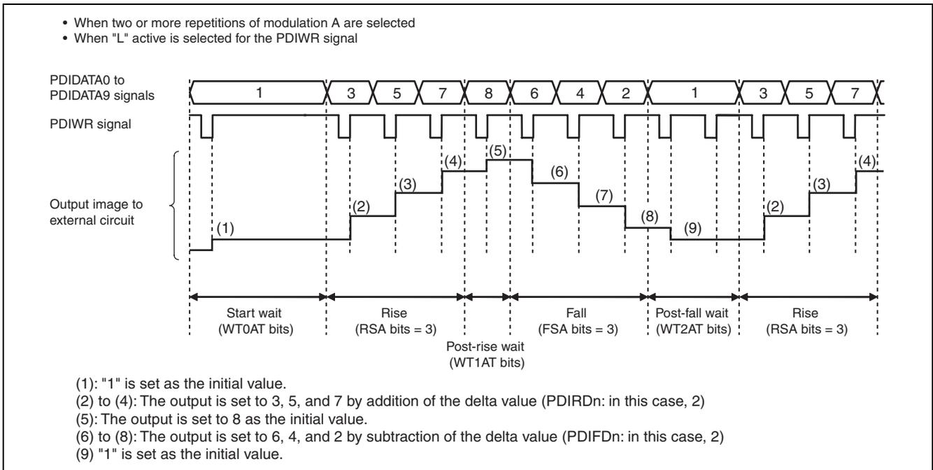
**Figure 30.17 Initial Value and Delta Value Timing for Each Modulation (When wait times are used)**
