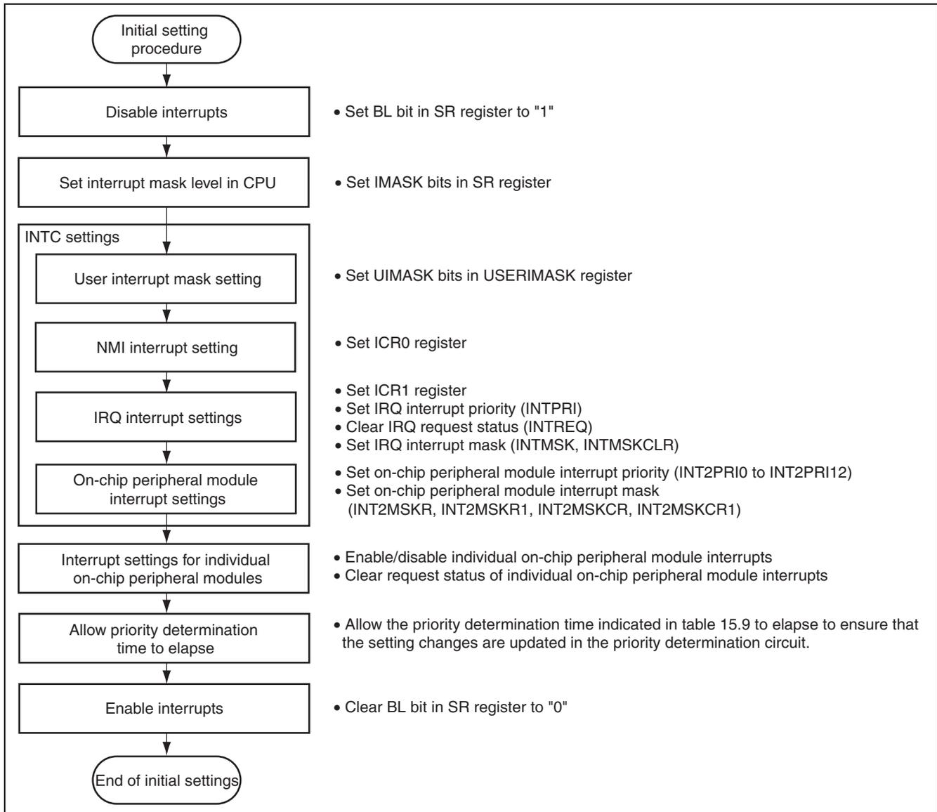
**Figure 15.8 INTC Initial Setting Procedure Example**
