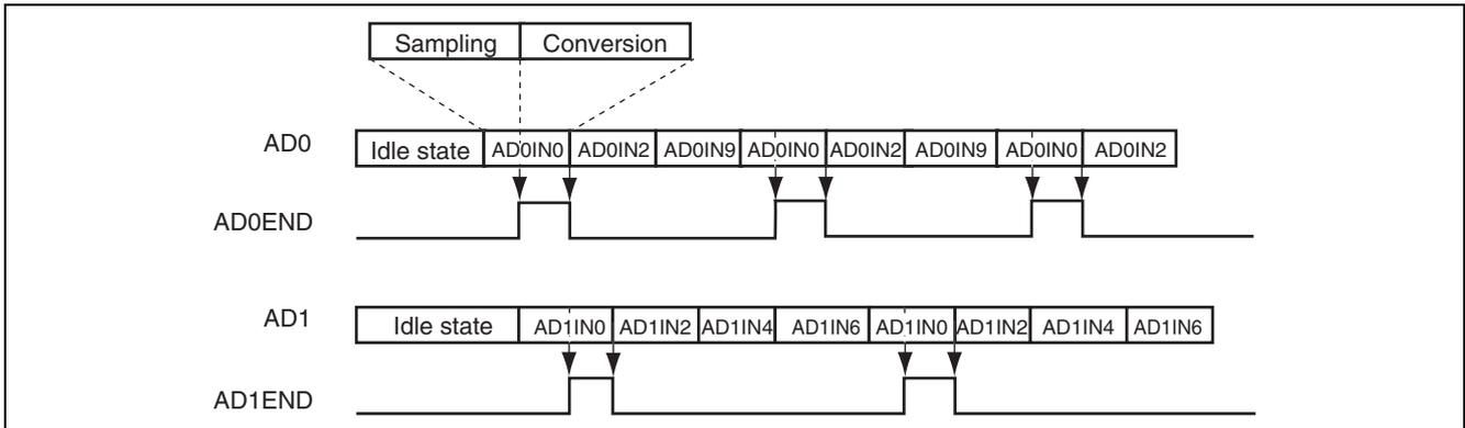
**Figure 27.10 Example of AD0END and AD1END Outputs**
