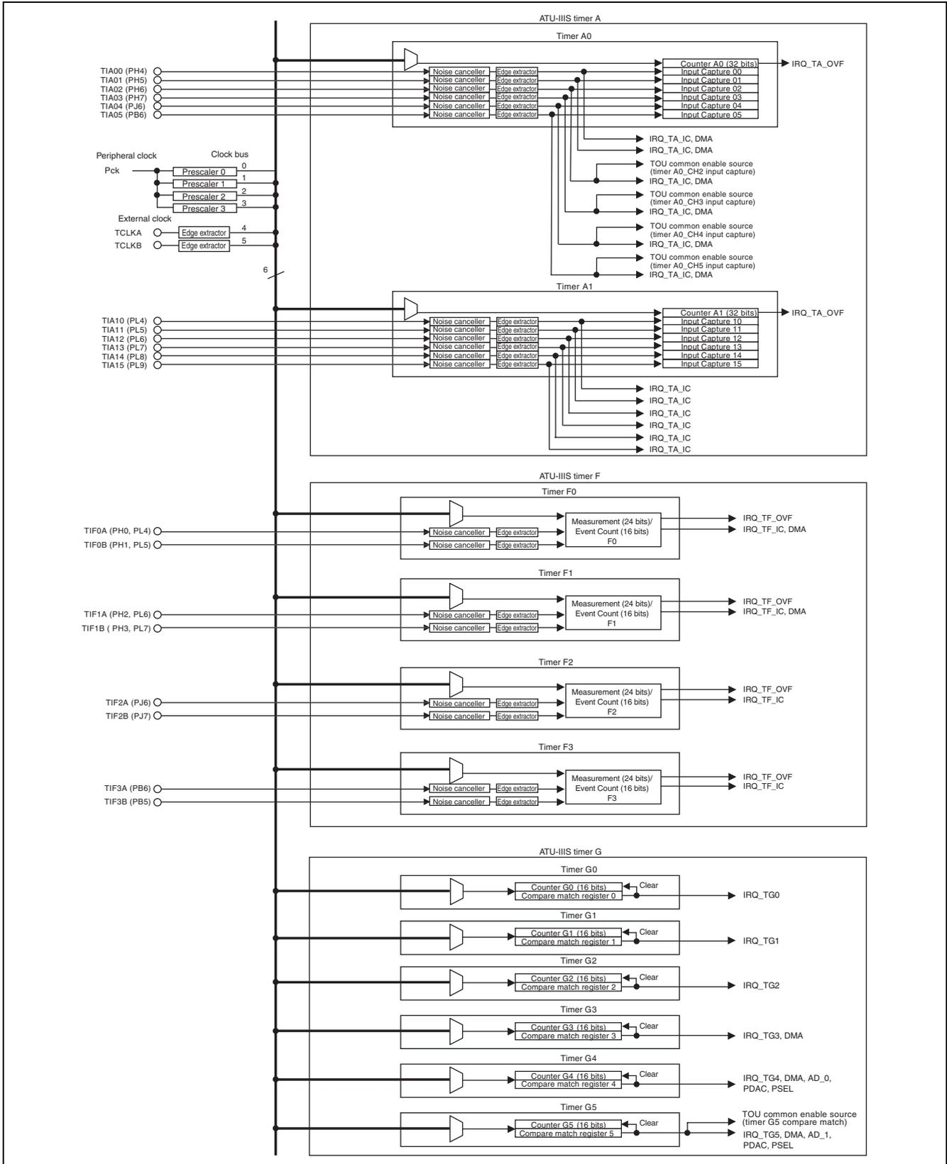
Figure 21.1 Block Diagram of ATU-IIIS (1)
