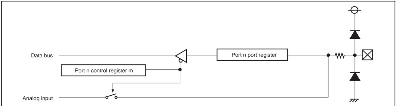
**Figure 18.5 Port Peripheral Circuit Diagram (Input Port 1)**
