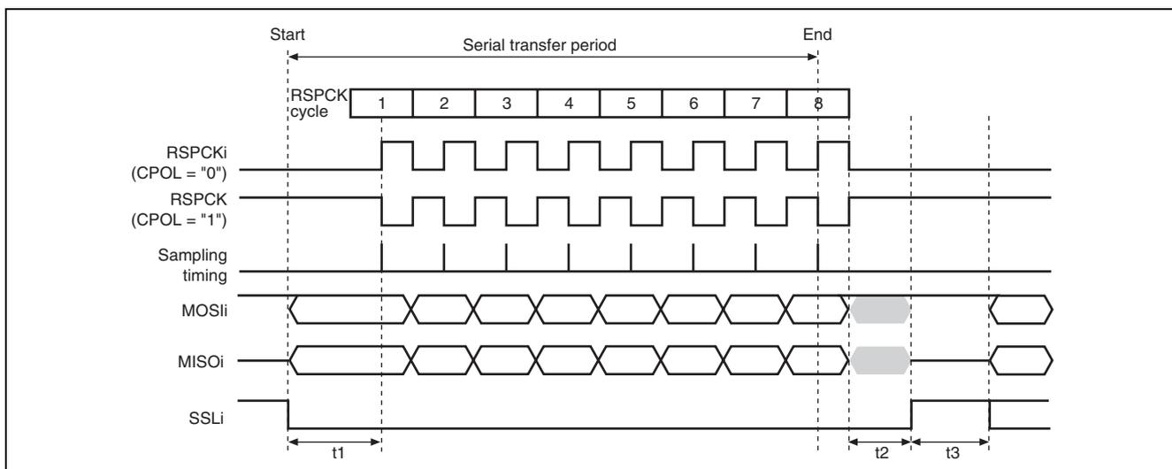
Figure 24.11 RSPI Transfer Format (CPHA = "0")
