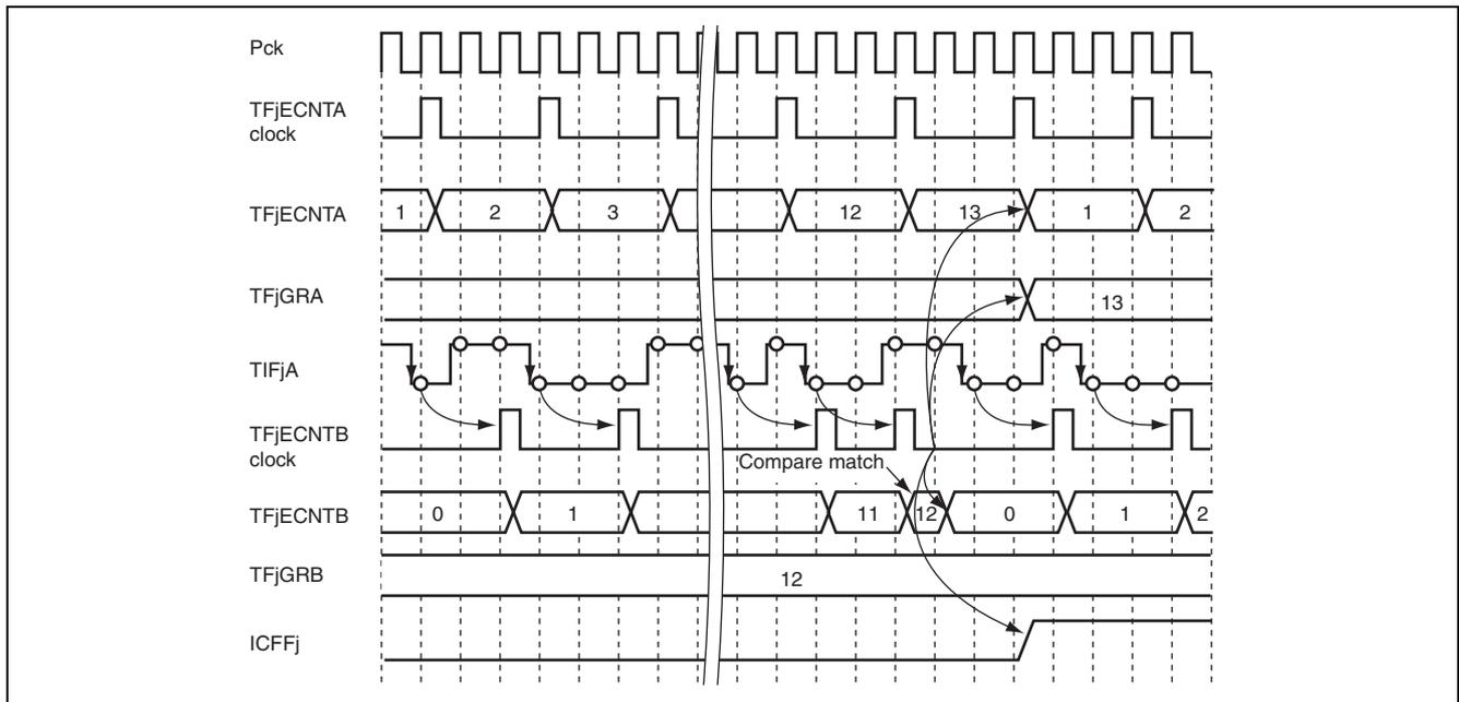
Figure 21.16 Operation Example of Valid Edge Interval Counting
