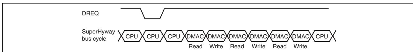
**Figure 20.4 DMA Transfer Timing Example in Burst Mode
