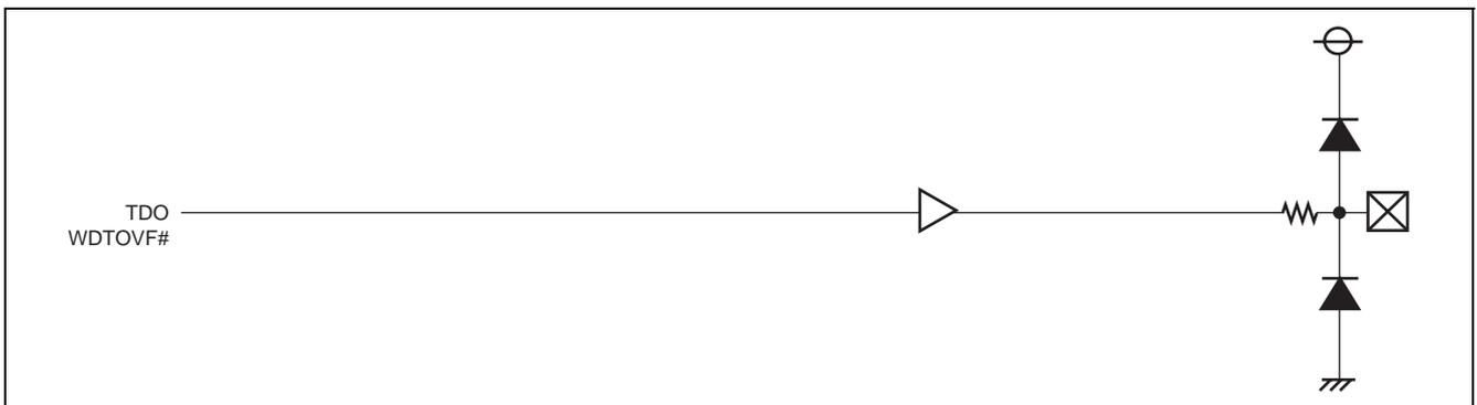
Figure 18.12 Port Peripheral Circuit Diagram (Output Port 1)
