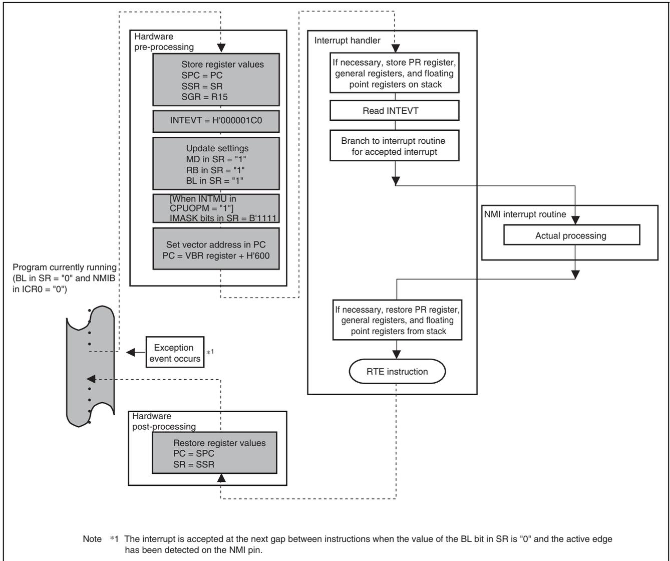
**Figure 15.6 NMI Interrupt Operation Example (When Value of NMIB Bit in ICR0 is "0")**
