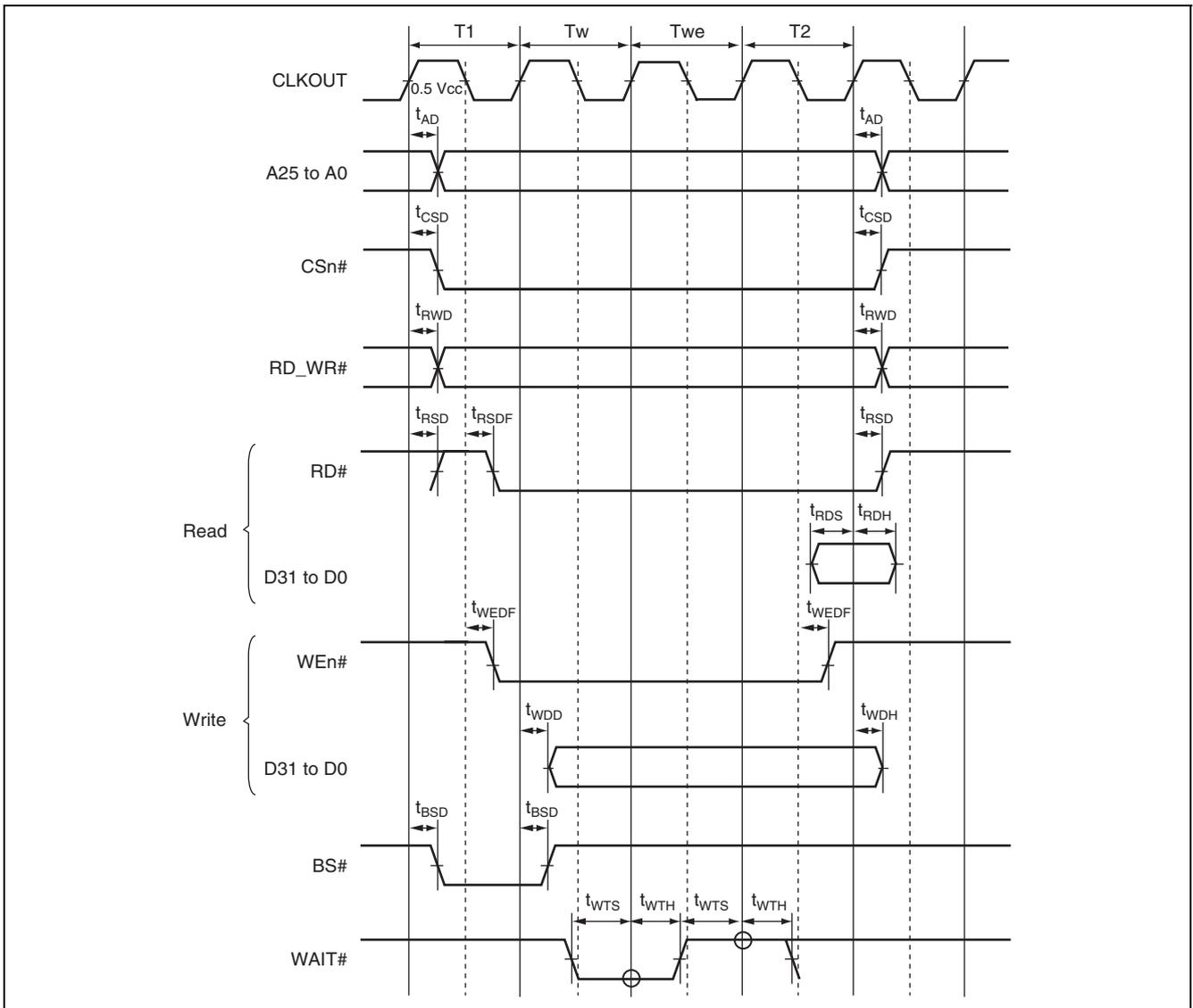
Figure 38.14 SRAM Bus Cycle (One Software Wait Cycle, One External Wait Cycle)
