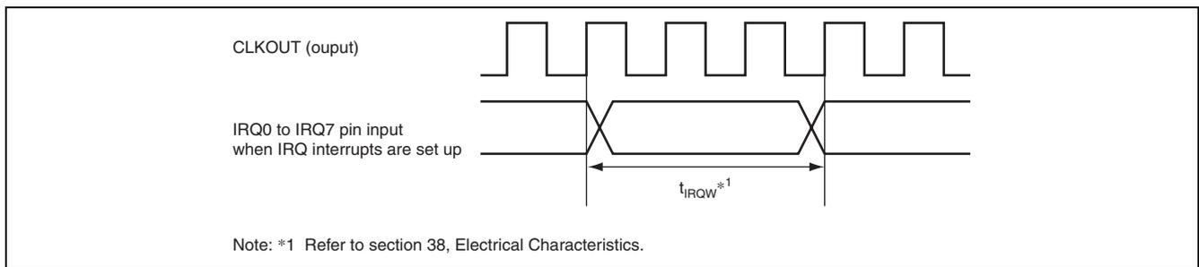
**Figure 15.10 Time Requested to Detect Interrupts from IRQ**
