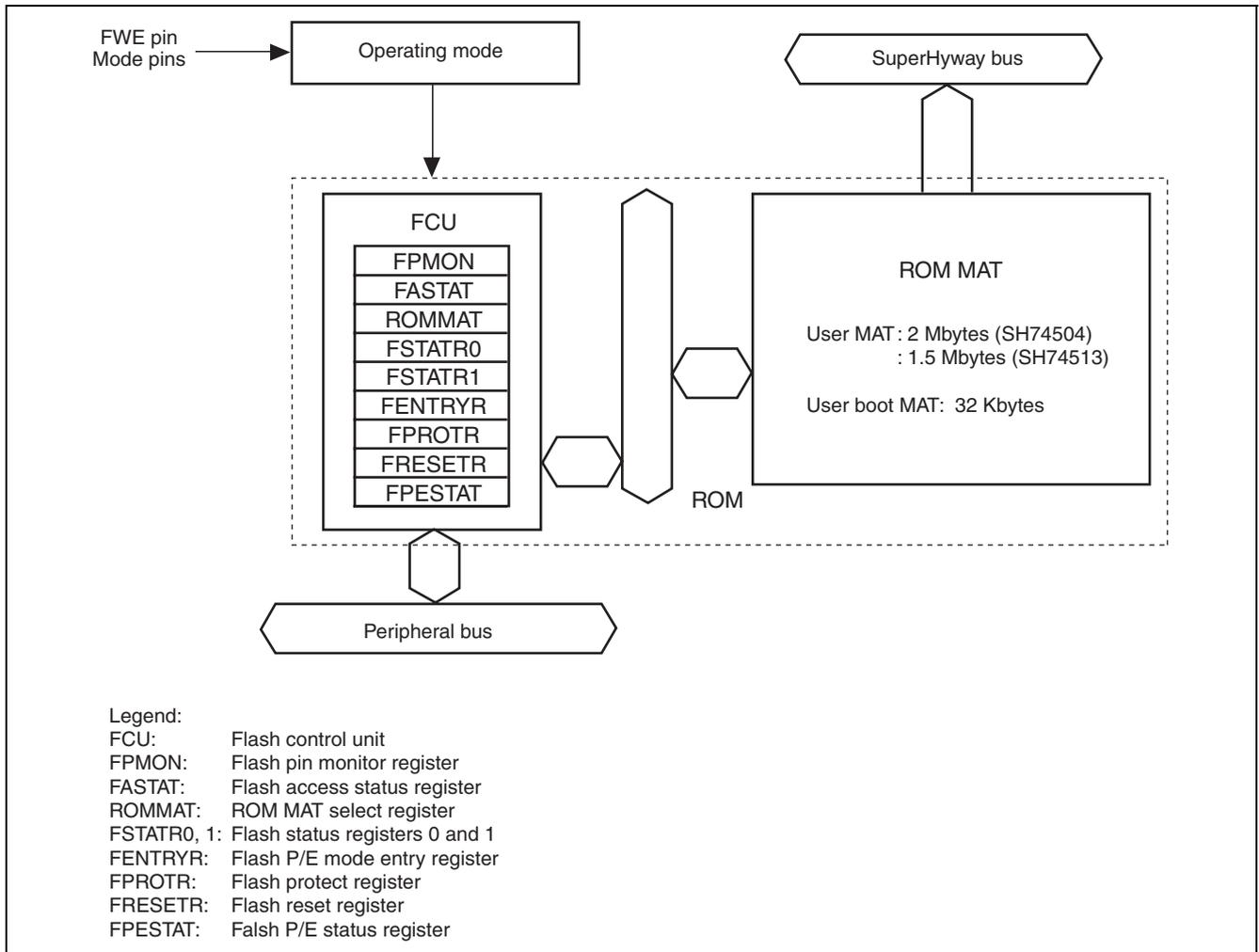
**Figure 12.2 Block Diagram of ROM**
