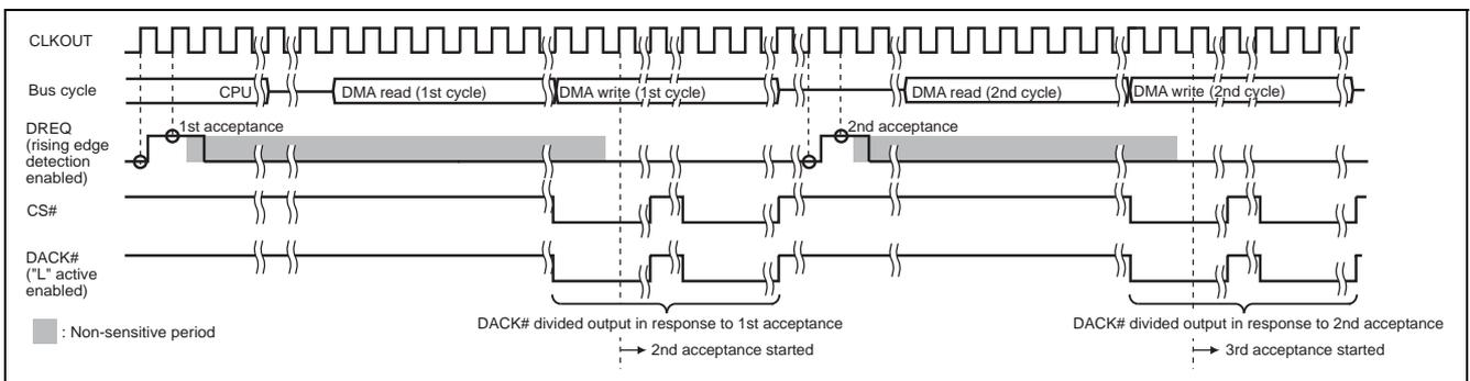
**Figure 20.18 Timing Example during DACK# Signal Output Division
