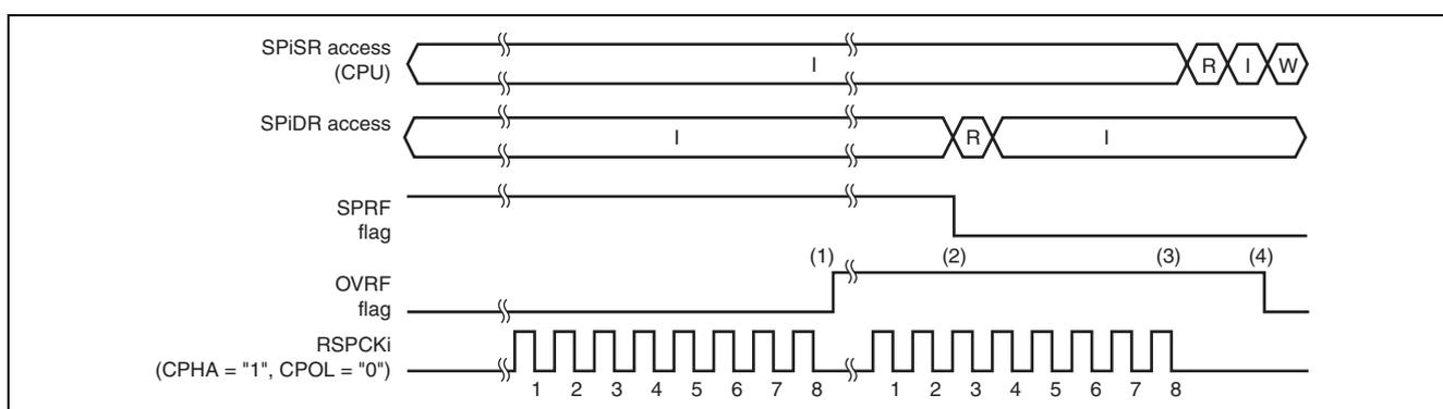
**Figure 24.18 SPRF and OVRF Bit Operation Example**
