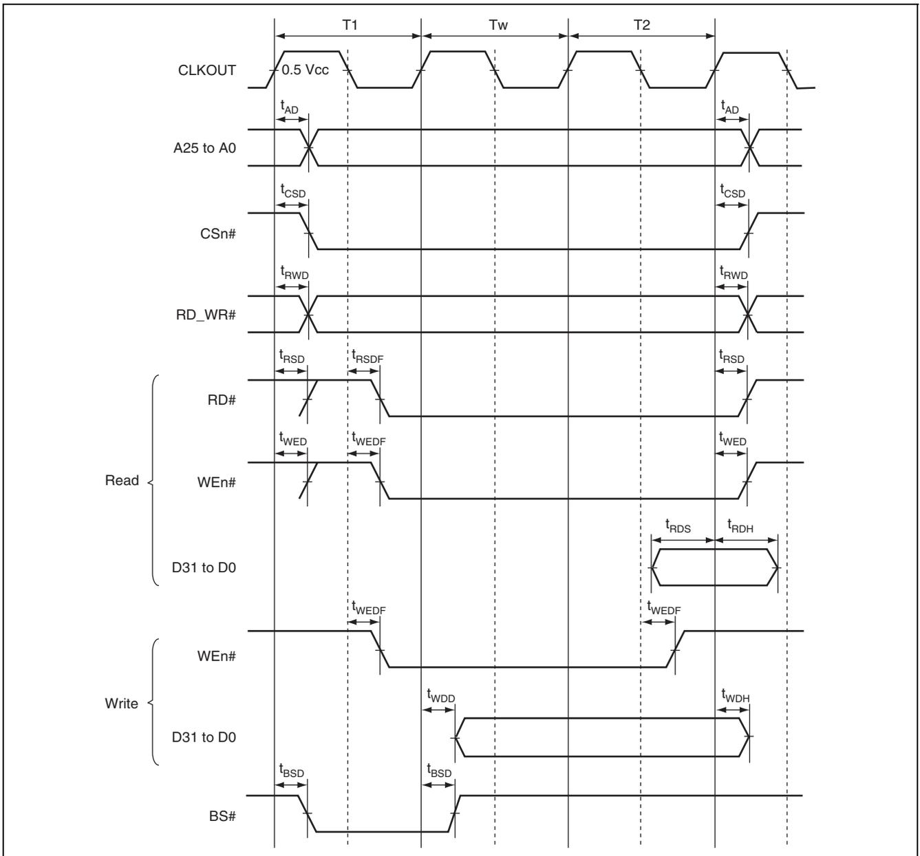
Figure 38.17 SRAM Bus Cycle with Byte Control (One Software Wait Cycle)
