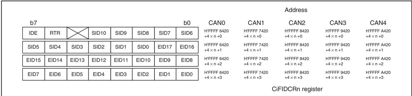
**Figure 26.15 Structure of CiFIDCRn register (i = 0 to 4; n = 0, 1)**
