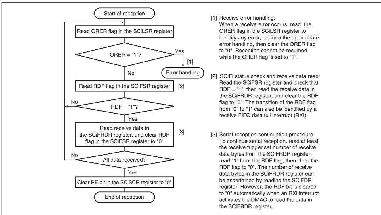
**Figure 23.15 Sample Flowchart for Receiving Serial Data (1)**
