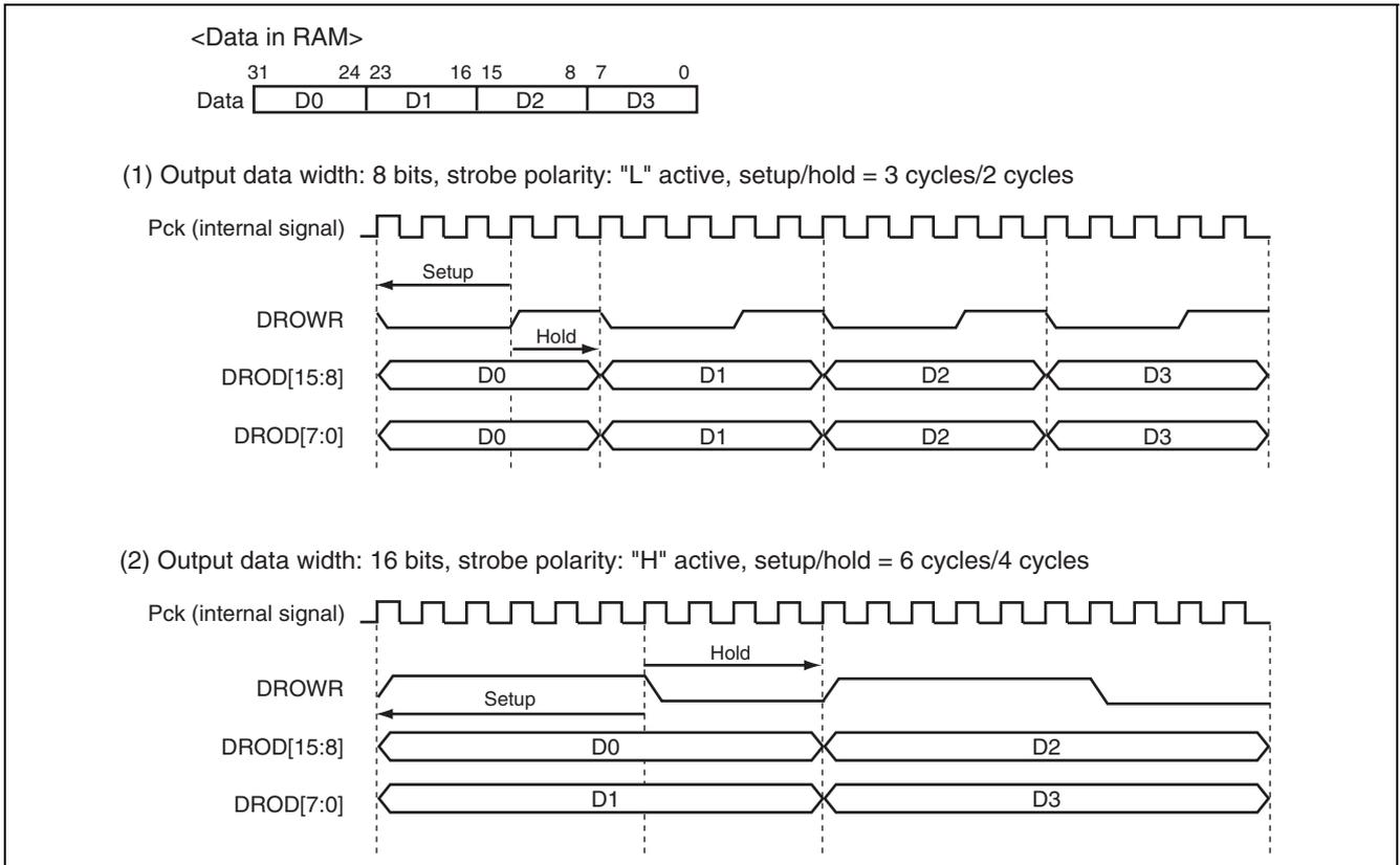
**Figure 29.4 Data Format Example for Periodic Output**
