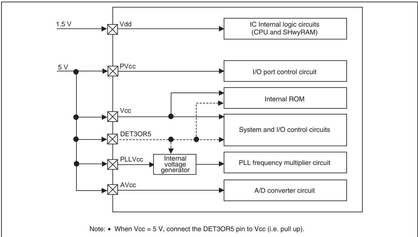
**Figure 34.1 Power Supply Circuit Structure (when  $PV_{cc} = V_{cc} = 5\text{ V}$ )**
