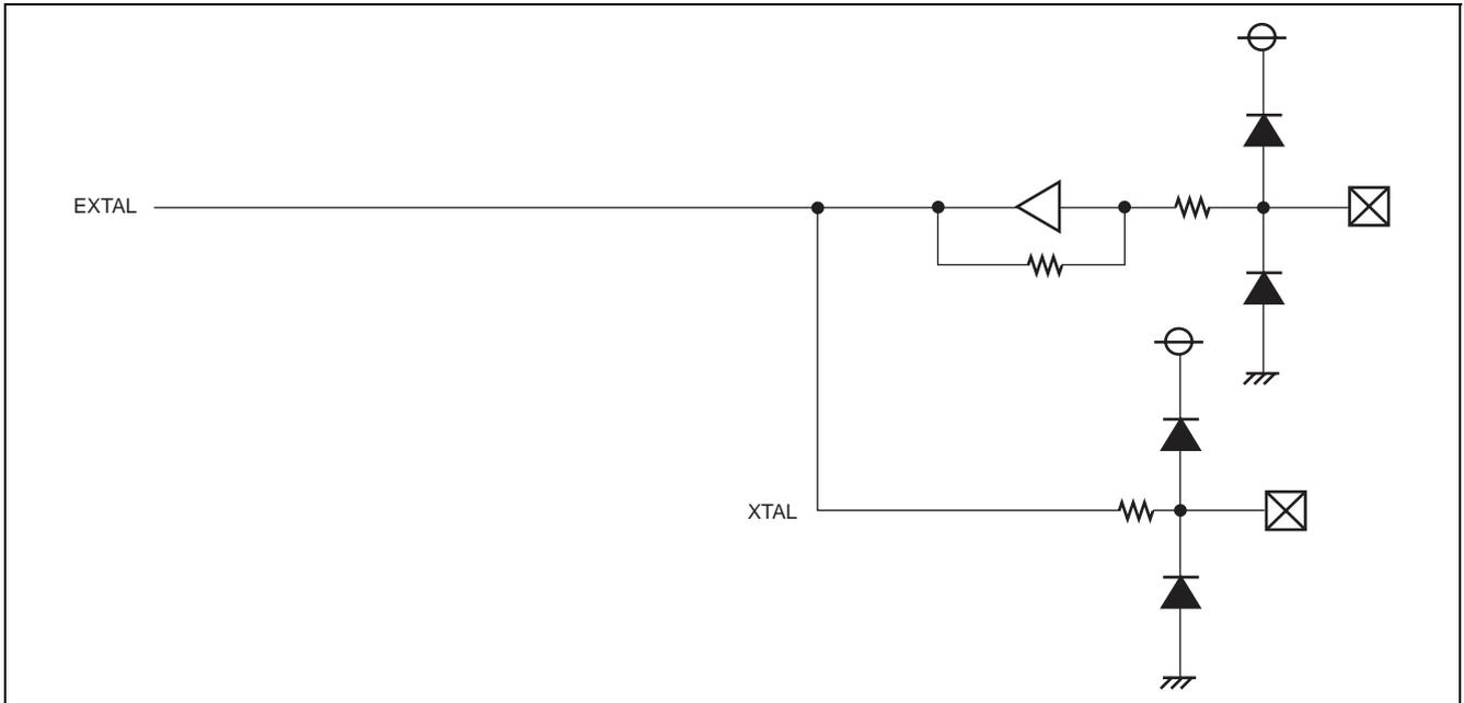
Figure 18.11 Port Peripheral Circuit Diagram (Input Port and Output Port)
