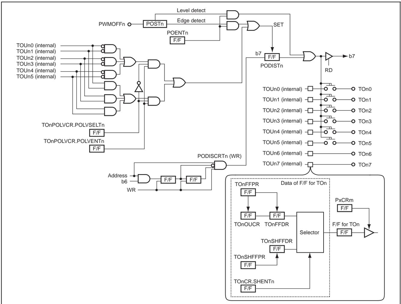
Figure 21.43 Circuit Configuration of PWM Output-Prohibit Function
