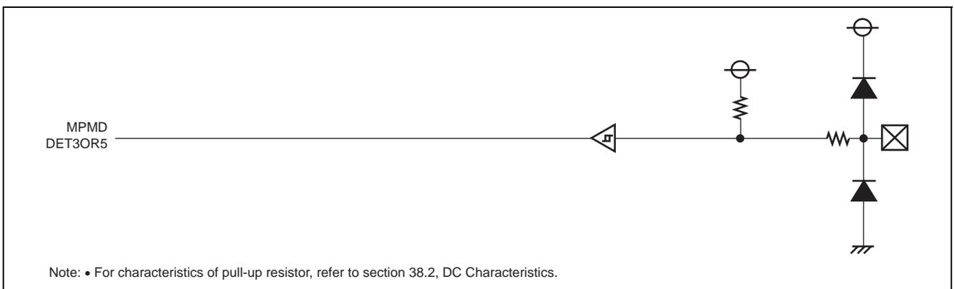
**Figure 18.7 Port Peripheral Circuit Diagram (Input Port 3)**
