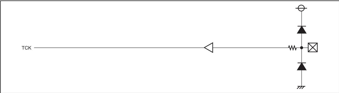
Figure 18.10 Port Peripheral Circuit Diagram (Input Port 6)
