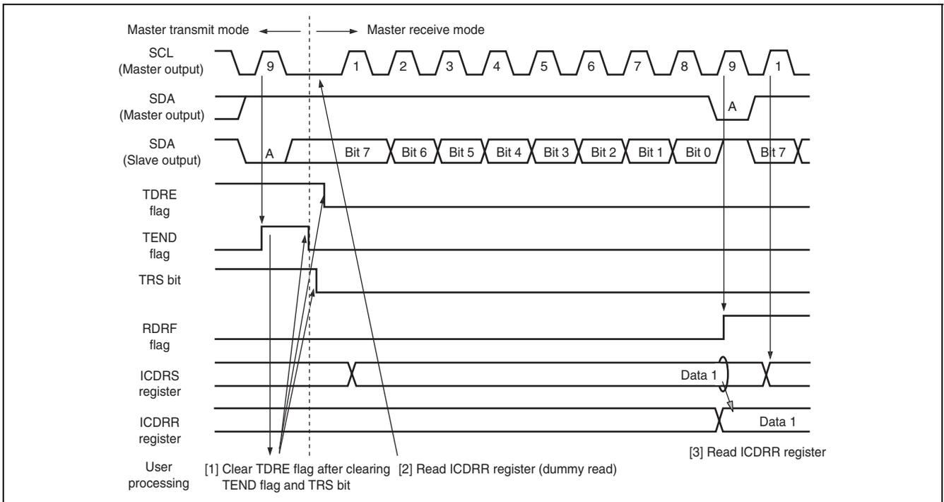
**Figure 25.7 Master Receive Mode Operation Timing (1)**
