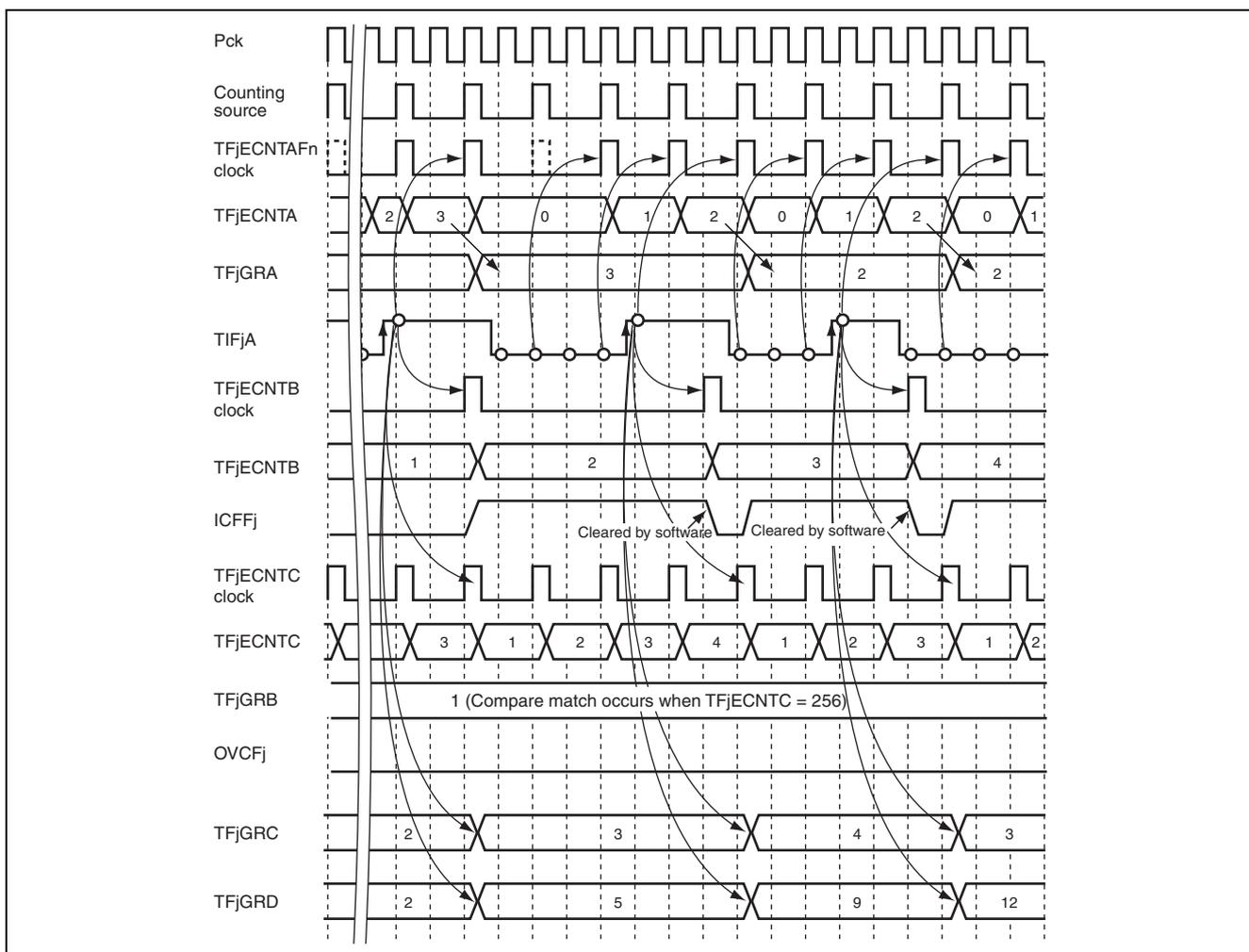
Figure 21.20 Operation Example of Rotation Speed/Pulse Measurement
