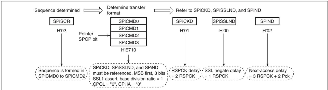
**Figure 24.19 Determination Procedure of Serial Transfer Mode in Master Mode**
