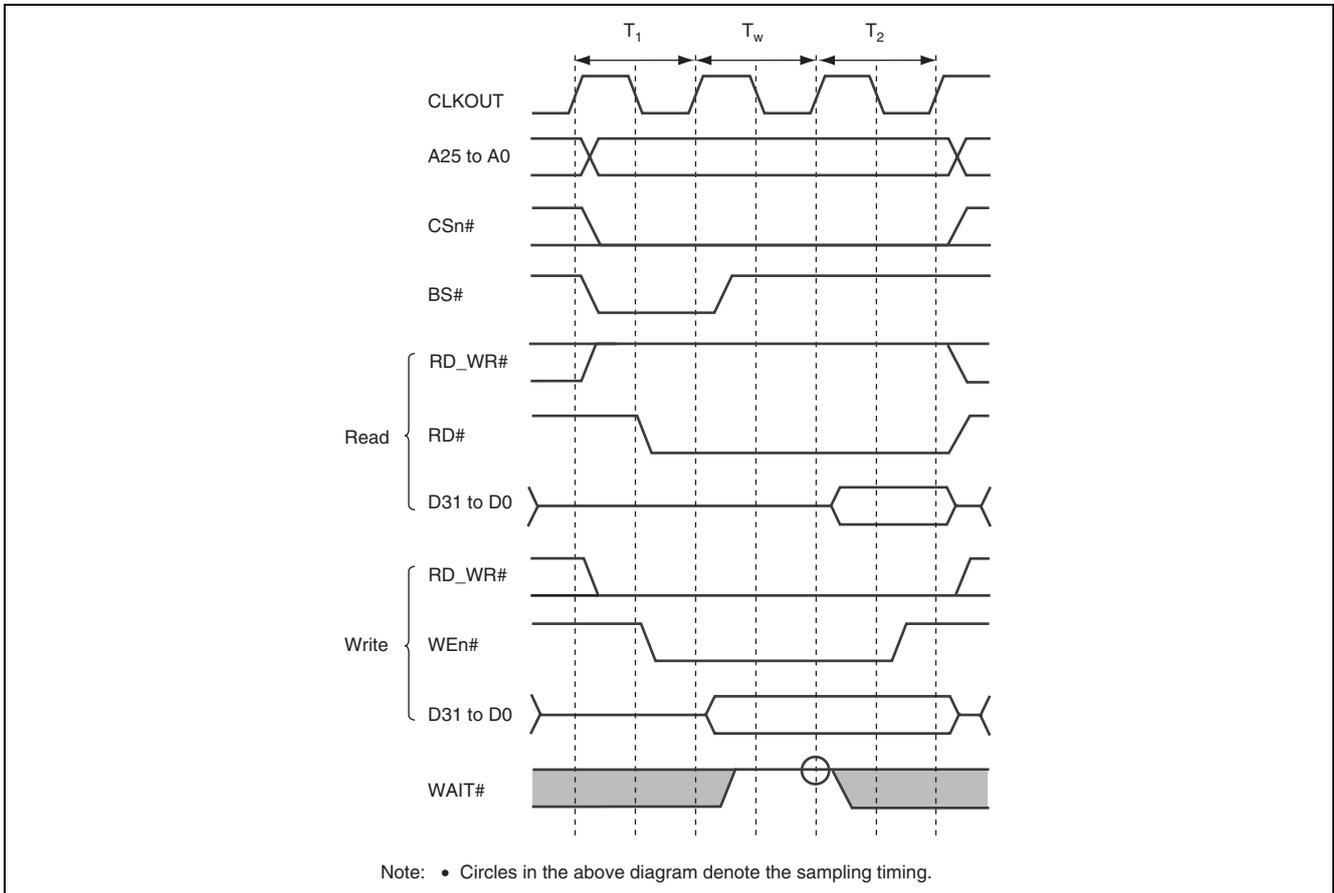
**Figure 19.7 SRAM Interface Wait Timing (Software Wait Only)**
