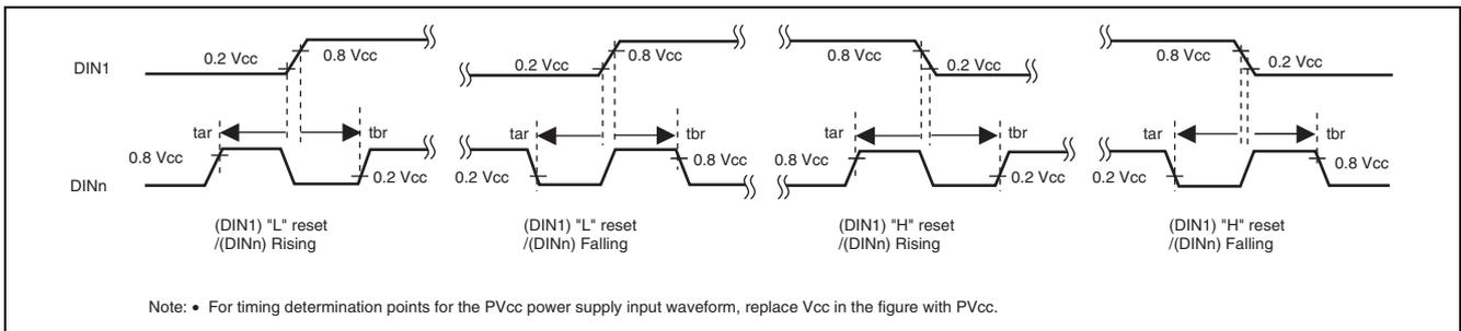
**Figure 38.35 DIN1/DIN2 to DIN4 Related Timing in Special Mode (DIN1 Reset Release Edge and Preceding or Subsequent Sampling Edge Interval)**
