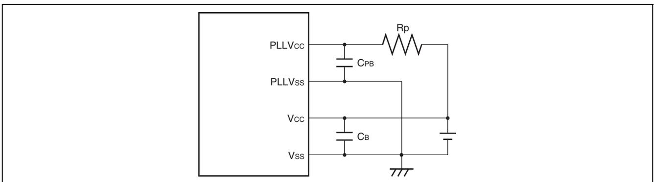
Figure 14.6 PLL Frequency Multiplier Circuit Power Supply Connection Notes
