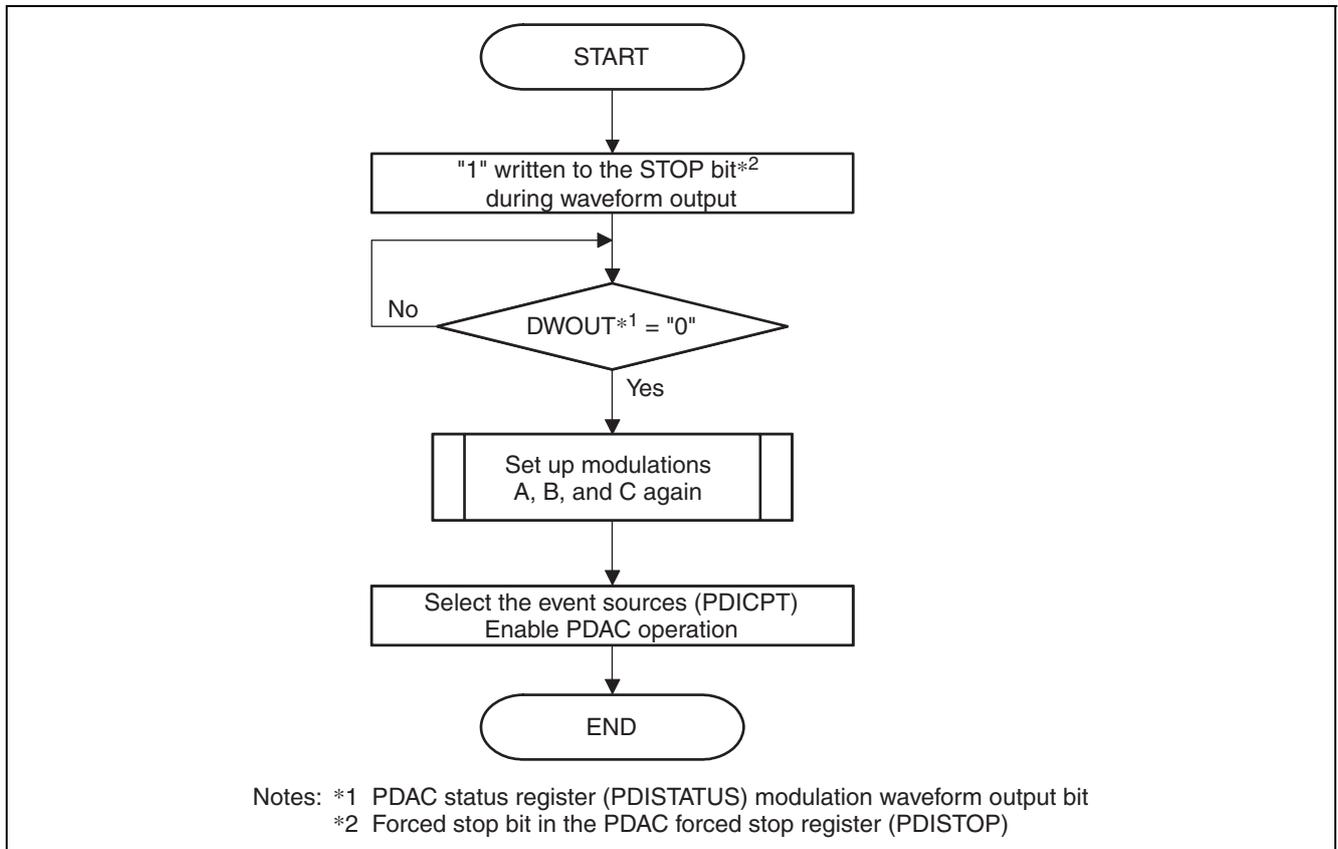
**Figure 30.15 Example of Forced Stop and the Following Recovery Procedure**
