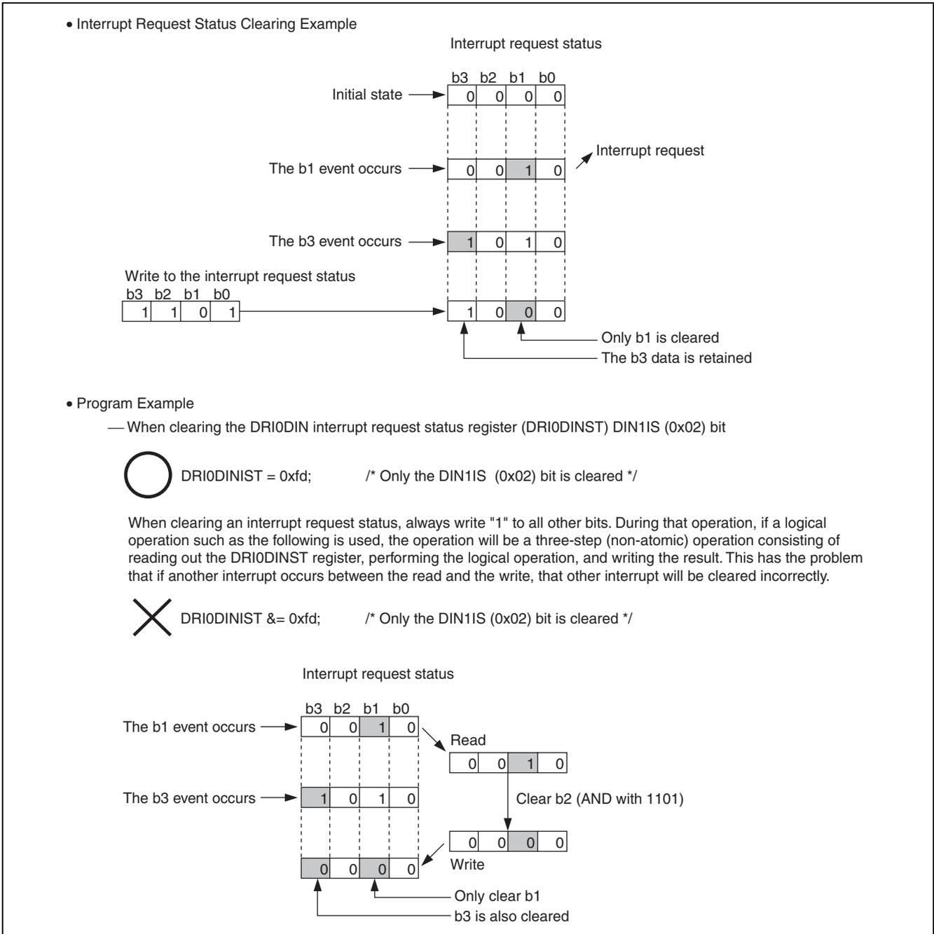
**Figure 28.3 Interrupt Request Status Clearing Examples**
