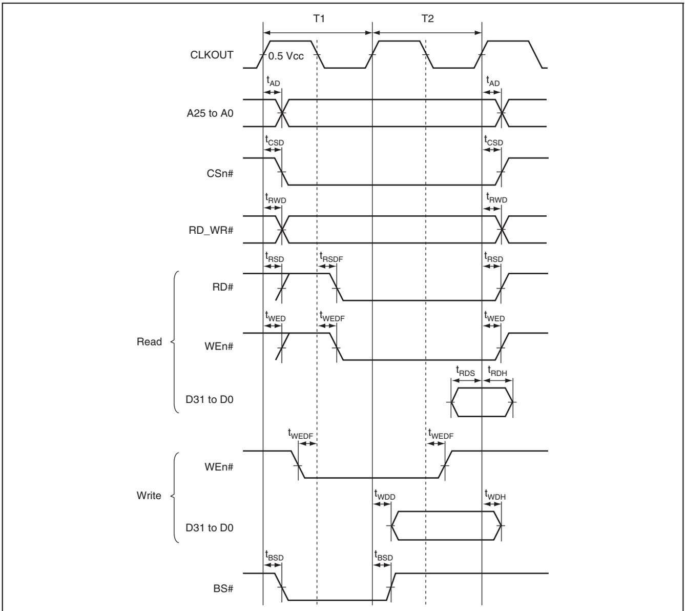
Figure 38.16 SRAM Bus Cycle with Byte Control (No Waits)
