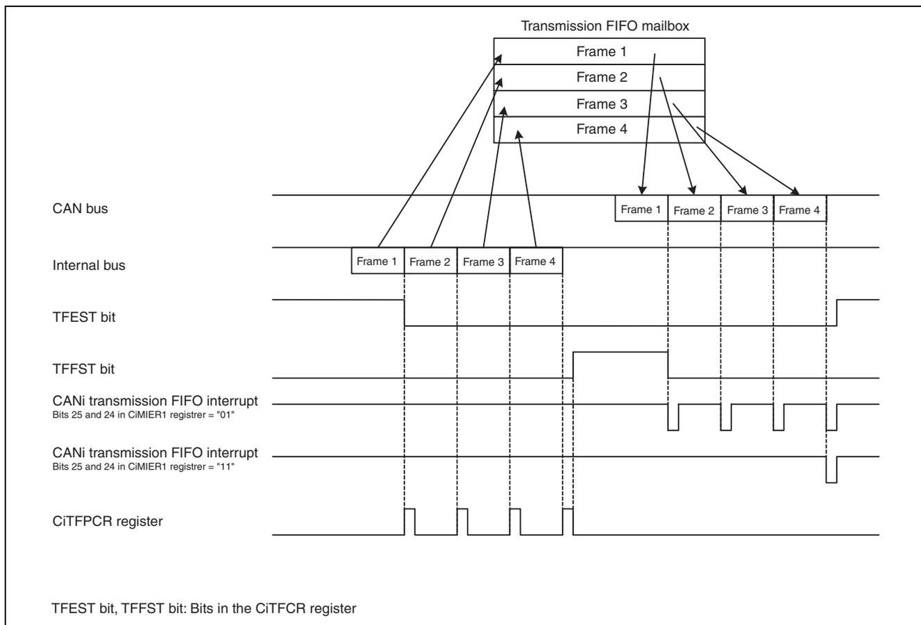
**Figure 26.3 Transmit FIFO Mailbox Operation (Bits 25 and 24 in CiMIER1 Register = "01" and "11")**
