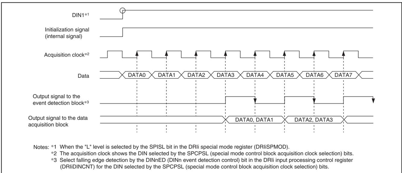
Figure 28.6 Timing Chart when Special Mode is Enabled
