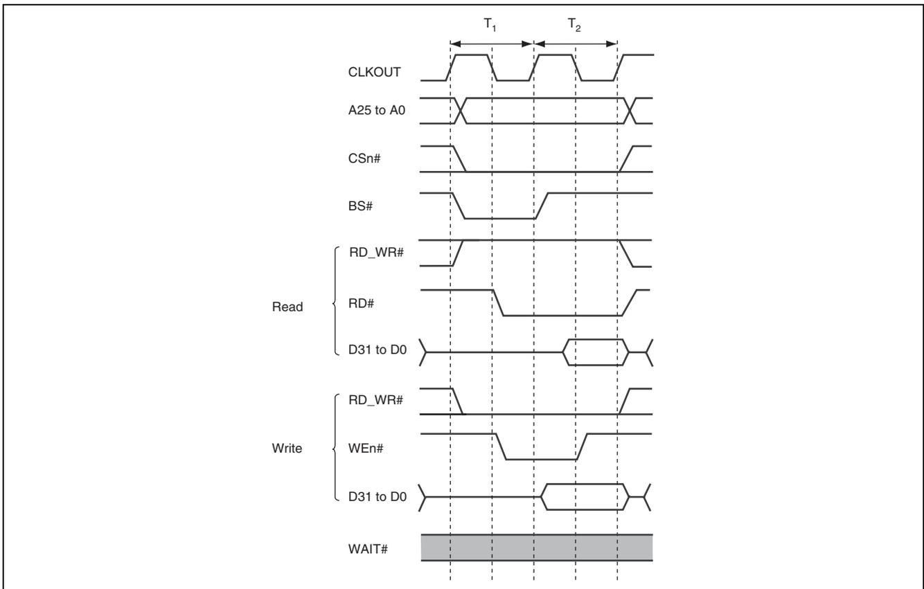
Figure 19.3 Basic Timing of SRAM Interface (No Wait)
