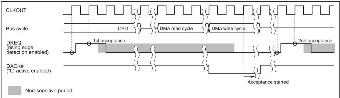
**Figure 20.11 Example of DREQ Input Detection (Cycle Steal Mode 1, DACK Write Cycle Output)**
