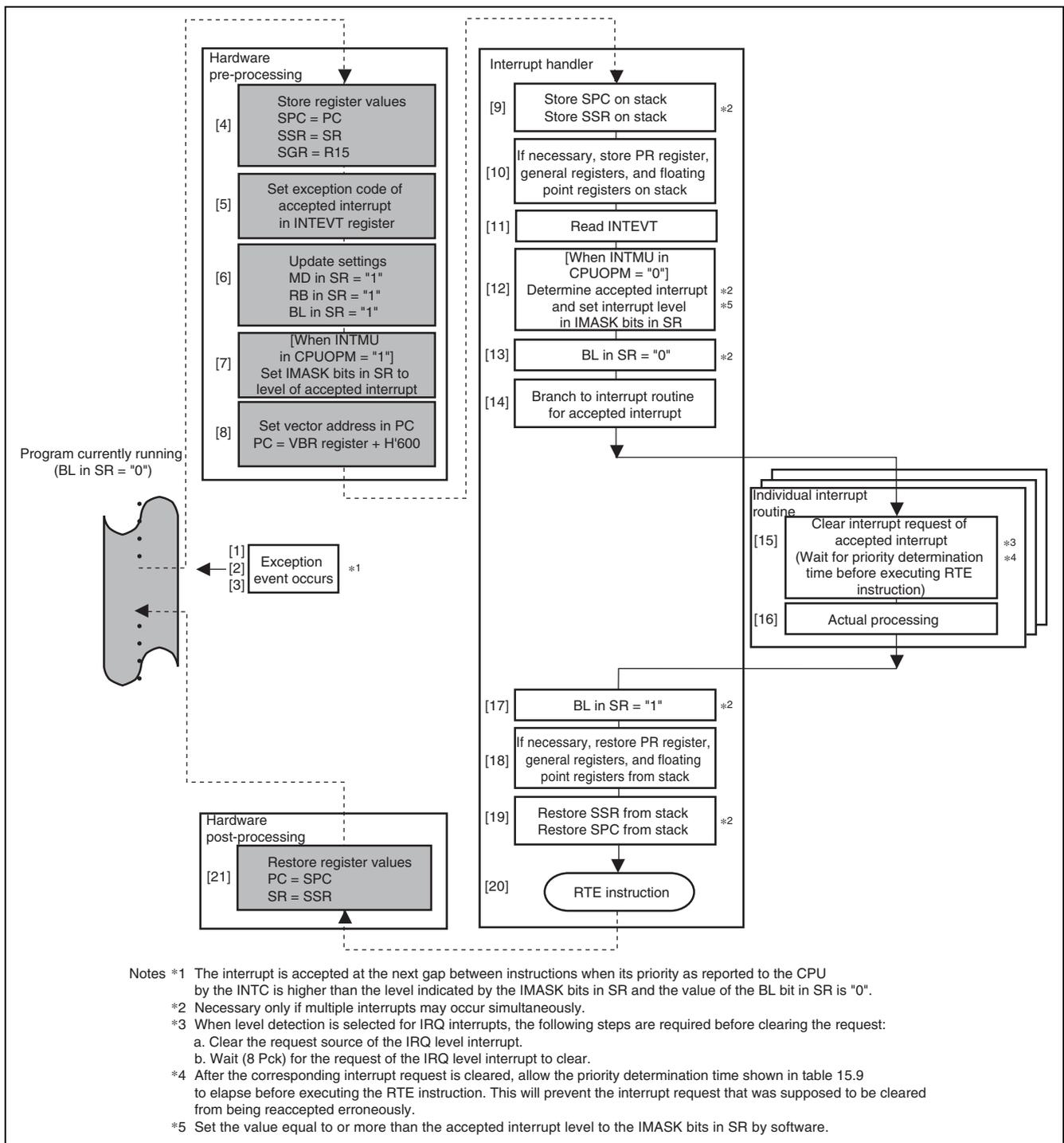
Figure 15.5 General Interrupt Operation Example 2
