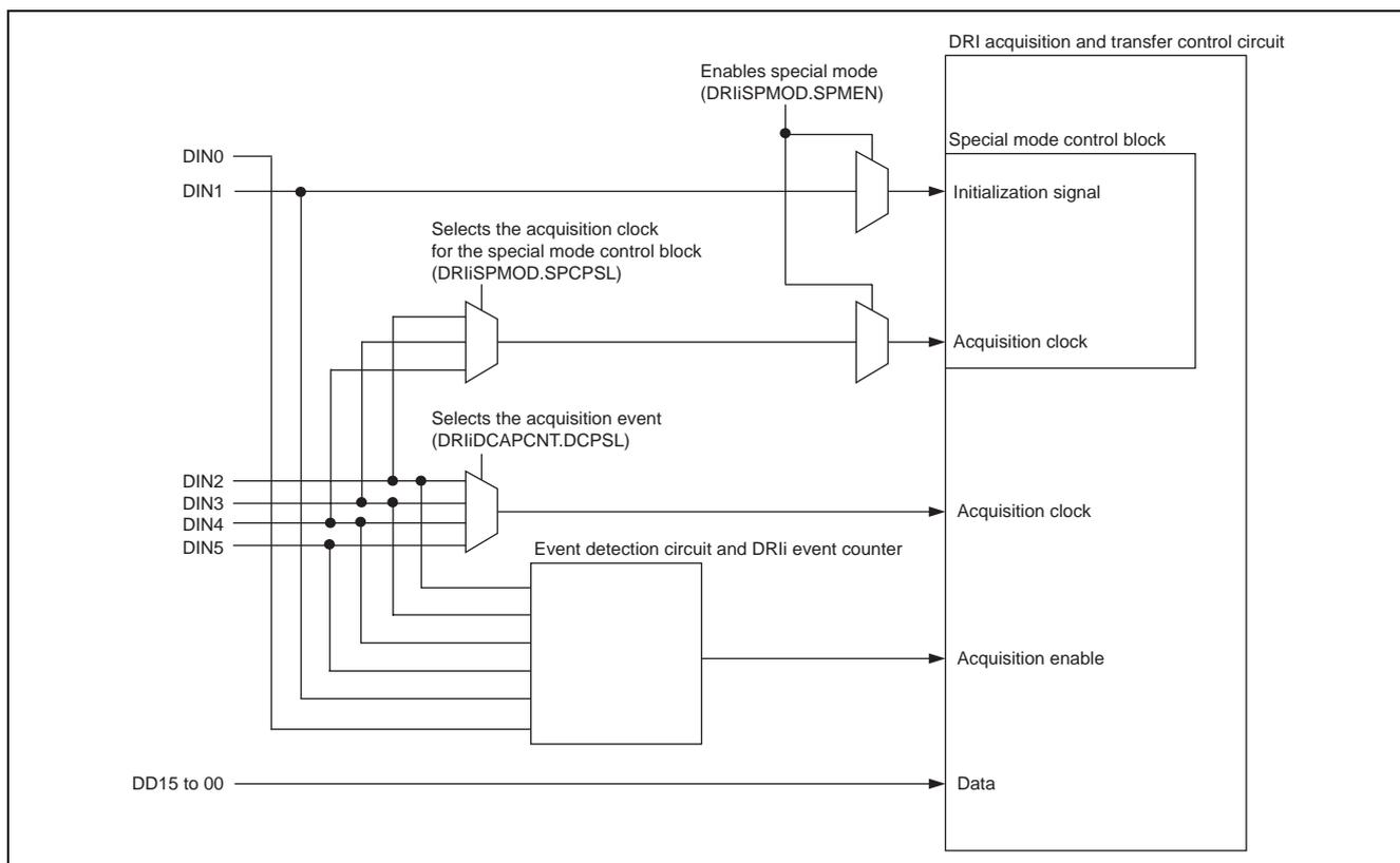
**Figure 28.13 Signal Connections to Turn on/off Special Mode**
