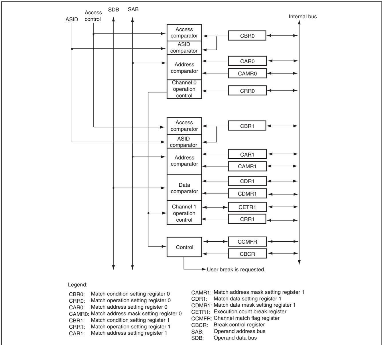
Figure 35.1 Block Diagram of UBC
