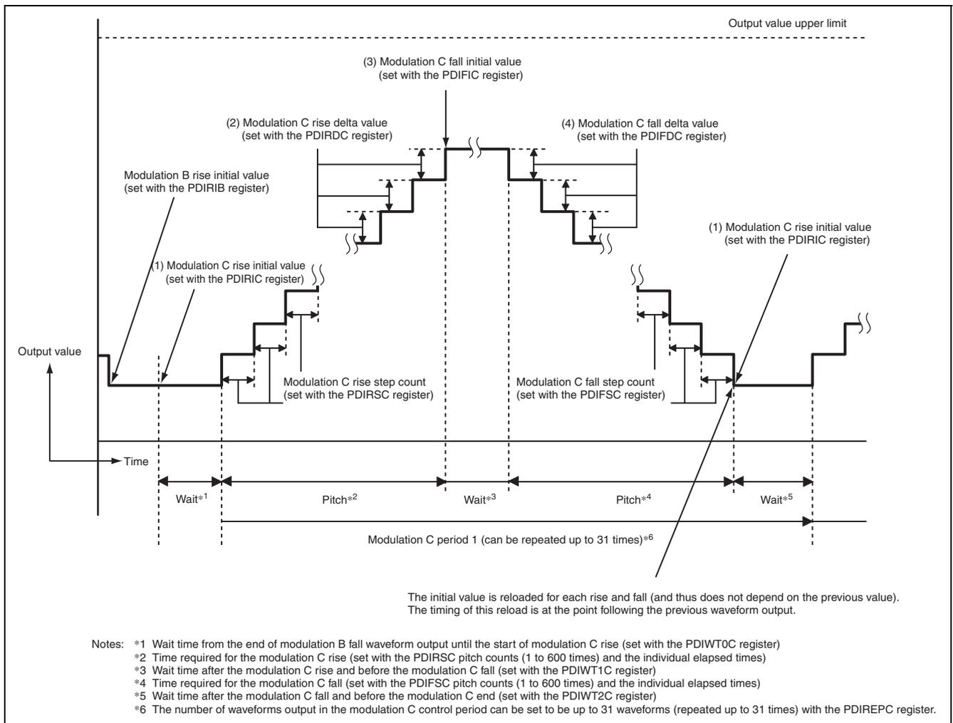
**Figure 30.11 Operational Overview of the Modulation C Waveform Output**
