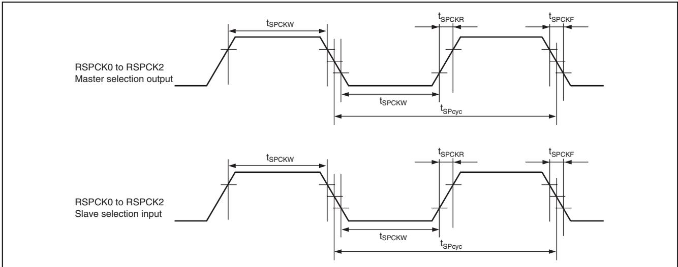
Figure 38.27 RSPI Clock Timing
