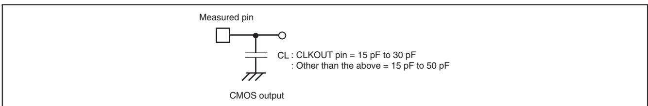
**Figure 38.1 Measurement Circuit for Output Switching Characteristics**
