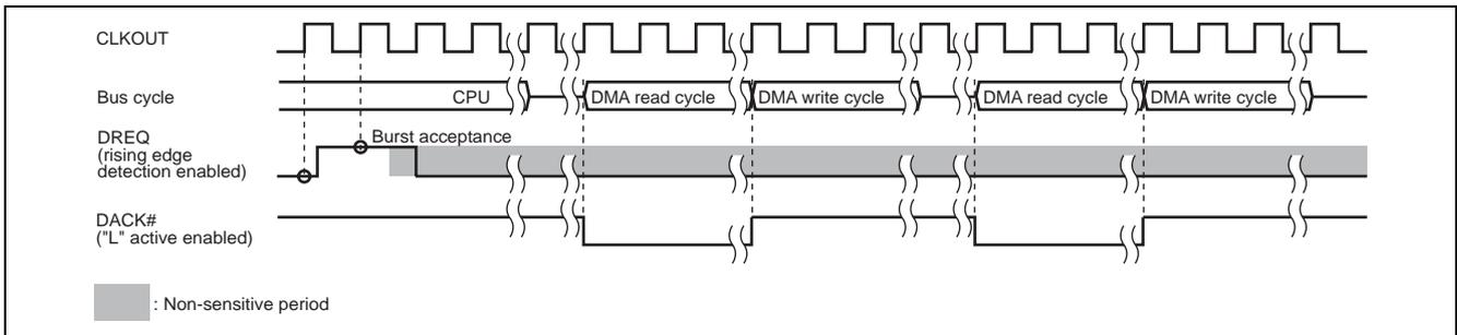
**Figure 20.14 Example of DREQ Input Detection (Burst mode, DACK Read Cycle Output)**
