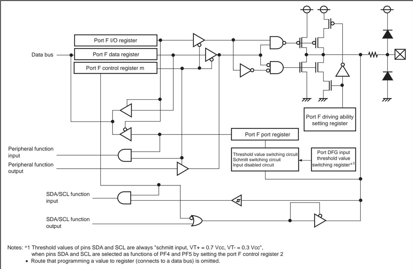
Figure 18.3 Port Peripheral Circuit Diagram (Input/Output Ports 3)
