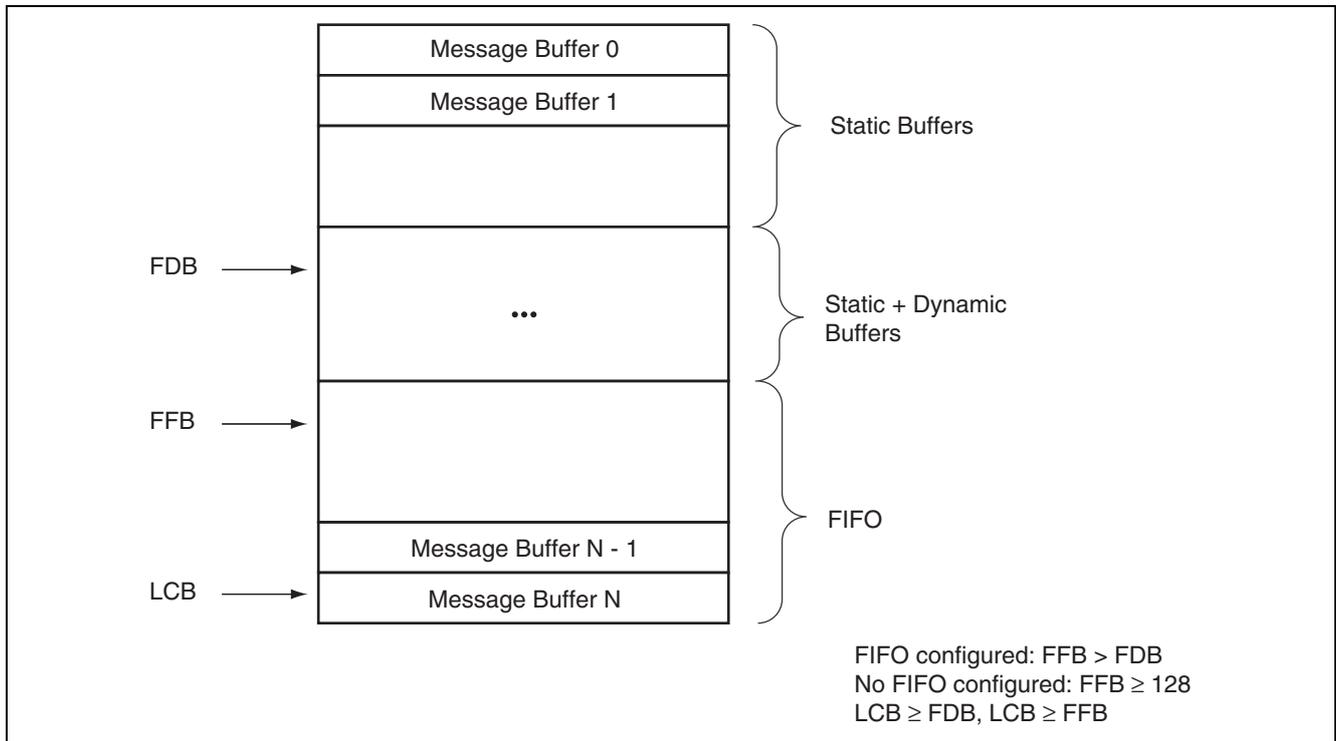
**Figure 32.3 Message Buffer Structure**
