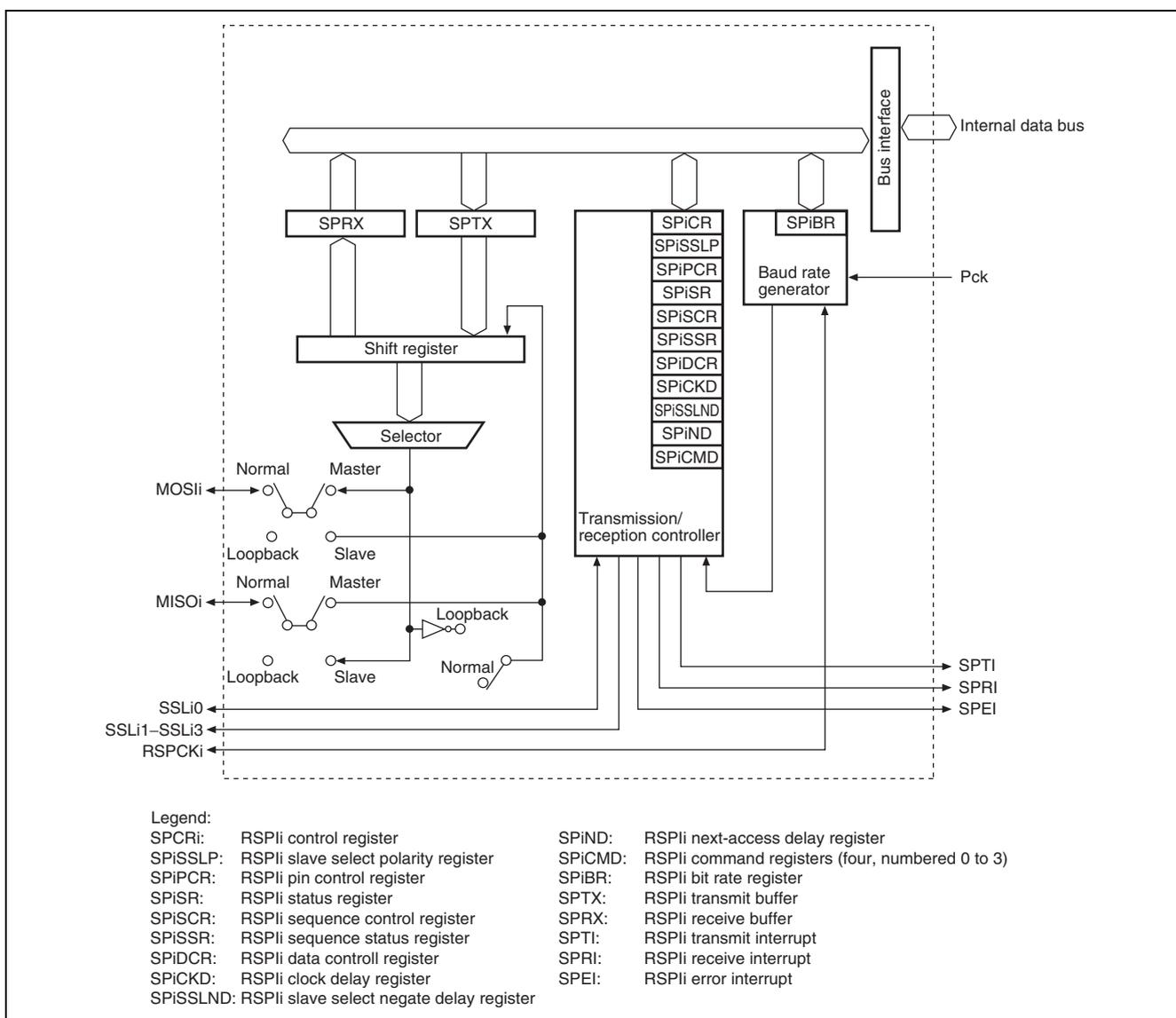
Figure 24.1 Block Diagram of RSPIi
