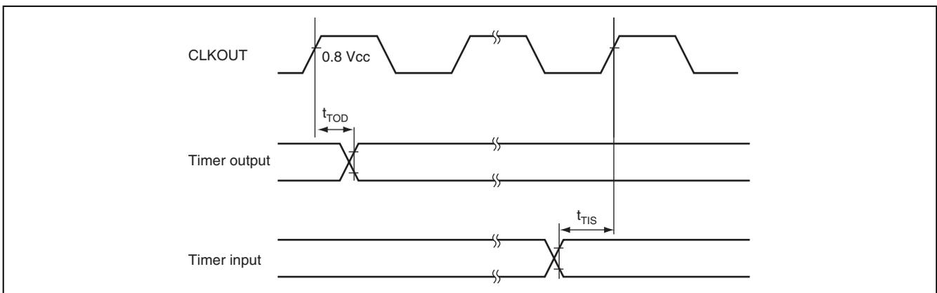
**Figure 38.21 ATU-IIIS Input/Output Timing**
