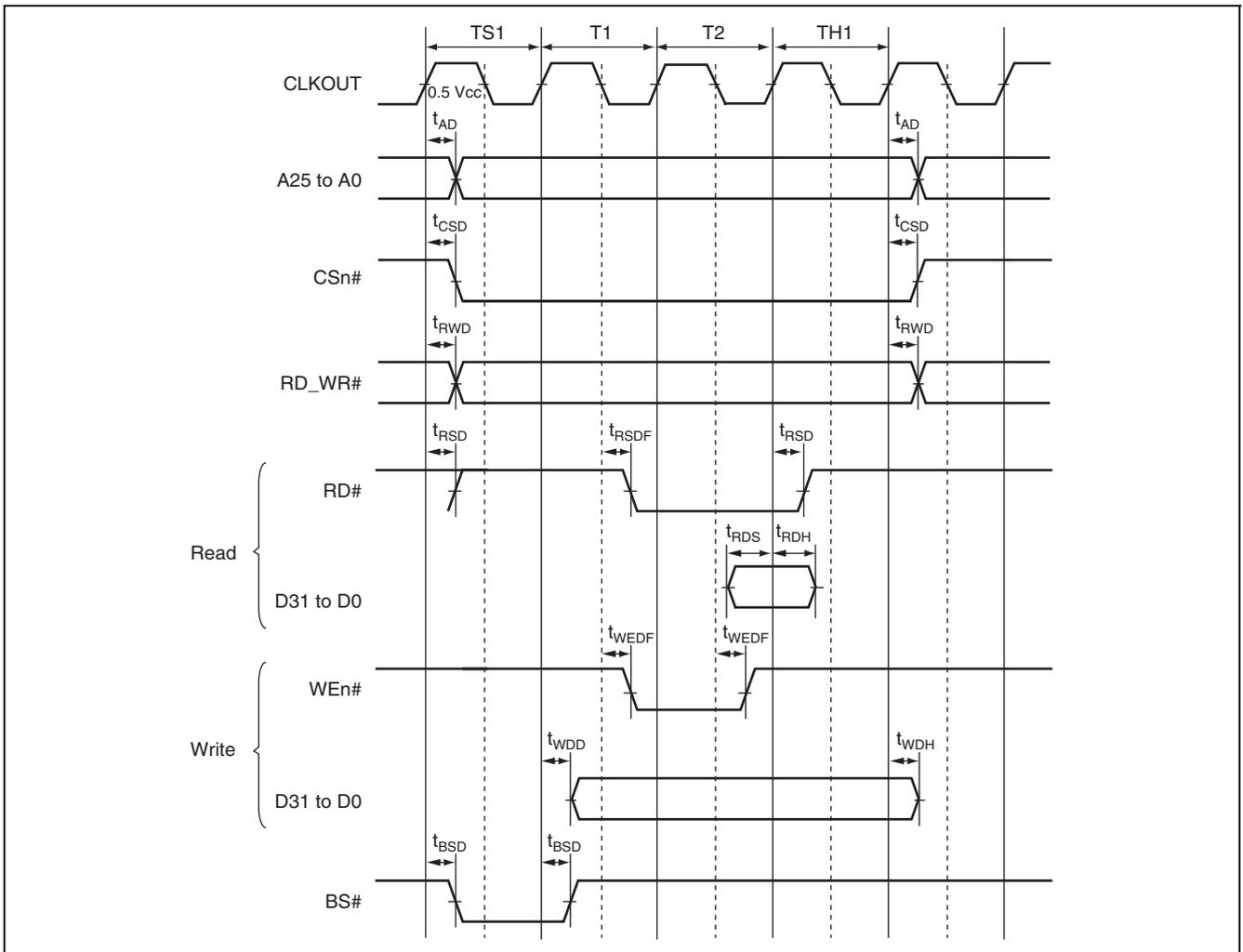
Figure 38.15 SRAM Bus Cycle (No Waits, No Address Setup/Hold, RDS = 1, RDH = 1, WTS = 1, WTH = 1)
