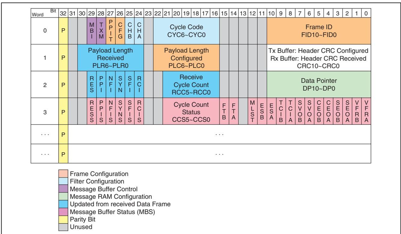
Figure 32.18 Header Section of a Message Buffer in the Message RAM
