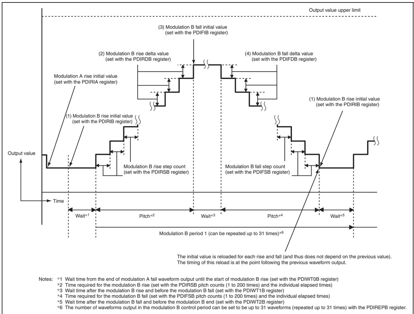
**Figure 30.10 Operational Overview of the Modulation B Waveform Output**
