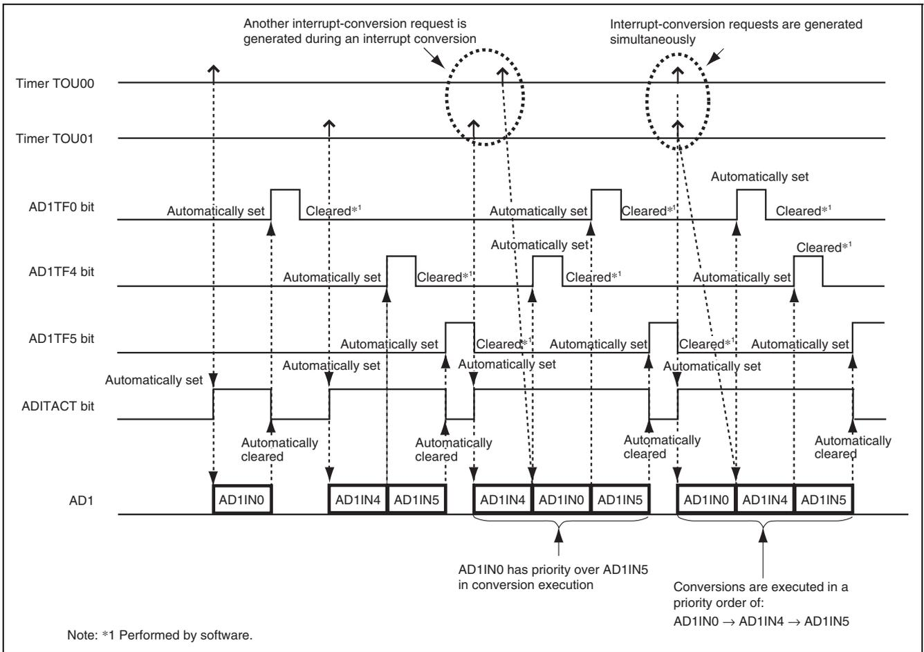
Figure 27.6 Example Operation of Interrupt Conversion
