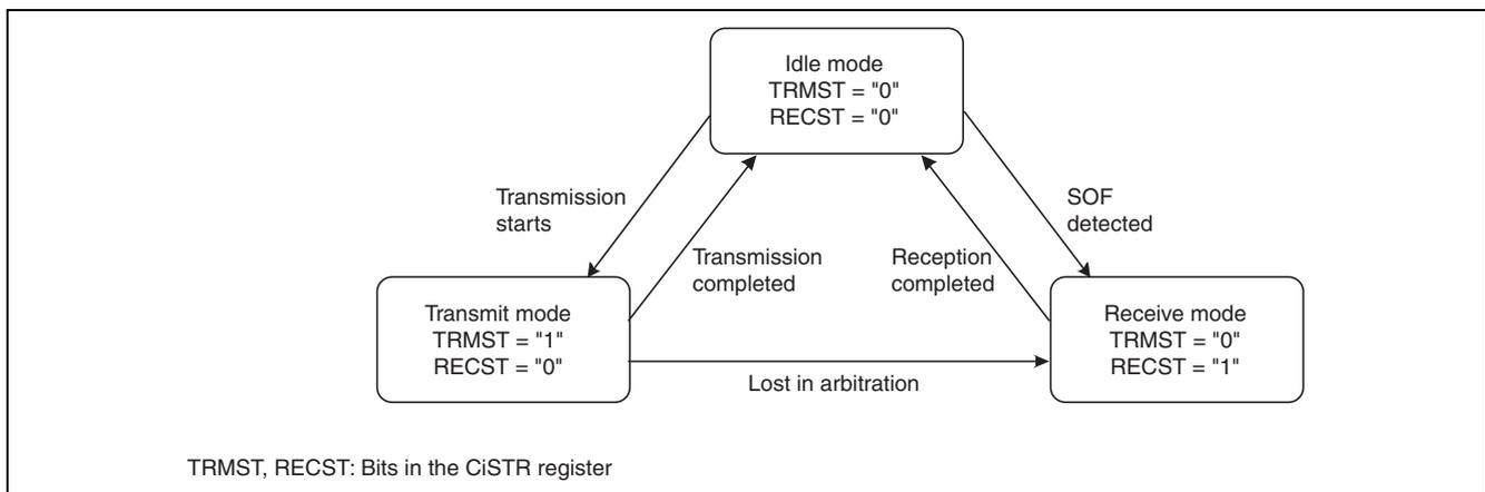
**Figure 26.10 Sub Mode in CAN Operation Mode (i = 0 to 4)**
