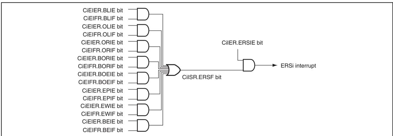
**Figure 26.26 Block Diagram of CANi Error Interrupt [ERSi]**
