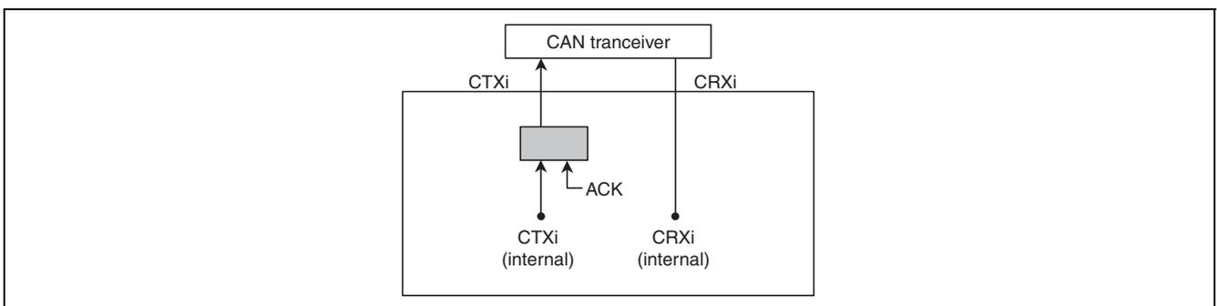
**Figure 26.7 Connection when Self-Test Mode 0 is Selected**
