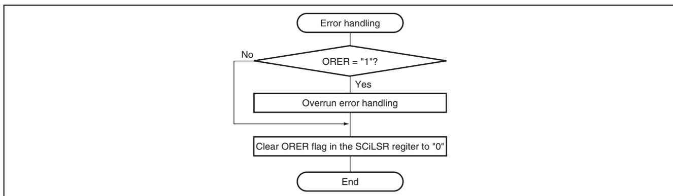
**Figure 23.16 Sample Flowchart for Receiving Serial Data (2)**
