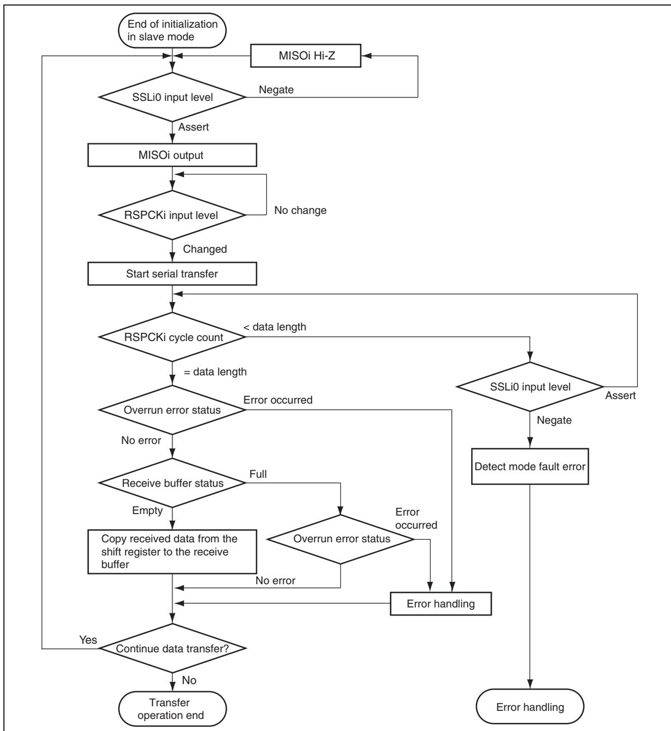
**Figure 24.25 Transfer Operation Flowchart in Slave Mode (CPHA = "1")**
