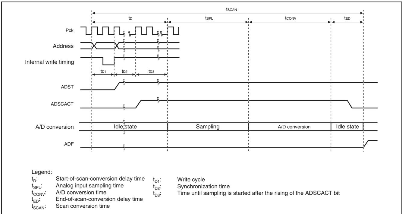
**Figure 27.8 Timing Diagram for Scan Conversion (Single Channel, Single Cycle)**
