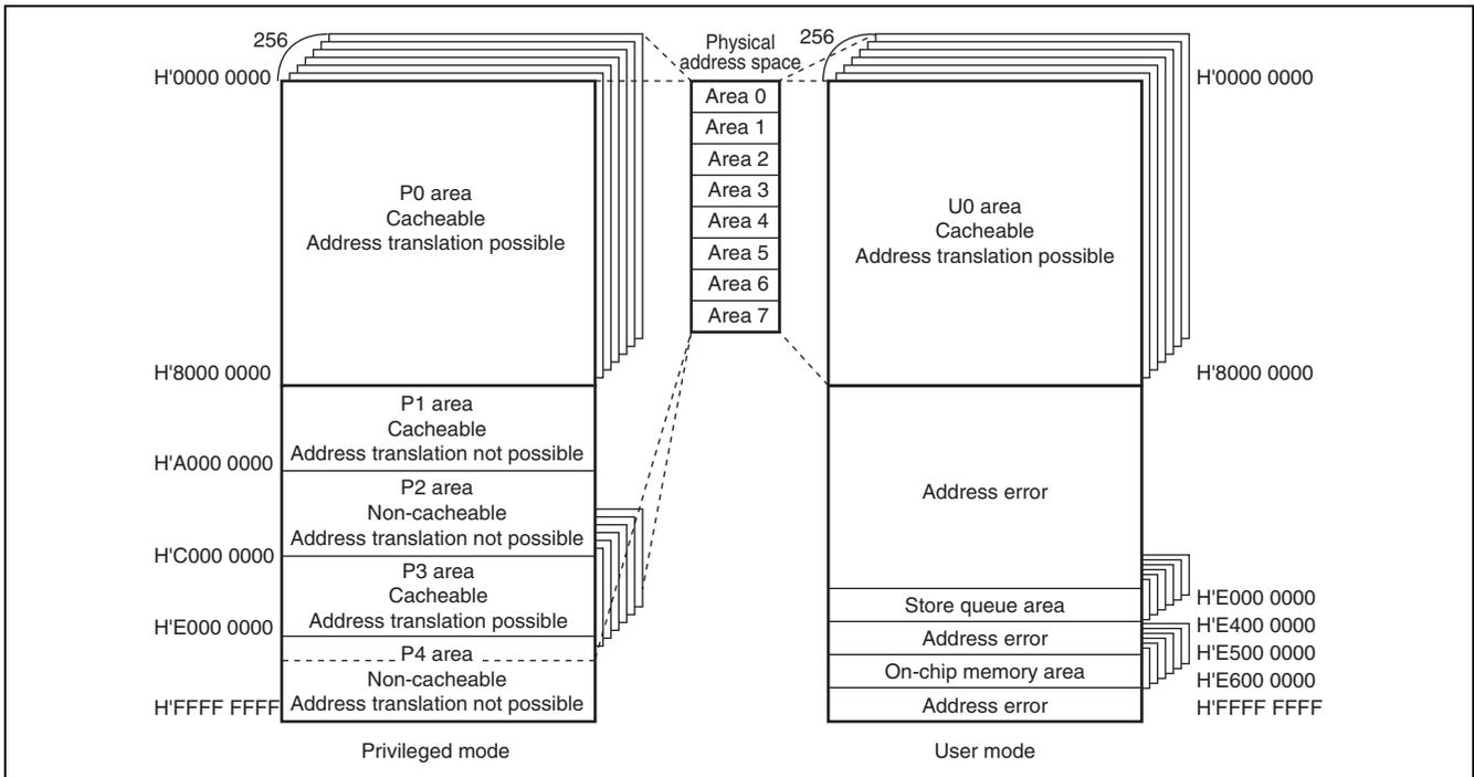
Figure 7.3 Virtual Address Space (AT in MMUCR = 1)
