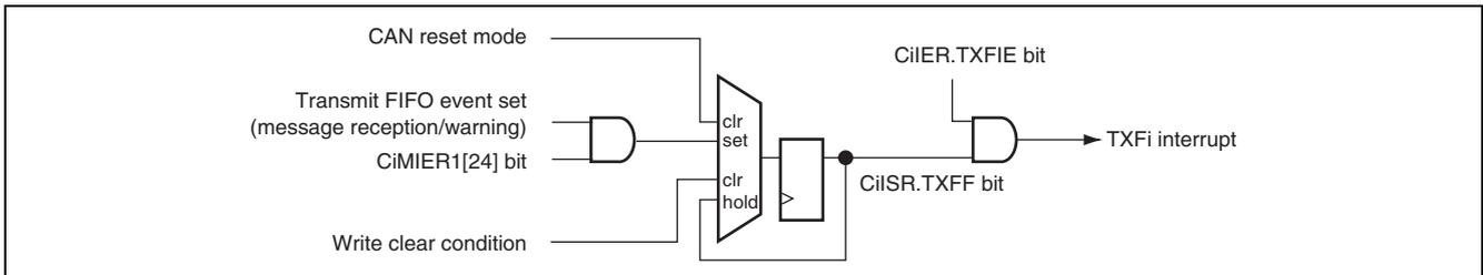
**Figure 26.25 Block Diagram of CANi Transmit FIFO Interrupt [TXFi]**
