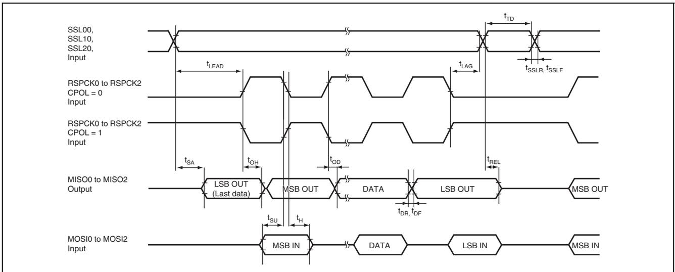
Figure 38.31 RSPI Timing (Slave, CPHA = "1")
