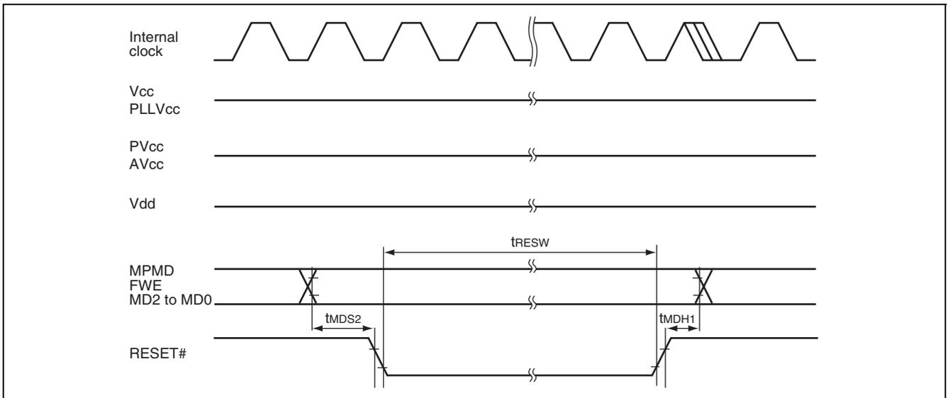
**Figure 38.6 Operation Mode and Oscillation Timing during Operation**
