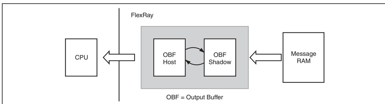
**Figure 32.14 Double Buffer Structure Output Buffer**
