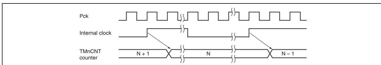
Figure 22.4 Count Timing when Operating on Internal Clock
