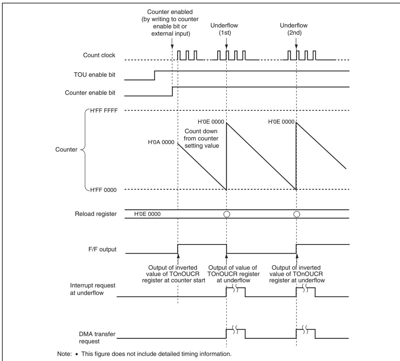
**Figure 21.36 Operation Example of Continuous Output Mode**
