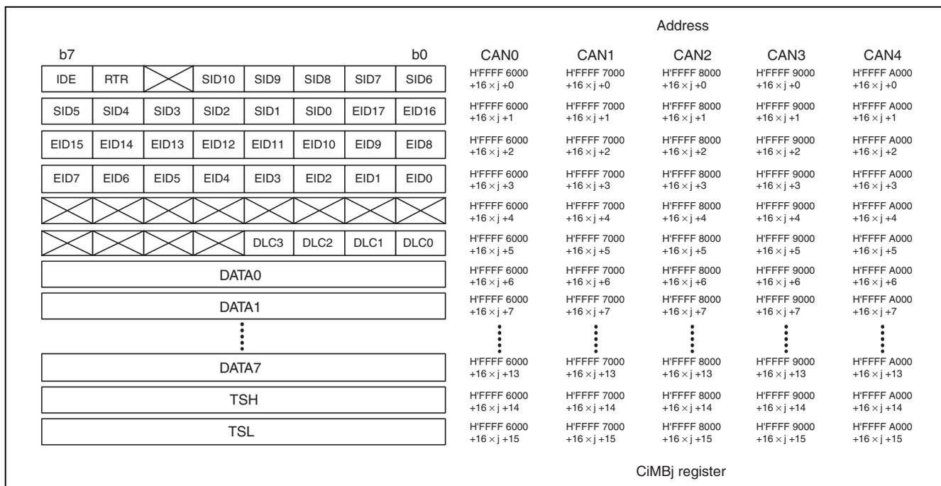
Figure 26.13 Structure of CiMBj Register (i = 0 to 4; j = 0 to 63)
