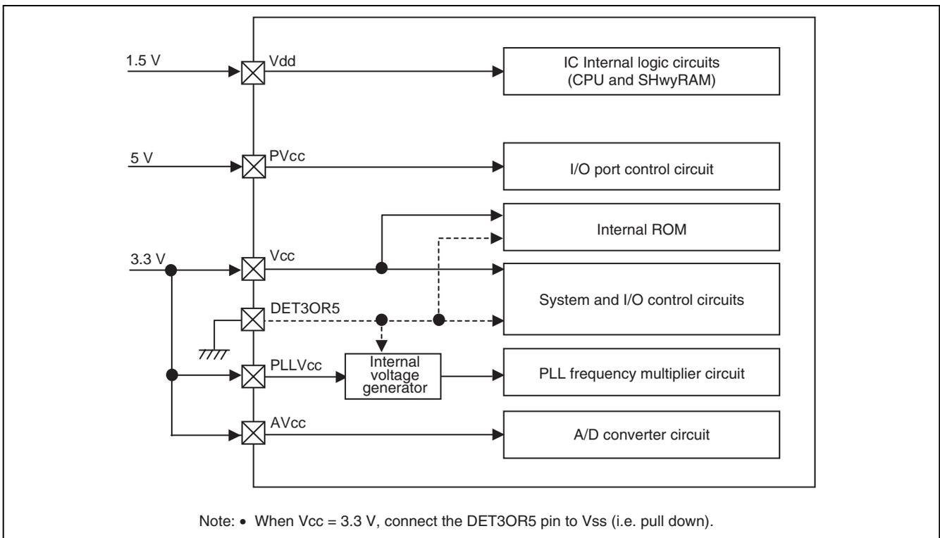
**Figure 34.2 Power Supply Circuit Structure (when  $PV_{cc} = 5\text{ V}$ ,  $V_{cc} = 3.3\text{ V}$ )**
