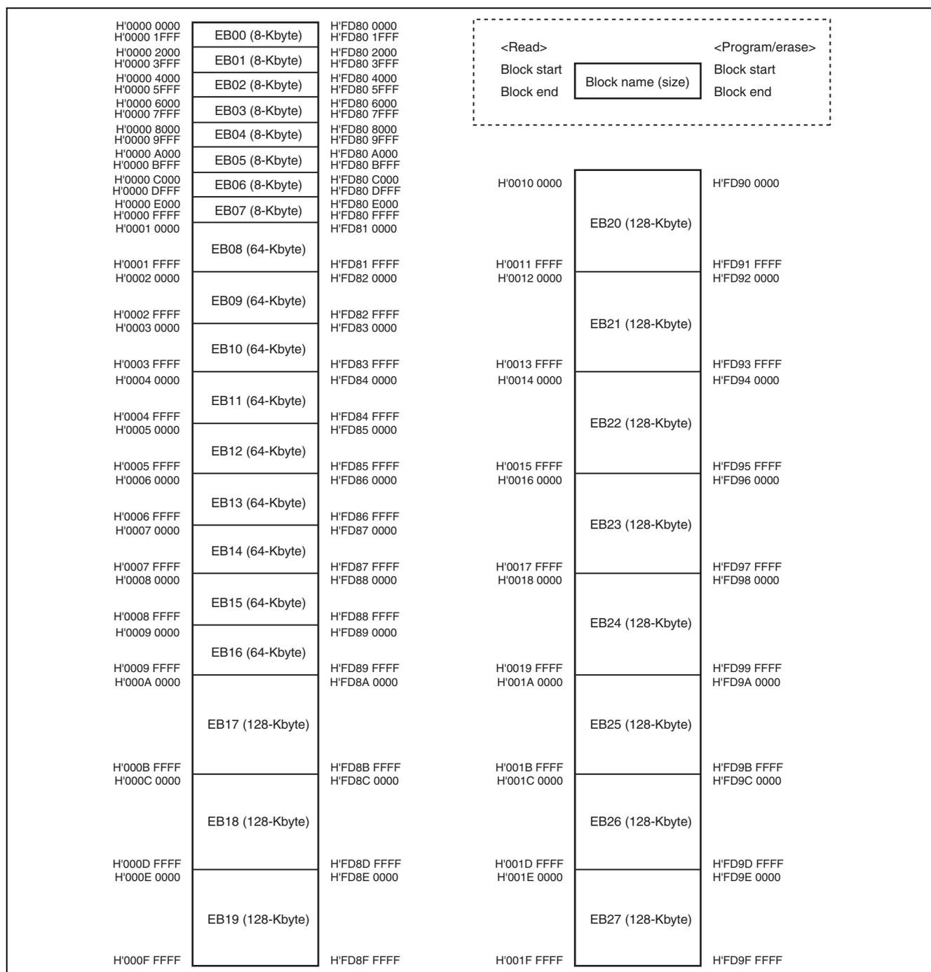
Figure 12.3 SH74504 User MAT and Block Allocation
