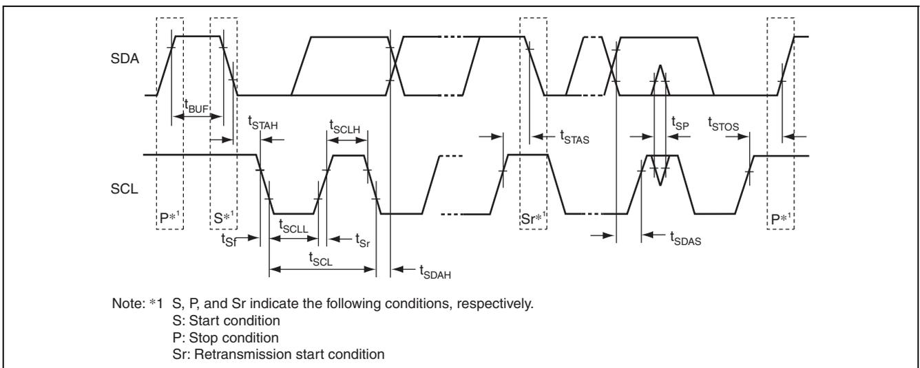
**Figure 38.32 IIC3 Module Input/Output Timing**
