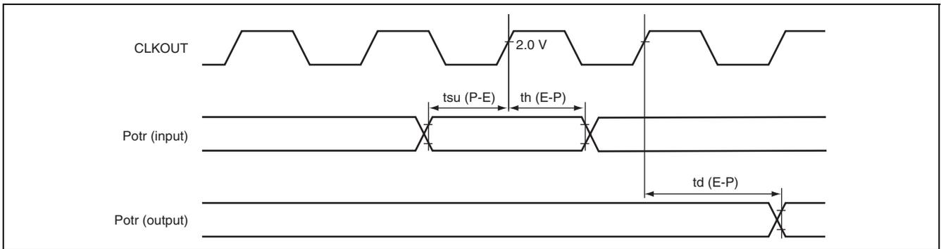
**Figure 38.23 I/O Port Input/Output Timing**
