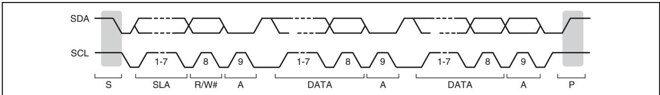
Figure 25.4 I<sup>2</sup>C Bus Timing
