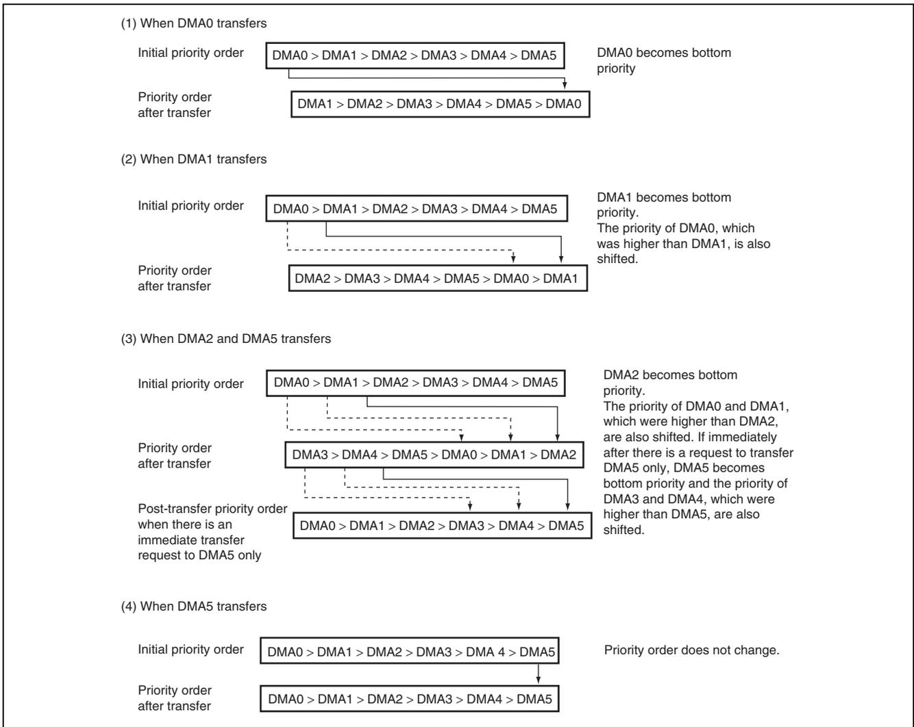
**Figure 20.5 Example 1 of Changes in Channel Priority (Round Robin)**
