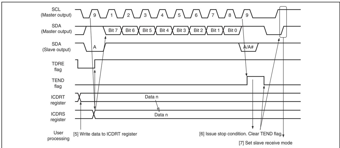
**Figure 25.6 Master Transmit Mode Operation Timing (2)**
