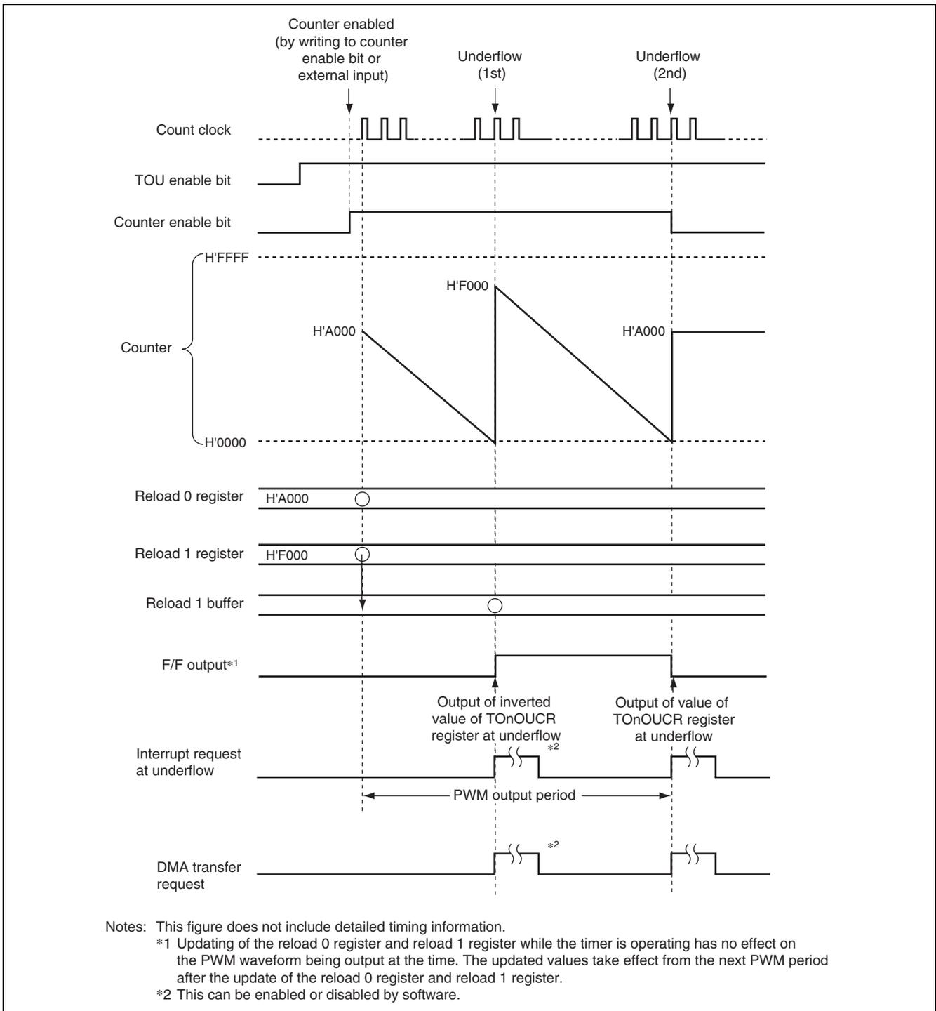
Figure 21.32 Operation Example of One-Shot PWM Output Mode
