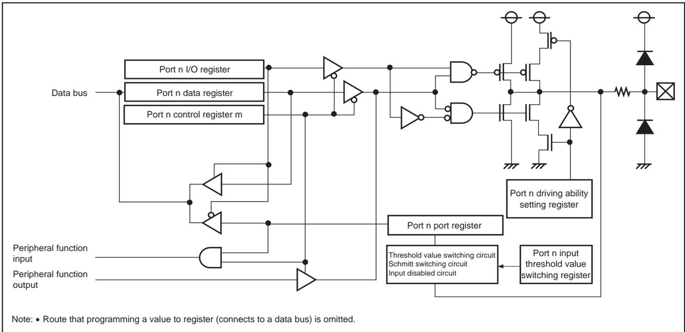
**Figure 18.1 Port Peripheral Circuit Diagram (Input/Output Ports 1)**
