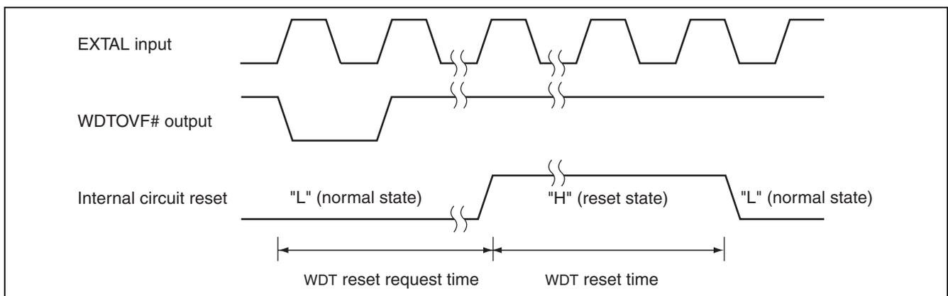
Figure 17.3 WDT Overflow Hardware Reset During Normal Operation
