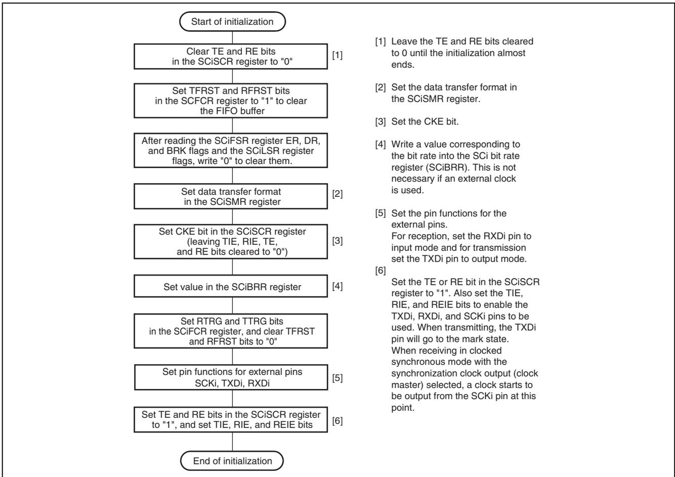
Figure 23.12 Sample Flowchart for SCIFi Initialization
