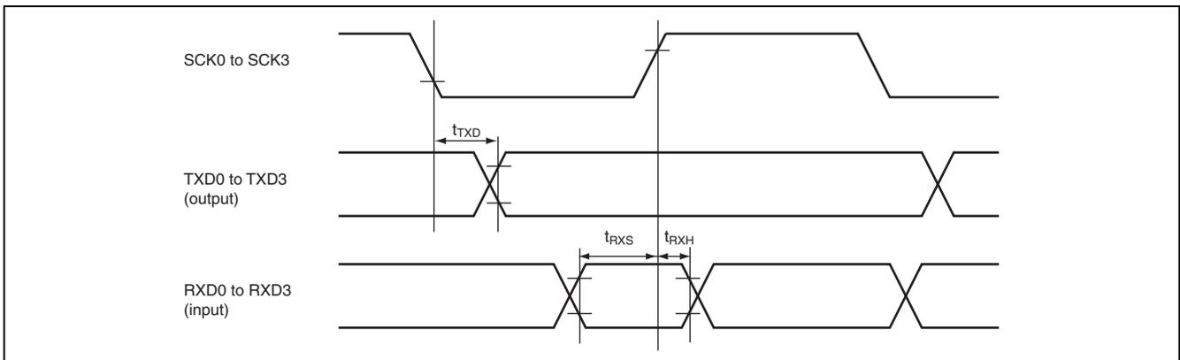
**Figure 38.26 SCI Input/Output Timing**
