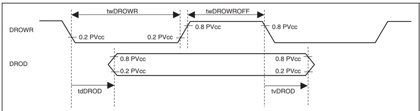
**Figure 38.37 Strobe Polarity with "L" Active Selected**
