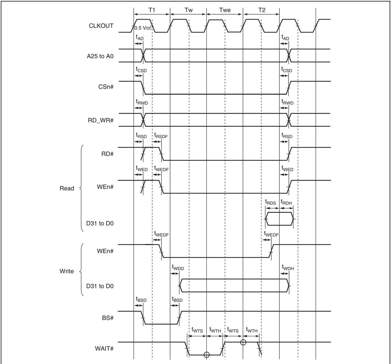
Figure 38.18 SRAM Bus Cycle with Byte Control (One Software Wait Cycle, One External Wait Cycle)
