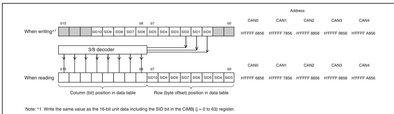
**Figure 26.5 Write and Read of CiAFSR Register (i = 0 to 4)**
