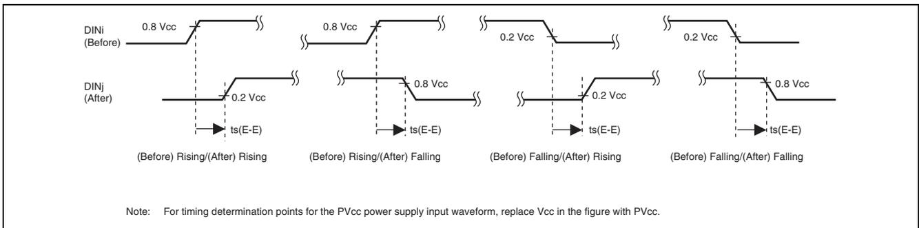
**Figure 38.34 Edge Detection Timing (Edge Interval to Prevent DRI Internal Simultaneous Edge Detection Timing)**
