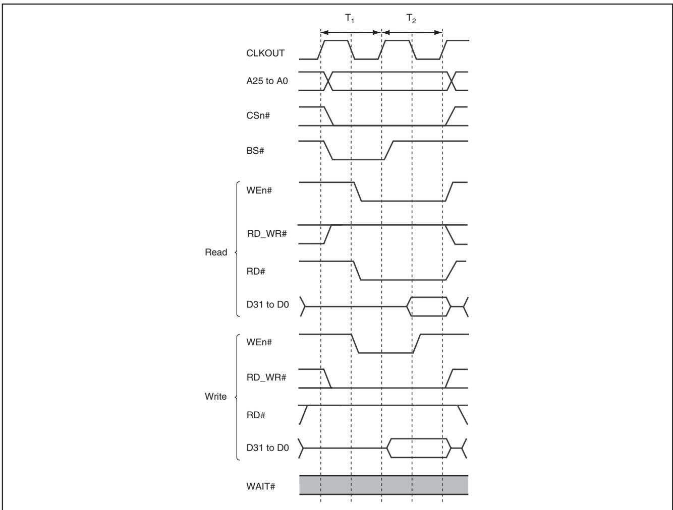
Figure 19.12 Byte Control SRAM Basic Access Timing (With No Wait States)
