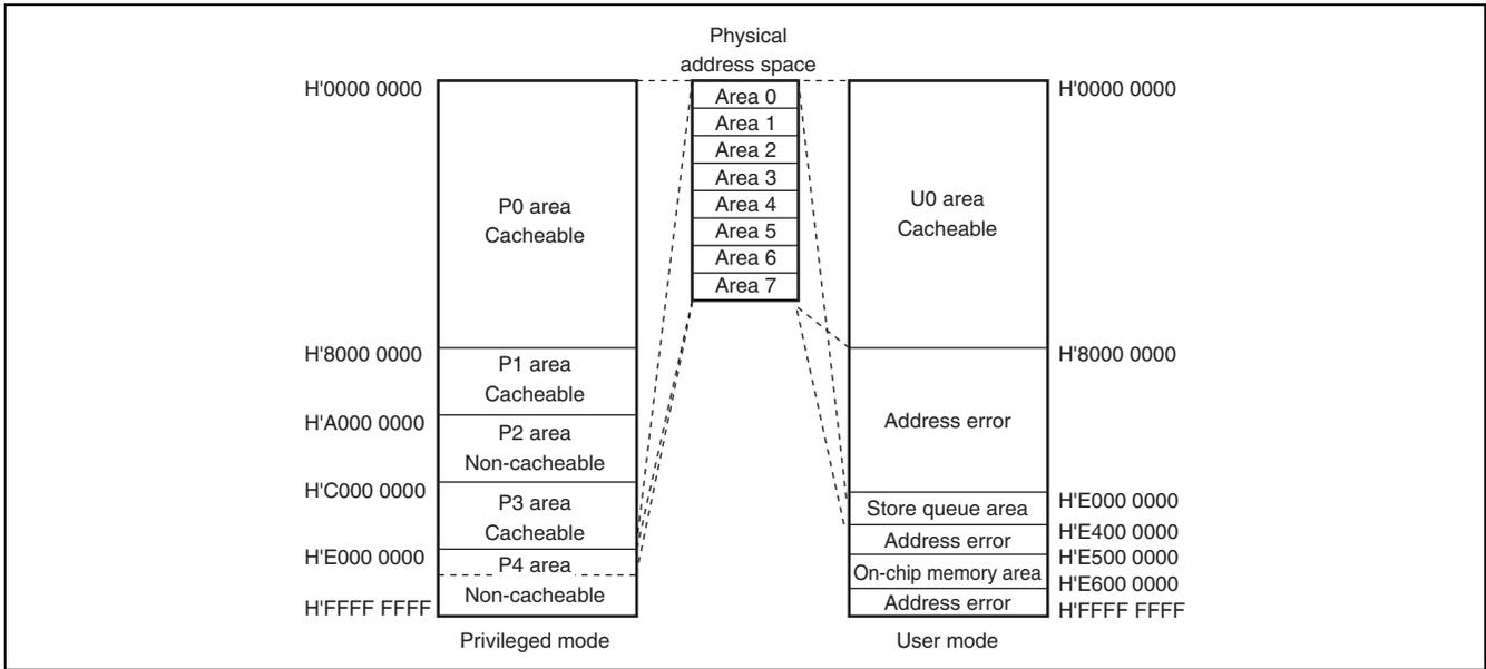
Figure 7.2 Virtual Address Space (AT in MMUCR = 0)
