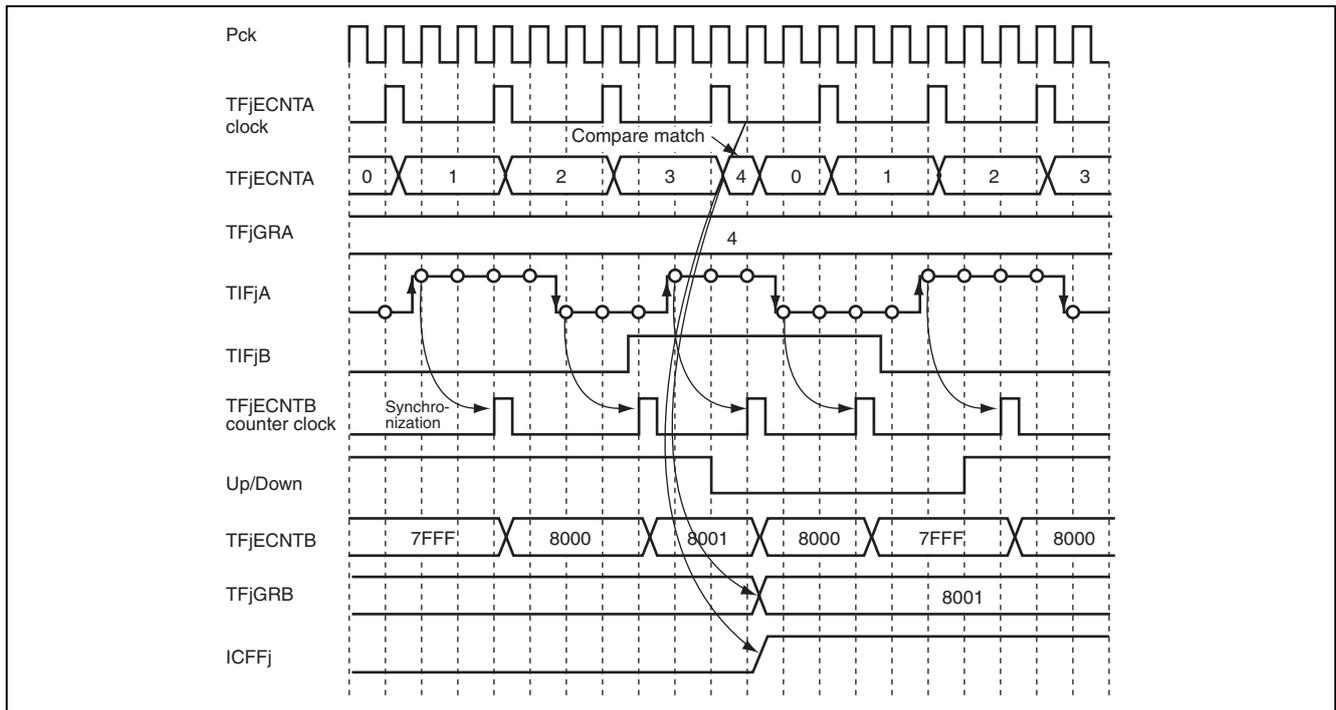
**Figure 21.21 Operation Example of Up/Down Event Count**
