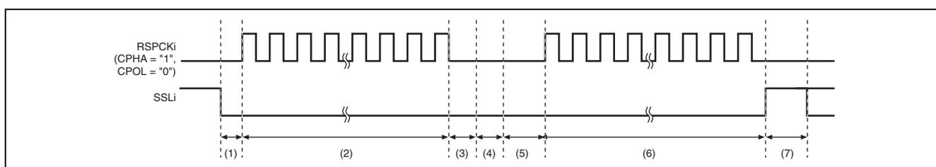
**Figure 24.20 Example of Burst Transfer Operation using SSLKP Bit**
