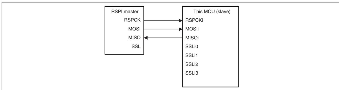
**Figure 24.10 Master (Clock-Synchronous Operation)/Slave (Clock-Synchronous Operation) Configuration Example (This MCU = Slave, CPHA = "1")**
