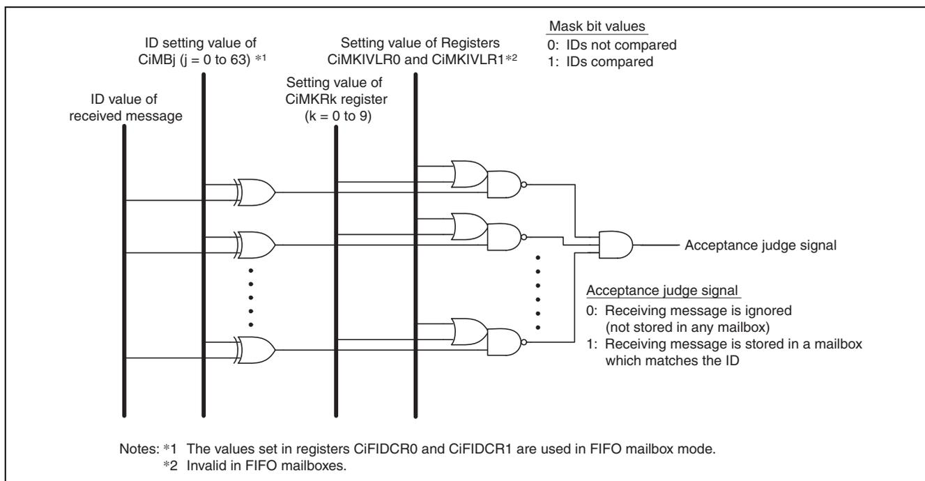
**Figure 26.17 Acceptance Filtering (i = 0 to 4)**
