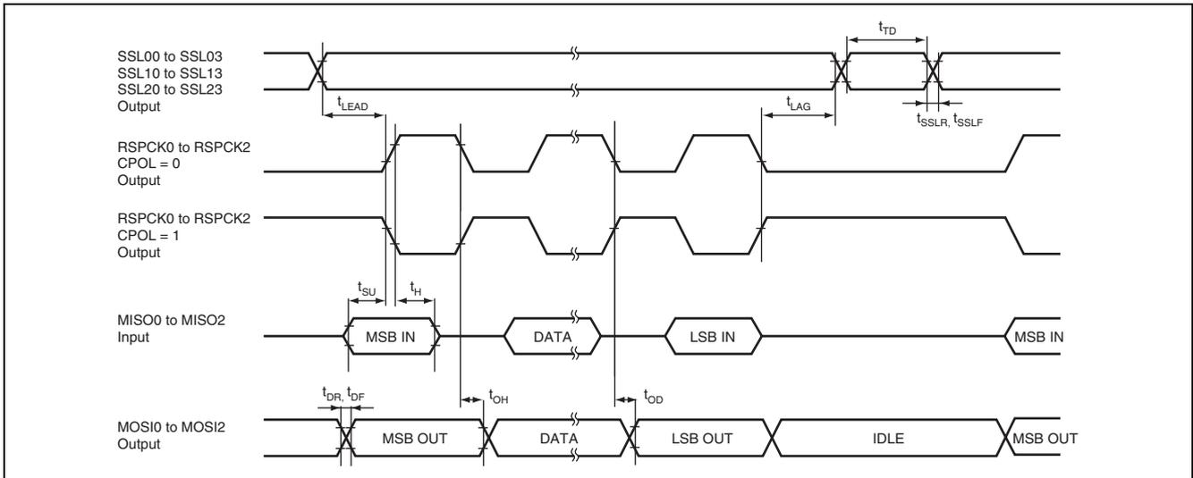
Figure 38.28 RSPI Timing (Master, CPHA = "0")
