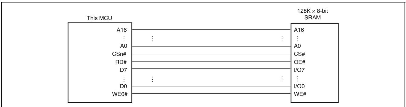
**Figure 19.6 Example of 8-Bit Data-Width SRAM Connection**
