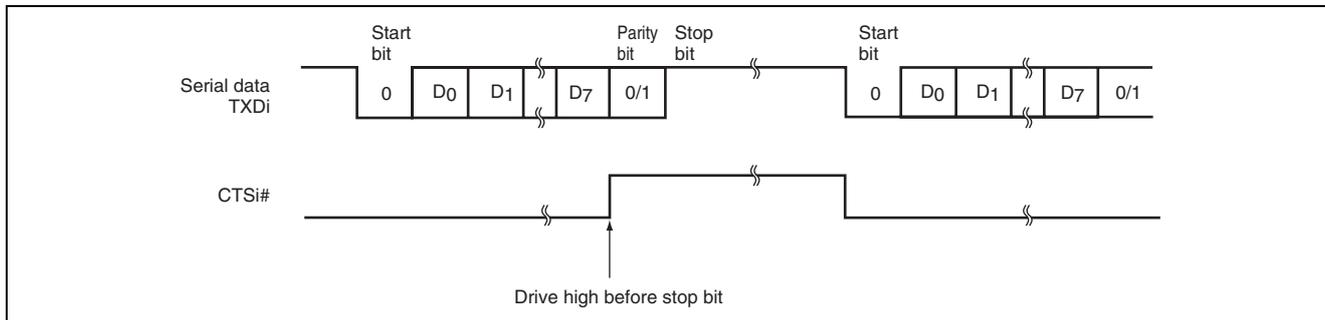
Figure 23.6 Example of Operation Using Modem Control (CTSi#)
