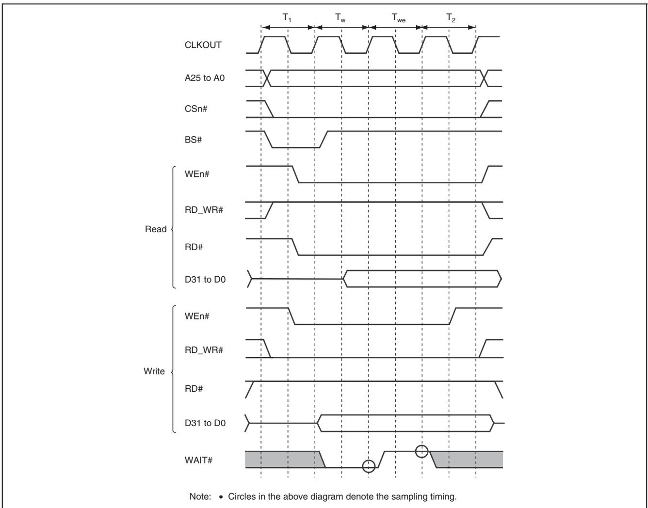
**Figure 19.14** Byte Control SRAM Basic Access Timing (One Internal Wait Cycle + One External Wait)
