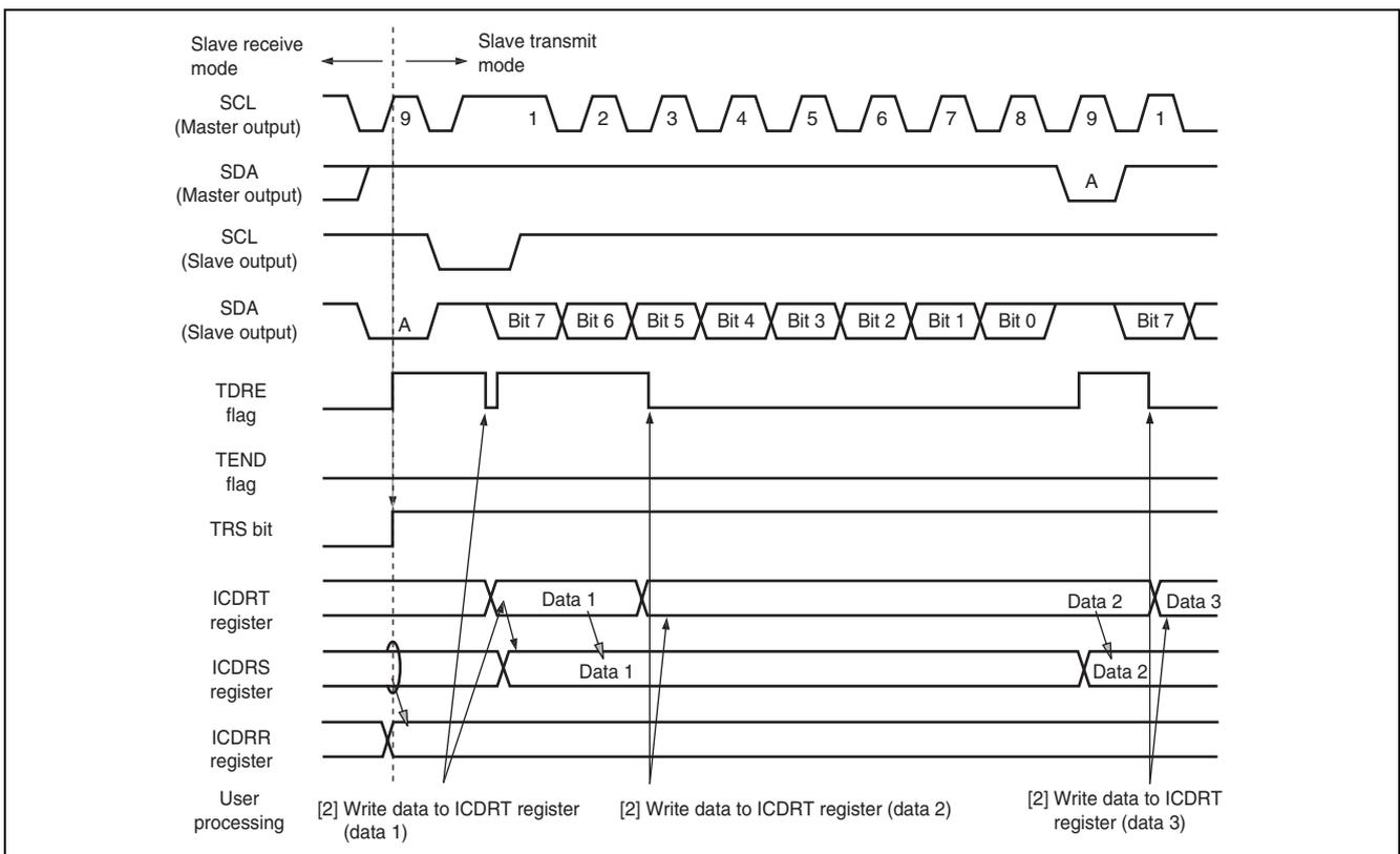
Figure 25.9 Slave Transmit Mode Operation Timing (1)
