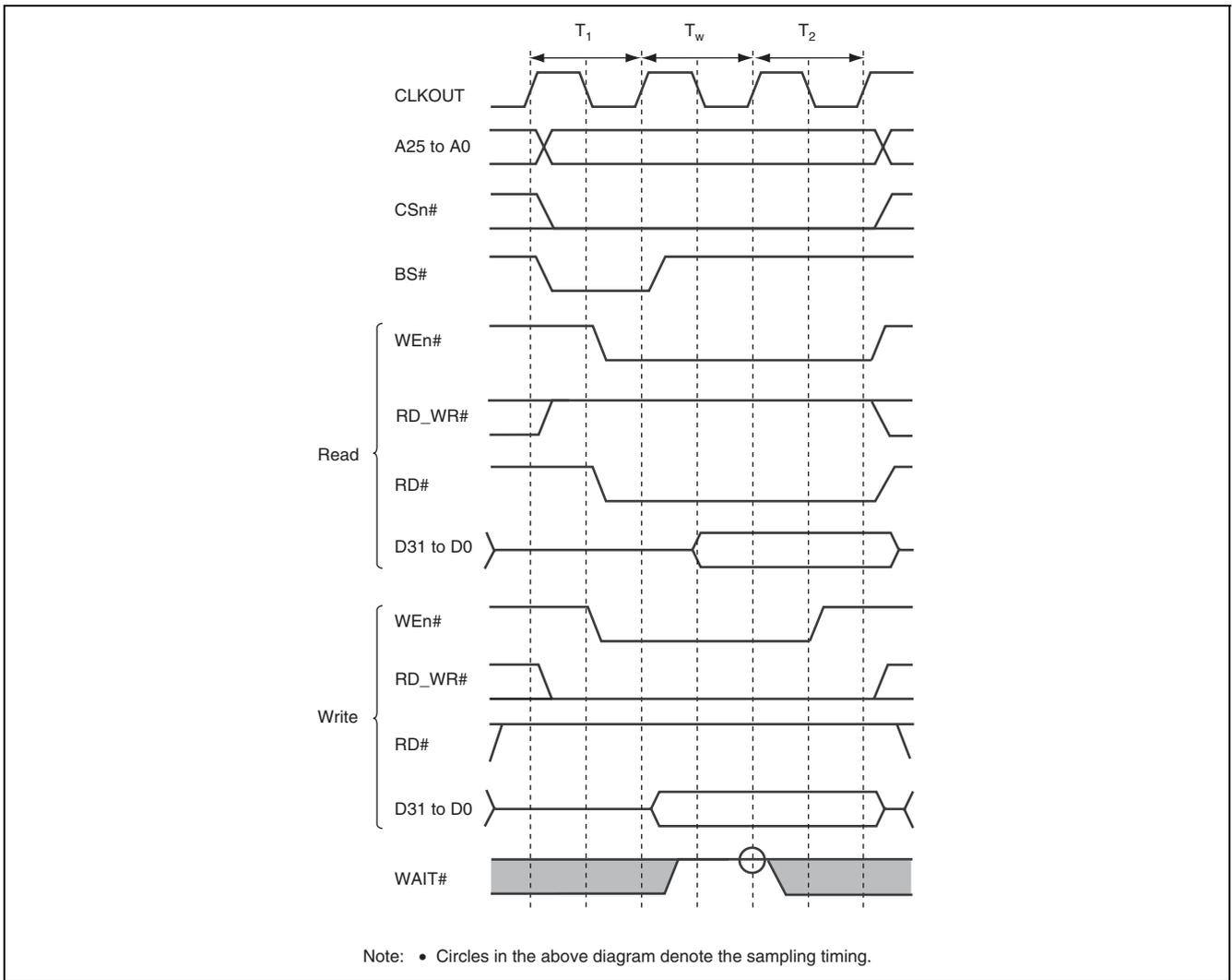
**Figure 19.13 Byte Control SRAM Basic Access Timing (One Internal Wait Cycle)**
