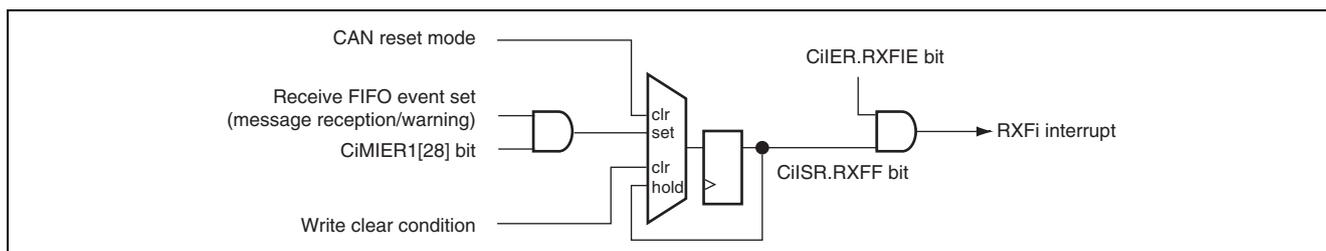
**Figure 26.24 Block Diagram of CAN<sub>i</sub> Receive FIFO Interrupt [RXFi]**
