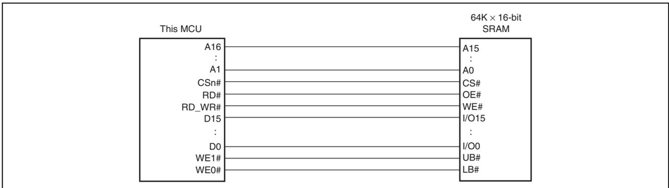
Figure 19.11 16-Bit Data Width Byte Control SRAM Connection Example
