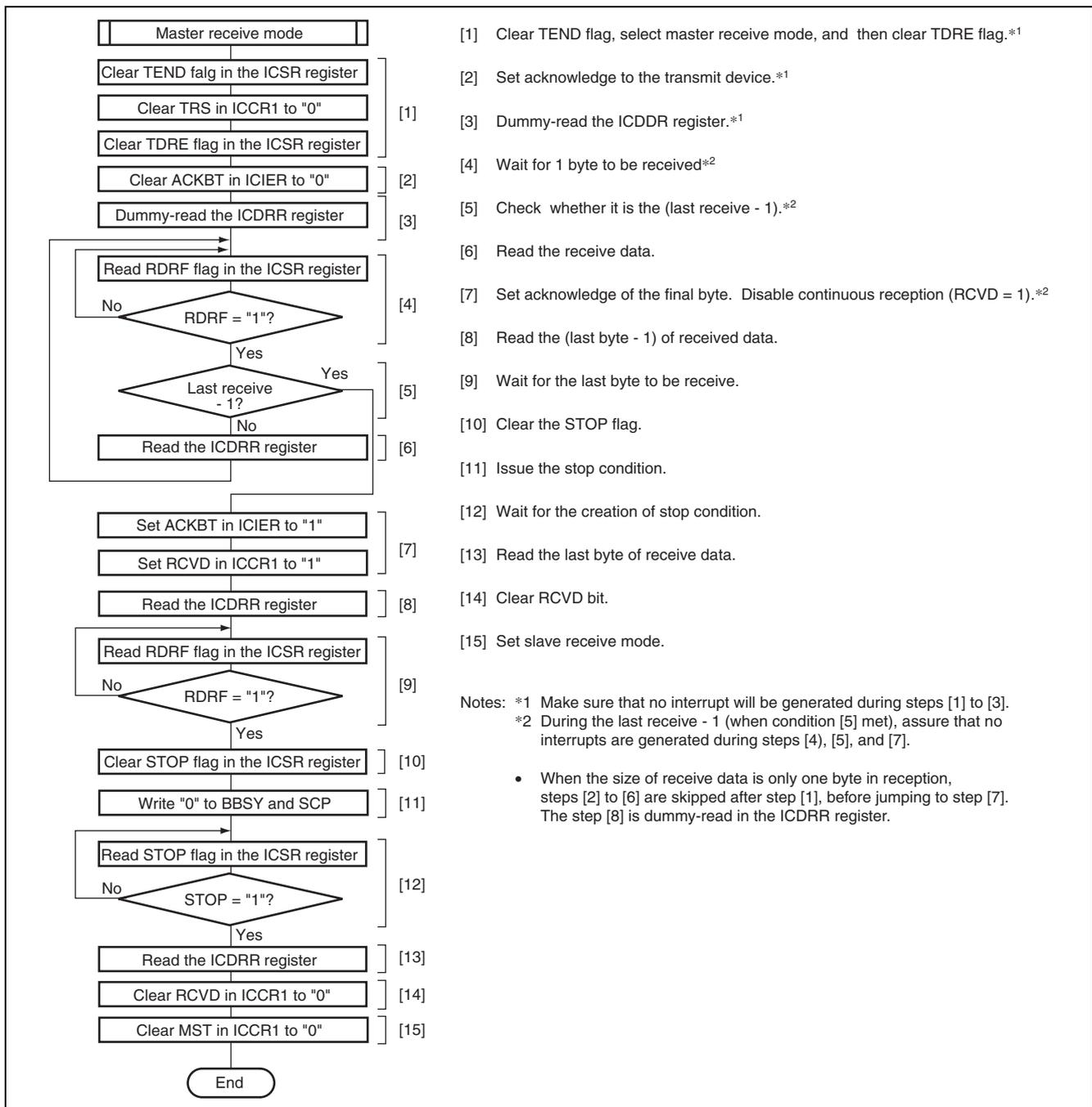
Figure 25.20 Sample Flowchart for Master Receive Mode
