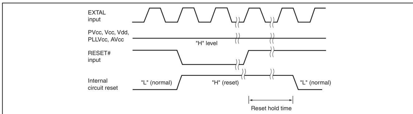
Figure 16.3 Reset During MCU Operation
