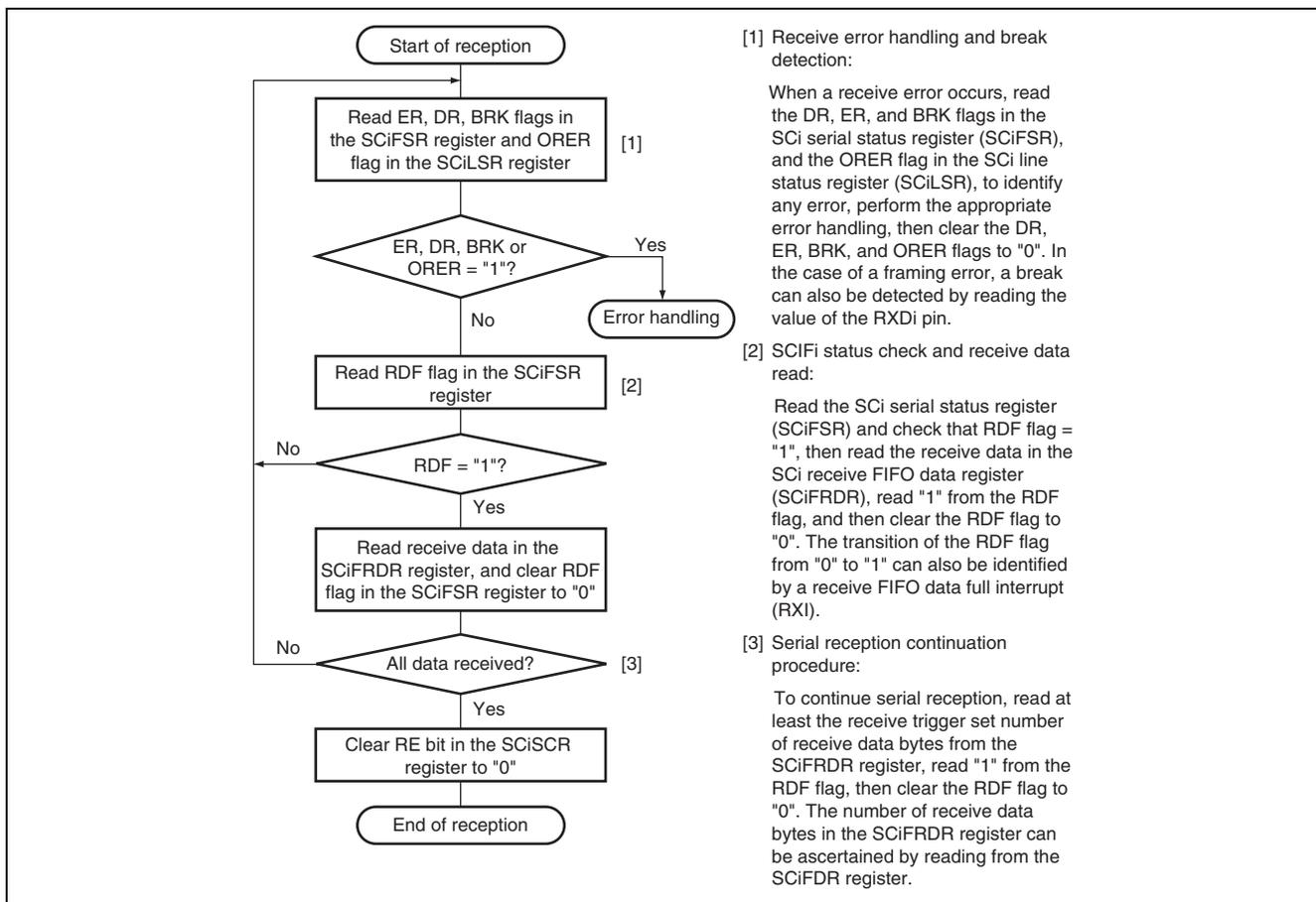
Figure 23.7 Sample Flowchart for Receiving Serial Data (1)
