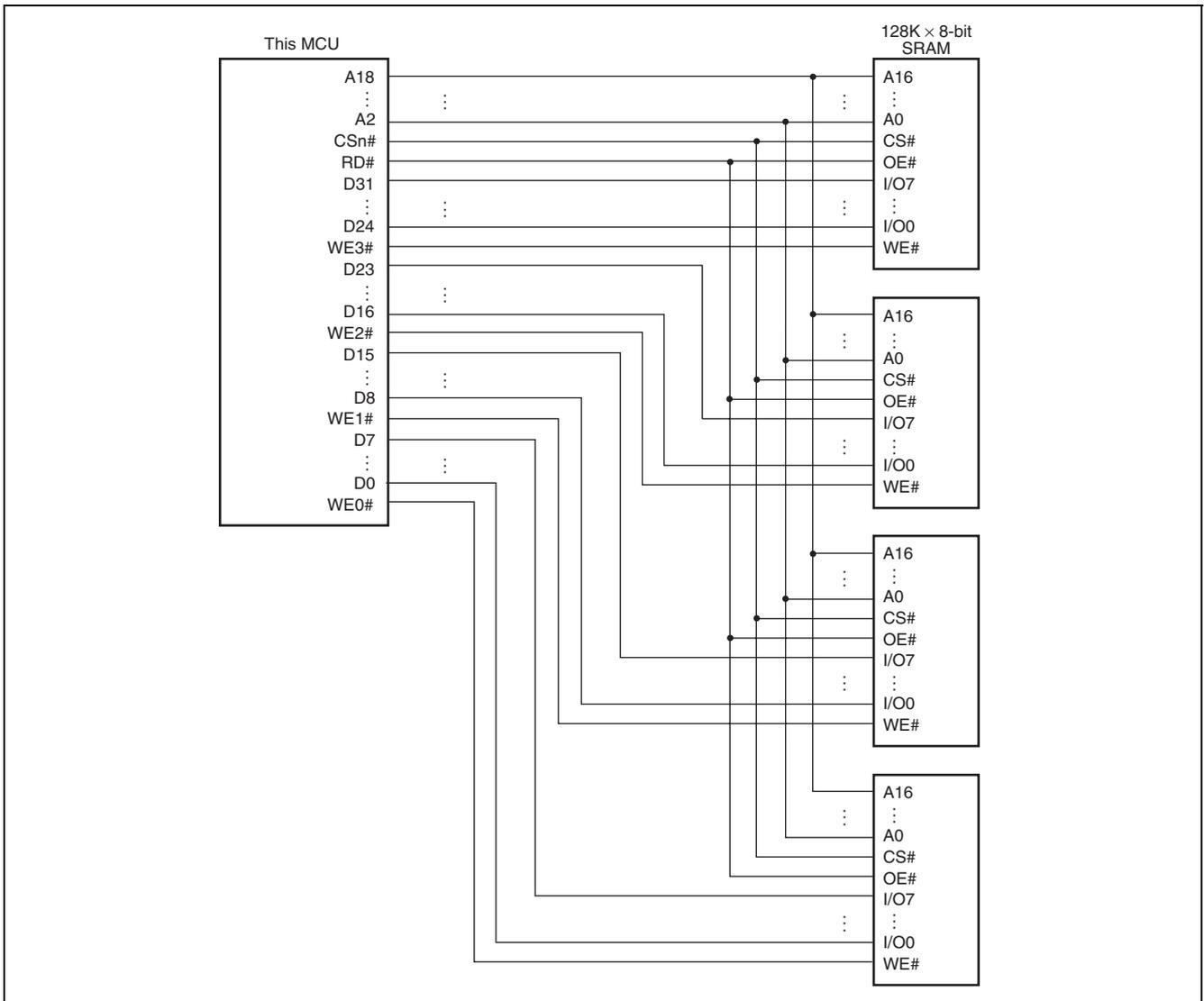
**Figure 19.4 Example of 32-Bit Data-Width SRAM Connection**
