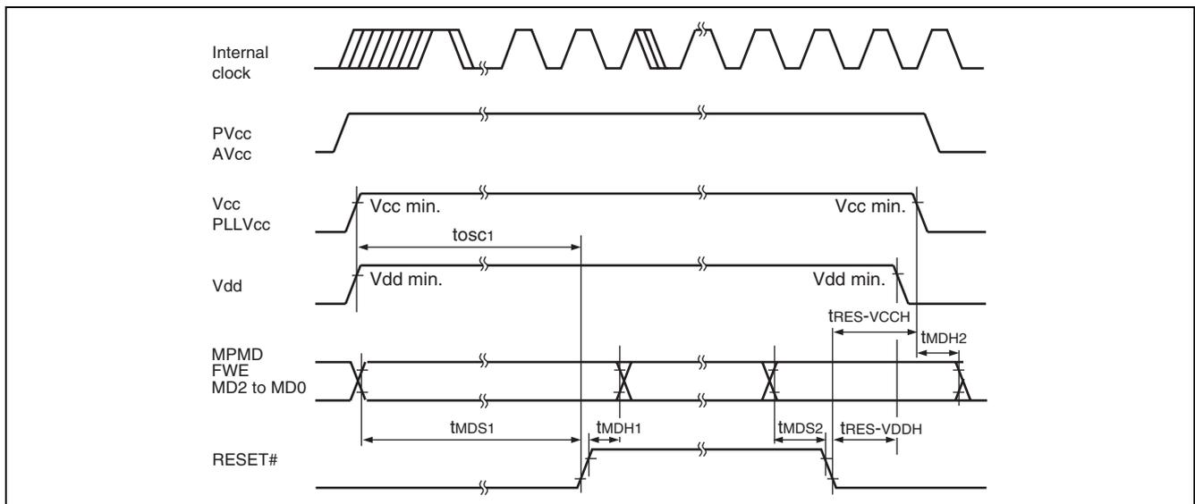
**Figure 38.5 Operation Mode and Oscillation Timing at Power-On/Off**
