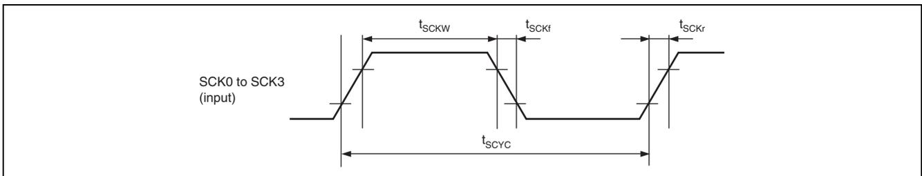
**Figure 38.25 SCK Input Timing**
