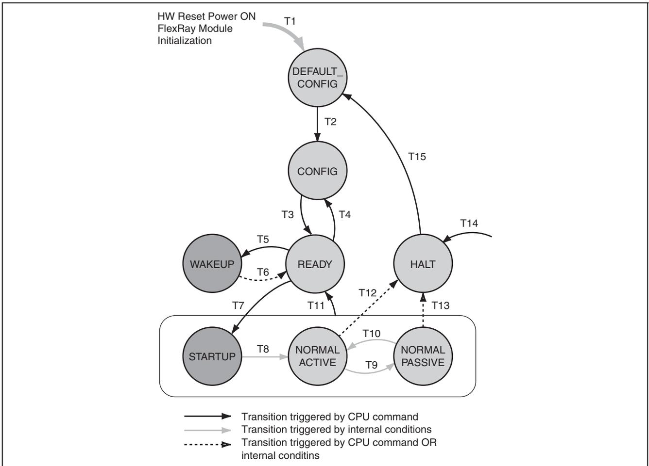
**Figure 32.6 Overall State Diagram of FlexRay Communication Controller**
