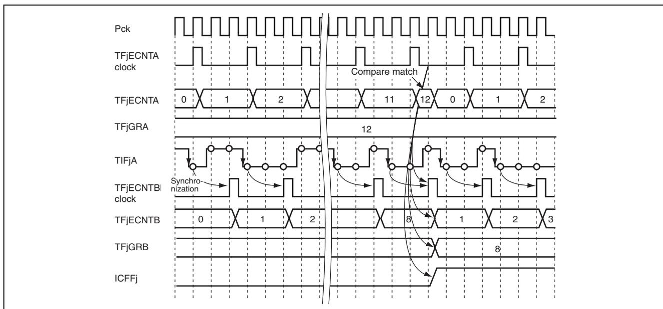
**Figure 21.15 Operation Example of Edge Count in Given Time
