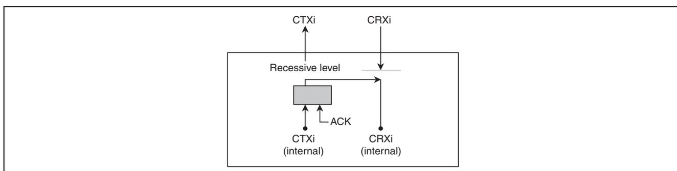
**Figure 26.8 Connection when Self-Test Mode 1 is Selected**
