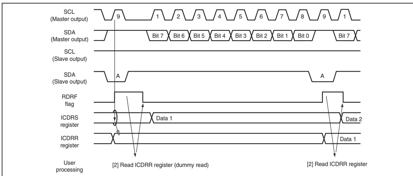
**Figure 25.11 Slave Receive Mode Operation Timing (1)**
