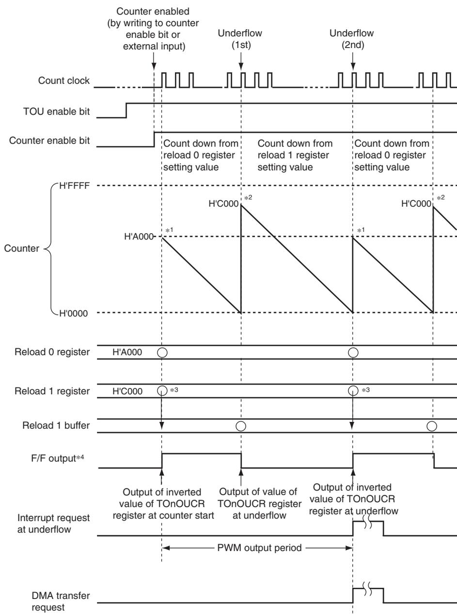
Figure 21.28 Operation Example of PWM Output Mode
