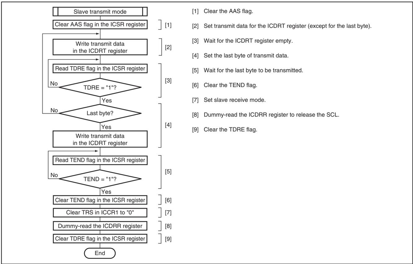
Figure 25.21 Sample Flowchart for Slave Transmit Mode
