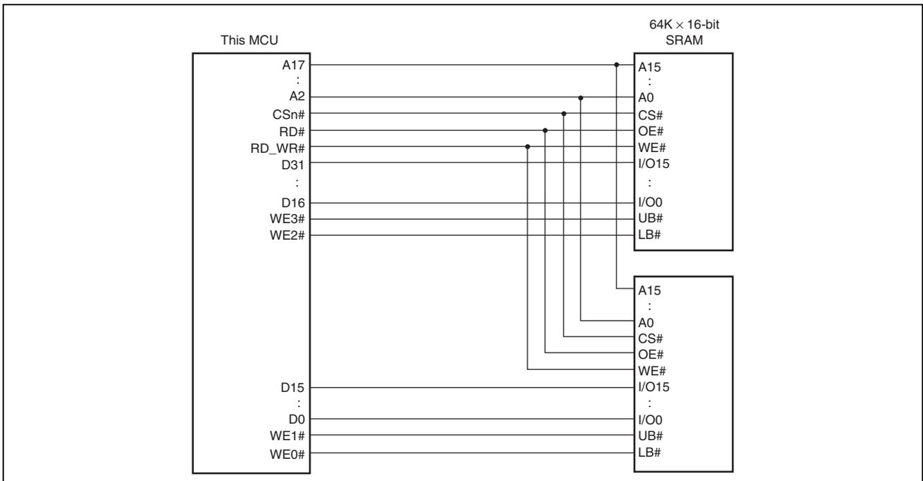
Figure 19.10 32-Bit Data Width Byte Control SRAM Connection Example
