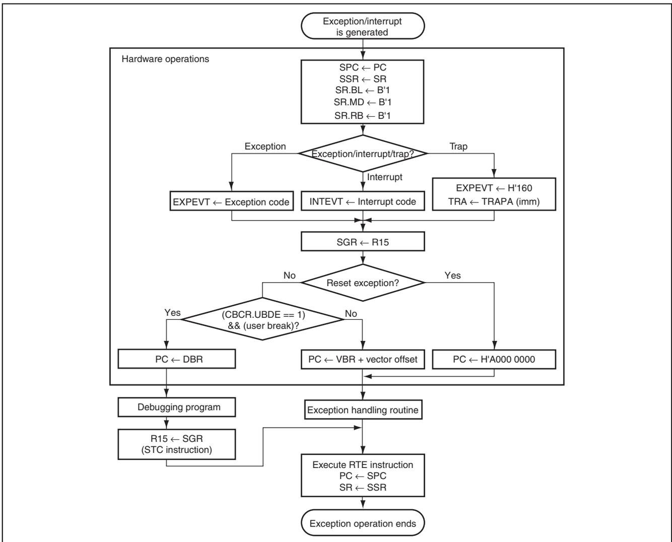
Figure 35.2 Flowchart of User Break Debugging Support Function
