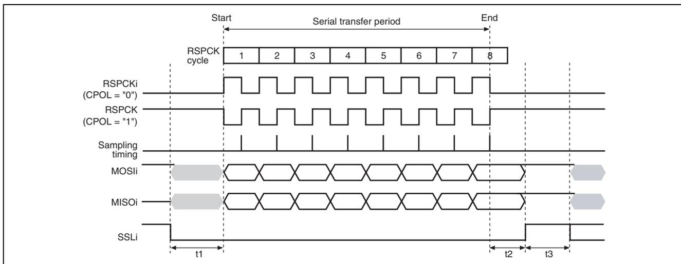
Figure 24.12 RSPI Transfer Format (CPHA = "1")
