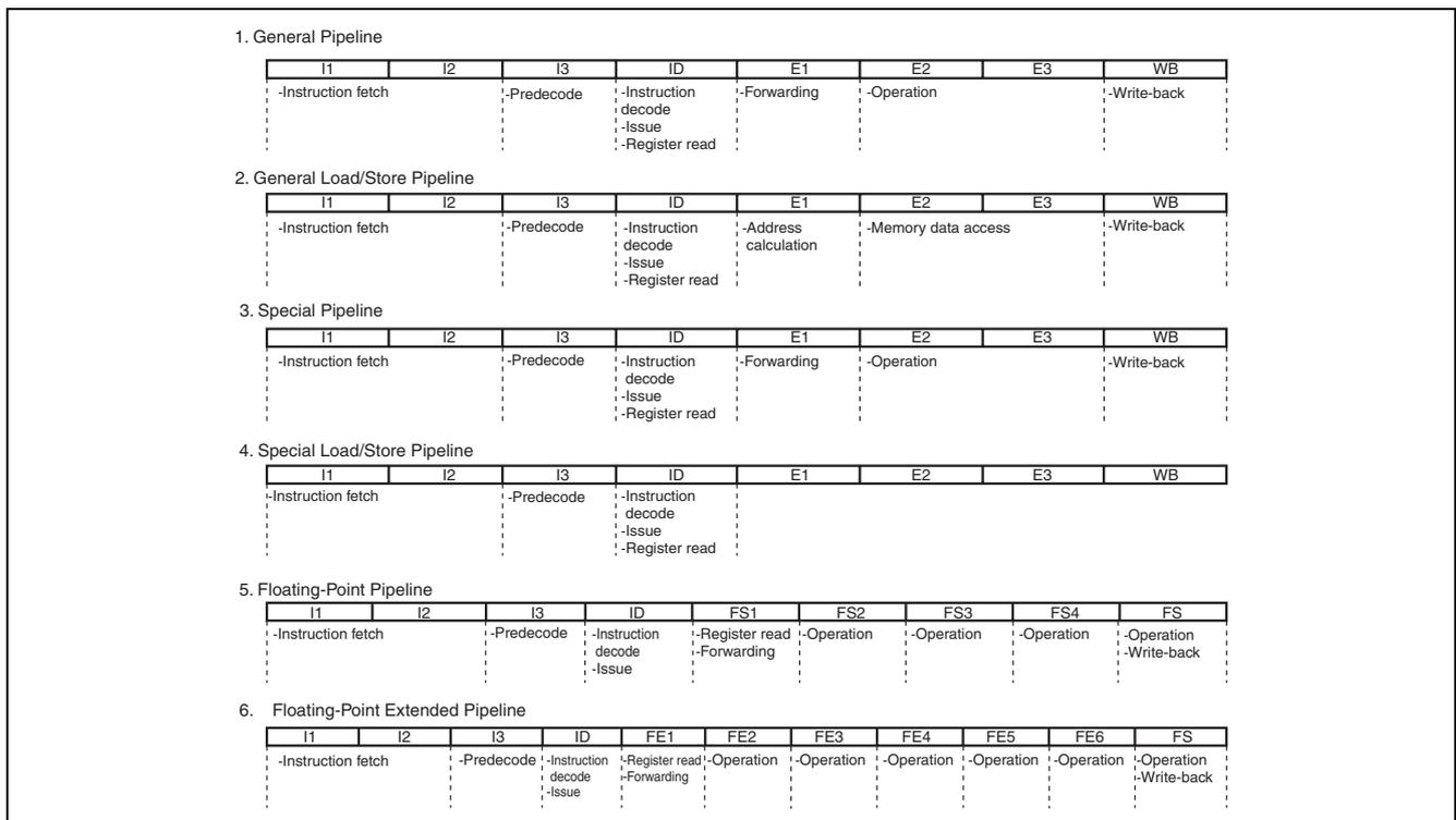
**Figure 4.1 Basic Pipelines**
