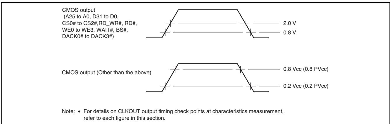
**Figure 38.3 Output Timing Check Points at Characteristics Measurement**
