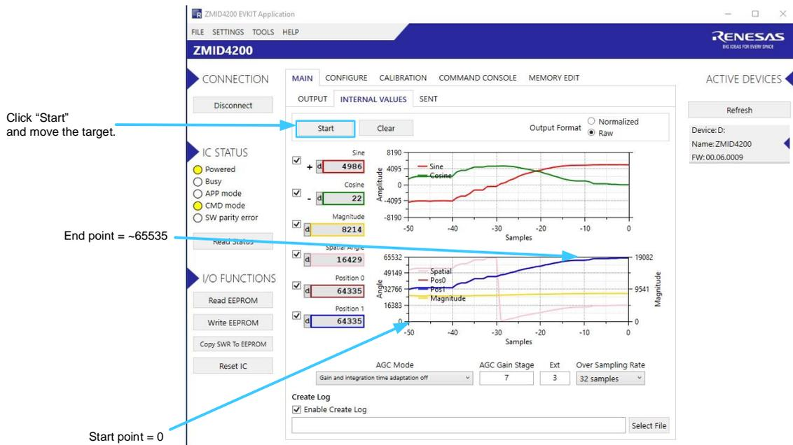
Figure 14. Output Calibration Verification
