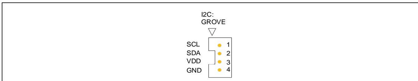
**Figure 5-3 Pin Assignments of the Grove Connector**
