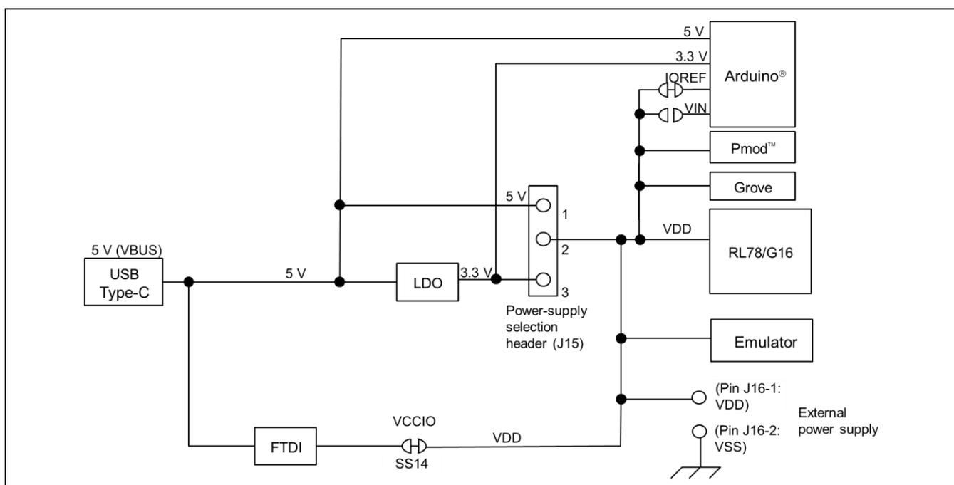
**Figure 6-2 Block Diagram of the Power-Supply Circuit**
