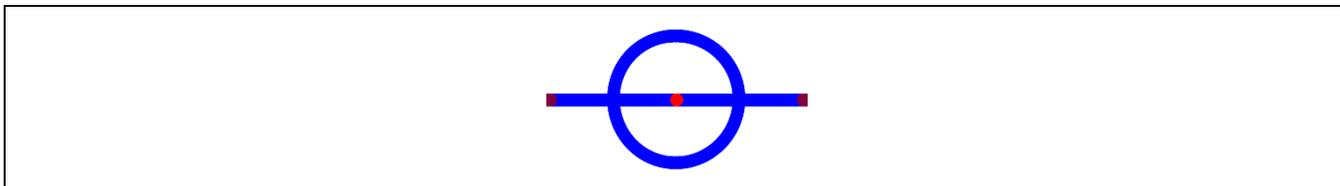
In the circuit schematics, the symbol below indicates that there are only short-circuit pads without any pattern for cutting.
