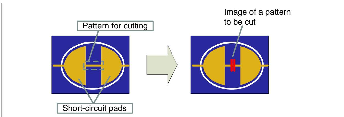
Figure 6-1 Pattern for Cutting and Short-circuit Pads
