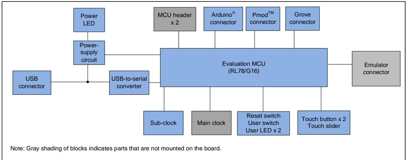
**Figure 1-1 Block Diagram**
