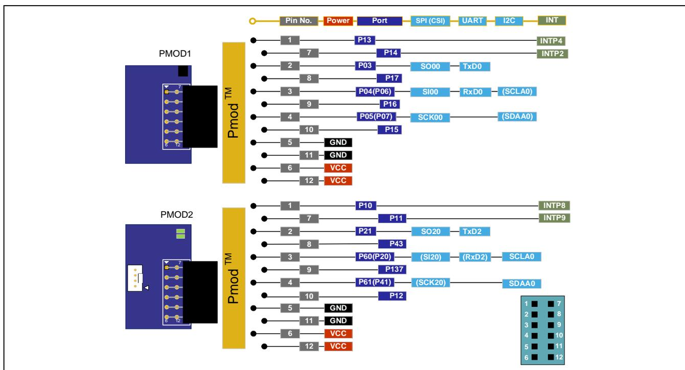
Figure 5-2 Pin Assignments of the Pmod™ Connectors
