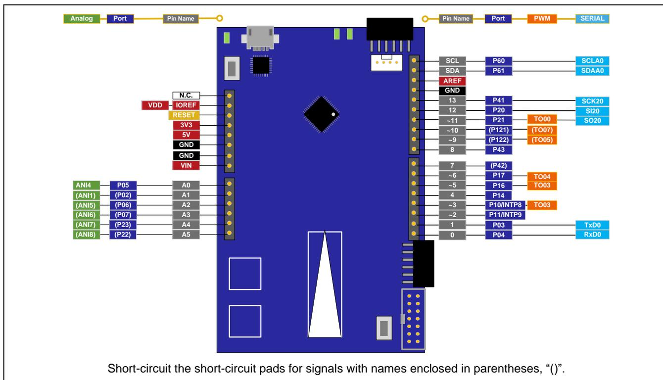
Figure 5-1 Pin Assignments of the Arduino® Connectors
