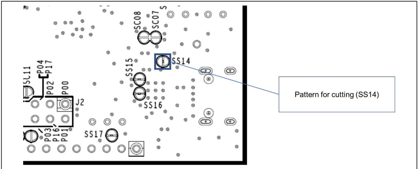
Figure 5-11 Position of the Pattern for Cutting (SS14)
