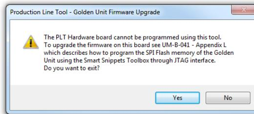
Figure 92. GU FW Upgrade - hardware version compatibility
