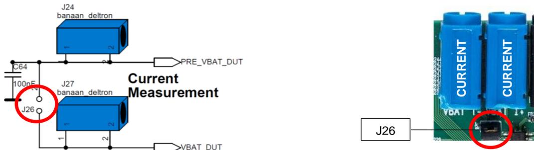
**Figure 12. Connections for "Floating Current" measurements**
