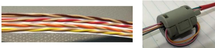
**Figure 120. Example of twisted pair cable with 4 pairs and ferrite**
