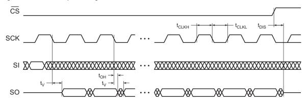
Figure 15-3. WP Timing for Write Status Register Byte 1 Command When SPRL = 1
