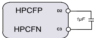
Figure 39: Charge Pump Flying Capacitor
