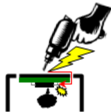
Figure 5-2 Cases where static electricity sneaks from the gap of the cover panel
