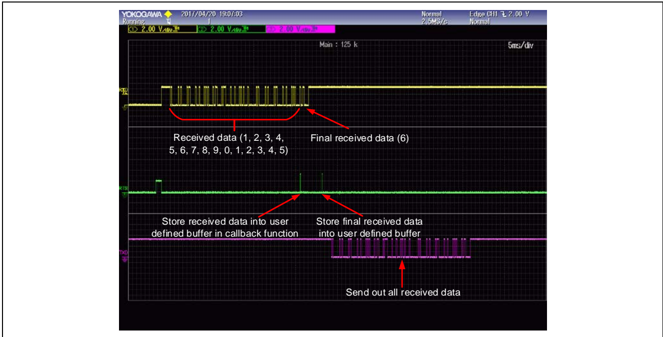
Figure 11. UART0 Waveform (not using semi-hosting)
