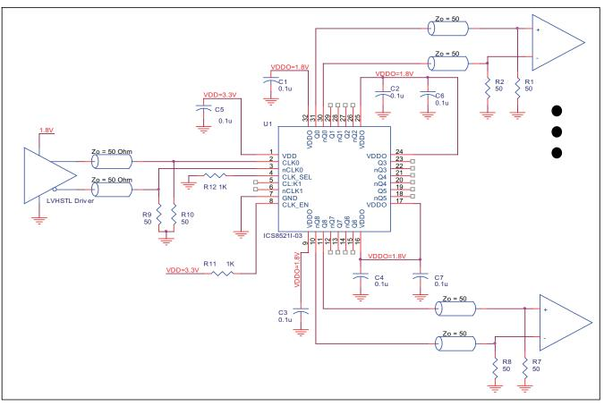
FIGURE 3B. RECOMMENDED LAYOUT OF BYPASS CAPACITOR PLACEMENT
