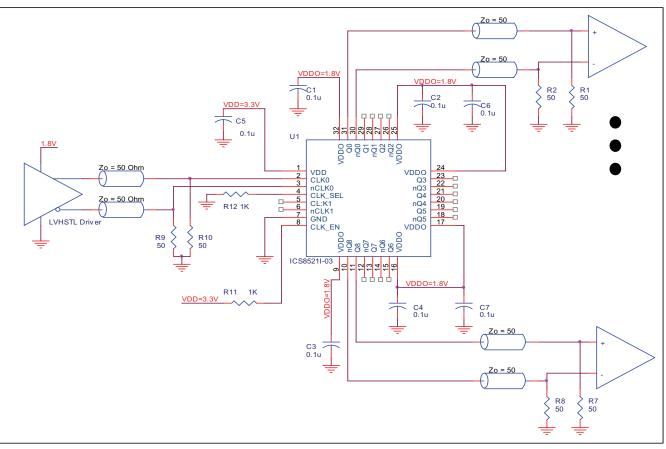
FIGURE 3A. 8521-03 SCHEMATIC EXAMPLE
