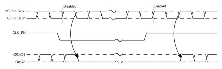
FIGURE 1. CLK\_EN TIMING DIAGRAM
