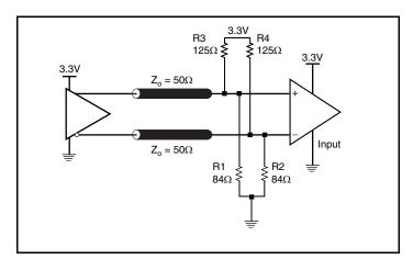
Figure 4B. 3.3V LVPECL Output Termination
