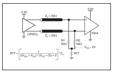
Figure 4A. 3.3V LVPECL Output Termination
