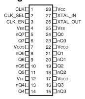
28-Lead TSSOP, 173MIL 4.4mm x 9.7mm x 0.925mm package body G Package Top View
