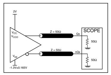
3.3/3.3V LVPECL Output Load AC Test Circuit
