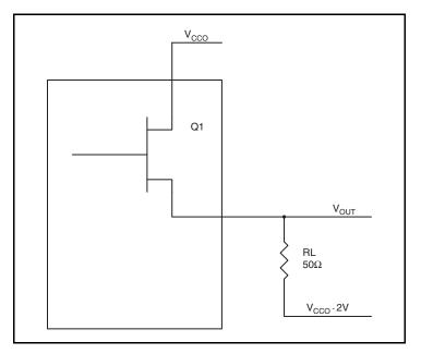
Figure 5. LVPECL Driver Circuit and Termination
