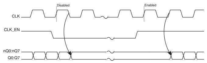
Figure 1. CLK\_EN Timing Diagram
