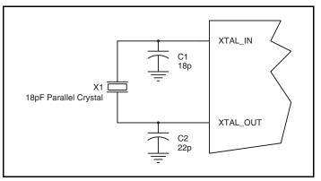
Figure 2. Crystal Input Interface
