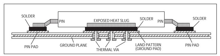
Figure 3. Assembly for Exposed Pad Thermal Release Path - Side View (drawing not to scale)
