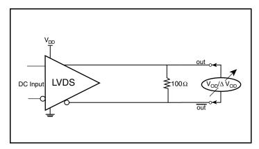
**Differential Output Voltage Setup**
