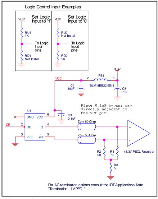
Figure 3. IDT8N3S271 Schematic Example
