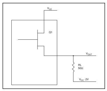
Figure 4. LVPECL Driver Circuit and Termination
