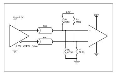
Figure 2A. 2.5V LVPECL Driver Termination Example
