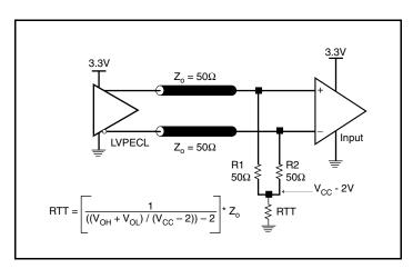
Figure 1A. 3.3V LVPECL Output Termination
