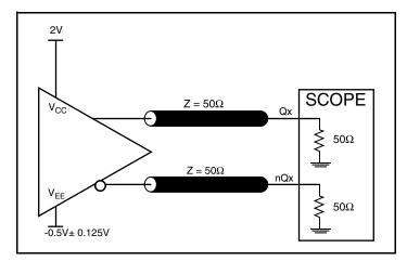
2.5V LVPECL Output Load Test Circuit
