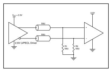
Figure 2C. 2.5V LVPECL Driver Termination Example
