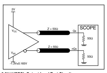
3.3V LVPECL Output Load Test Circuit
