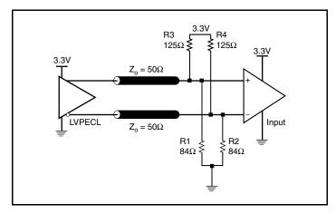
Figure 1B. 3.3V LVPECL Output Termination
