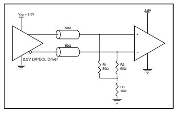
Figure 2B. 2.5V LVPECL Driver Termination Example
