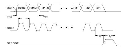
Figure 2. Timing Diagram for Programming the MK1716-01
