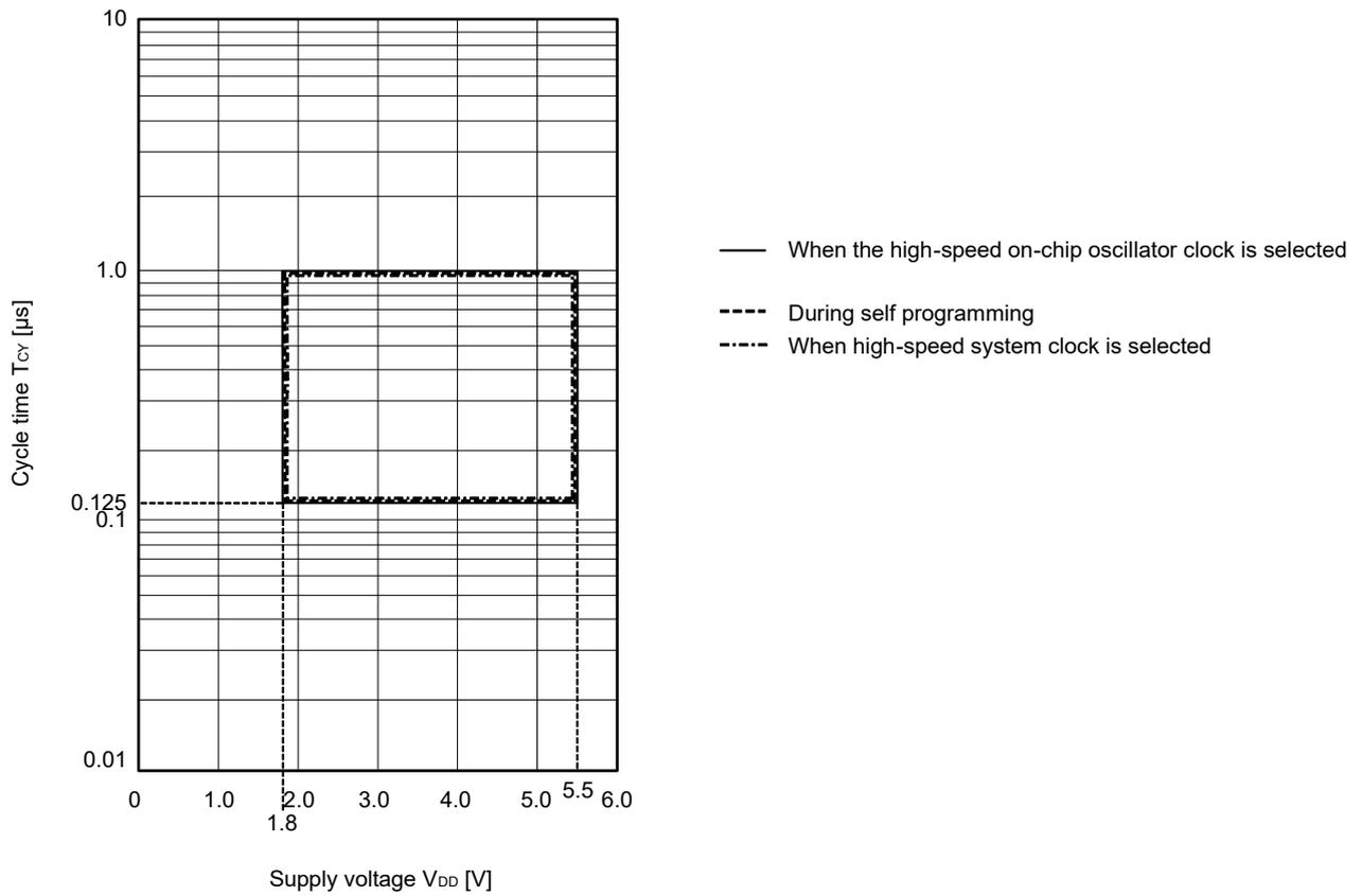
T<sub>CY</sub> vs V<sub>DD</sub> (LV (low-voltage main) mode)
