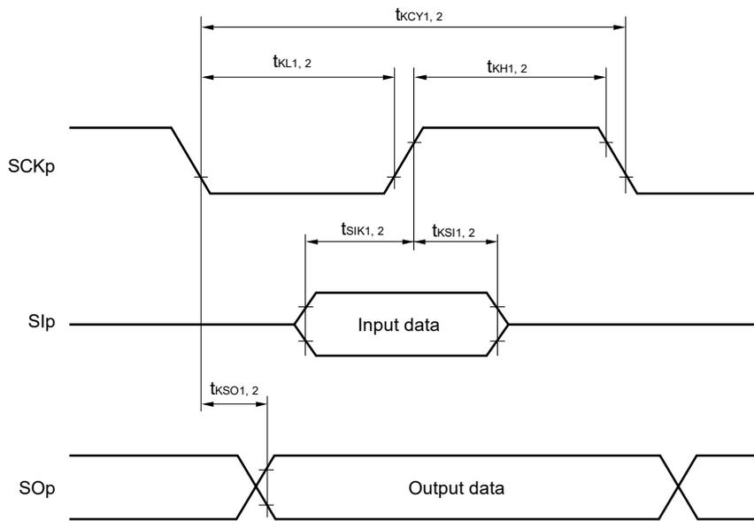
**Simplified SPI (CSI) mode serial transfer timing (during communication at same potential)
