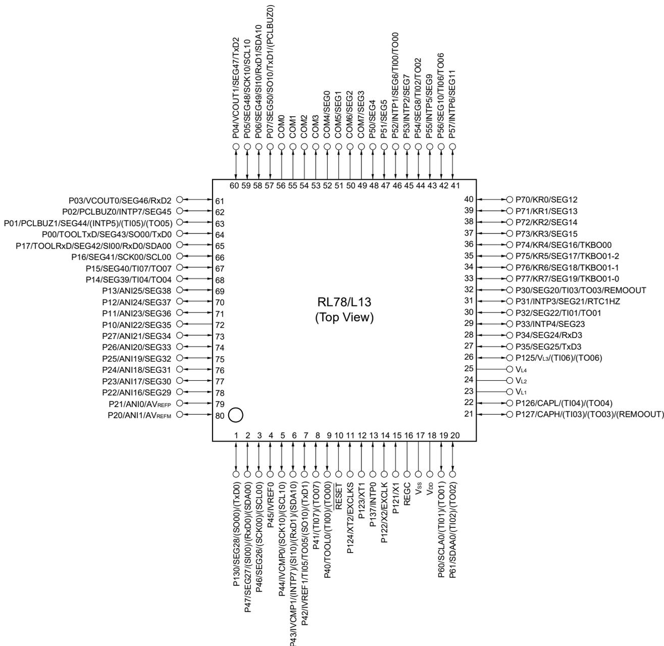
**Caution** Connect the REGC pin to V<sub>SS</sub> via a capacitor (0.47 to 1 μF).
