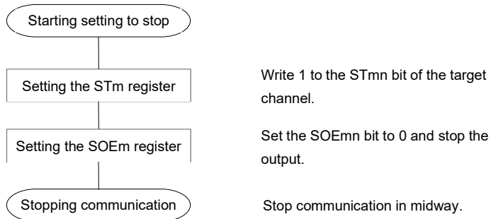
Figure 15-123. Procedure for Stopping UART Transmission
