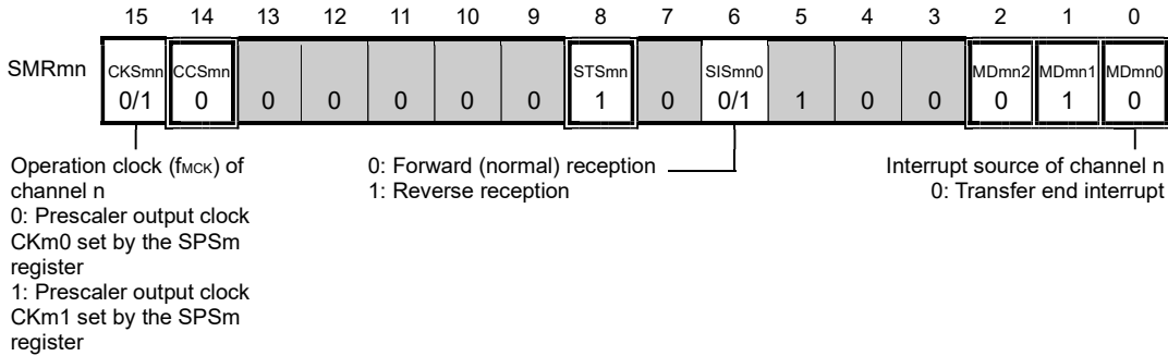
Figure 15-129. Example of Contents of Registers for UART Reception of UART (UART0, UART1) (1/2)
