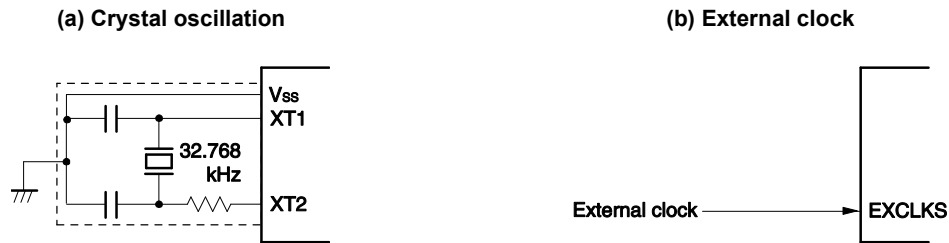
Figure 5-24. Example of External Circuit of XT1 Oscillator
