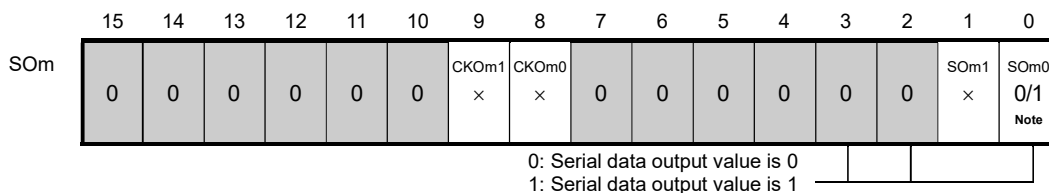
Figure 15-121. Example of Contents of Registers for UART Transmission of UART (UART0, UART1) (2/2)
