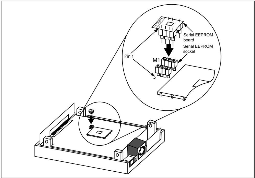
Figure 7.6 Installing Serial EEPROM Board
