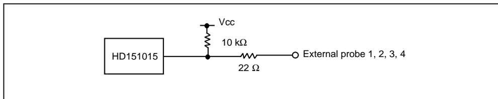
**Figure 2.8 Interface Circuit for External Probe 1**
