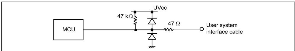
Figure 7.1 Default User System Interface Circuit
