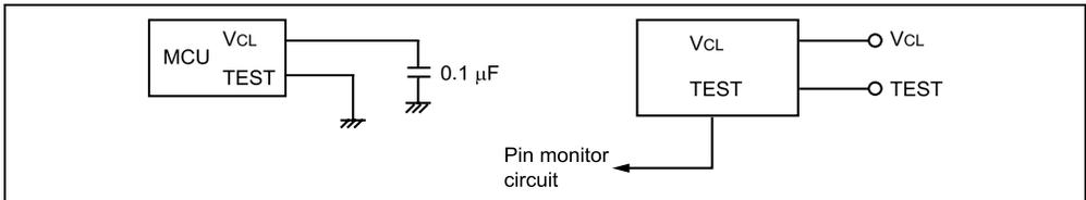
**Figure 7.4 V<sub>CL</sub> and TEST System Interface Circuit**
