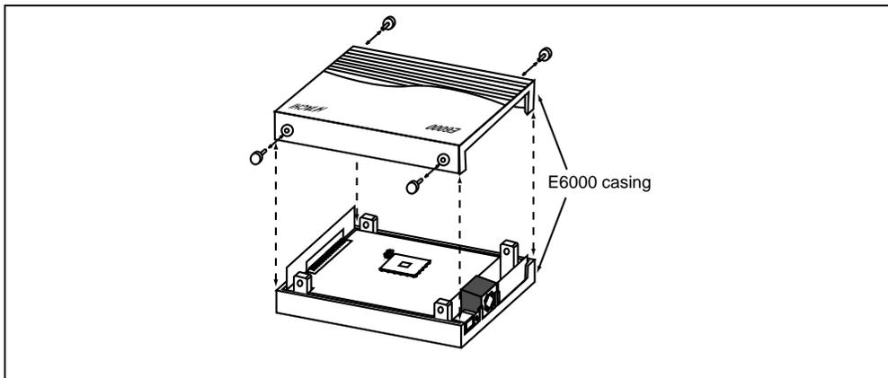
**Figure 7.5 Removing and Fastening the Emulator Cover**
