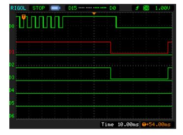
Figure 5. Single Wire functionality waveform
