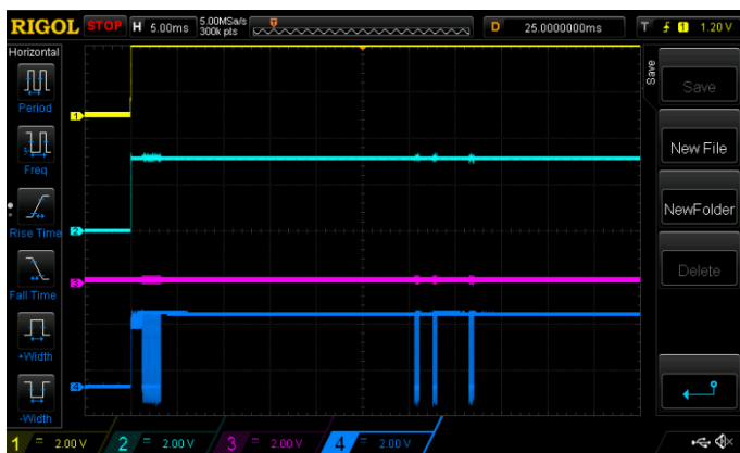
Figure 8. Nikon (immediate only) shutter release pattern
