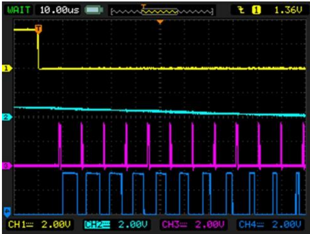
Figure 8. PWM generator turns on
