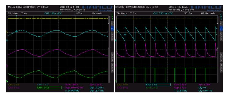
Figure 14. Fast Level Shifter operations. Period of Input signal is 42 ns. Propagation delay time creates effect of phase shift for 180 degrees. The delay time effect is VDD dependent.
