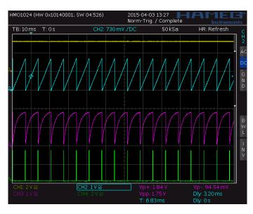
Figure 17. Maximum rising edge ramp rates on differentiator input.
