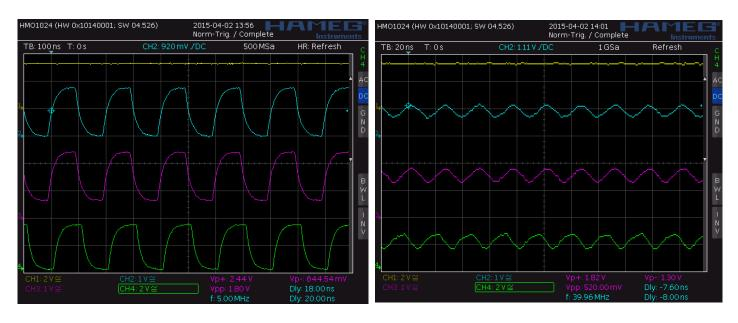
Figure 13. Fast Level Shifter operation. Input signal period is 200 ns (5 MHz). Waveform is limited by oscilloscope probes and parasitic capacitances. Also, pin-to-pin propagation delay influence is visible.
