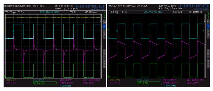
Figure 9. Fast Level Shifter operation. Period of Input signal is 50 ms
