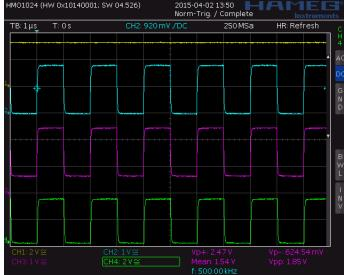
Figure 12. Fast Level Shifter operation. Period of Input signal is 2 us
