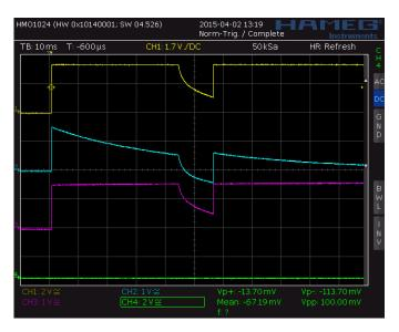
Figure 3. VDD is applied. Differentiator input is in Hi-Z state. LS\_OUT remains unchanged.
