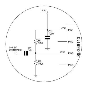
Figure 1. Fast Level Shifter schematic
