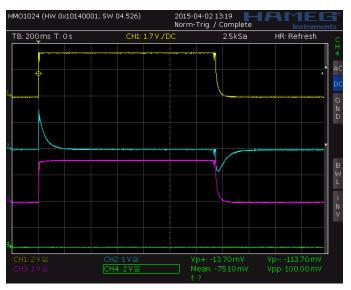
Figure 4 VDD is applied. Differentiator input is in Hi-Z state. LS\_OUT remains unchanged. Long timebase
