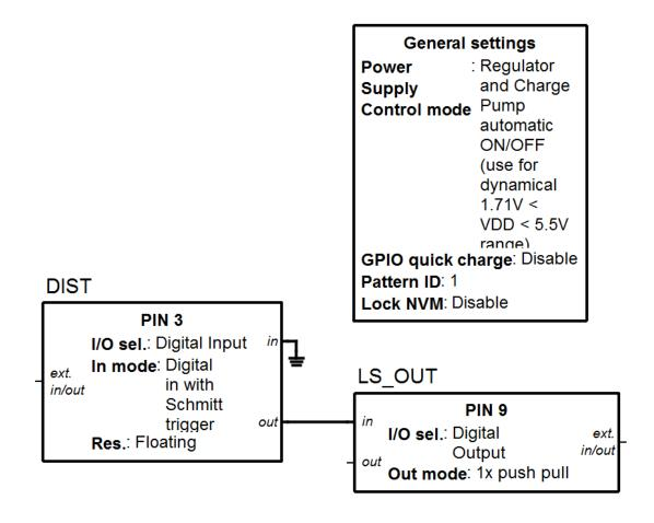
Figure 1.1. Block Diagram for Design
