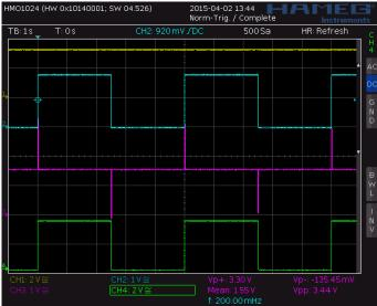
Figure 8. Fast Level Shifter operation. Period of Input signal is 5 seconds
