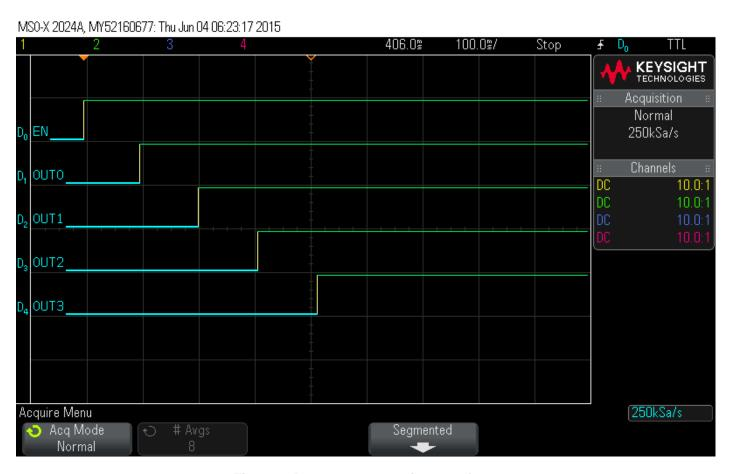
Figure 2. Power up sequencing waveform
