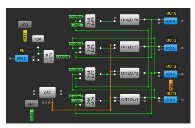
Figure 3. Power up and down sequencer block diagram
