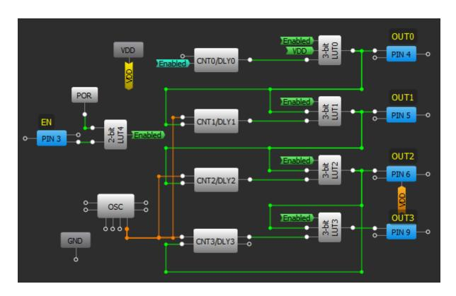
Figure 1. Power up sequencer block diagram
