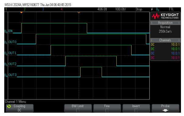
Figure 4. Power sequence up and down waveform
