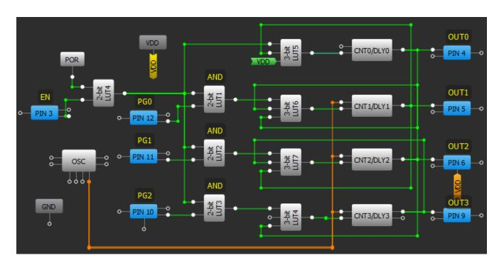
Figure 5. Power up and down sequencer with PG input block diagram
