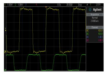
Figure 4. Level-Shift Response at 15MHz
