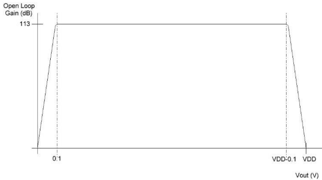
Figure 7. AOL vs VOUT Characteristics for SLG88102V
