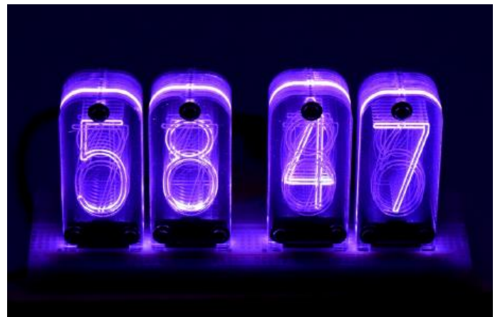
Figure 17. Four pseudo Nixie digits of a digital clock showing 58:47. These are mounted on a breadboard
