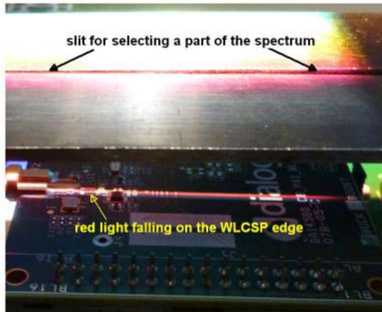
Figure 6: Dark red light falling on the WLCSP
