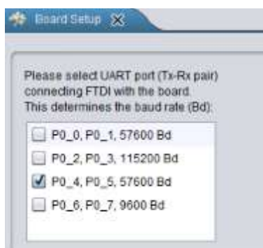
Figure 8: Board setup if UART is used
