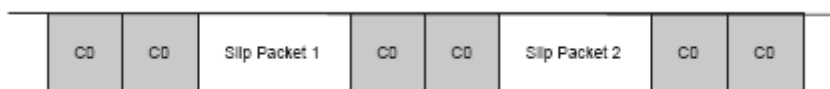
Figure 4-1 SLIP Packets with 0xC0 at the Start and End of Each Packet
