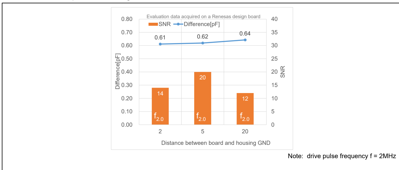
Figure 5-56 Board-Housing GND Distance and Sensitivity Characteristics
