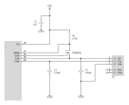
Figure 3. IO-Link Channel 0
