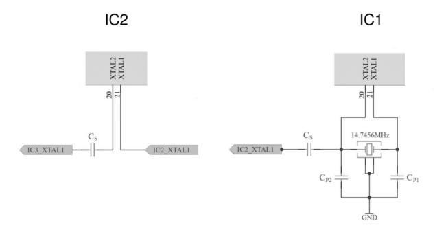
Figure 2. Crystal Oscillator Connection
