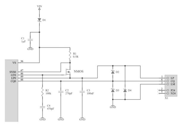
Figure 6. IO-Link Channel 0 Extended Circuitry
