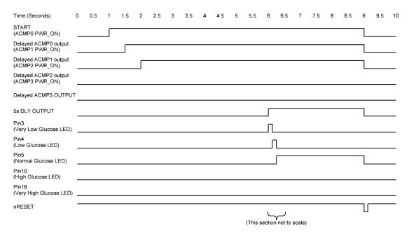
Figure 4: System signals when 300mv < ANALOG\_IN < 350mv
