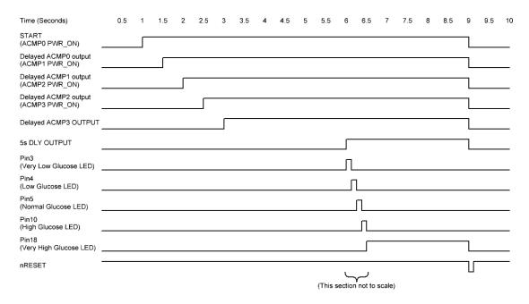
Figure 5: System Signals when ANALOG\_IN > 400 mv
