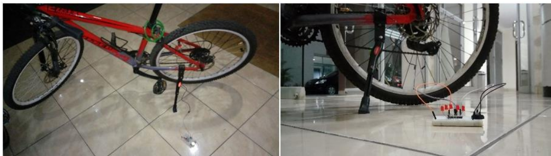
Figure 9: Magnet and Magnetic Switch Attached to Bicycle
