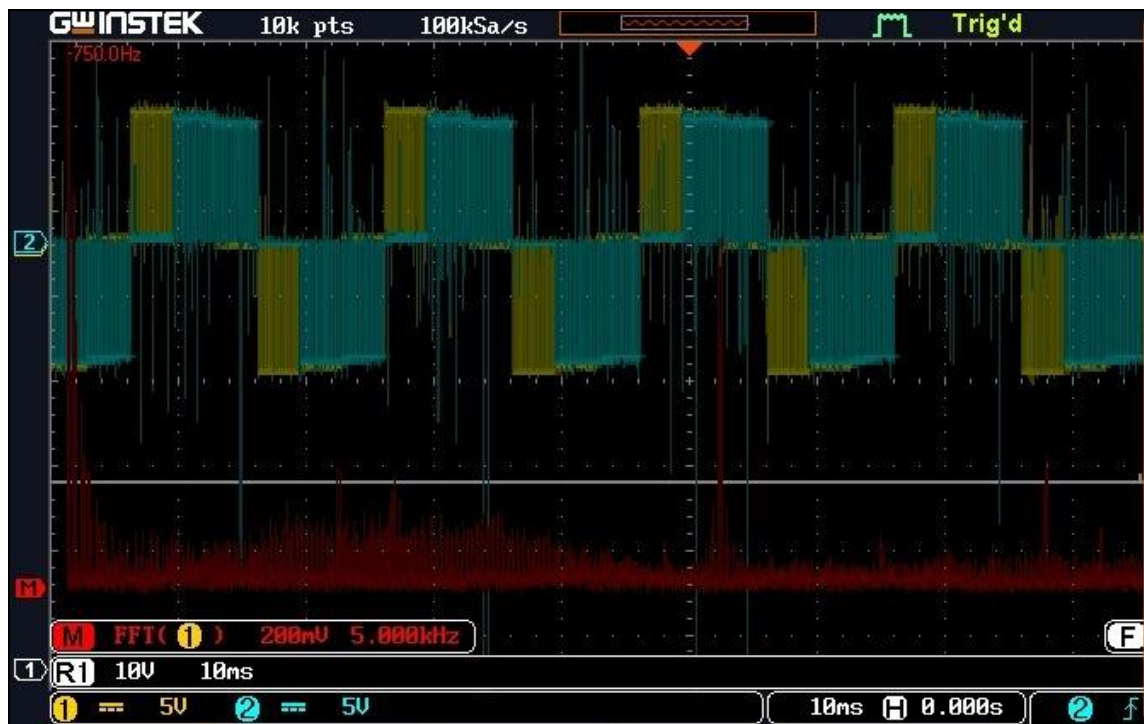
Figure 10: Vab, Vac and FFT for Reference Value 0.8
