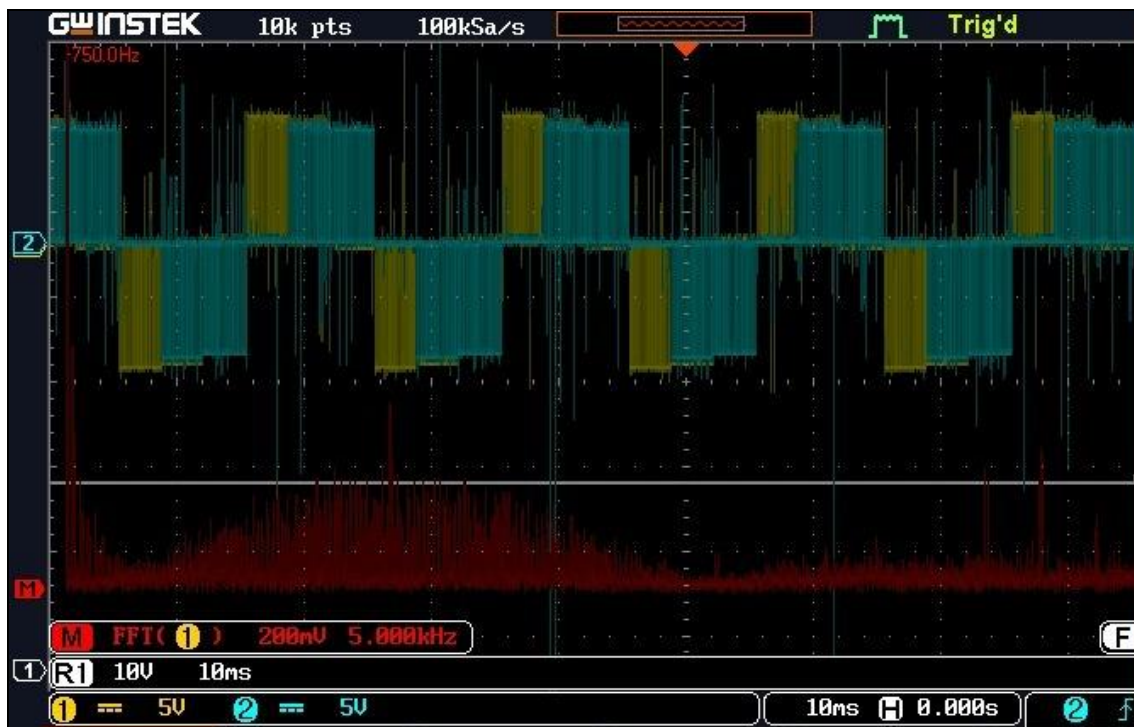
Figure 11: Vab, Vac and FFT for Reference Value 0.5
