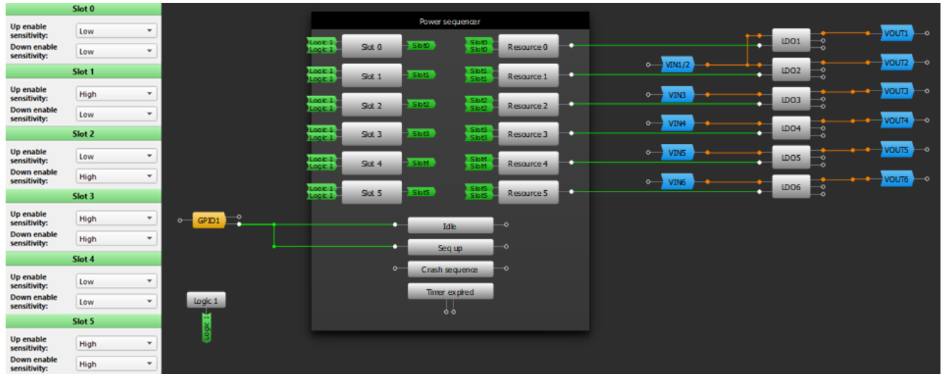
Figure 8: Power Sequencer triggered by GPIO with different up/down sensitivity settings
