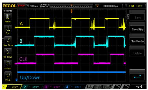
Figure 4: Timing Diagrams for Clockwise Encoder Rotation
