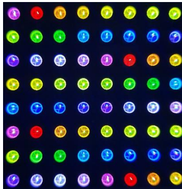
Figure 12. 8x8 LED Matrix, all LEDs ON After Sending the First Fragment of Data
