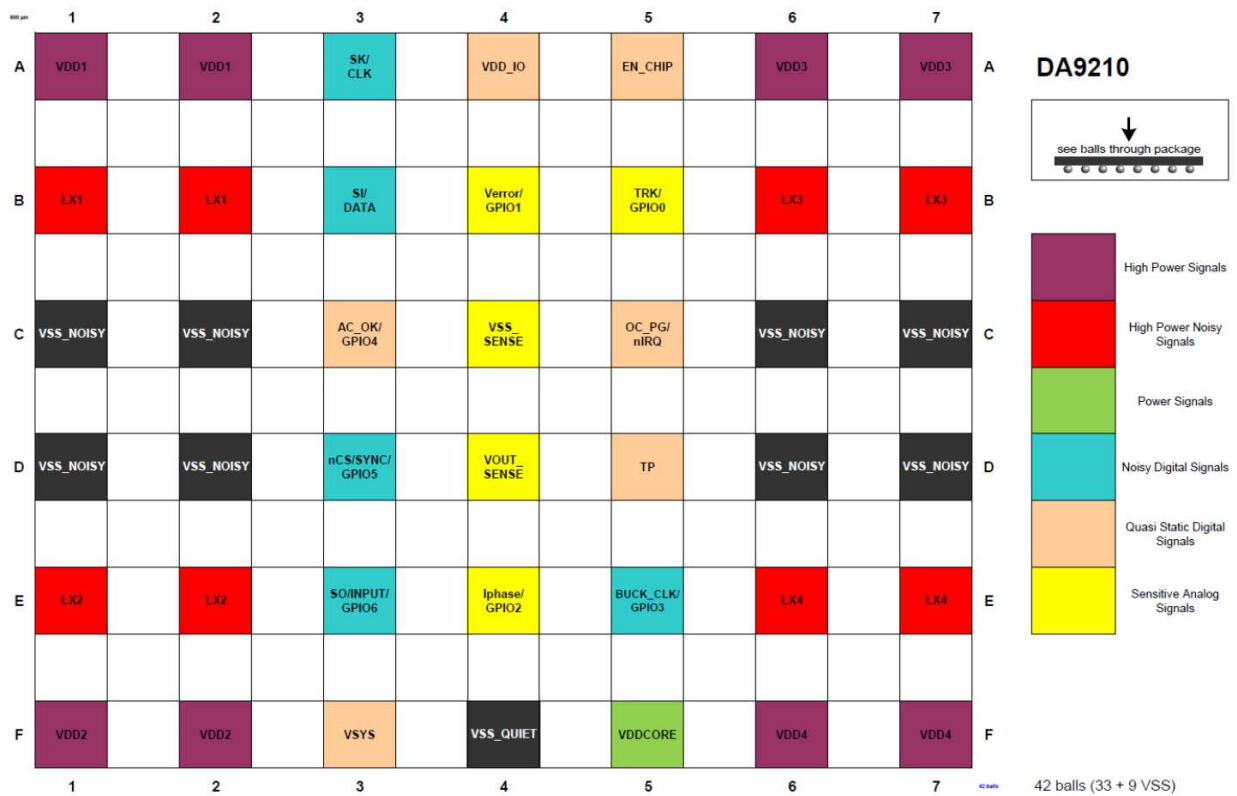
Figure 2: DA9210 42VF-BGA ball map
