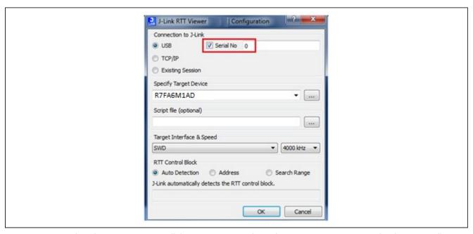
4. For parts other than Cortex-M33, click **OK**. For MCUs based on Cortex M33 Core, refer the Appendix.
