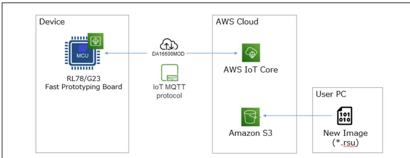
Figure 2-2 System Configuration of Demo Project (OTA)
