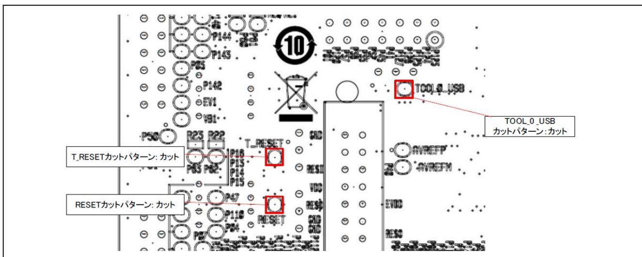
Figure 7-7 Settings for Using Emulator Connector (Solder Side)
