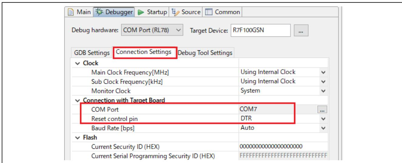
**Figure 8-4 Connection Settings for Using COM Port**
