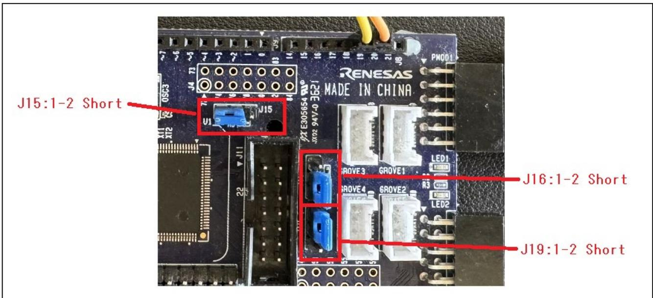
Figure 7-1 Settings for Using COM Port Debugging (Top Side)
