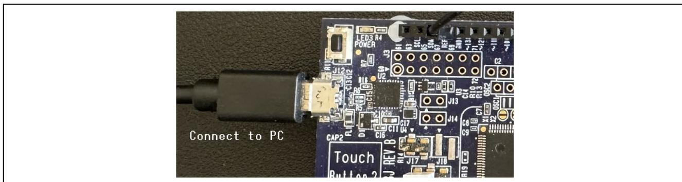
**Figure 4-6 Supplying Power to the MCU Board**
