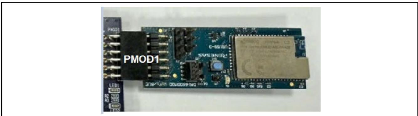
Figure 4-2 Connecting DA16600MOD to PMOD1 of the MCU Board
