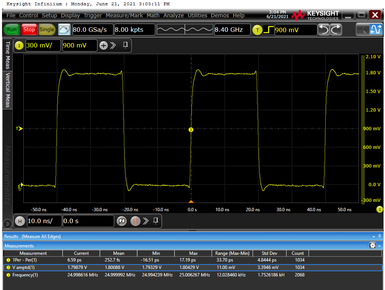
Figure 5. Typical 1.8V LVCMOS 25MHz Waveform at Receiver Side
