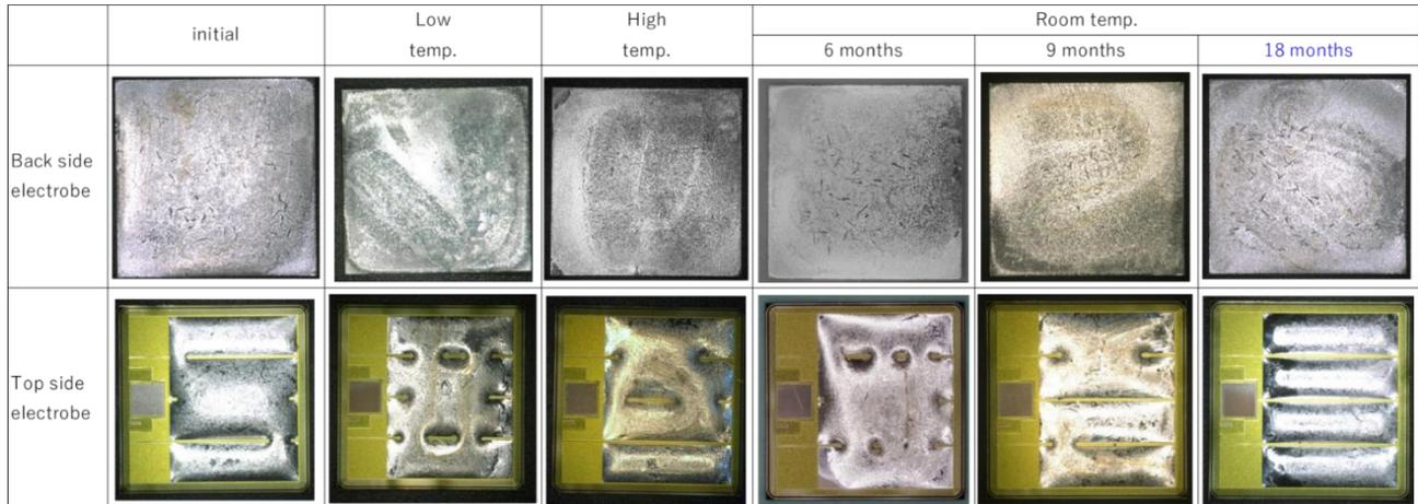
**Figure 4 Representative electrode photo after soldering**
