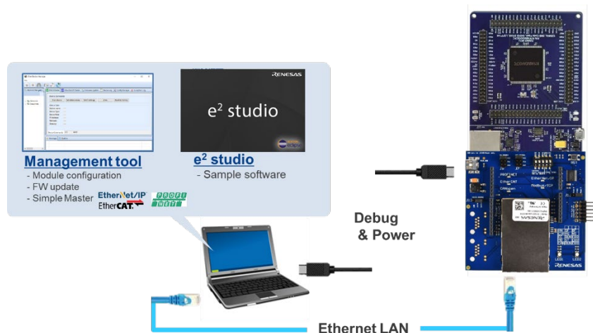
R-IN32M3 module adapter board configuration (ex: with EK-RA6M3)
