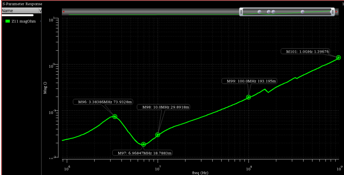
Figure 11: AVDD to AGND Path Impedance Including Capacitor
